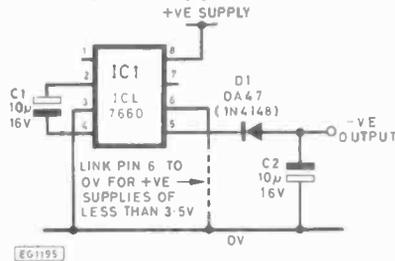
**Fig. 3 Basic voltage converter circuit. D1 is not necessary for supplies >6.5V. Include it if high temperatures are anticipated**
