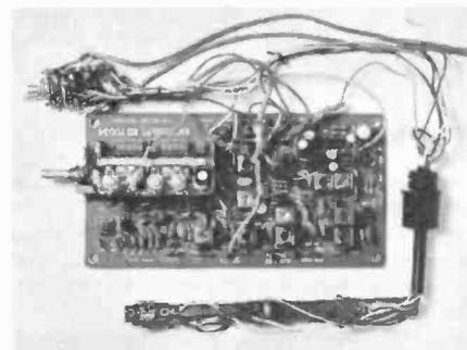
Connections for a tuning meter, stereo beacon and a.f.c. switch are provided. With the addition of a 12V supply and simple stereo amp this would make a high quality portable radio or it could form the heart of a hi-fi system, as it was originally intended to do in the EX222 receiver. The tuners are new and the price is £6, including VAT plus postage.
