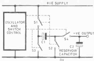
**Fig. 2 Principle of i.c. operation**
