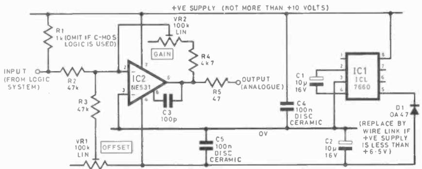
**Fig. 8 Logic level to analogue converter circuit**
