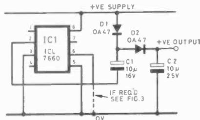
**Fig. 6 Positive voltage converter circuit**
