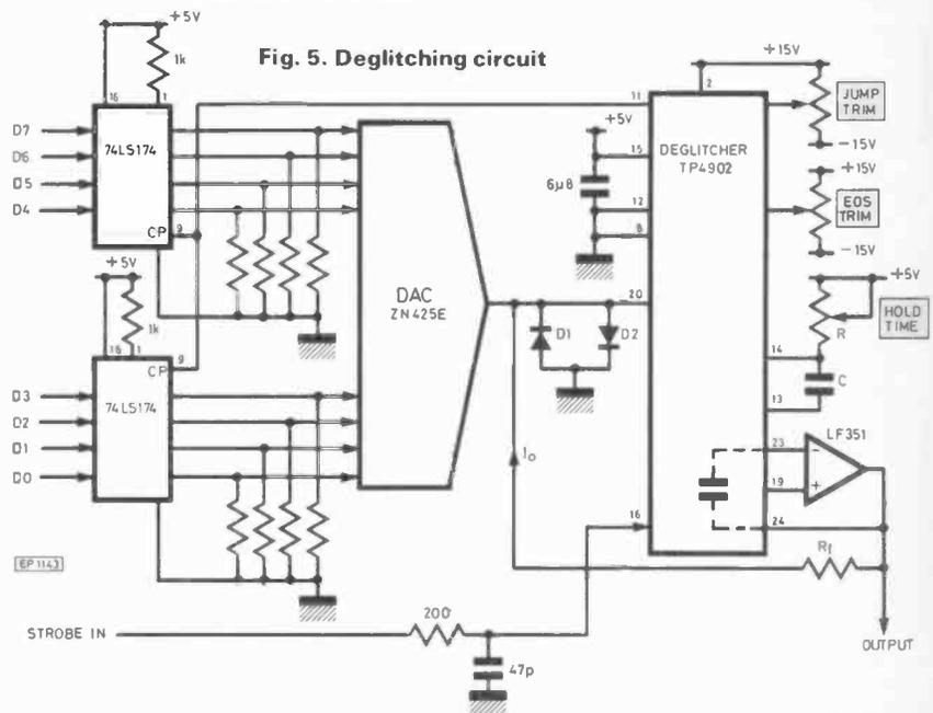
**Fig. 5. Deglitching circuit**
