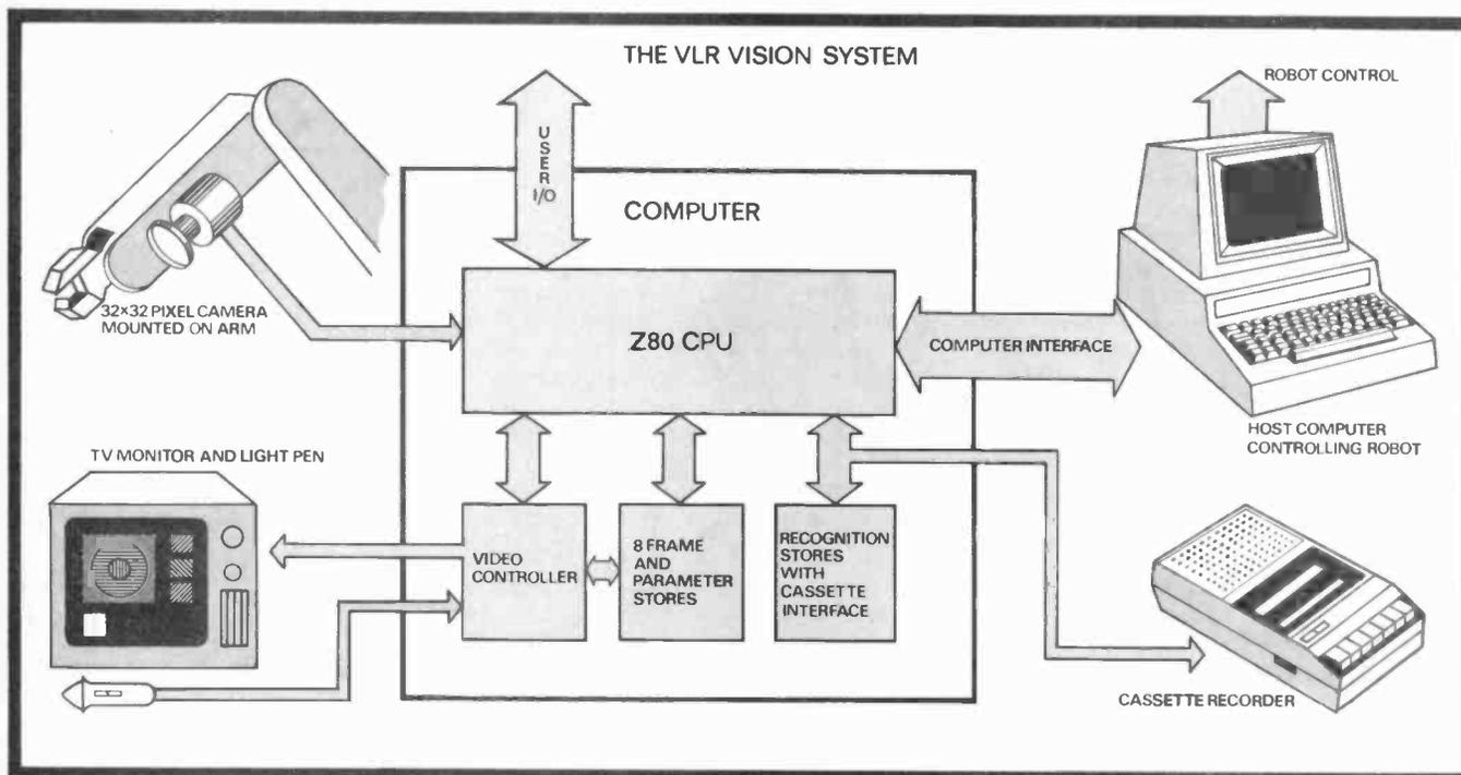
A typical configuration of the COLVIS high-speed system: Commands may be entered either with the light pen or via the user I/O channel. The host computer interrogates the system for visual information which it then uses to control the robot
