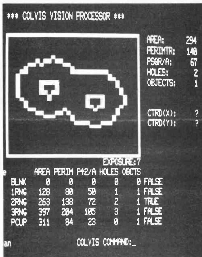
Fig. 1. VDU showing object identification
