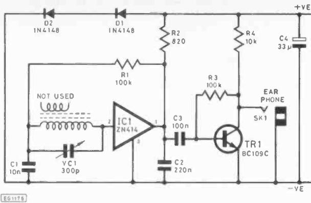
Fig. 1. Circuit diagram of the MW Radio
