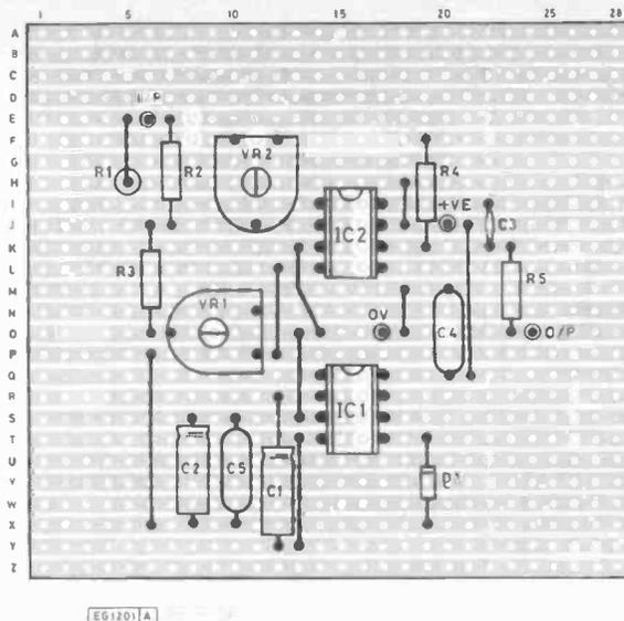
Fig. 9 Logic system with a d.c. coupled analogue output. Omit R1 if input is CMOS logic
