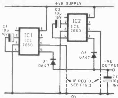
**Fig. 5 Parallel connection of i.c.s**
