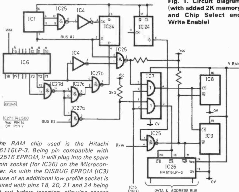
The RAM chip used is the Hitachi HM6116LP-3. Being pin compatible with the 2516 EPROM, it will plug into the spare 24-pin socket (for IC26) on the Microcontroller. As with the DISBUG EPROM (IC3) the use of an additional low profile socket is required with pins 18, 20, 21 and 24 being bent out before insertion, allowing access for modifications. The p.c.b. wiring of address and data lines are compatible. Modifications are however required for the control signals—p.c.b. modifications being:
