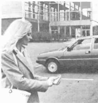
Motorola's Converted Lancia Delta. An electronic key allows windows to be wound up and down, and doors to be unlocked remotely, but the vehicle is "no gimmick". The whole car can be tested via one diagnostic socket
