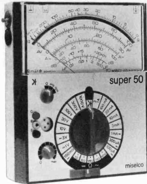
**Model:** Miselco 'Super' 50. **Ranges:** Voltage d.c. 150mV-1000V (8 ranges). Voltage a.c. 0-1000V (5 ranges). Current d.c. 20 $\mu$ A-3A (10 ranges). Current a.c. 3mA-3A (6 ranges). Resistance 0-50M $\Omega$  (5 ranges). Decibels -10 to +61 (5 ranges). **Special Features:** Diode test facility. **Price:** £50. **Supplier:** Alcon Instruments Ltd., 19 Mulberry Walk, London SW3 6DZ. (01-352 1897).
