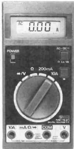
**Model:** Soar ME-531. **Ranges:** Voltage d.c. 200mV-1000V (5 ranges). Voltage a.c. 2V-1000V (4 ranges). Current d.c. 200mA-10A (2 ranges). Current a.c. 200mA-10A (2 ranges). Resistance 200 $\Omega$ -2M $\Omega$  (5 ranges). **Special Features:** Autoranging. Continuity. Diode tester. **Price:** £56.20. **Supplier:** Maplin Electronic Supplies, PO Box 3, Rayleigh, Essex SS6 8LR. (0702 554155).
