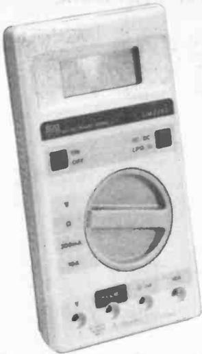
**Model:** ISI DM3350. **Ranges:** Voltage d.c. 0-1000V (4 ranges). Voltage a.c. 0-600V (4 ranges). Current a.c./d.c. 0-10A (2 ranges). Resistance 0-2M $\Omega$  (5 ranges). **Special Features:** Autoranging, Continuity. **Price:** £51.75. **Supplier:** Semiconductor Supplies International Ltd., Dawson House, 128/130 Carshalton Road, Sutton, Surrey SM1 4RS. (01-643 1126).
