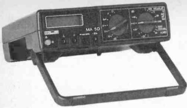
**Model:** BBC MA5D. **Ranges:** Voltage a.c./d.c. 300mV–1000V (5 ranges). Current a.c./d.c. 300 $\mu$ A–20A (6 ranges). Resistance 3k $\Omega$ –20M $\Omega$  (5 ranges). Capacitance 300nF–3000 $\mu$ F (5 ranges). Decibels (5 ranges). **Special Features:** Built-in battery charger. **Price:** £265.00. **Supplier:** House of Instruments, Clifton Chambers, 62 High Street, Saffron Walden, Essex. (0799 24922).
