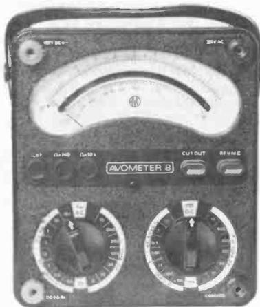
**Model:** Avometer Model 8 Mk 5. **Ranges:** Voltage d.c. 100mV-3000V (9 ranges). Voltage a.c. 3V-3000V (8 ranges). Current d.c. 50 $\mu$ A-10A (7 ranges). Current a.c. 10mA-10A (4 ranges). Resistance 2k $\Omega$ -20M $\Omega$  (3 ranges). Decibel range. **Special Features:** Automatic cut out. **Price:** £145.00. **Supplier:** House of Instruments. (0799 24922).
