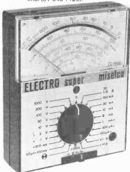
**Model:** Miselco Electro Super. **Ranges:** Voltage a.c./d.c. 100mV–1000V (9 ranges). Current a.c./d.c. 100 $\mu$ A–6A (8 ranges). Resistance 0–1M $\Omega$  (3 ranges). **Special Features:** dB scale. **Price:** £56.00. **Supplier:** Alcon Instruments Ltd., 19 Mulberry Walk, London SW3 6DZ. (01-352 1897).
