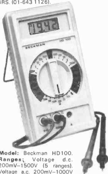
**Model:** Beckman HD100. **Ranges:** Voltage d.c. 200mV-1500V (5 ranges). Voltage a.c. 200mV-1000V (5 ranges). Current a.c./d.c. 200 $\mu$ A-2A (5 ranges). Resistance 200 $\Omega$ -20M $\Omega$  (6 ranges). **Price:** £132.25. **Supplier:** ITT. (0279 29522).
