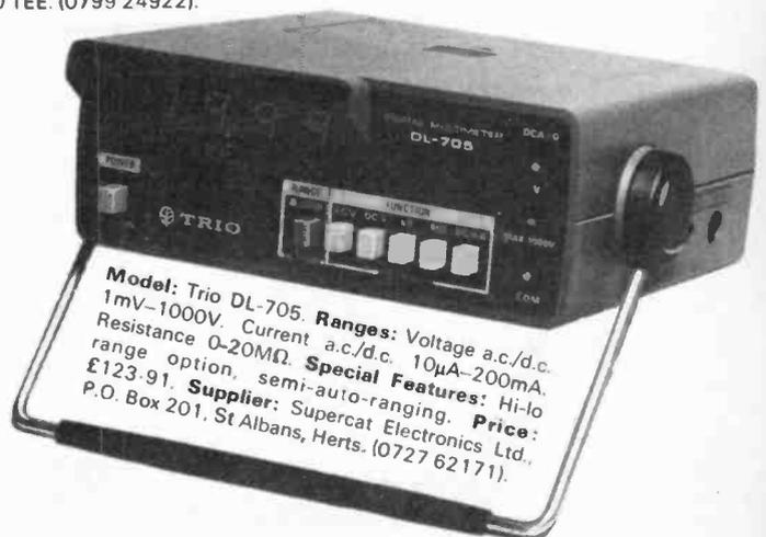
**Model:** Trio DL-705. **Ranges:** Voltage a.c./d.c. 1mV-1000V. Resistance 0-20M $\Omega$ . Current a.c./d.c. 10 $\mu$ A-200mA. **Special Features:** Hi-lo range option, semi-auto-ranging. **Price:** £123.91. **Supplier:** Supercat Electronics Ltd., P.O. Box 201, St Albans, Herts. (0727 62171).
