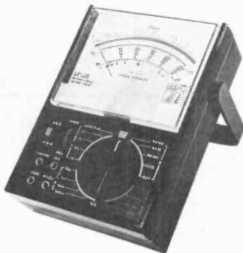
**Model:** YK375. **Ranges:** Voltage d.c. 0-25V-1000V (6 ranges). Voltage a.c. 10V-1000V (4 ranges). Current d.c. 25 $\mu$ A-10A (10 ranges). Resistance 2k $\Omega$ -20M $\Omega$  (5 ranges). Decibels (8 ranges). **Special Features:** Range doubler facility which enables readings to be taken at lower ranges. **Price:** £19.95. **Supplier:** Maplin Electronic Supplies, PO Box 3, Rayleigh, Essex. (0702 554155).
