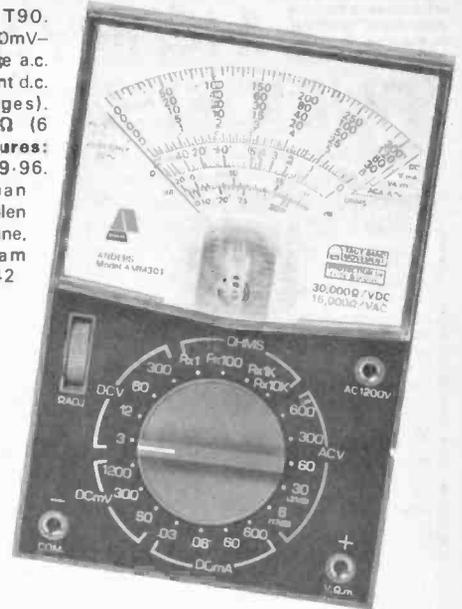
**Model:** Anders AMM301. **Ranges:** Voltage d.c. 60mV-300V (7 ranges). Voltage a.c. 6V-600V (5 ranges). Current d.c. 0.03mA-600mA (4 ranges). Resistance 0-2M $\Omega$  (4 ranges). **Special Features:** dB scale. **Price:** £29.33. **Supplier:** Anders Electronics Ltd., 48-56 Bayham Place, Bayham Street, London NW1 0EU. (01-387 9092).
