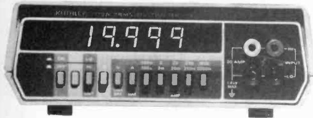
**Model:** Keithley 179A. **Ranges:** Voltage d.c. 200mV–1200V (5 ranges). Voltage a.c. 200mV–1000V (5 ranges). Current a.c./d.c. 200µA–20A (6 ranges). Resistance 0–20MΩ (5 ranges). **Special Features:** Hi-lo range option, over-range indication. **Price:** £385. **Supplier:** Keithley Instruments Ltd, 1 Boulton Road, Reading, Berks RG2 0NL. (0734 861287).
