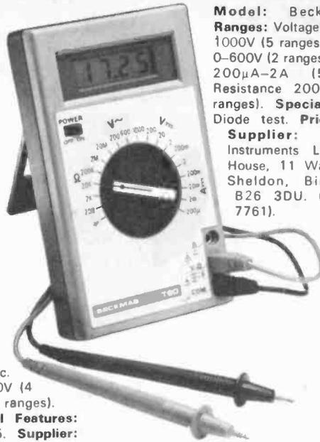
**Model:** Beckman T90. **Ranges:** Voltage d.c. 200mV-1000V (5 ranges). Voltage a.c. 0-600V (2 ranges). Current d.c. 200 $\mu$ A-2A (5 ranges). Resistance 200 $\Omega$ -20M $\Omega$  (6 ranges). **Special Features:** Diode test. **Price:** £49.96. **Supplier:** Beckman Instruments Ltd., Mylen House, 11 Wagon Lane, Sheldon, Birmingham B26 3DU. (021-742 7761).
