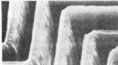
precedented accuracy can be achieved because the geometry of the cut is controlled entirely by the shape of the light beam.
