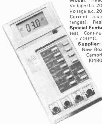
**Model:** Hitachi VR3525. **Ranges:** Voltage d.c. 200mV–1000V (5 ranges). Voltage a.c. 200mV–750V (4 ranges). Current a.c./d.c. 200 $\mu$ A–10A (5 ranges). Resistance 200 $\Omega$ –20M $\Omega$ . **Special Features:** Autoranging. Diode test. Continuity. Temp. –20°C to +700°C. **Price:** £120.75. **Supplier:** Reltech Instruments, New Road, St. Ives, Huntingdon, Cambridgeshire PE17 4BG. (0480 63570).
