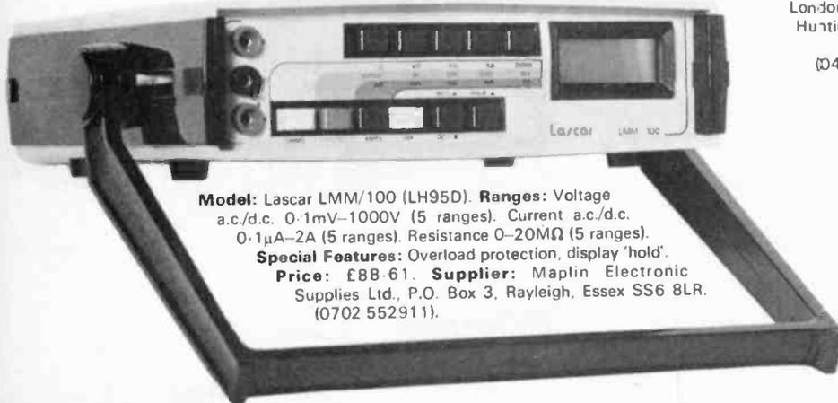
**Model:** Lascar LMM/100 (LH95D). **Ranges:** Voltage a.c./d.c. 0.1mV–1000V (5 ranges). Current a.c./d.c. 0.1µA–2A (5 ranges). Resistance 0–20MΩ (5 ranges). **Special Features:** Overload protection, display 'hold'. **Price:** £88.61. **Supplier:** Maplin Electronic Supplies Ltd., P.O. Box 3, Rayleigh, Essex SS6 8LR. (0702 552911).
