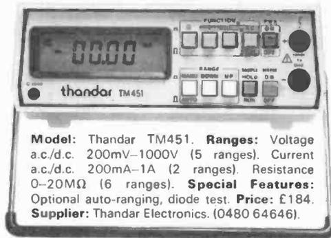
**Model:** Thandar TM451. **Ranges:** Voltage a.c./d.c. 200mV–1000V (5 ranges). Current a.c./d.c. 200mA–1A (2 ranges). Resistance 0–20MΩ (6 ranges). **Special Features:** Optional auto-ranging, diode test. **Price:** £184. **Supplier:** Thandar Electronics. (0480 64646).
