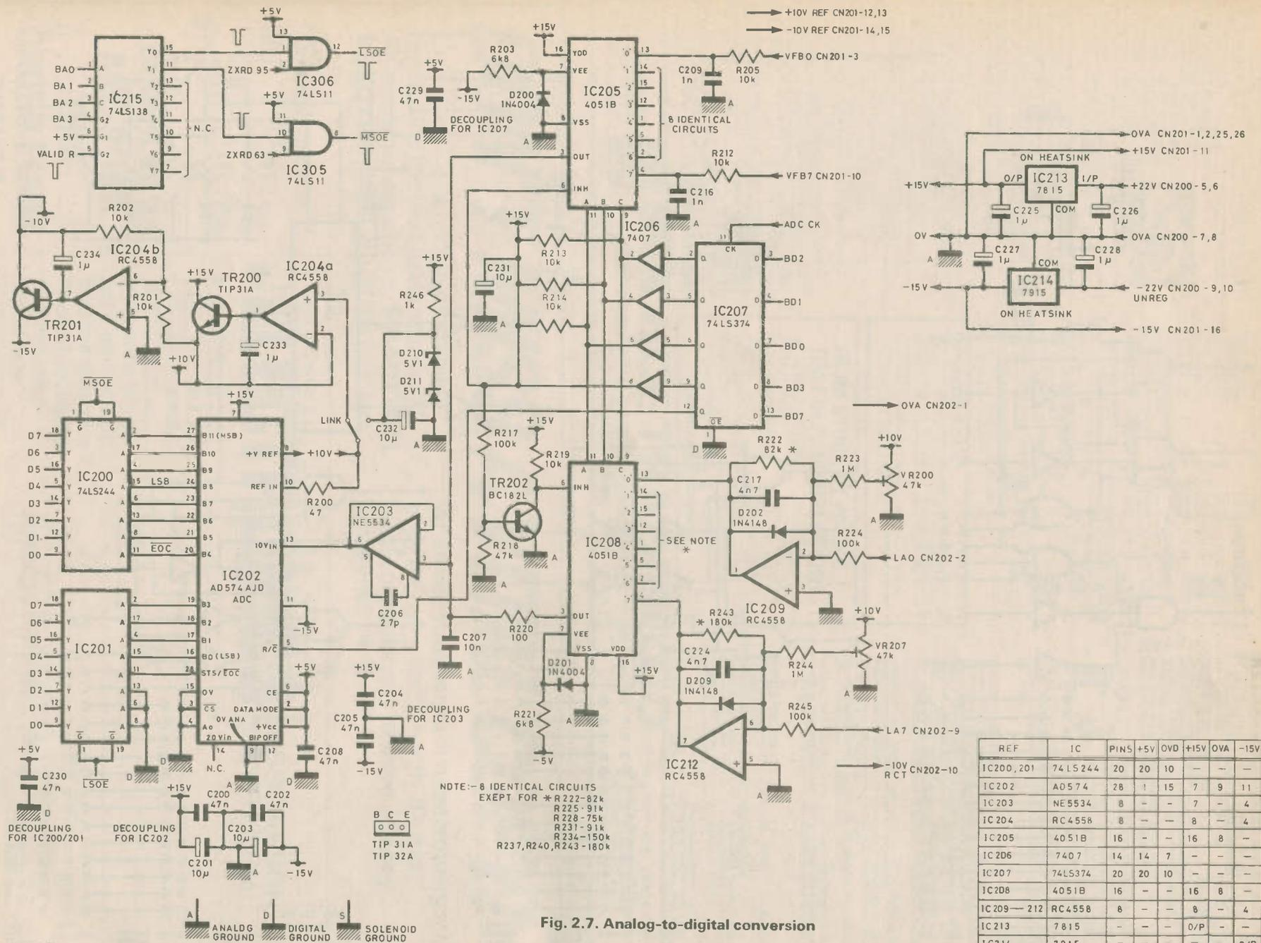
Fig. 2.7. Analog-to-digital conversion
