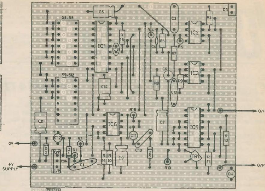
Fig. 8. Veroboard layout of the Opto-Lock
