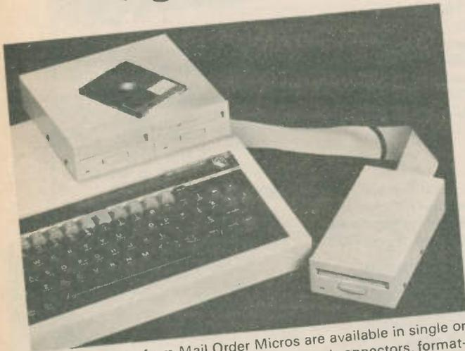
The 3in. drives from Mail Order Micros are available in single or dual units. They are supplied with leads and connectors, formatting/utility disc and a manual. The drives can be powered from the p.s.u. of the BBC micro. The single drive has 80 tracks and a 200Kbytes capacity, whilst the dual drive has a 400Kbytes capacity. Mail Order Micros. (Address below.)
