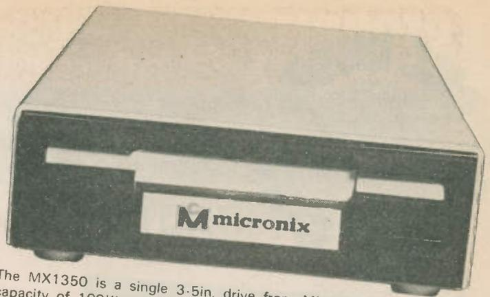
The MX1350 is a single 3.5in. drive from Micronix, it will provide a capacity of 100Kbytes of storage; a dual unit, the (MX2350) is also available with a 200Kbyte storage capability. Both these units are 40 track and are single-sided, and are boxed in metal housings, supplied complete with power cable, disc drive cable, formatter disc and DFS manual. Prices respectively are £181.70 and £353.05. **Micronix Computers Ltd.**, Suite 2, 26 Charing Cross Road, London WC2. (01-240 0213/0217)
