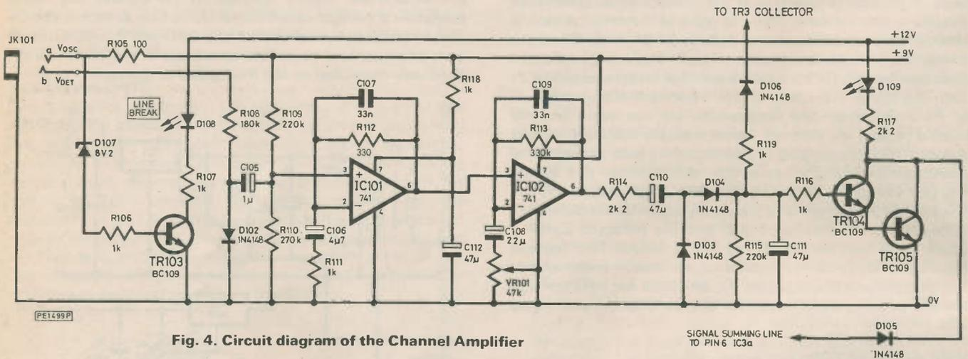
Fig. 4. Circuit diagram of the Channel Amplifier
