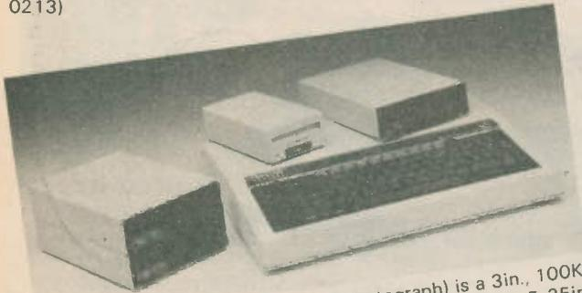
The Teac FD30A (shown centre in photograph) is a 3in., 100K, single-sided drive, and is fully compatible with Teac's 5.25in. drives. The actual floppy disc used in the 30A is stored in a hard case, not the soft sleeve used by other floppy discs. This makes loading more positive and reduces the disc's susceptibility to damage by handling. The FD30A is priced at £159 and is available from **Viglen Computer Supplies**, Unit 7, Trumpers Way, London W7 2QA. (01-843 9903)
