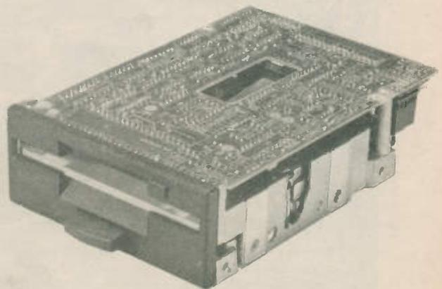
The 350 1Mbyte floppy disc drive from Shugart is a 3.5in., double-density, single drive unit with 80 tracks. The drive is supplied complete with a formatter disc, manual and interconnecting leads. Mail Order Micros. (Address left.)
