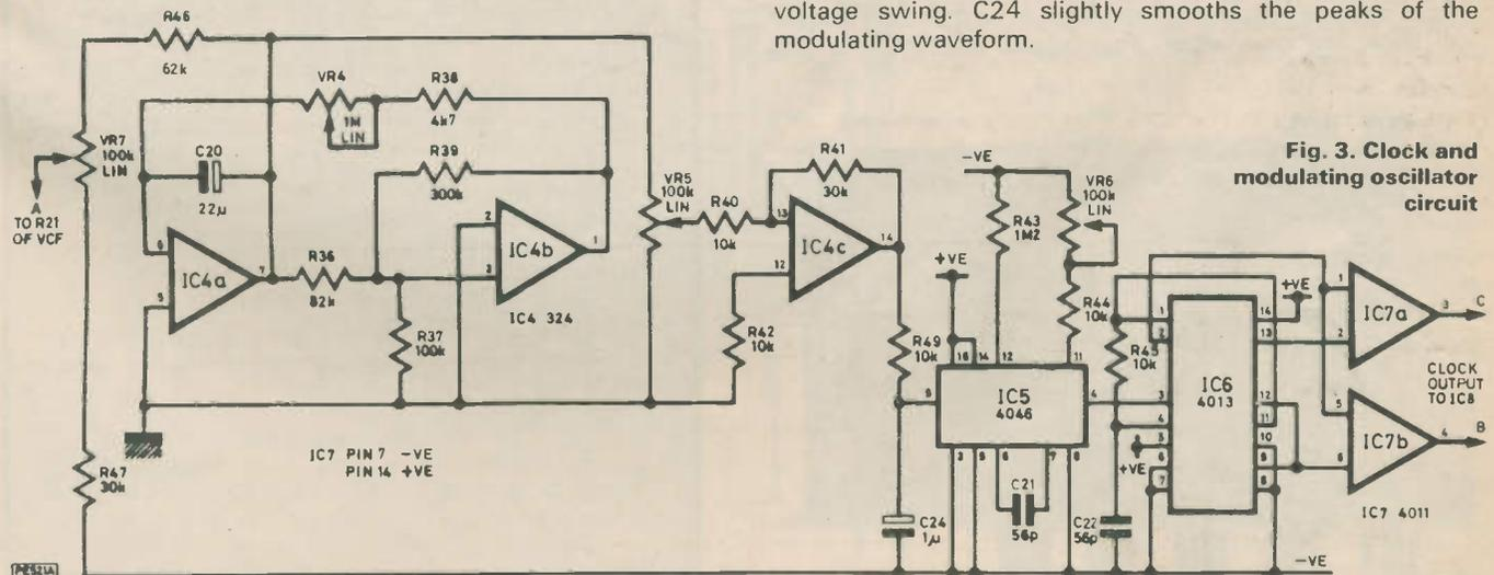
Fig. 3. Clock and modulating oscillator circuit
