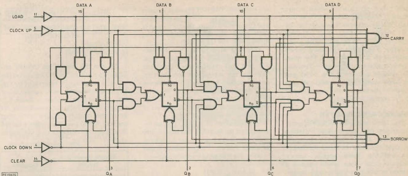
Fig. 1.2. Internal logic of the 74193
