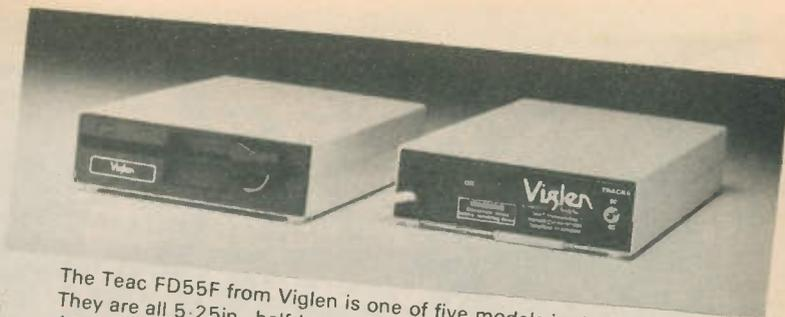
The Teac FD55F from Viglen is one of five models in the FD55 series. They are all 5.25in. half-height drives with capacities which vary from 125K to 1.6Mbytes. The 55F is a 40/80 track switchable, double-sided, single drive unit with a 400K capacity and is priced at £225. **Viglen Computer Supplies**, Unit 7, Trumplers Way, London W7 2QA. (01-843 9903)
