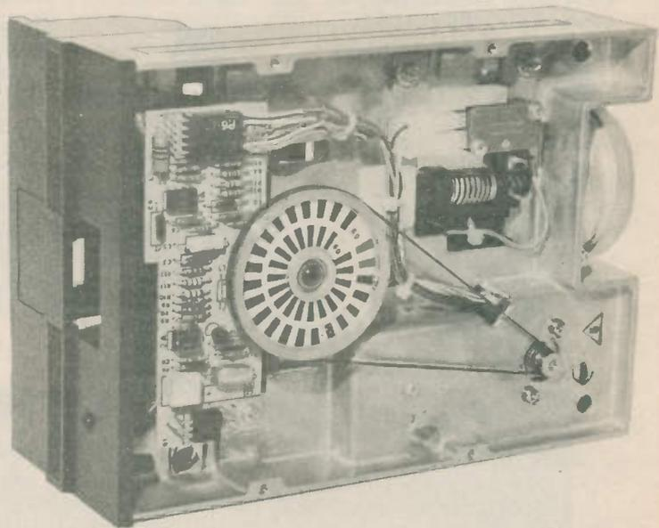
An internal view of a standard height disc drive showing the drive belt arrangement. (Courtesy of Cumana Ltd.)
