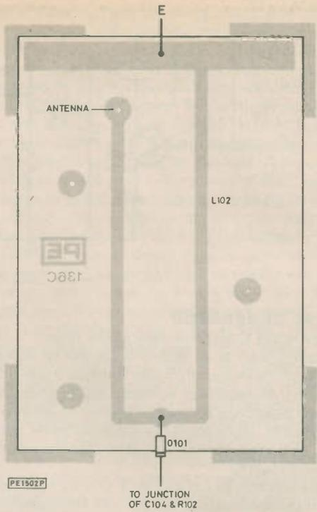
Fig. 8 (below). The P.c.b. and component layout of the Oscillator board
