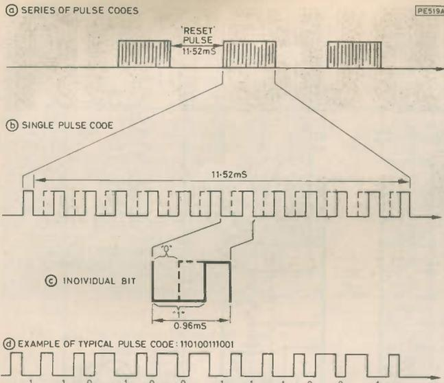
Fig. 2. Pulse code waveforms
