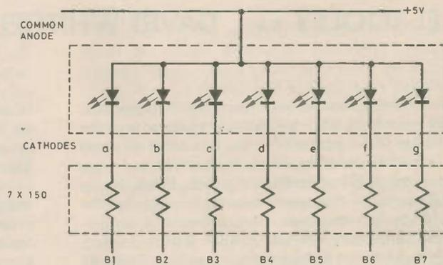
**Fig. 1.10. Typical arrangement for driving a seven-segment i.e.d. display**
