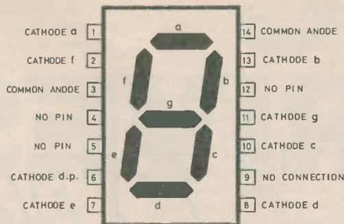
**Fig. 1.9. Normal format for a common anode seven-segment i.e.d. display**
