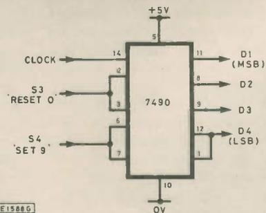
Fig. 1.8. Simple BCD counter using a 7490
