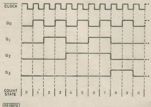
Fig. 1.7. Timing diagram for the BCD outputs of a 7490
