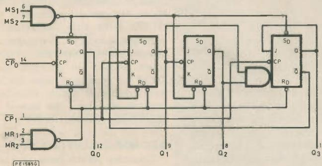
Fig. 1.5. Internal logic of the 7490
