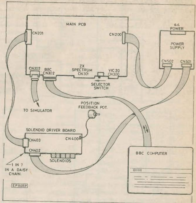
Fig. 2.2. The system interconnected with ribbon cable
