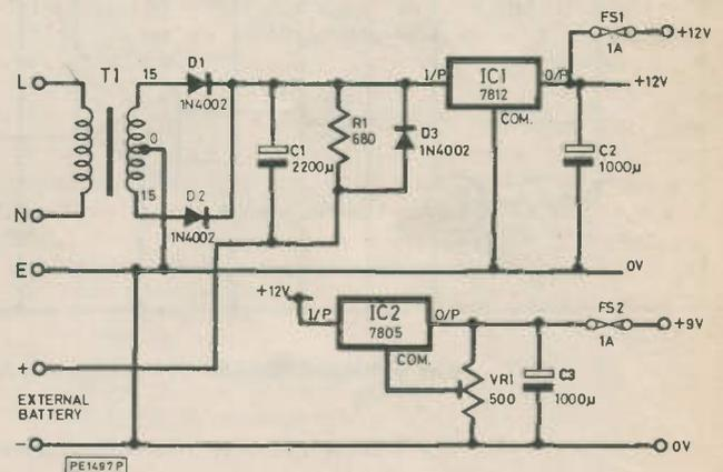
Fig. 3. Power Supply circuit diagram
