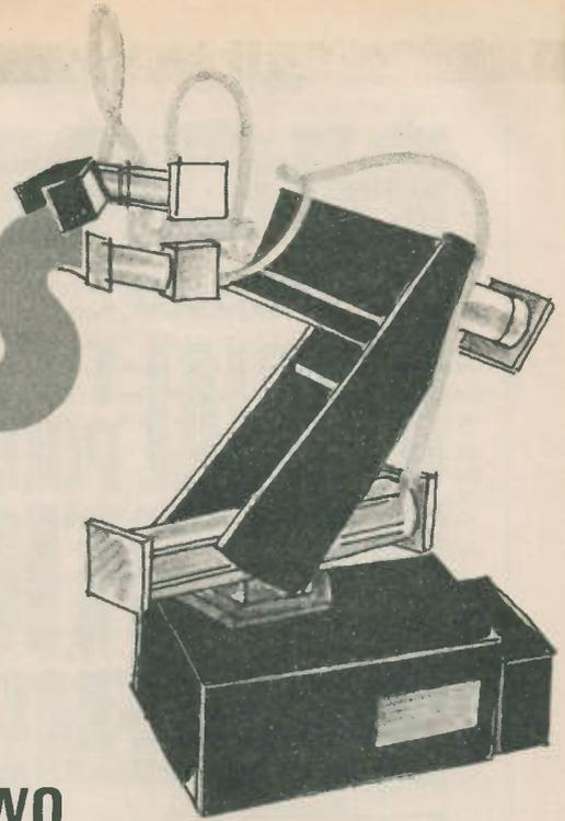
THE ROBOTS are directly controlled by a BBC, VIC-20, or Spectrum computer, and the way that control is achieved is explained here. It involves digital-to-analog conversion, multiplexing to each of the axes; and then conversion of the position data back from analog into digital form, to be fed back to the computer for display on the TV.
