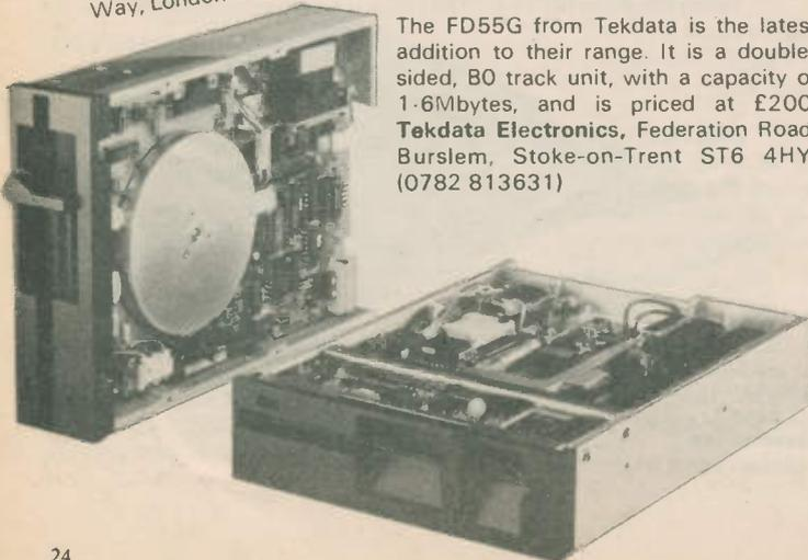
The FD55G from Tekdata is the latest addition to their range. It is a double-sided, 80 track unit, with a capacity of 1.6Mbytes, and is priced at £200. **Tekdata Electronics**, Federation Road, Burslem, Stoke-on-Trent ST6 4HY. (0782 813631)
