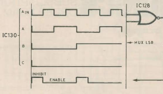
Fig. 2.5. Demultiplexer inhibit timing
