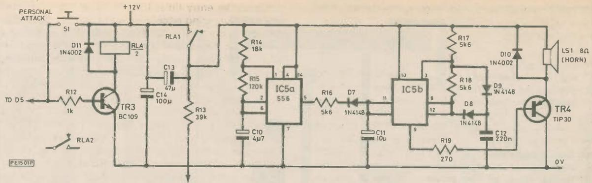
Fig. 6. The Noise Generator circuit diagram
