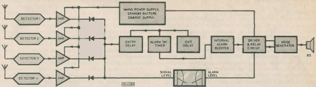
Fig. 1. Schematic diagram of the complete unit
