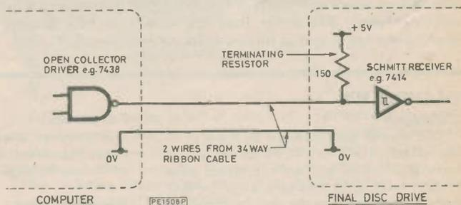
**Fig. 3. Disc interface signal driving**
