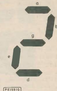
**Fig. 1.11. Typical seven-segment display output**
