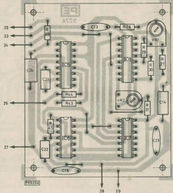
Fig. 7. Delay board component layout
