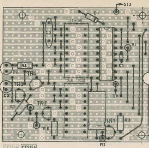
Fig. 7. Veroboard layout of the Opto-Key
