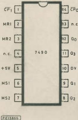
Fig. 1.6. Pin connections for the 7490
