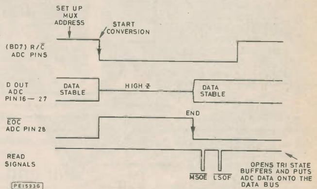
Fig. 2.8. Sequence for read and conversion
