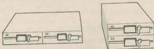
**Fig. 2. Twin drive configurations**
