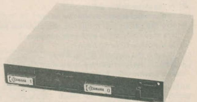
The Cumana range of disc drives include the CD200K: a 40 track, single-sided drive with 200K of memory. The CD400K: an 80 track, single-sided drive with 400K of memory. The CD400/S: a 40/80 track, single-sided drive. The CD800/S: a double-sided version of the 400/S; and the CD400/D, a 40 track, double-sided drive with 400K of memory. Prices for the drives vary from £350 to £575. **Cumana Ltd.**, Unit 1, The Pines Industrial Estate, Broad Street, Guildford GU3 3BH. (0483 503121)
