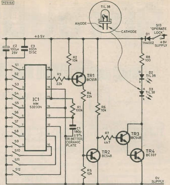
Fig. 5. Circuit diagram of the Opto-Key
