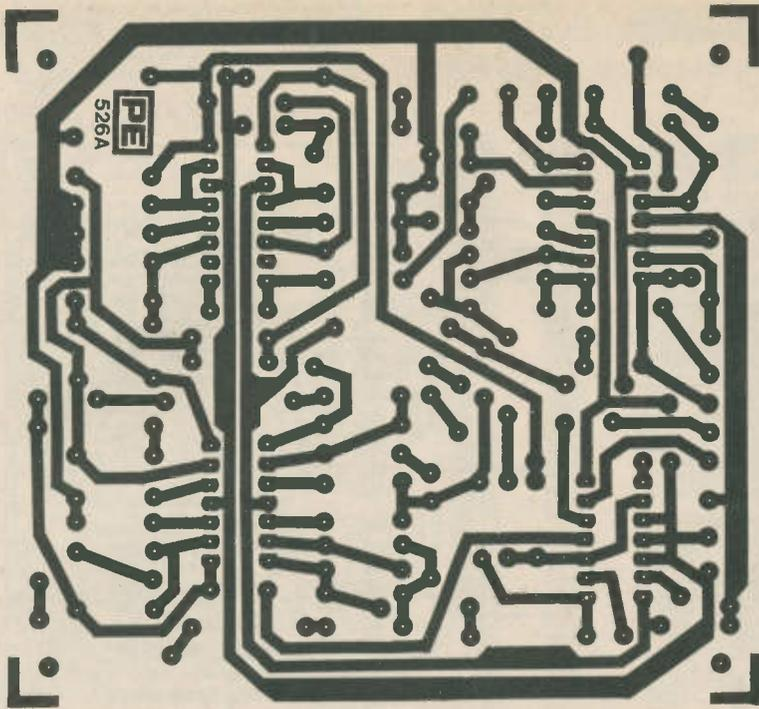
Fig. 4. Main board p.c.b. layout (actual size)
