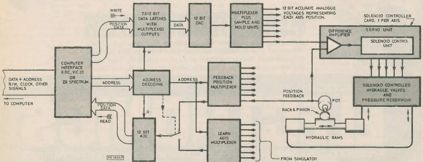
Fig. 2.1. Block diagram of the NEPTUNE Robot system
