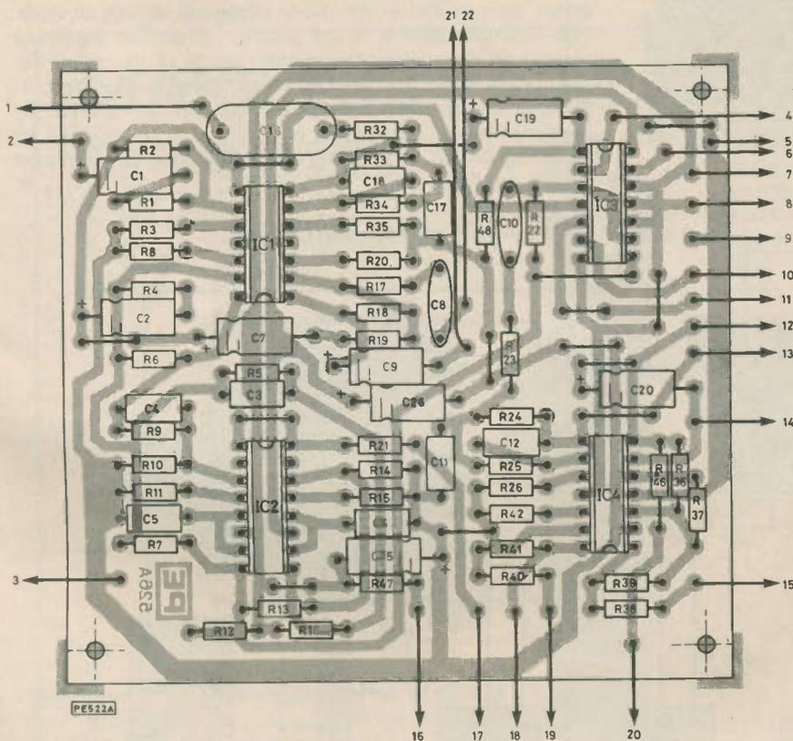
Fig. 5. Main board component layout
