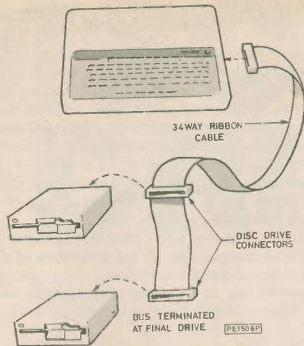
Fig. 4. Daisy-chain disc cable arrangement
