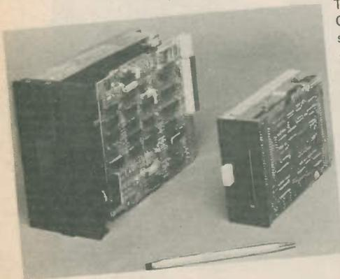
The Shugart SA300 from Mail Order Micros is 3.5in., single-sided microfloppy drive with 40 tracks and 500K memory capacity. The drive is compatible with 5.25in. units and is available in either a single or dual drive configuration. A formatter, instruction manual and connecting cables are supplied. The single drive is priced at £102.35, and the dual unit at £201.28. Mail Order Micros, 2a Green Street, Sandbach, Cheshire CW11 9AX. (0782 811711)
