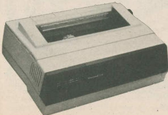
**Model:** Honeywell L38 **Print format:** Dot Matrix **C.P.S.:** 400 **Interface:** Centronics Compatible **Paper:** 381mm Tractor **Notes:** Adjustable tractor **Price:** £438+VAT **Supplier:** Geveke Electronics, Landsbury Ind. Est., 102 Lower Guildford Rd., Knaphill, Surrey (04867 88676).
