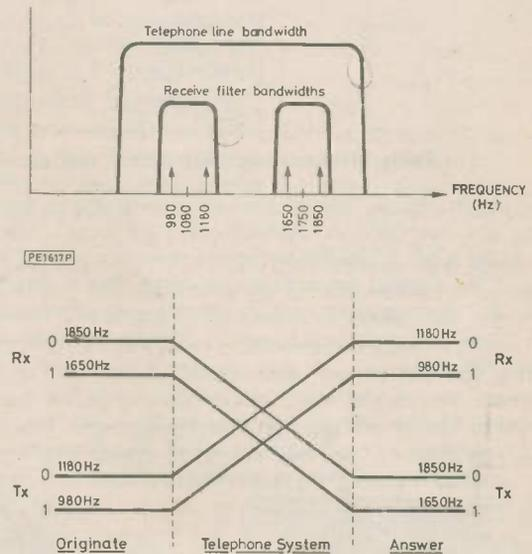
Fig. 6. V21 channels for 300/300 baud
