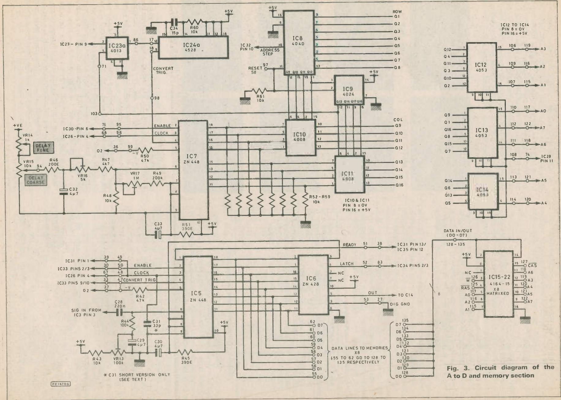
Fig. 3. Circuit diagram of the A to D and memory section
