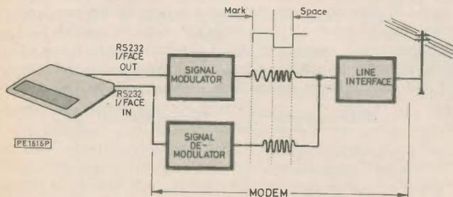
Fig. 5. Basic modem configuration
