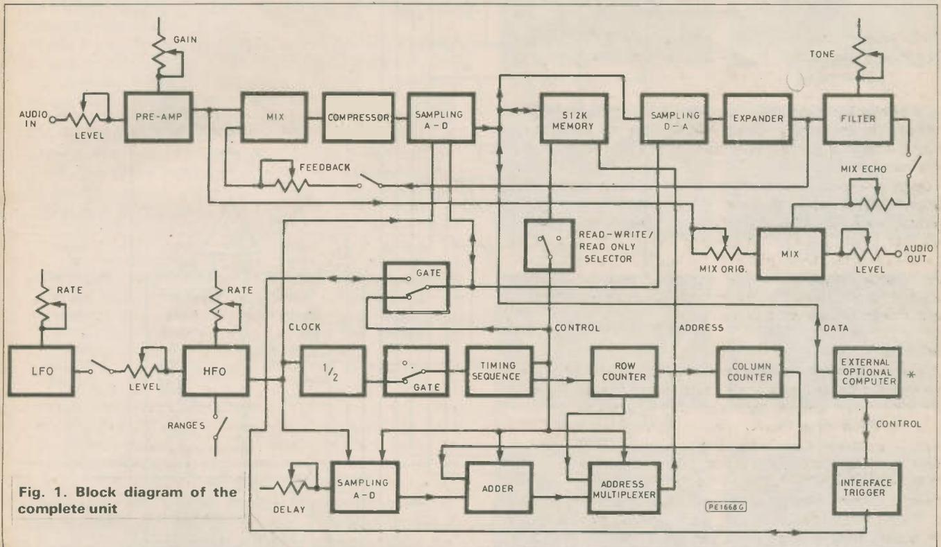
Fig. 1. Block diagram of the complete unit
