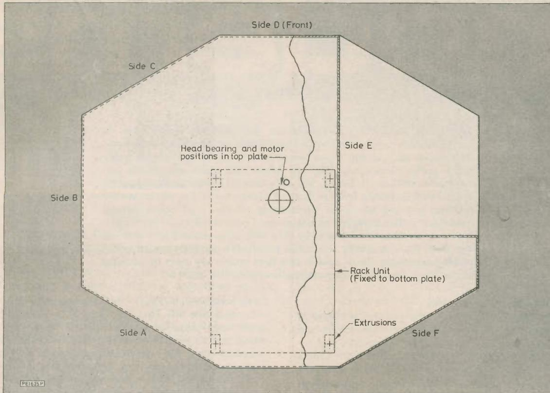
Fig. 3. Plan view of the RUR body. Also housed within the body is a specially manufactured lead-acid battery power source
