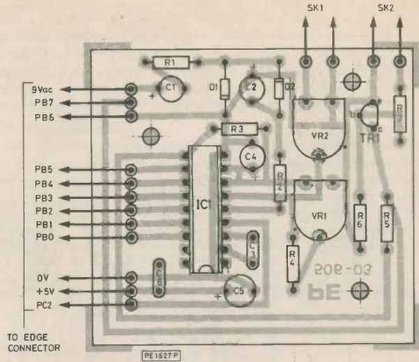
Fig. 5. Construction of the interface p.c.b.
