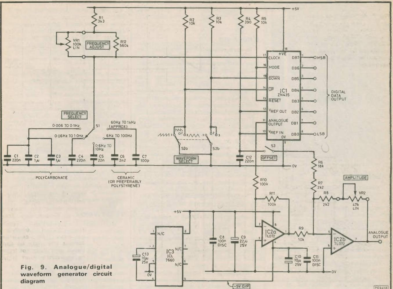
Fig. 9. Analogue/digital waveform generator circuit diagram
