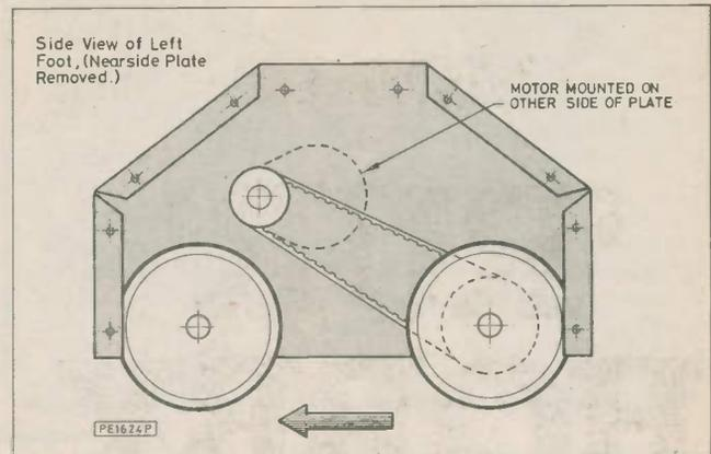
Fig. 2. Foot drive system. Only one wheel is driven
