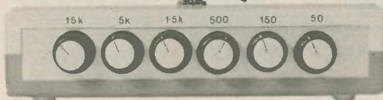
This low cost unit is an ideal add-on for electric guitars, providing a wide range of musical effects. The unit incorporates six graphic equaliser channels with centre frequencies between 50Hz and 15kHz.
