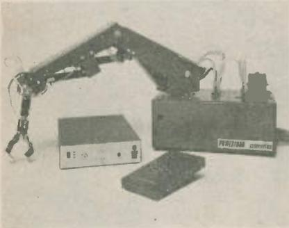
Powertran Cybernetics, has now launched Mark II versions of the Genesis programmable hydraulic robots. The Mark II Genesis P101 and P102 are a result of Powertran's policy of continued development rather than a radical redesign, and represent detail improvements over the originals. In addition to the RS232 of the Mark I version, there is now a parallel I/O port.
