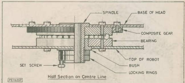
Fig. 1. The head ball bearing assembly
