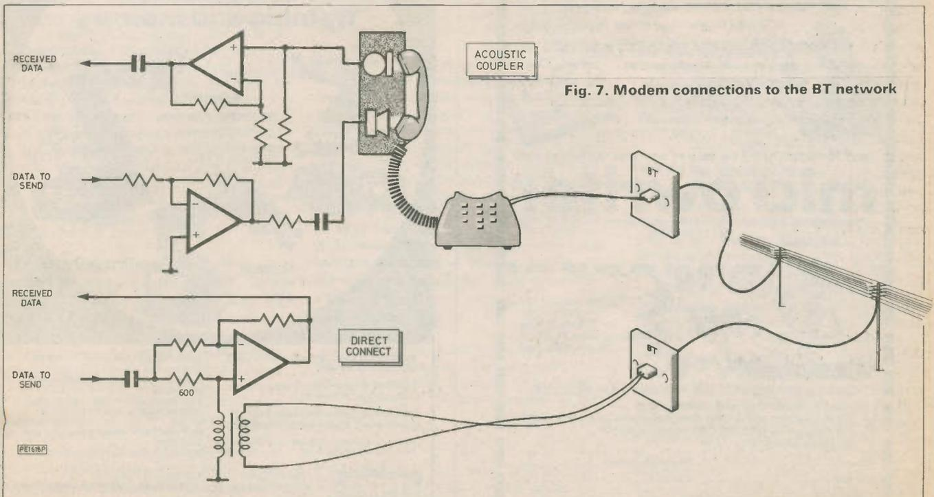
Fig. 7. Modem connections to the BT network
