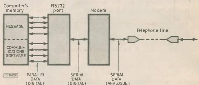
Fig. 1. Computer communications by telephone
