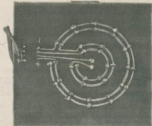
The track-side of the eye p.c.b. Note that the l.e.d.s may be illuminated in rings—outer, inner, and centre (single) l.e.d.
