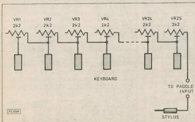
Fig. 1. Circuit of the simple stylus keyboard
