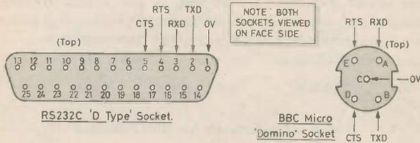
**Fig. 2. Serial port connectors**
