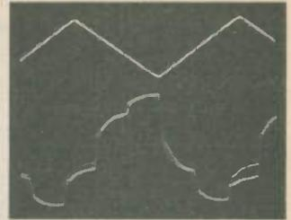
Photo 10. Audio frequency close to sample frequency
