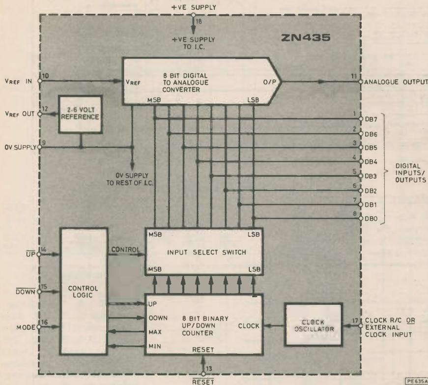
mode input is held at logic 0 to prevent continuous counting in the event of an excessively high analogue input voltage.
