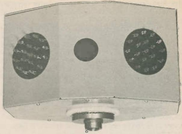
The RUR head incorporates 'eye-catching' I.e.d. eyes, and a hole for an ultrasonic range-finder. The swivel bearing can also be seen
