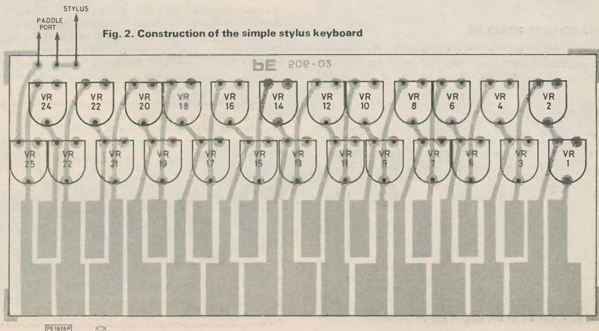
Fig. 2. Construction of the simple stylus keyboard
