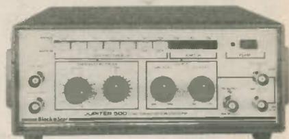
The frequency range is 0.1Hz to 500kHz in seven switched decade ranges with fine frequency control. Sine, square, triangle and TTL (30 loads) waveforms are selectable and an adjustable d.c. offset up to 15V can also be applied to the output. The unit is supplied with a comprehensive instruction manual and sells at £126.50 inc. VAT.
