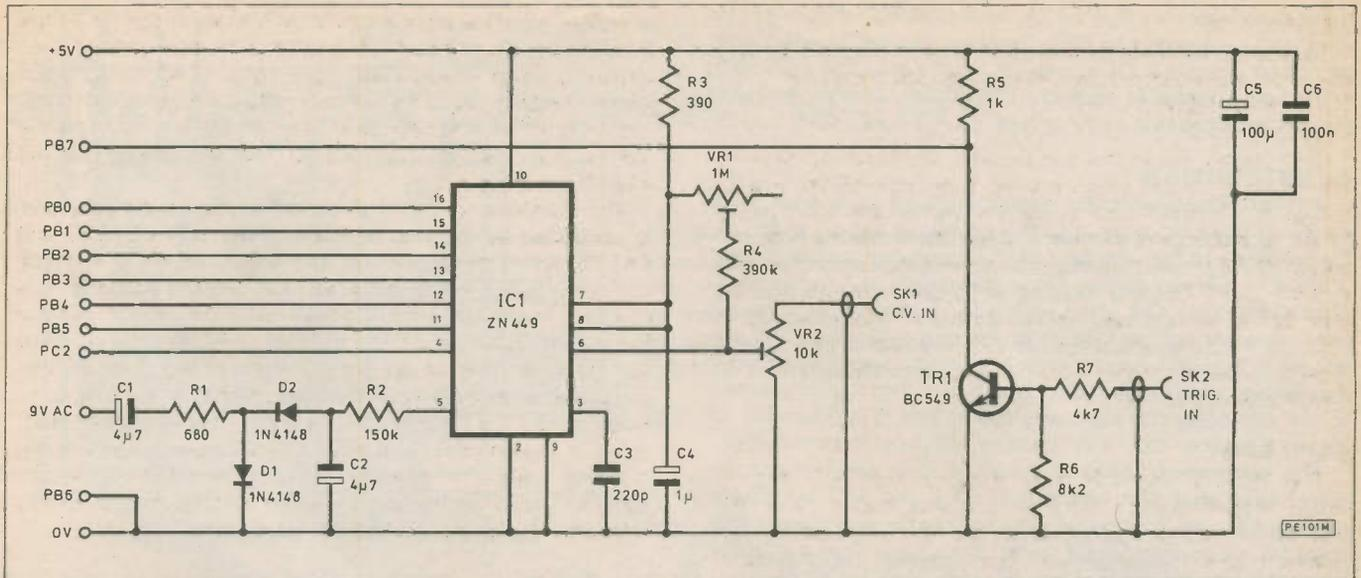
Fig. 4. The synthesiser interface circuit diagram
