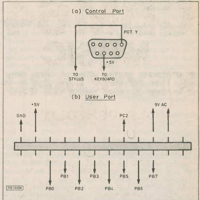
Fig. 3. Connection details for (a) the controller port and (b) the user port
