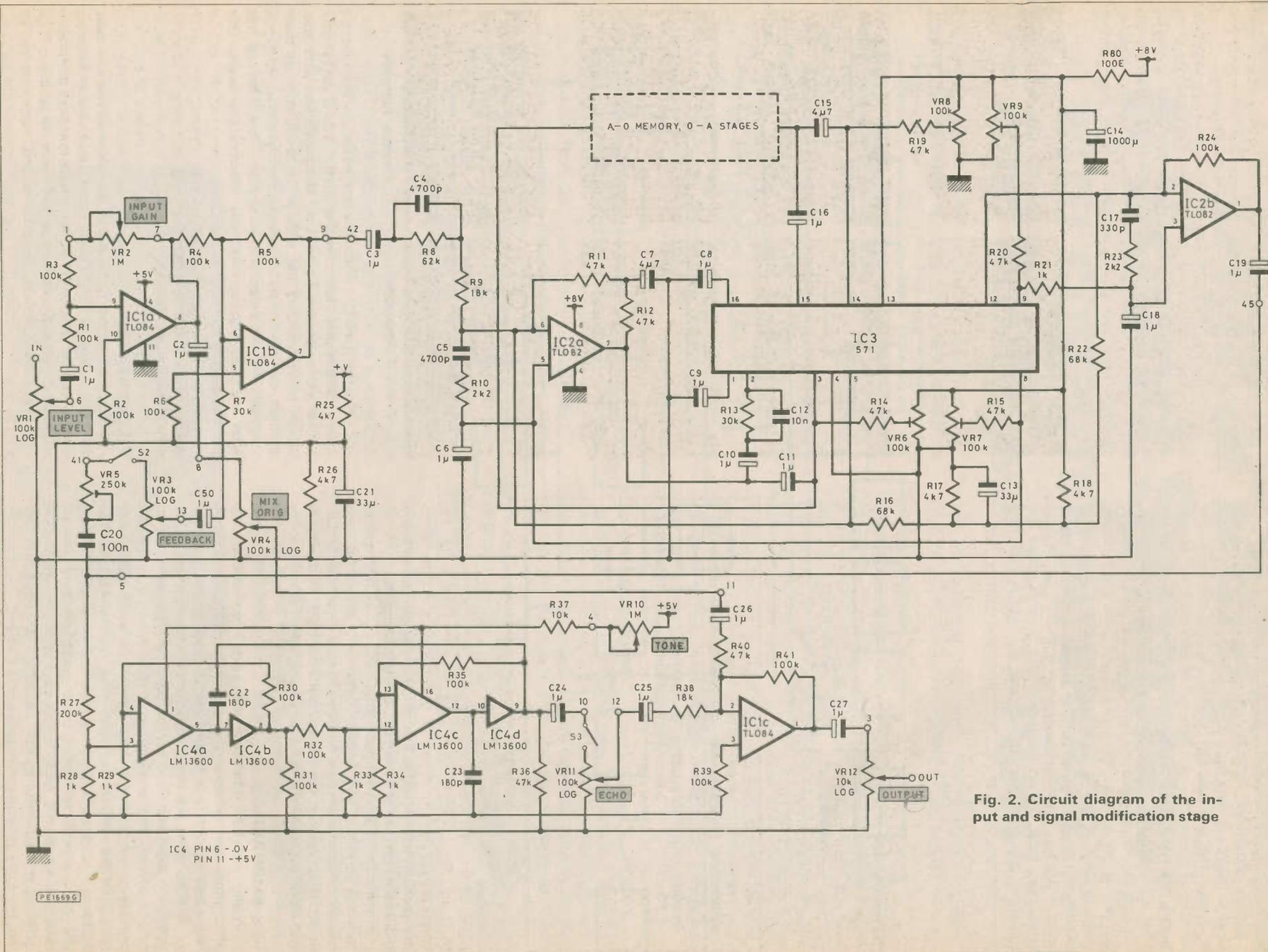
Fig. 2. Circuit diagram of the input and signal modification stage
