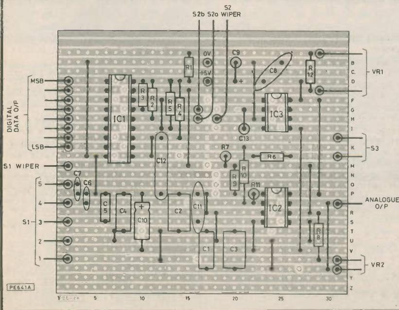
Fig. 10. Stripboard layout of the waveform generator
