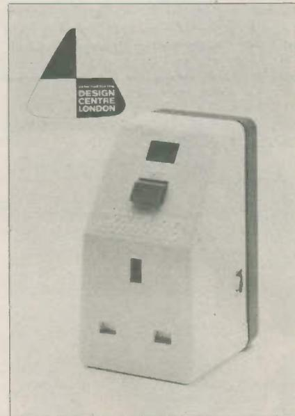
casing. The fuse can be changed in seconds without the use of a tool. The device can be used on all standard 13 amp sockets. A fool-proof and abuse-proof reset mechanism has been incorporated. There is a red "flag" on its side which indicates "on/off" and it has a test button so that you know it is working properly.
