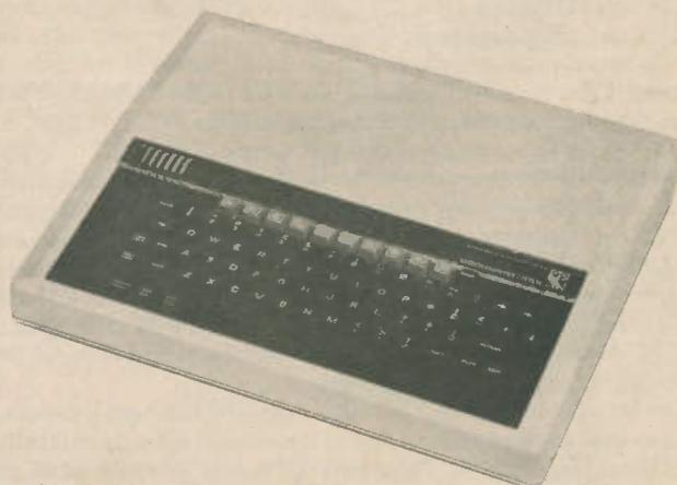
Photo illustrating the BBC Micro which employs a 6502 CPU as the main processor, but may use a Z80 as a second processor
