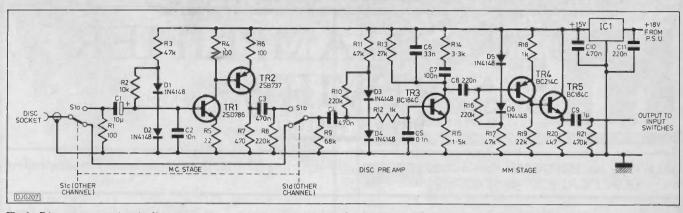
Fig.1. Disc pre-amp circuit diagram
