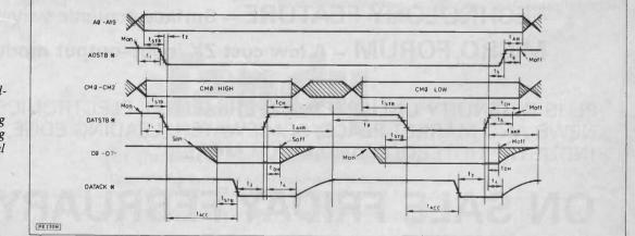
Fig.4. The Read-Modify-Wřite sequence timing diagrams showing all the main signal lines
