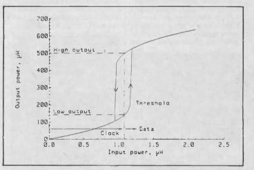
Fig.1. Bistable amplifier chracteristic (theoretical).
