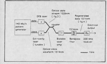
Fig.2. Experimental all-optical regenerator
