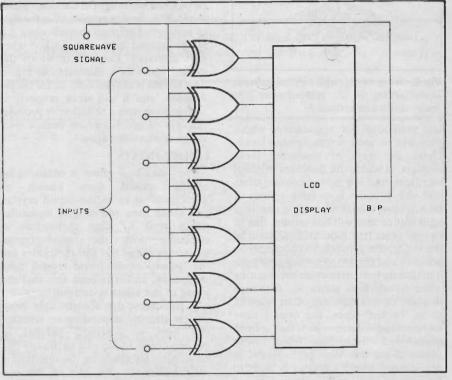
Fig.4. Driving an l.c.d. via XOR gates
