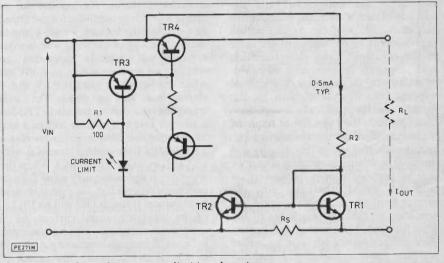
Fig.6. Low voltage drop current limiting detection
