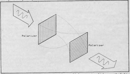
**Fig.3.** In the "relaxed" state the cell produces a 90 degree twist which steers the light through the polarizers. When activated the twisting effect is eliminated, and the light is blocked by one of the olarizers.
