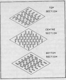
Fig.2. Sections through twisted nematic liquid crystal in the relaxed state (the molecules when activated).
