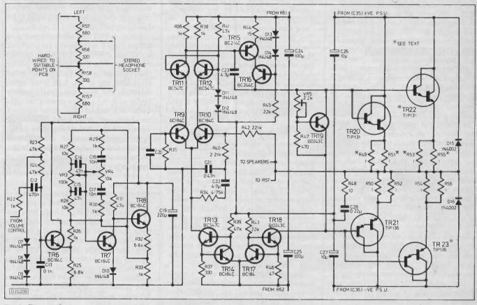
Fig.2. Tone and power amp circuit diagram
