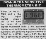
resistors and switches are required – details supplied), or a sensitive digital thermometer (-50°C to +150°C) reading 0-1°. The kit has a sensitivity of 200mV for a full-scale reading, automatic polarity and overload indi-cation. Typical battery life of 2 years (PP3) £17.00
