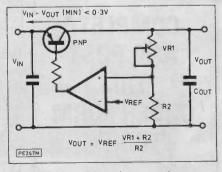
Fig.2. A typical low drop regulator
