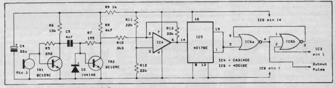
Fig.3. Ultrasonic ranger receiver circuit diagram
