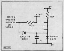
**Fig.5.** Diode clamp for strobe and clock lines
