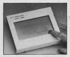
**Photo.3.** Graphic l.c.d. with X-Y touch key overlay
