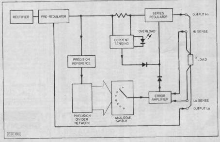
Fig.1. Block diagram of the PE Hi-Stab
