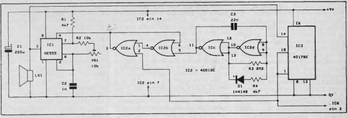
Fig.2. Ultrasonic ranger transmitter circuit diagram
