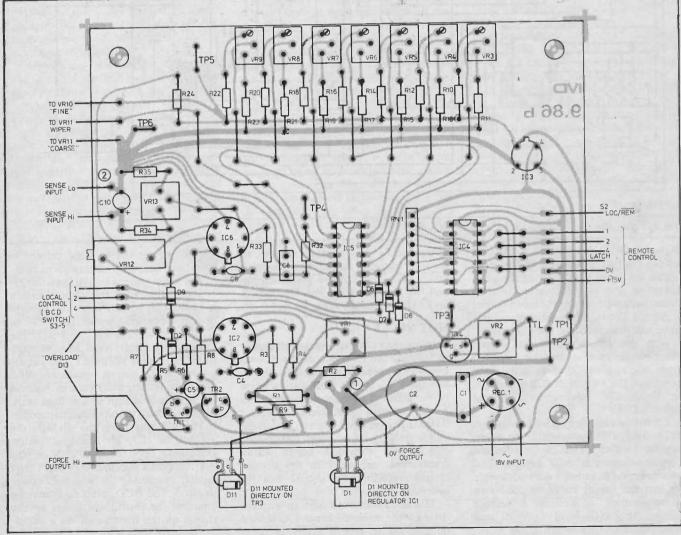
Fig.3. P.c.b. layout of the PE Hi-Stab
