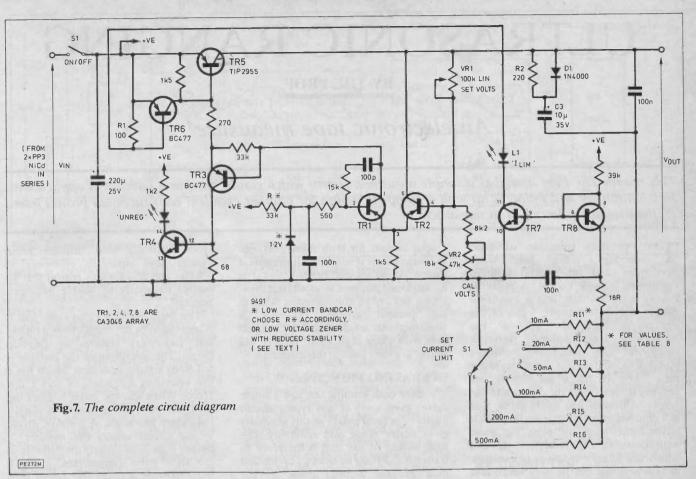
whatever the voltage, this will be the minimum to which VR1 will reduce the output voltage.
