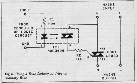
it virtually cuts off the current through R2, and the dissipation in R2 is very low.
