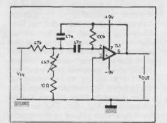
Fig.12. Final filter stage (one of three)
