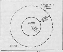
Fig 2. Geostationary orbit
