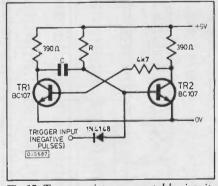
Fig.15. Two-transistor monostable circuit
