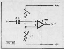
**Fig.13.** Voltage reference stage (one of three)
