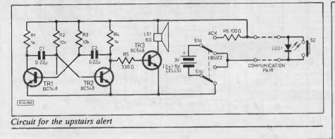
One Sunday afternoon I decided a hitech solution was required. Using a few bits out of my 'rubbish box' I cheaply and quickly constructed the circuit given. The circuit uses two 1.5v cells to power it and the average power consumption is very low.
