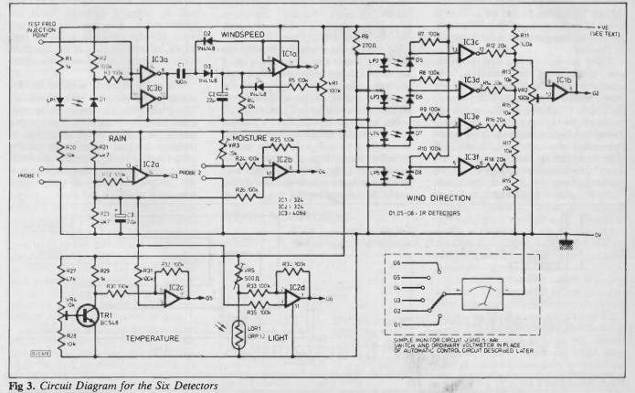
As the temperature at TR1 rises, so its gain will increase, causing a voltage drop at the collector. Since IC2c inverts, the output of IC2c will rise correspondingly. Downward drops of temperature will reverse the gain factor and consequent level change direction. A voltmeter can again be used to read the voltage, at G5.
