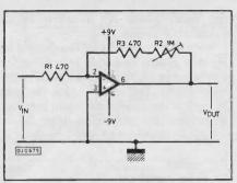
**Fig.7.** Simple pre-amp with gain between 1 and 2000.
