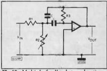
**Fig.10.** Multiple feedback tuned active filter
