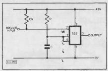
Fig.16. Monostable based on a 555 timer
