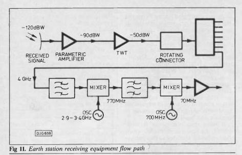
is the noise temperature and G the gain of the aerial. A G/T value of 40 dB/k is required for good signal pick up.
