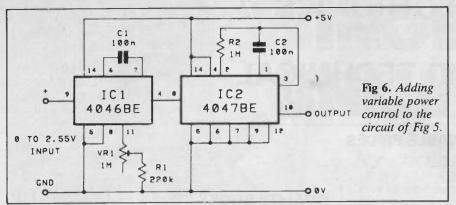
triggered (non-retriggerable) monostable. This is triggered by the output from IC1. With a low frequency input signal the pulses from IC2 are well spread out, and the mark-space ratio is quite low. As the input voltage is raised and the output frequency from IC1 increases, the pulses from IC2 become bunched together and the mark-space ratio increases as well. This gives a simple but effective method of pulse width modulation.
