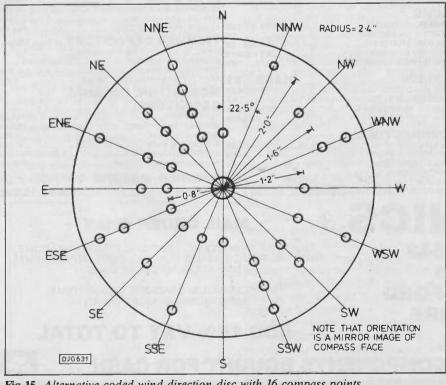
Fig 15. Alternative coded wind direction disc with 16 compass points.
