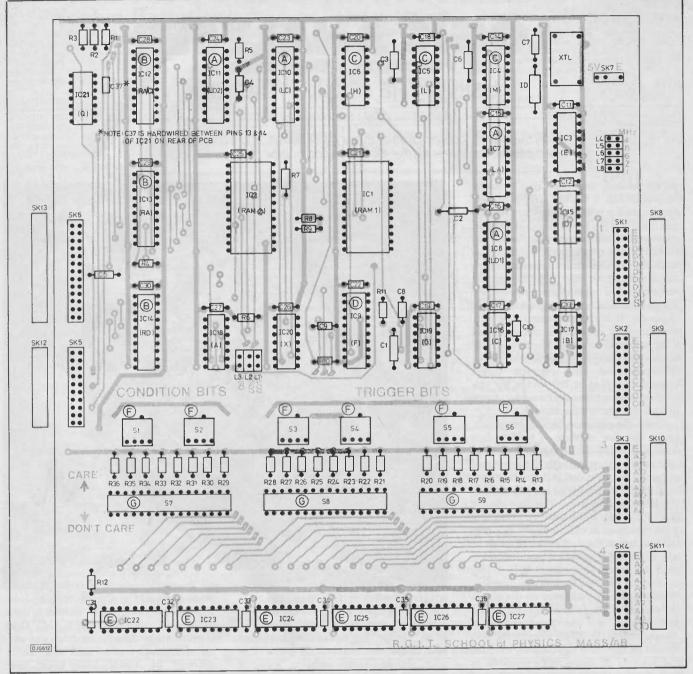
Fig 3. Component positioning details on the printed circuit board. (Top side tracking shown only)
