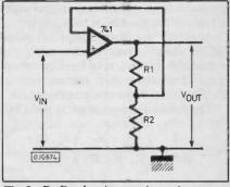
**Fig.9.** Defined gain non-inverting amplifier
