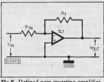
Fig.8. Defined gain inverting amplifier
