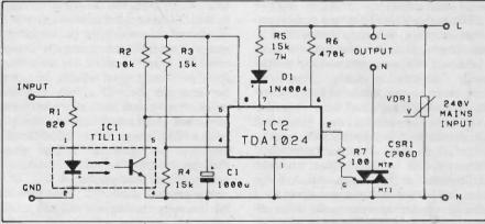
Fig 5. Mains controller circuit incorporating zero crossing detector
