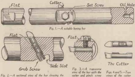
Fig. 2.—A sectional view of the bar showing the position of the cutter
