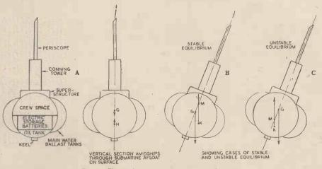
Fig. 4.—Showing how a submarine can recover from a list
