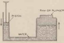
Illustrating the principle of the hydraulic press which Bramah raised to the status of an engineering creation
