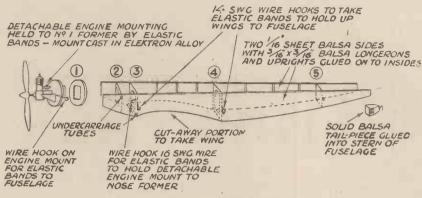
Fig. 3.—Method of assembling the fuselage
