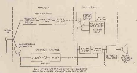
Fig. 1.—Simplified circuit diagram of the Vocoder
