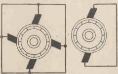
Fig. 3.—(Left) Brush connections for a two-pole motor. (Right) Connections for a four-pole motor
