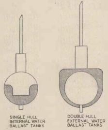
Fig. 2.—Vertical cross sections showing circular pressure hulls and water ballast tanks (shaded)
