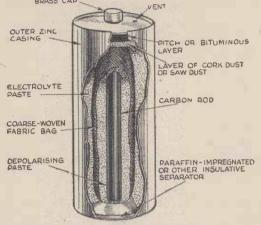
From this diagram the essentials of dry battery construction may be seen at a glance
