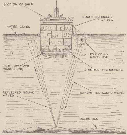
The fundamental principle of the modern "echo" system of ocean depth sounding
