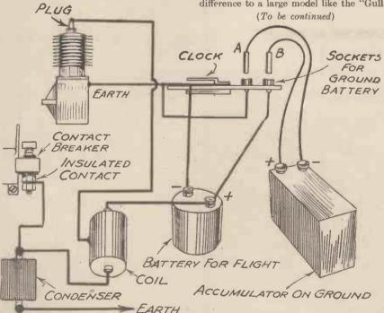
Fig. 4.—Wiring diagram of the ignition system
