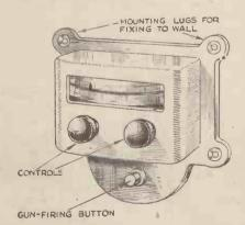
Showing the depth indicator instrument dial by means of which the sound impulse is indicated and the sea depth read off at a glance in fathoms from the calibrated dial
