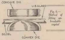
has been strained can be made to snap if a needle is placed between the bezel and the band of the case near the hinge and the bezel forced downwards.
