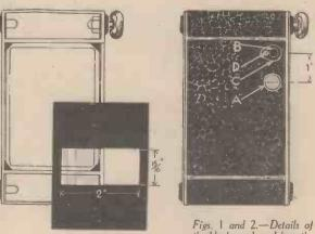
Figs. 1 and 2.—Details of the black mask and how the back cover of the camera is drilled
