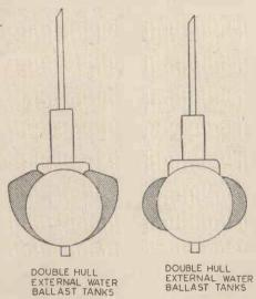
Fig. 3.—Further cross sections (see Fig. 2)
