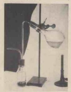
Preparing bromine by heating a mixture of potash bromide, manganese dioxide and concentrated sulphur. The bromine distils over as a heavy red vapour condenses in the bottle
