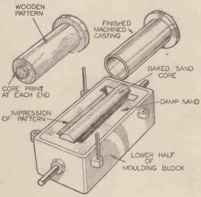
(Left) The principle on which a simple casting is made. The pattern is pressed first into one half of a sand mould, and then into the other. The core, made from sand, bound with oil and baked, is placed between the two halves of the mould when they are assembled. Only the bottom half of the moulding box is shown in the illustration. (Right) Diagrammatic illustration of the method of making a centrifugal casting
