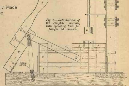
the Pyruma. Thus care should be taken to leave clearance for these holes when making the mould. Some constructors may feel that a bearing sleeve could be inserted with advantage in moving portion E. From personal experience, however, I found this
