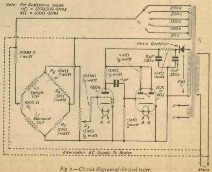
Two identical bobbins are required for the coils, and may be constructed as shown in Fig. 3. The writer used cardboard postal tube with paxolin end cheeks glued to it. The coils are each wound with 8,000 turns of 32 s.w.g. enamelled wire. There is no need to wind in layers; random winding is good enough.
