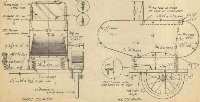
Figs. 1 and 2.—These two views of the side-car show clearly the shape of the body and method of springing.
