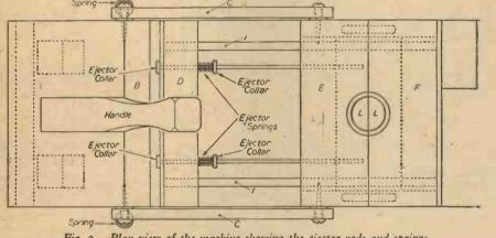
Fig. 2.—Plan view of the machine showing the ejector rods and springs.
