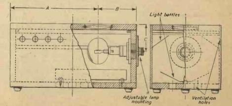
Fig. 4.—General arrangement of lamp housing. Factors governing dimensions: A. Height of draw tube of microscope above base if used as shown in Fig. 2. B. Distance between centre of filament and flange of lampholder plus thickness of inner disc and end of housing. C. Focal length of condensing lens.
