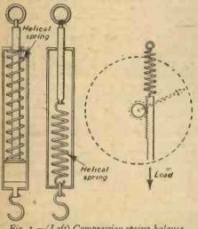
Fig. 1.—(Left) Compression spring balance. Fig. 2.—(Centre) Tension spring balance. Fig. 6.—(Right) Magnifying the deforma-tion of a helical spring with a circular scale.
