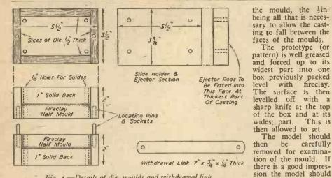
Fig. 4.-Details of die, moulds and withdrawal link.
