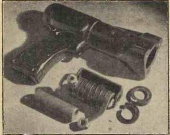
An interesting example of the use of Bakelite plastics is in the production of electrically-operated tools. The body of this D.C. stud welding gun is moulded in a high-strength grade of Bakelite material and incorporates metal inserts, including the heavy copper solenoid shown.
