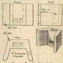
Fig: 2.-Details of the boiler.
