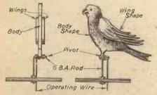
Fig. 4.—Details of the movement for actuating the mechanical "bird."
