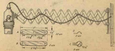
The completed extension bracket, and details of lattice strips and end fittings.
