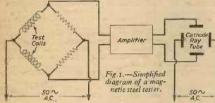
duced into one coil, whilst the sample to be checked is introduced into the other. If the two are identical with regard to chemical composition, hardness, tempering, grain size, etc., then the bridge will remain balanced. But if the sample differs from the standard in any respect, then an out-of-balance indication will be obtained from the bridge.
