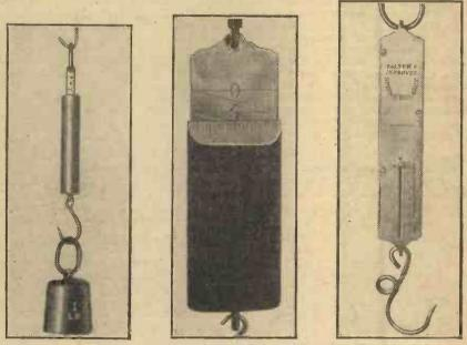
Fig. 3.—(Left) The earliest type of spring balance made first by Richard Salter about 1790. This exact copy was made in 1825 by William Salter. Fig. 4.—(Centre) This balance is described and illustrated in the Patent of George Salter No. 7724, dated 1838. Note the method of indicating weights by means of parallel and diagonal lines marked on the slide and divisions on the external tube. Fig. 5.—(Right) Type of balance used in the middle of the last century.
