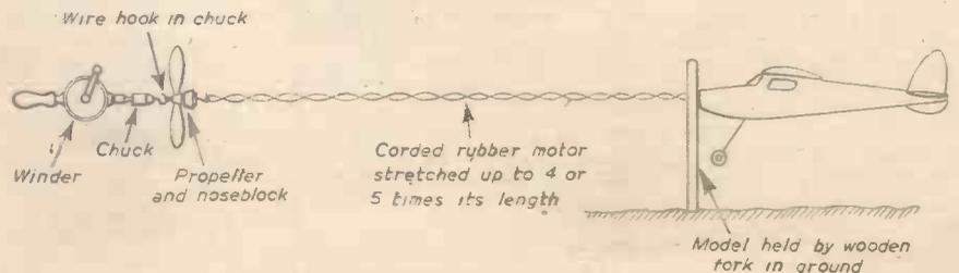
Fig. 7.—Stretch-winding a "corded" motor.
