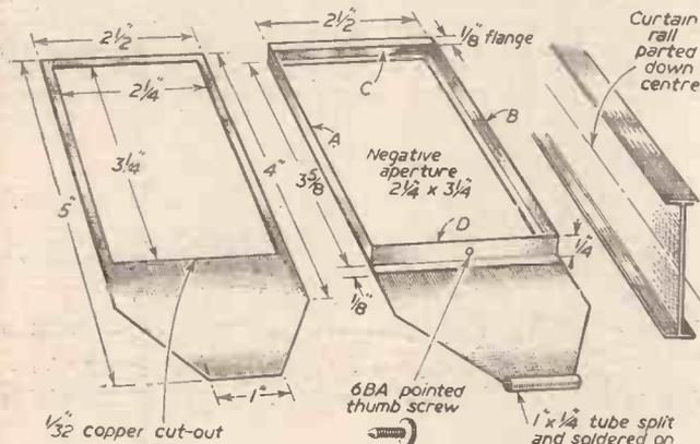
Fig. 3.—Details of negative carrier.
