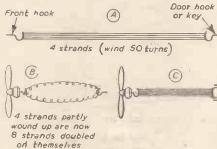
Fig. 6.—Make up the motor as at A; double the 4 strand skein over the propeller hook as at B, so that the motor becomes 8 strands. Allow the motor to go slack as at C.
