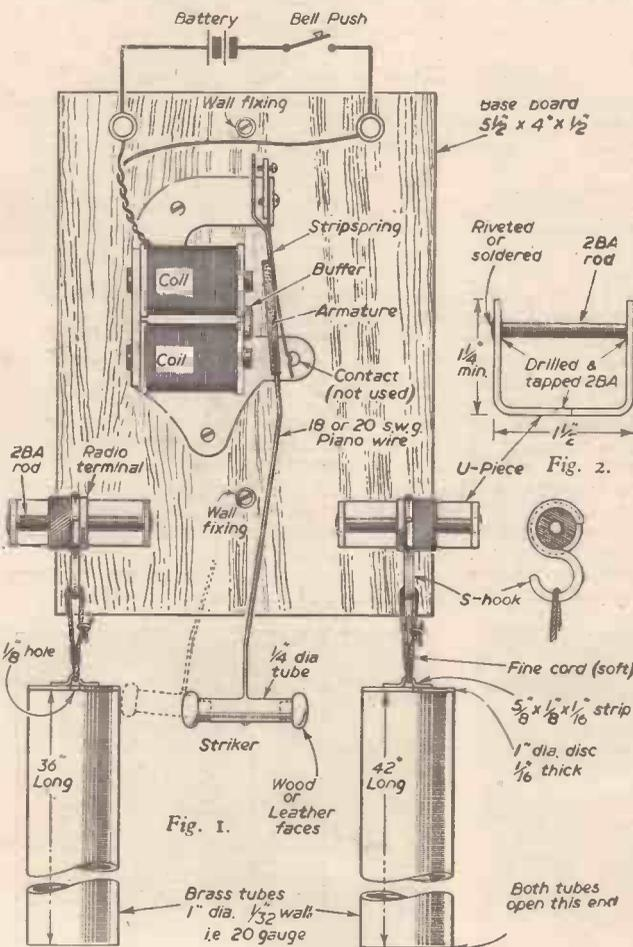
Figs. 1 and 2.—General arrangement of door chime mechanism, and detail of chime supports.
