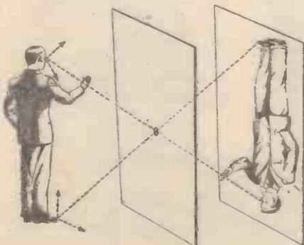
Fig. 1.—Diagram showing image formation.
