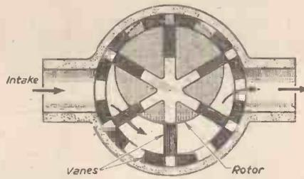
The Cozette supercharger. An inner rotor revolves at the same speed as the outer revolving vanes.
