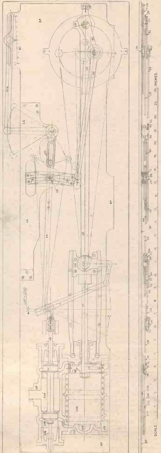
Fig. 5.—Elevation and sectional plan of a valve-gear flat model.
