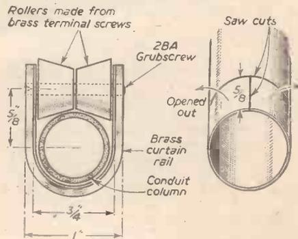
Fig. 4.—Details of rollers.
