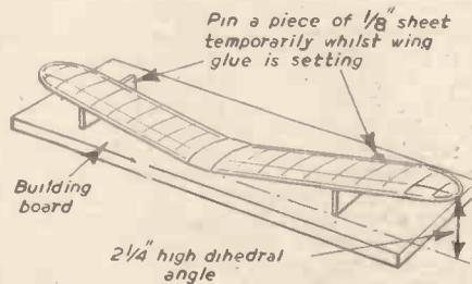
Fig. 4a.—Setting the wings to the correct dihedral on a building board.
