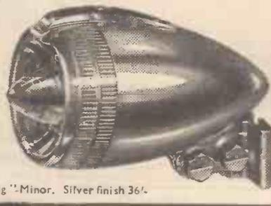
The "King" Minor has a 2 1/2" dia. 5 1/2 oz. headlamp with silver plated brass reflector and single bulb type "light unit" which with central conical lens formation provides ample local light while projecting an intense spot beam. Push-in sleeved connectors allow for variable cable lengths.
