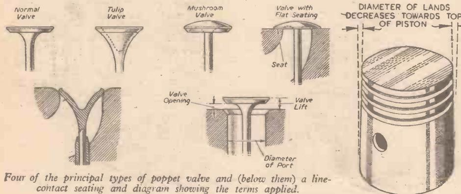
Four of the principal types of poppet valve and (below them) a line-contact seating and diagram showing the terms applied.
