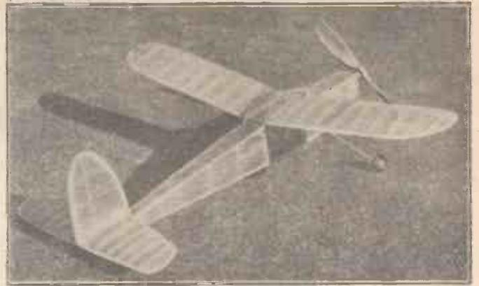
Fig. 5.—Not a wrinkle should be visible on the finished monoplane.
