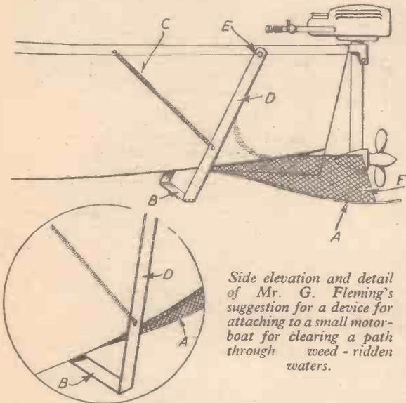
The barge was the first for some time to use this section of the canal, and apparently they had trouble farther down with weeds. The scythes were held inwards, and as they cut the weeds the bow-wash drew them out from underneath and left the screw in clear water.
