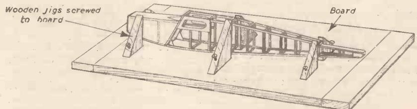
Fig. 3.—Keeping the fuselage true by simple jigs screwed to the building board for keeping the fuselage upright and free from twists as the cement sets.
