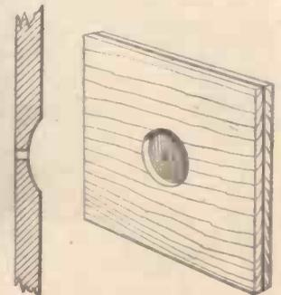
Fig. 2.—Enlarged section of pinhole and detail of mounting.
