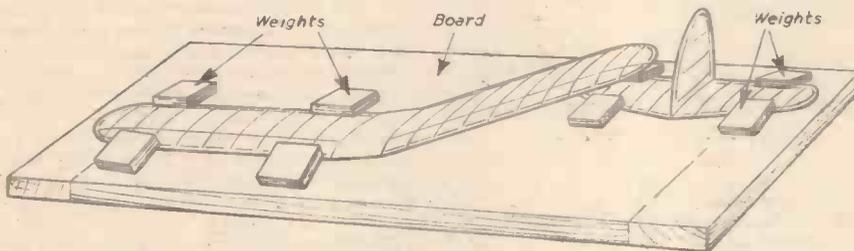
Fig. 4.—Weighting the wing surfaces prevents warping whilst the dope dries. Dope each wing separately, and add weights carefully. Do not apply weights until dope is sufficiently dry to prevent sticking to board.
