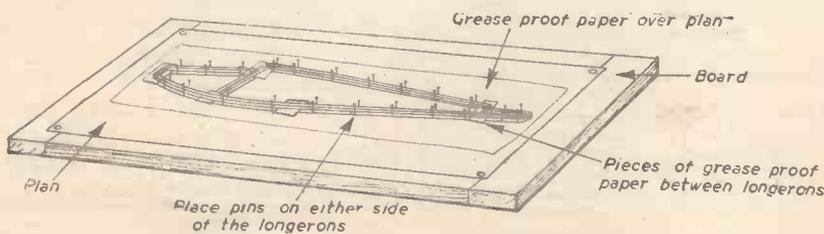
Fig. 2.—Pinning down the fuselage outline to the building board.
