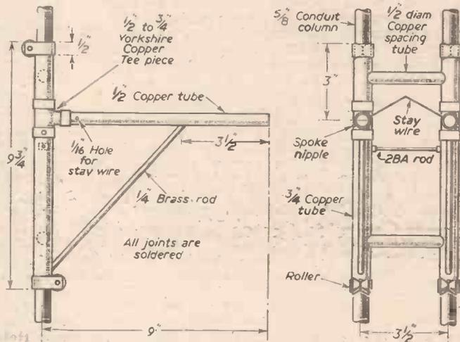
Fig. 2.—Details of bracket.
