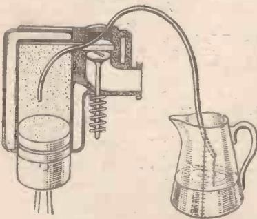
Method of extracting the oil from the cylinder.
