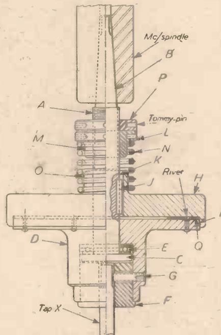
Half-sectional elevation of a friction-driven tap-holder.
