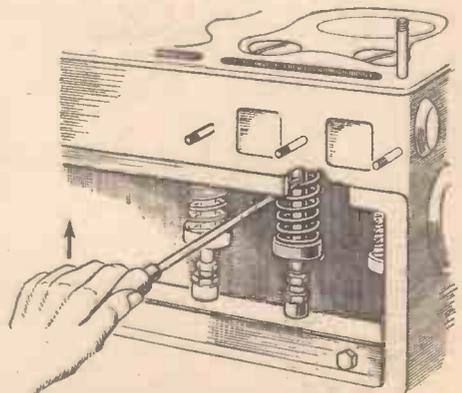
Detecting a weak spring by inserting a screw-driver in the coil.
