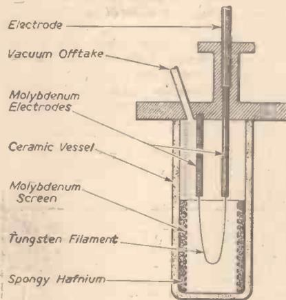
Apparatus for the production of iodide hafnium.
