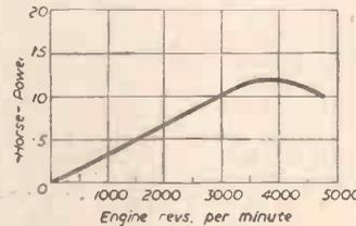
(Left) Graph showing how supercharging raises the point at which power begins to fall off. (Right) Graph showing how the power of an engine falls off after the attainment of maximum engine speed.
