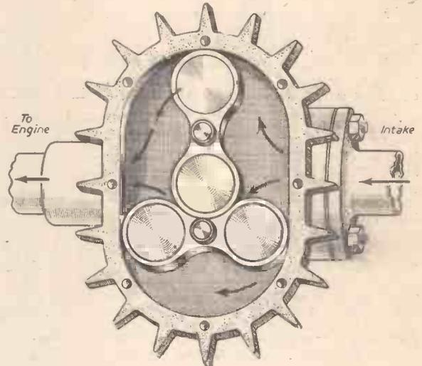
The Roots supercharger for increasing the power of the engine.
