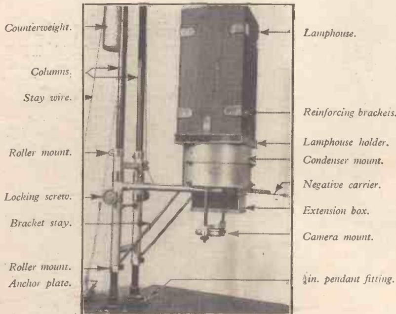
Fig. 5.—Side view of the enlarger, indicating the various component parts.
