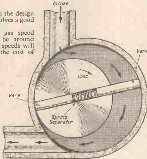
The Zoller supercharger employs a pair of vanes separated by a spring they are attached to and rotate by an eccentric.
