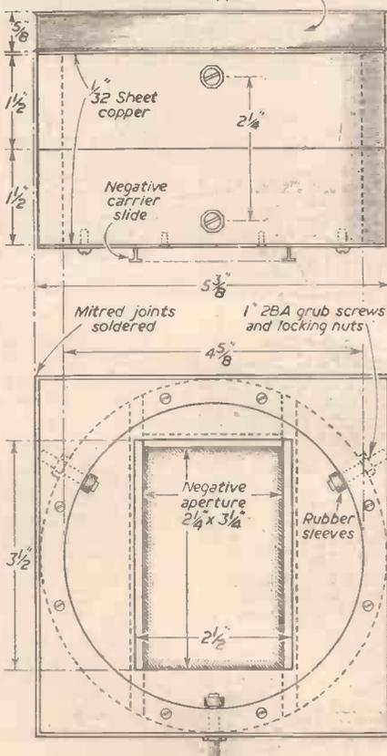
Fig. 1.—Elevation and plan of condenser mount.
