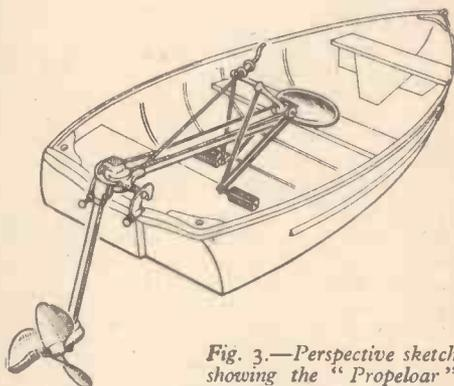
Fig. 3.—Perspective sketch showing the "Propeloar" in position on a small boat.
