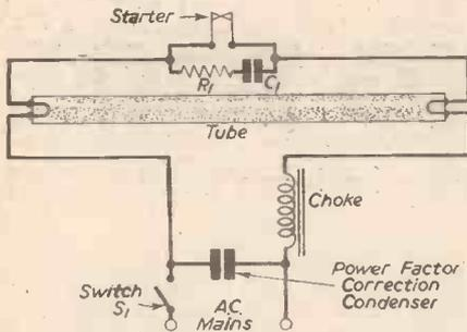
Fig. 1.—Circuit diagram for a single fluorescent tube.
