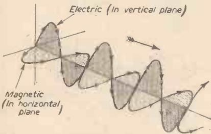
Fig. 2.—Graphical representation of an electro-magnetic wave.
