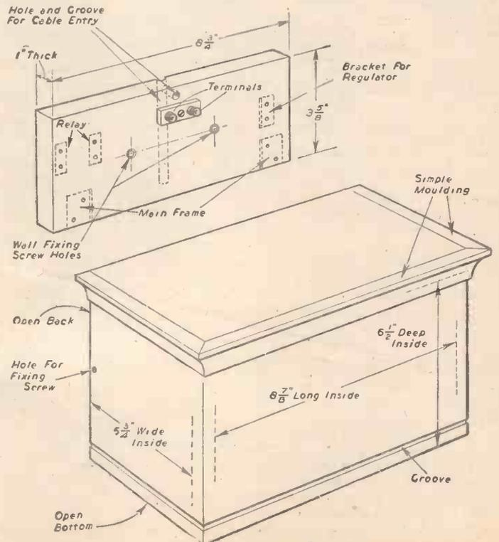
Fig. 9 (Right).—Details of backboard and cover box.
