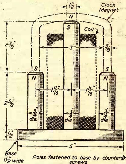
Method of re-magnetising a Bulle clock magnet by means of a powerful electromagnet.
