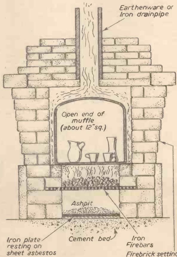
Sectional diagram showing the inner and outer construction of a simple pottery kiln.
