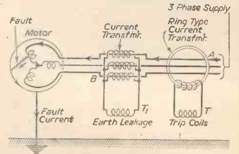
Fig. 7.—Connections of two types of current-operated earth leakage trips.
