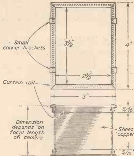
Fig. 11.—Plan and side elevation of extension box.
