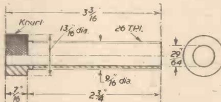
Fig. 2.—Section and end view of the internal sleeve.
