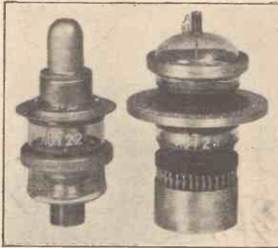
Fig. 12.—Forced air cooled ultra-high frequency triodes (1,000 Mc./sec.).
