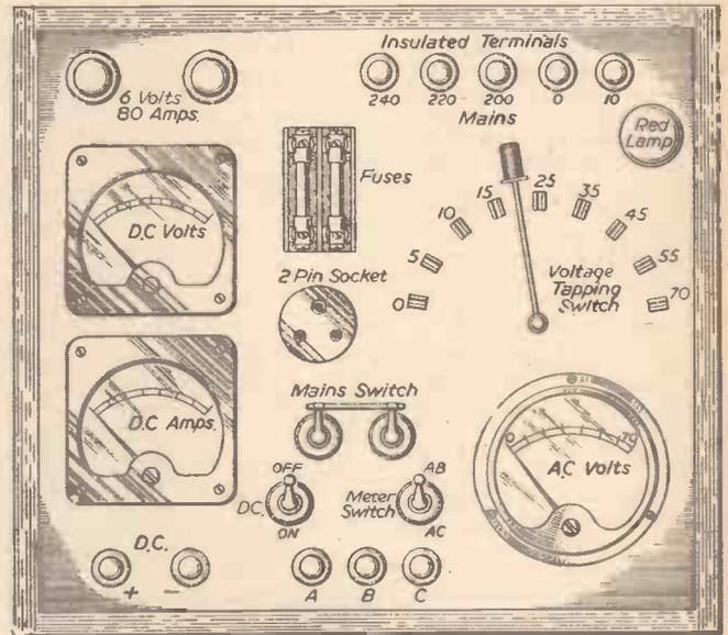
Fig. 1.—The panel of the control box.
