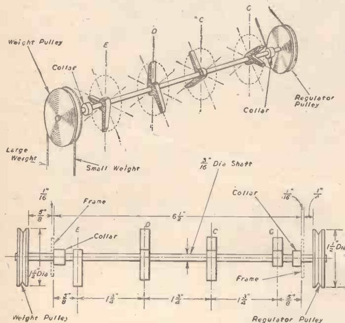
Fig. 7 (Above).—Perspective view and plan of camshaft.
