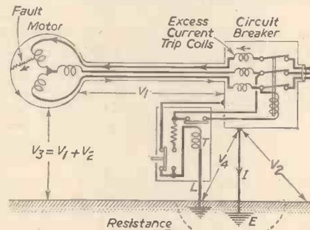
Fig. 6.—Incorrect location of earth electrode for voltage-operated leakage trip.
