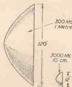
Fig. 3 (Left).—Relative size of parabolic reflectors required to produce identical beams at various frequencies.
