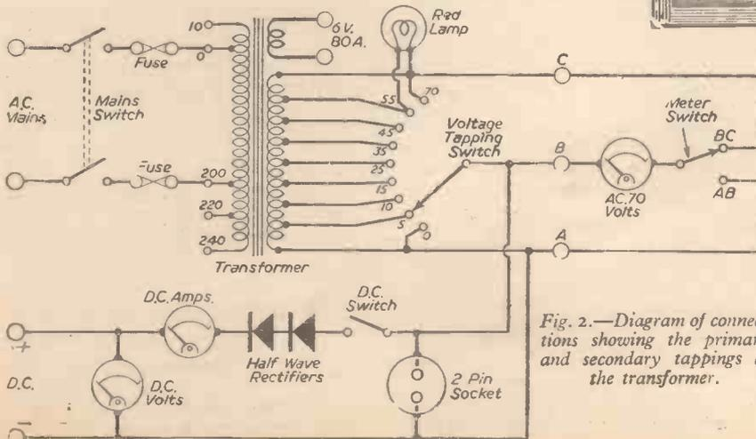
Fig. 2.—Diagram of connections showing the primary and secondary tappings of the transformer.
