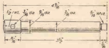
Fig. 4.—The main spindle, showing the hole for tommy bar, and threaded end for cutter.
