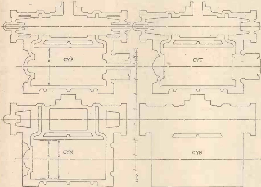
Fig. 6.—The four plates which make up the cylinder.
