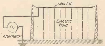
Fig. 9.—Simple aerial circuit.
