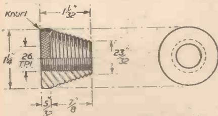
Fig. 3.—Part section and end view of the taper-screwed body.
