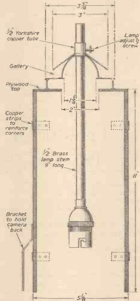
Fig. 7.—Sectional view of lamphouse and gallery.
