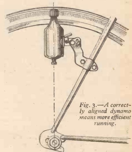
Fig. 3.—A correctly aligned dynamo means more efficient running.
