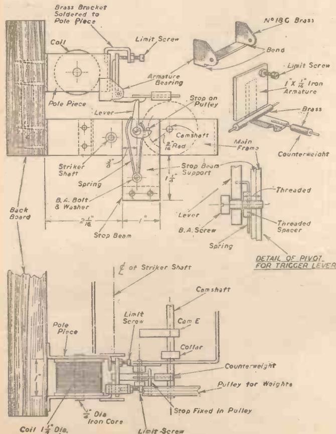
Fig. 3 (Left).—Details of trigger mechanism and relay, and section showing pivot for trigger lever.
