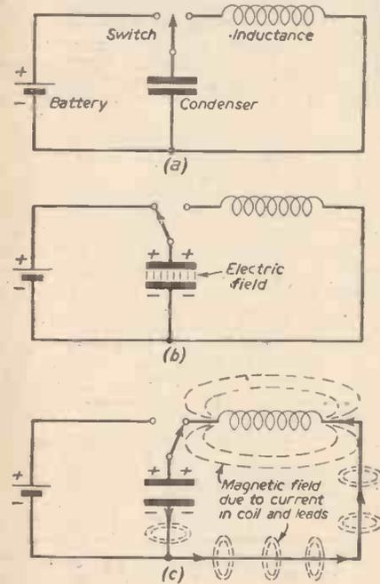
Fig. 5.—Simple oscillatory circuits.
