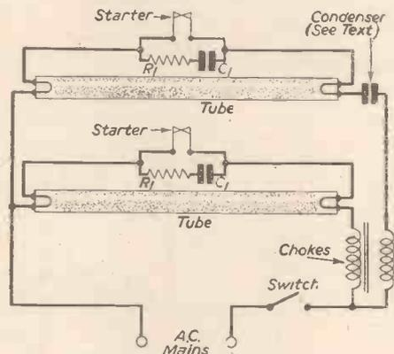
Fig. 2.—Circuit arrangement for twin tubes.
