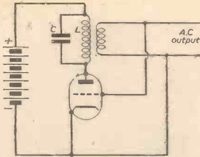
Fig. 10.—A simple valve oscillator circuit.
