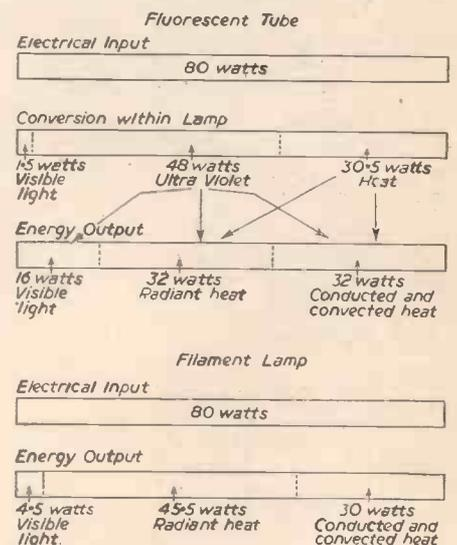
Fig. 3.—The relative efficiency of a fluorescent tube and a filament lamp.
