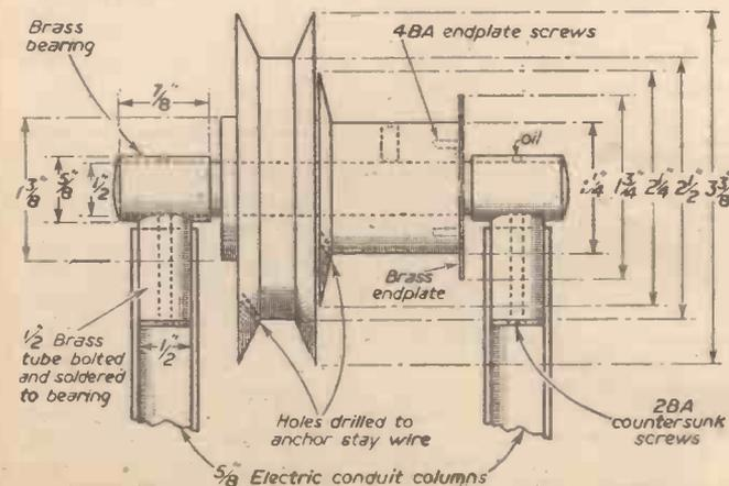
Fig. 9. (Left).—Part sectional view showing details of pulley assembly.
