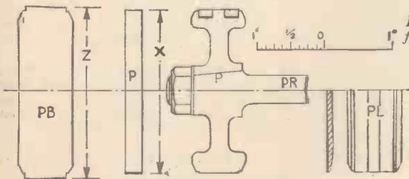
Fig. 8. (Right)—The four parts for forming the crosshead.
