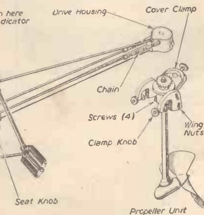
Fig. 1.—Diagram showing the layout of the various parts of the "Propeloar."
