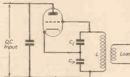
Fig. 11a.—Colpitts feedback oscillator circuit.
