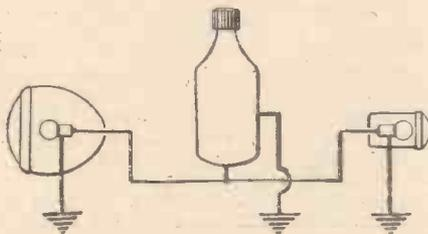
Fig. 1.—The lamps are connected in parallel with the dynamo, and earthing may be carried out either by using the mounting brackets or by connecting the casing of the two lamps to the dynamo casing by means of wires.
