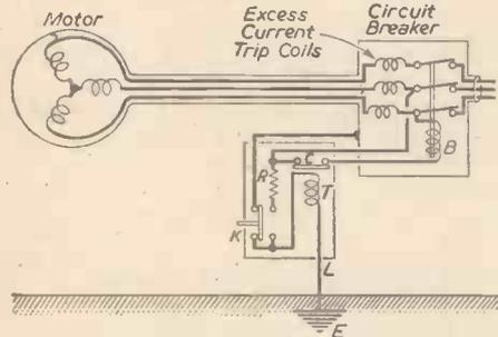
Fig. 5.—Connections of a voltage-operated trip in a three-phase motor circuit.
