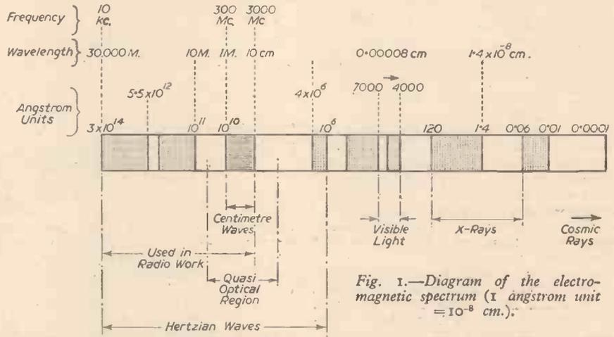
Fig. 1.—Diagram of the electro-magnetic spectrum (1 angstrom unit =  $10^{-8}$  cm.).
