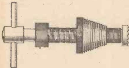
Fig. 1.—The completed re-seating tool.
