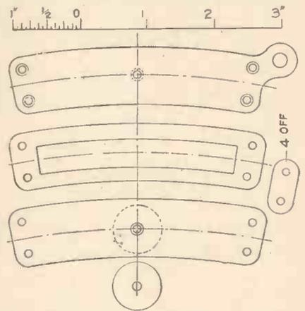
Fig. 9.—The plates for forming the expansion link.
