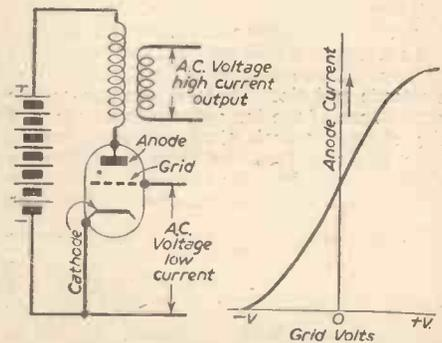
Fig. 8.—Simple triode amplifier.
