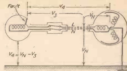
Fig. 3.—Conditions with earth fault on live side of single-phase apparatus with unearthed metallic sheathing.
