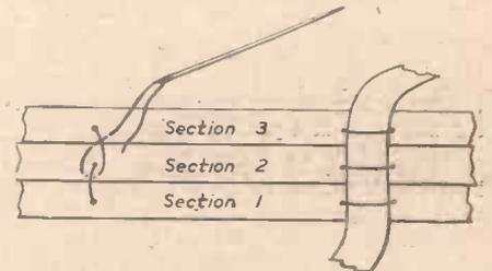
Fig. 3.—The kettle stitch. Thread shown dotted where passing under.
