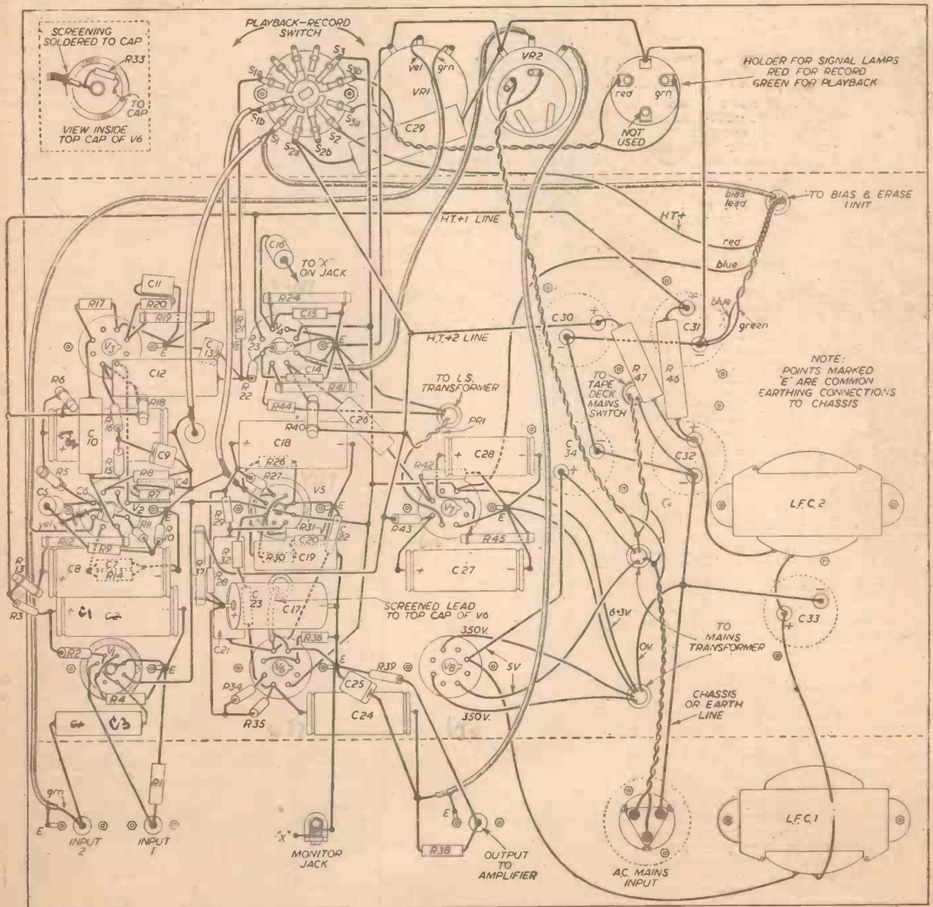
Fig. 8.—Detailed illustration of the wiring of the chassis. See text regarding the connections made to the various tags marked "E."
