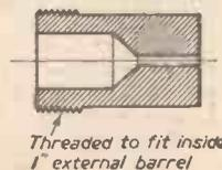
Fig. 3.—Jet turned up on the lathe.
