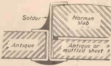
Fig. 3.—Method of double plating.
