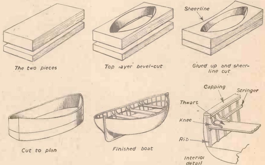
Fig. 2.—Various stages in the construction of fully-detailed boats.
