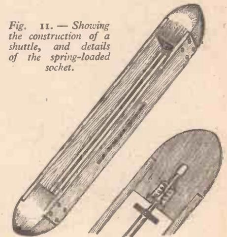
Fig. 11.—Showing the construction of a shuttle, and details of the spring-loaded socket.
