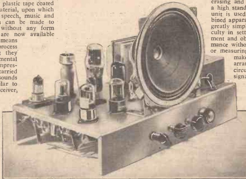
The amplifier unit of the tape recorder
