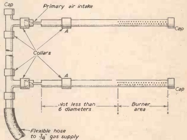
Fig. 1.—Showing the method of connecting the burner bars to the main stem of the gas supply.
