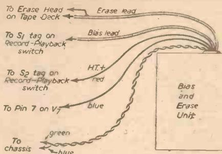
Fig. 6.—The Bias and Erase unit with details of the connections.
