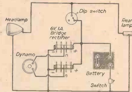
Fig. 2.—Lighting system for a motor-assisted bicycle.
