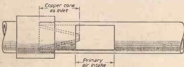
Fig. 2.—Showing injector made by rolling a copper cone and brazing into mouth of the burner.
