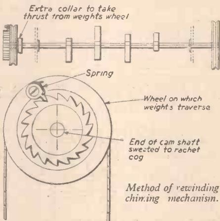
which the weights are suspended) the wheel on which a ratchet is fixed revolves freely on the camshaft. Engaging the ratchet is a cog-wheel which is sweated to the camshaft end.
