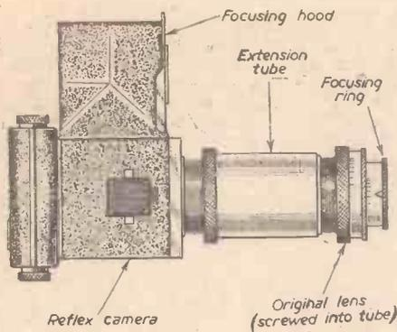
Fig. 3.—Using extension tubes for close-up shots.
