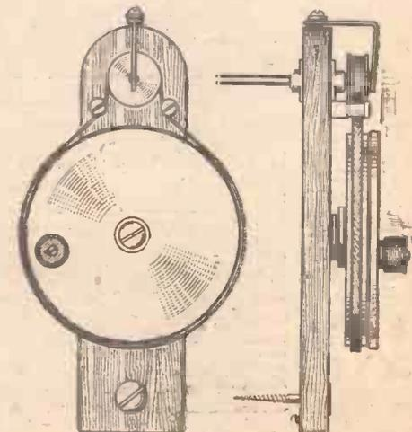
(Left) Side view showing heddle lever construction and mounting—one up and one down. (The hook on reed mounting is to hold weft threads which are not in use out of the way when using several shuttles.
