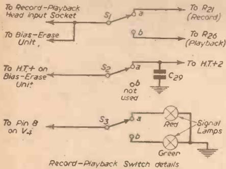
Fig. 5.—Details of wiring of the change-over switch.
