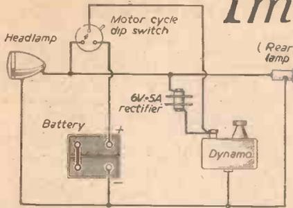
Fig. 1.—Stationary light for use with a dynamo.
