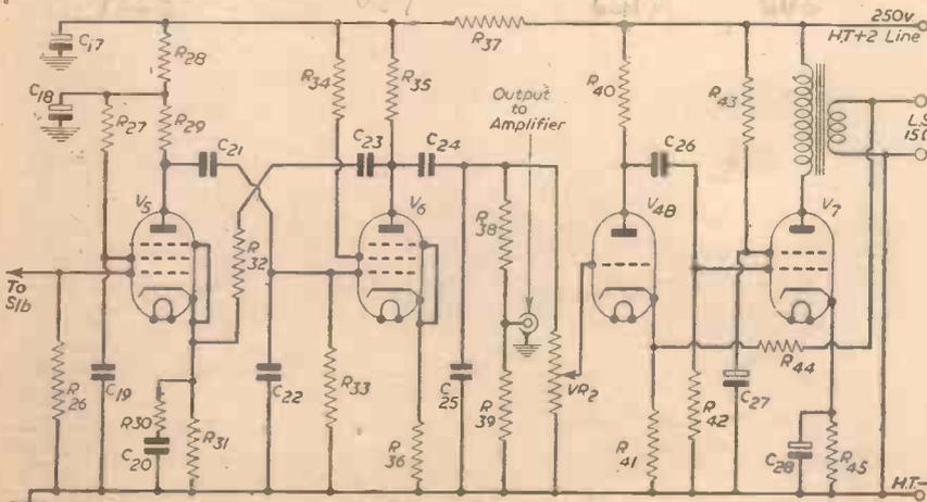
Fig. 2.—This is the play-back section of the instrument.
