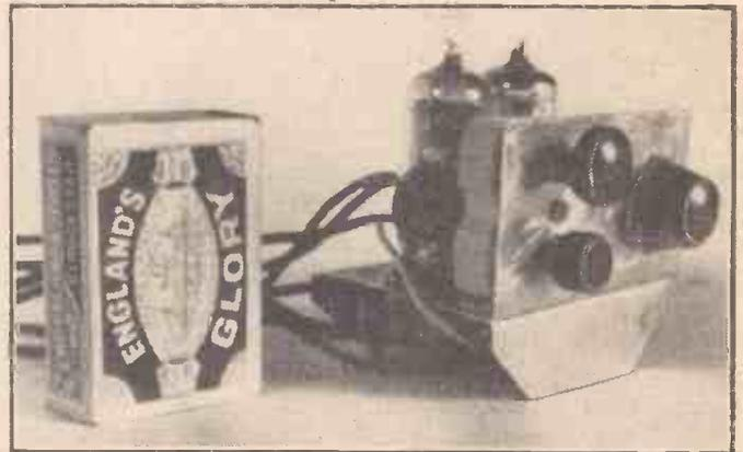
Miniature 2-valve radio made by the writer shown in comparison with a matchbox. (The original photograph showed the set approximately full size.)
