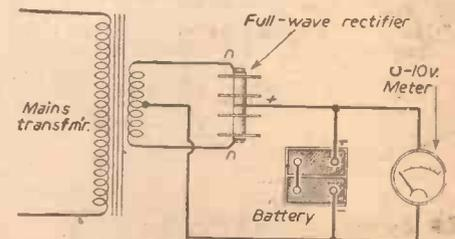
Fig. 3.—Circuit for charging the accumulator from the mains.
