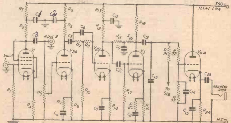
Fig. 1.—Theoretical circuit of the recording section of the equipment.
