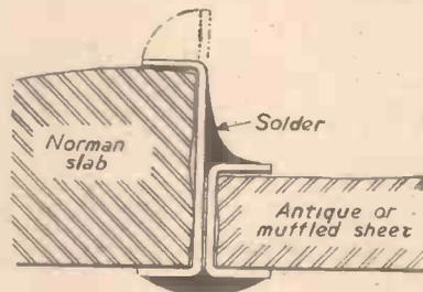
Fig. 2.—Leading up thick and thin glass.
