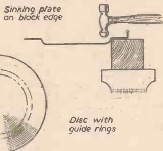
Fig. 1.—Shaping the blank.
