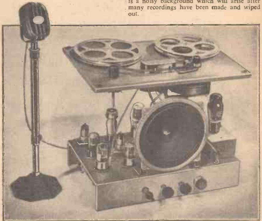
This illustration shows the chassis and tape deck out of the cabinet, and also the microphone.
