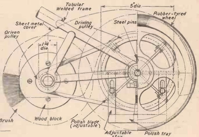
Figs. 1 and 2. Part sectional front and side views of the completed floor polisher.
