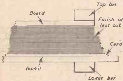
Fig. 5.—Book between boards in clamps, showing the edge partly cut.
