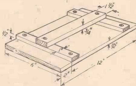
Fig. 3.—Details of a wooden float.
