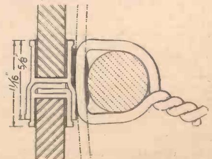
Fig. 5.—An orthodox make-off joint and wire tie.
