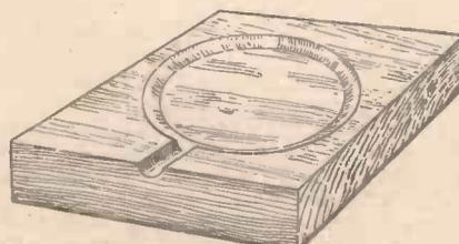
Fig. 4.—A wooden mould for small work.
