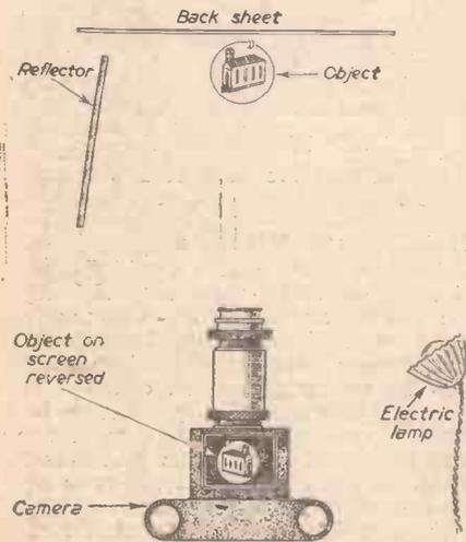
Fig. 4.—A useful lighting arrangement when taking photographs indoors.
