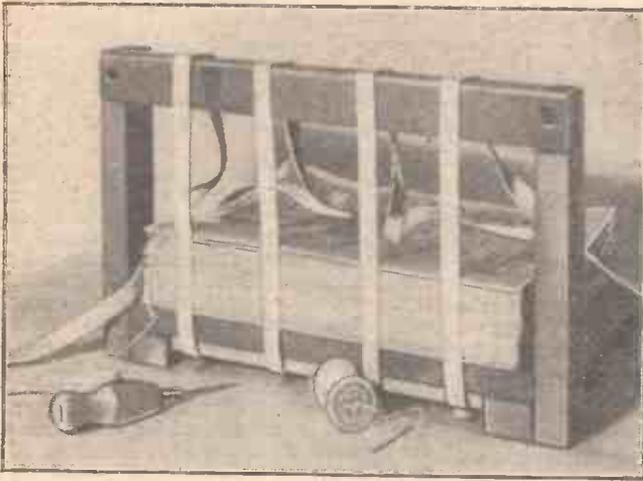
Fig. 2.—The volume being sewn. Twenty-three issues of *Practical Mechanics* are seen on the sewing frame. The bodkin is for beginners use.
