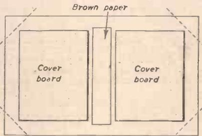
Fig. 6.—The cover cloth freshly glued with cover boards and brown paper in position ready for folding the cloth over.
