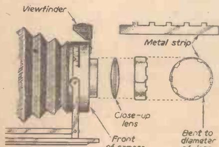
Fig. 1.—A push-on holder for close-up lens made from metal strip.
