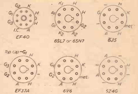
Fig. 7.—Valve-pin details of the various valves used in the Recorder.
