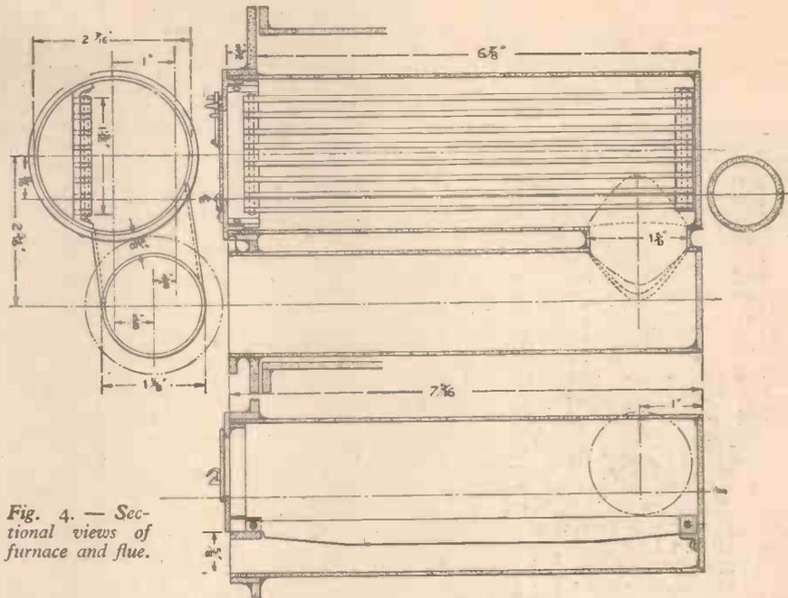
Fig. 4. — Sectional views of furnace and flue.
