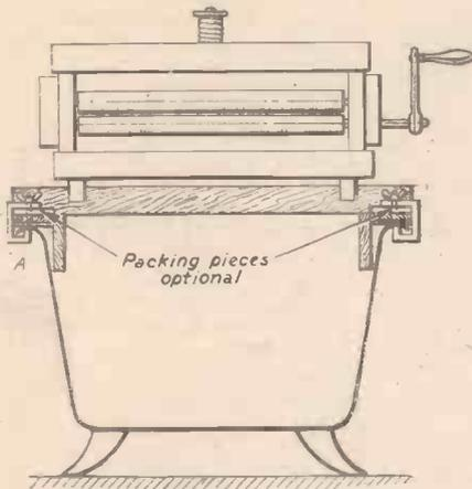
Fig. 1.—Showing the wringer in position on a bath.
