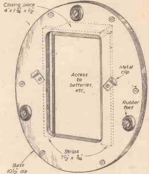
Fig. 7.—Views of the base and lead box.
