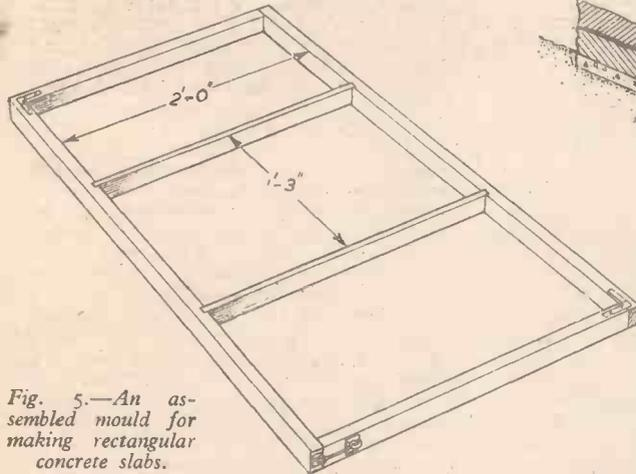
Fig. 5.—An assembled mould for making rectangular concrete slabs.
