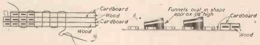
Fig. 3.—How the body of the ship is formed. Fig. 4.—Details of the bridge, funnels and boats.
