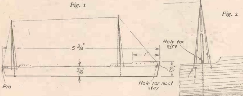
Figs. 1 and 2.—Details of the hull, masts and rigging.
