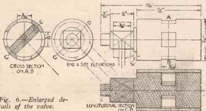
Fig. 6.—Enlarged details of the valve.
