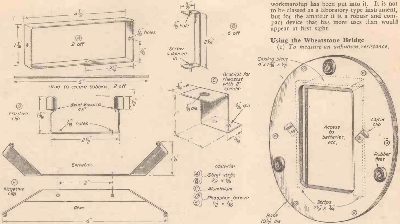
Fig. 5.—Details of the metal brackets and clips.
