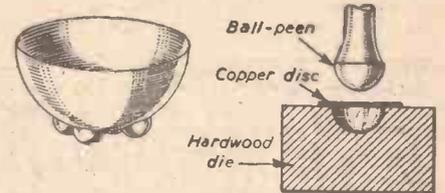
Fig. 4.—Method of forming hemisphere feet.
