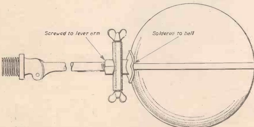
Fig. 1.—Showing how the fitment is attached to the ball valve and the end of lever arm.
