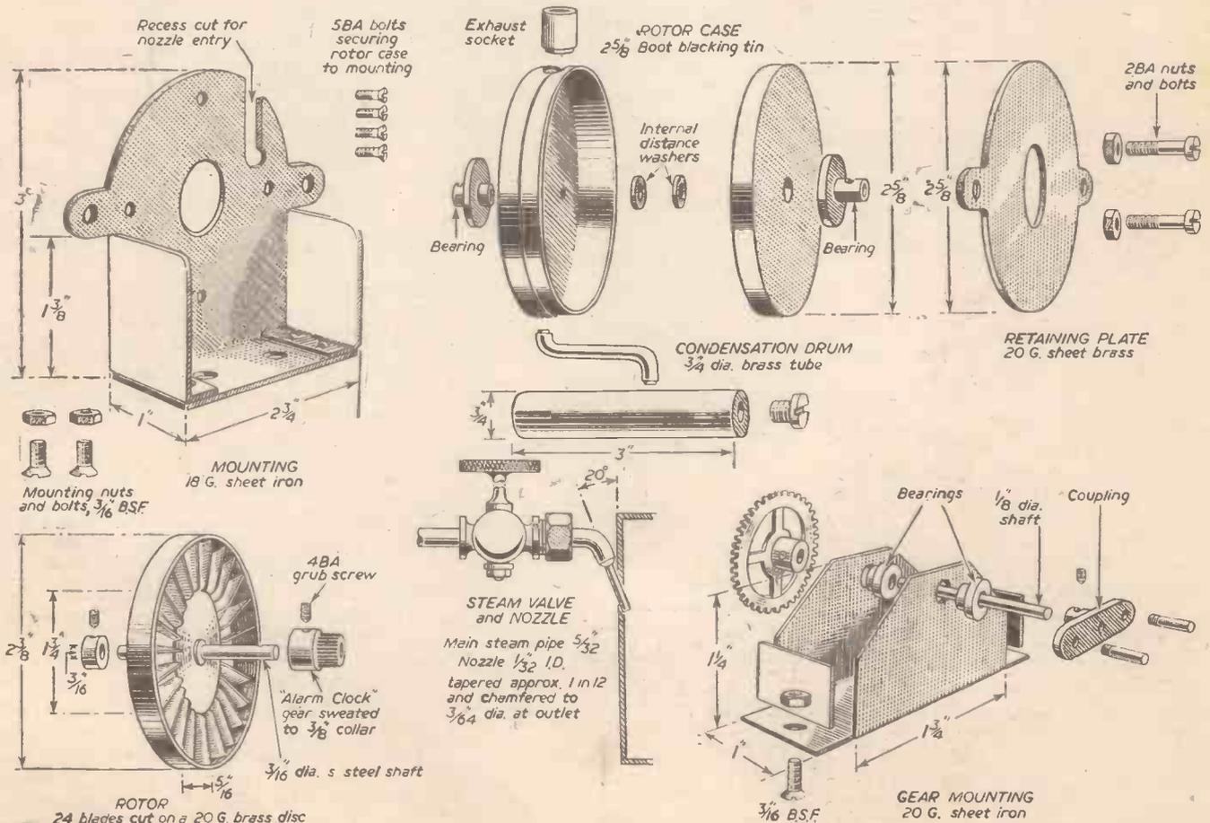
Fig. 1.—Details of the turbine and gear-case components.
