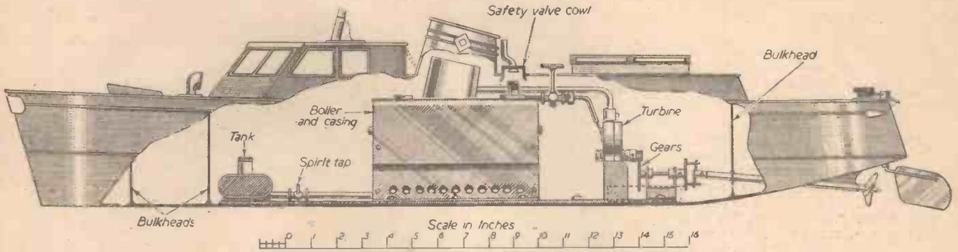
Fig. 3.—Showing the location of the turbine power unit in a model boat.
