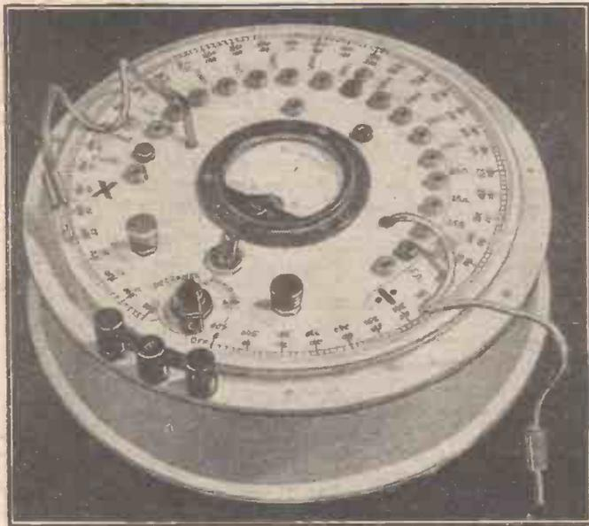
General view of the Wheatstone bridge testing set, showing the circular slide wire beneath the dial.
