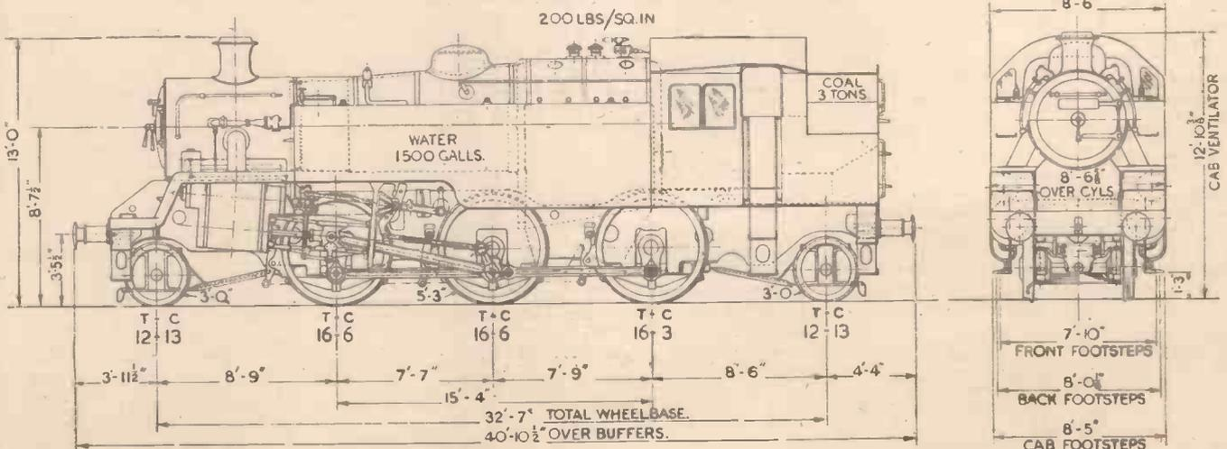
Side and front elevations of the new locomotive, giving some of the leading dimensions.
