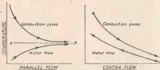
Fig. 2.—Parallel flow gives a low water temperature and high gas temperature. AB represents the theoretical limit of both. Contra-flow gives higher possible water temperature and lower gas temperature, hence higher efficiency.
