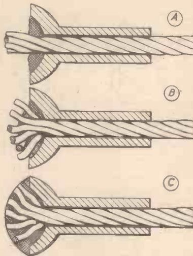
Fig. 2.—A: cable is soldered into the nipple; B: the end is splayed; C: the whole is fixed and sealed with a blob of solder.
