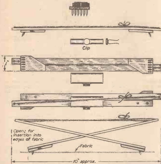
Fig. 14. Details of tenterhooks for fabric up to 15 in. wide.
