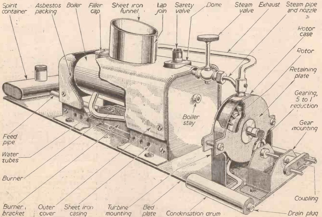
Fig. 5.—Part sectional view of the steam turbine unit for a model boat.
