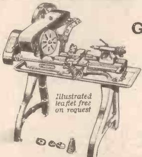
3 1/2in. back geared, screw cutting centre lathe, 18in. between centres. Height of centres, 3 1/2in., swing in gap, 10in. diameter, overall length of bed 34in., overall length of lathe, 41in., bore of headstock spindle 1 1/2in. clearance.
