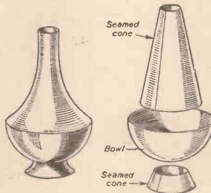
Fig. 3.—Fabricated cone shapes.
