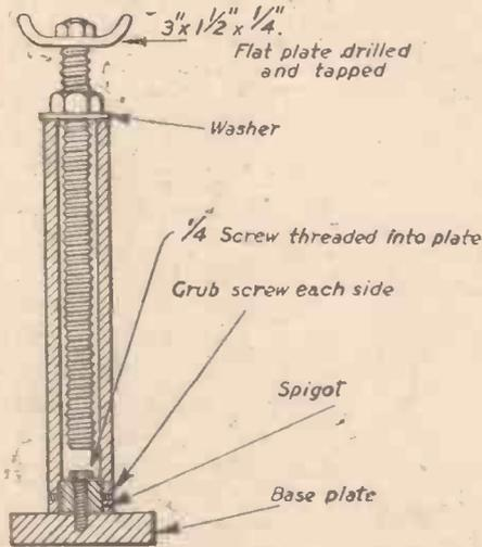
The completely assembled motor-car jack.
