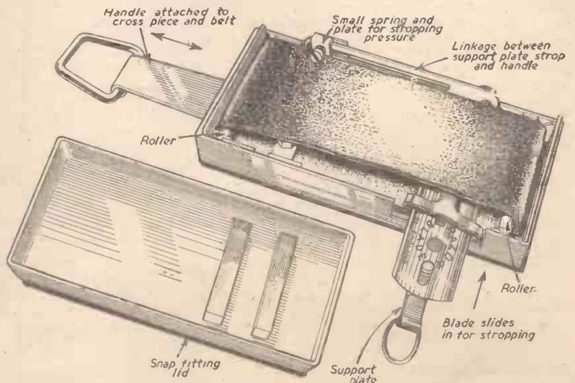
A view of the pocket razor-strop with half of the casing removed showing the interior mechanism.
