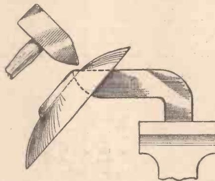
Fig. 1.—Forming a step on the first guide-line.
