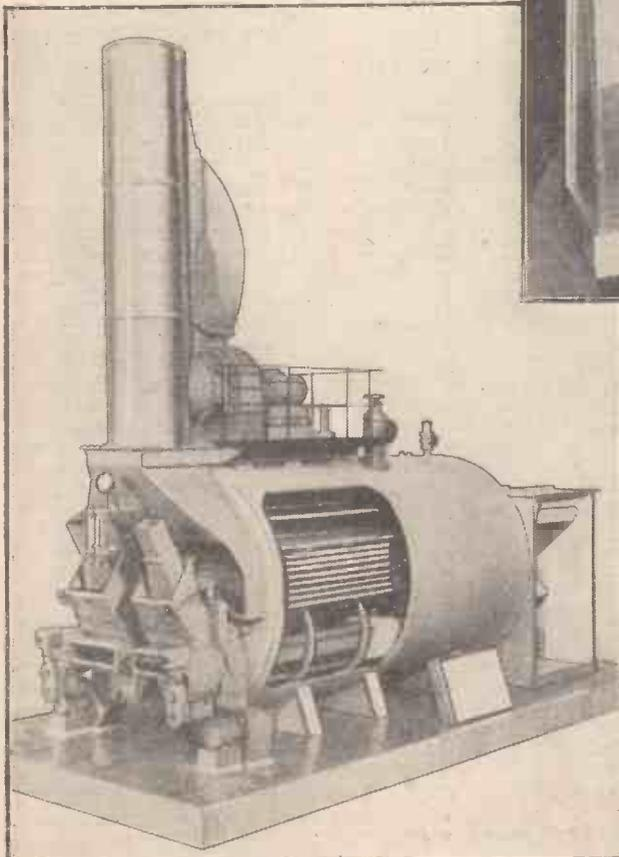
Fig. 3.—A model of Edwin Danks patent high-velocity economic-type boiler, to a scale of 1½ in. to 1 ft. Part of the boiler shell is cut away to reveal the interior.
