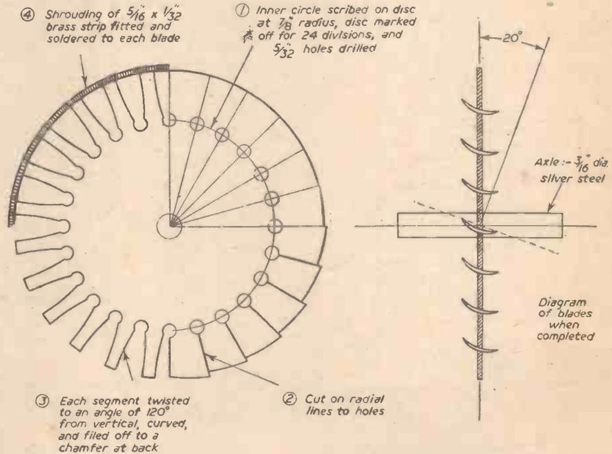
Fig. 2 (Above).—Constructional details of the turbine rotor.
