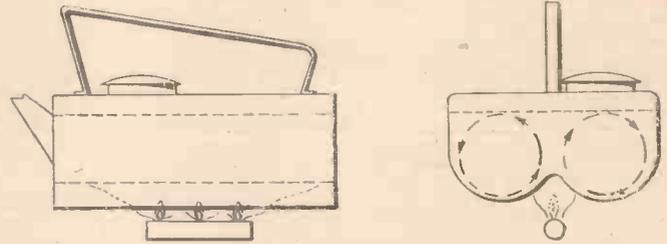
therefore pass through the mass of water as well as round it. A section of the additional outer casing is cut away to allow the gases from the internal tubes to pass directly out to atmosphere.
