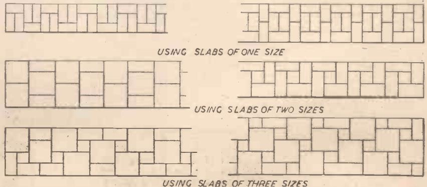
Fig. 2.—Alternative patterns for laying slabs used for paving.
