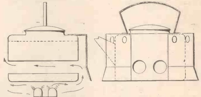
Fig. 5.—Two views of a conventional kettle with the addition of internal tubes and outer casing.
