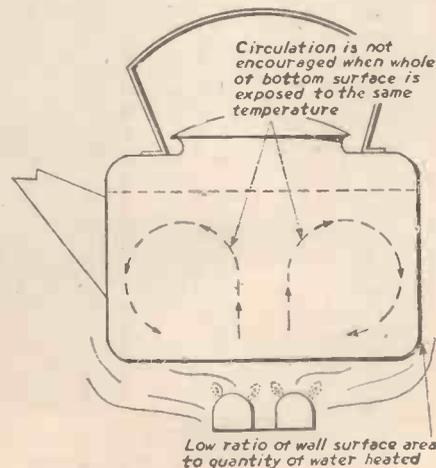
Fig. 3.—The conventional kettle.
