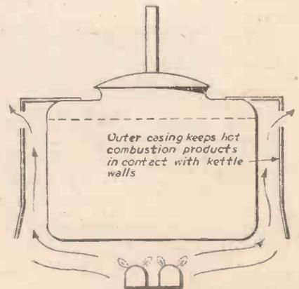
Fig. 4.—Sectional view showing cylindrical casing.
