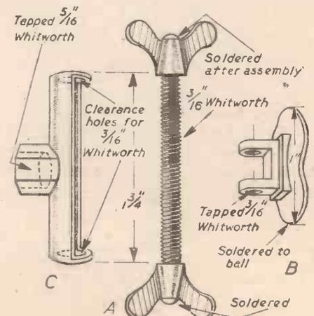
Fig. 2.—Details of the ball-valve adjustment device.
