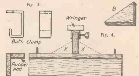
Figs. 3 and 4.—Details of bath clamp, and side elevation of base.
