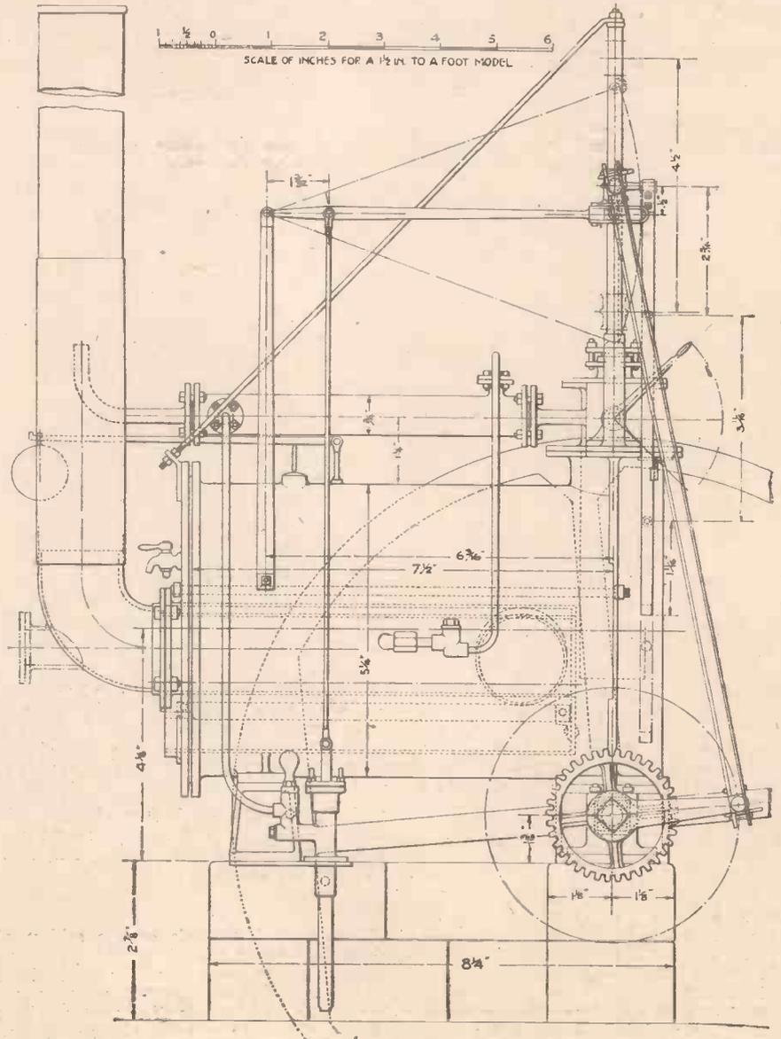
Fig. 2.—Side elevation of the Trevithick model.
