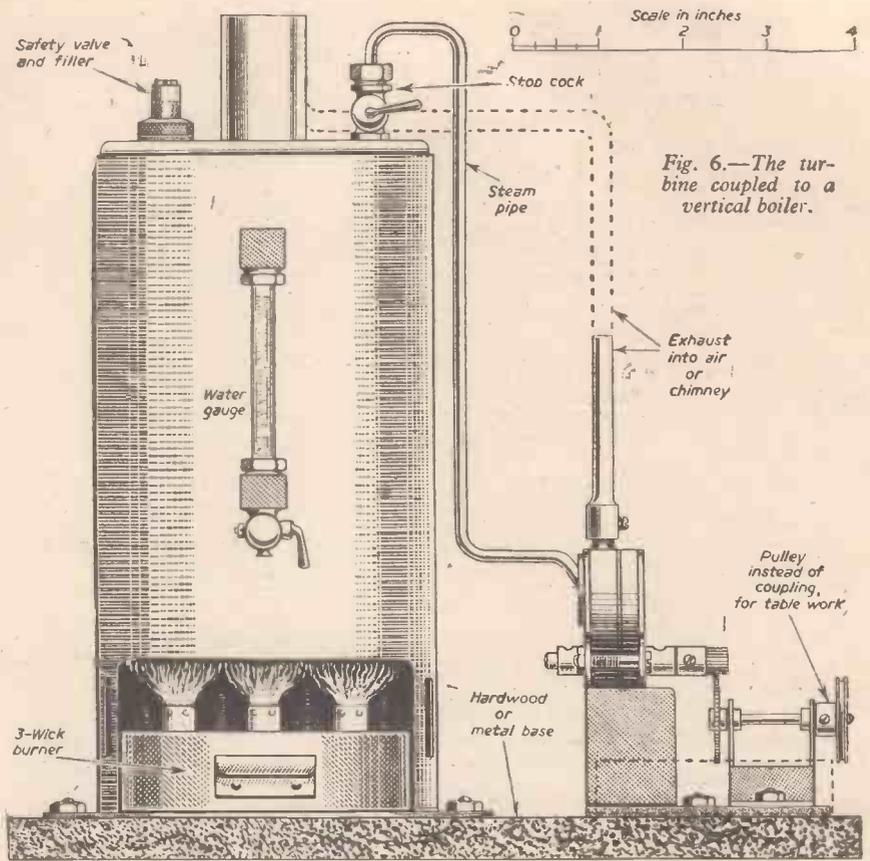
Fig. 6.—The turbine coupled to a vertical boiler.
