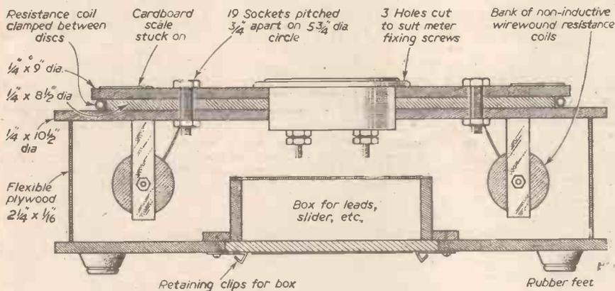
Fig. 4.—Sectional view of the testing set.
