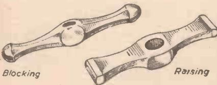
Fig. 2.—Blocking-and raising-hammer heads.
