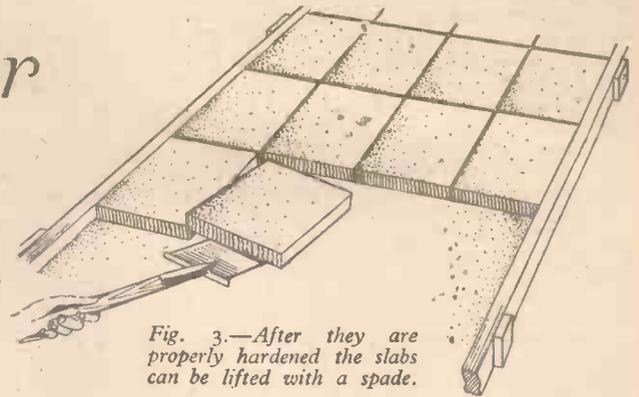
Fig. 3.—After they are properly hardened the slabs can be lifted with a spade.
