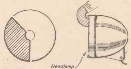
The formation and fitting of the Perspex reflector.
