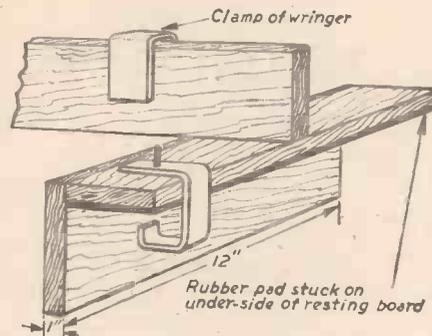
Fig. 2.—Perspective view of wooden base.
