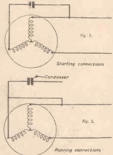
Connections for converting a three-phase motor to single phase.
