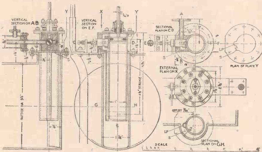
Fig. 5.—Details of the cylinder, valve and piston.
