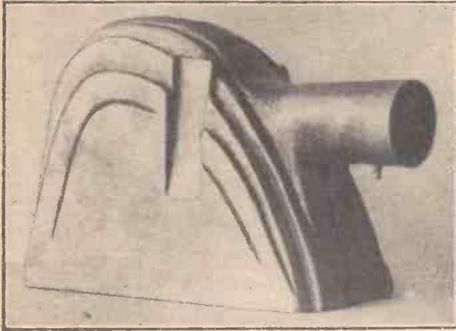
Fig. 1.—An electroformed film-projector housing shown as removed from the plating bath. The former was made of paraffin wax, hand carved.
