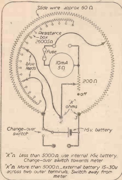
Fig. 8.—Circuit diagram which is stuck on back of lead box.
