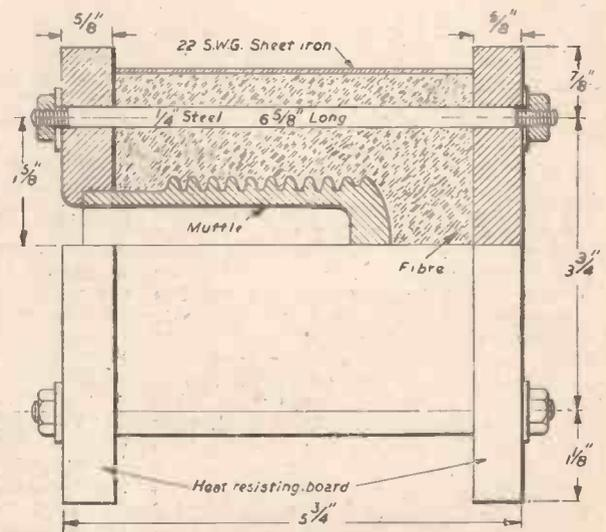
Fig. 2.—A side elevation in part section of a 200-watt electric furnace.
