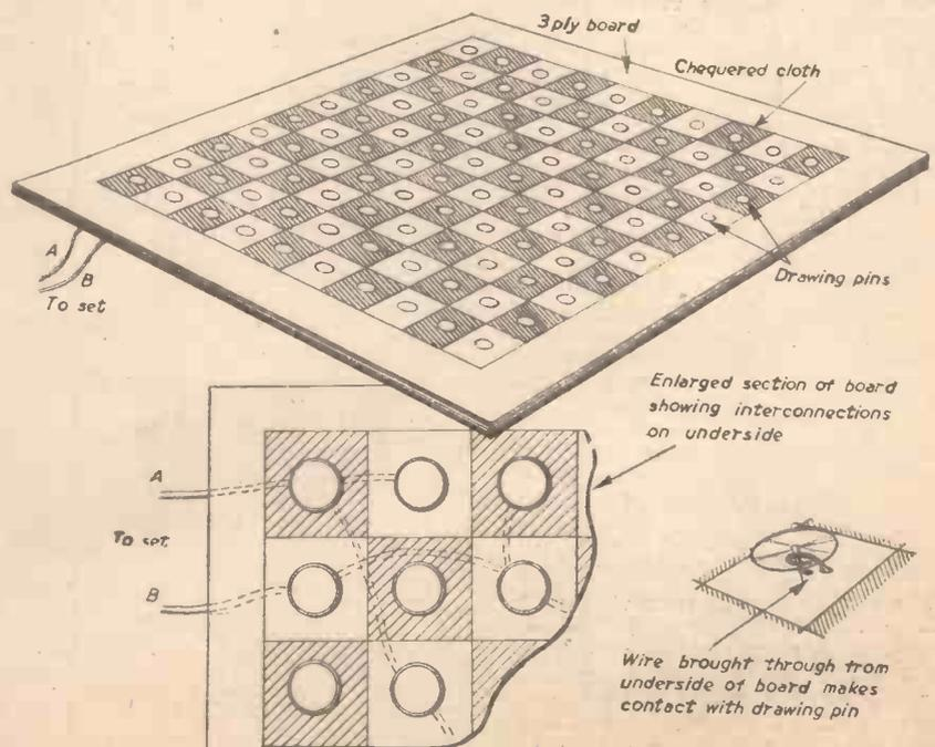
Fig. 2.—An easily made electrical board which can be used with the wireless set to provide entertainment and amusement.
