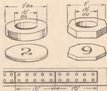
Fig. 8.—Details of the cups and pegging board.
