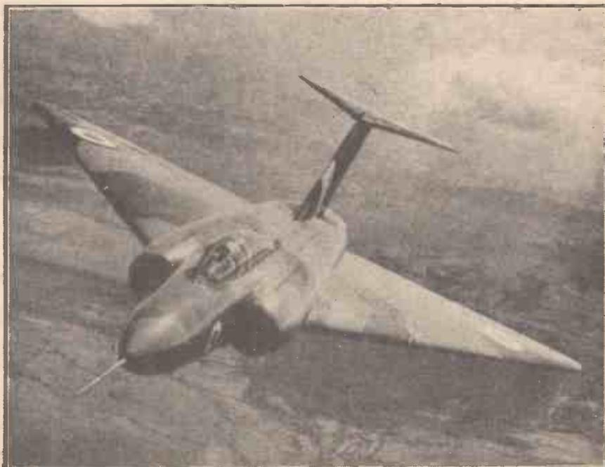
The Gloster GA5 all-weather delta fighter which has been designed for speed, high altitude flying, rapid climbing and manoeuvrability. The machine was seen at the S.B.A.C. Air Display, at Farnborough.
