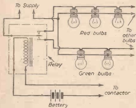
Fig. 1.—Relay circuit for changing colours.
