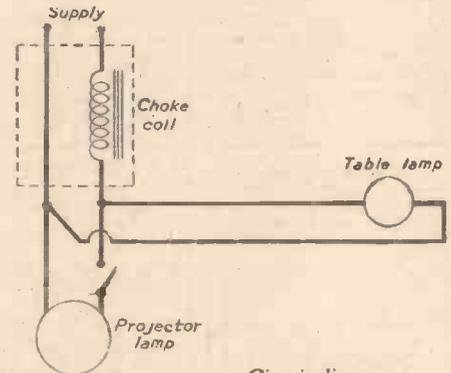
Circuit diagrams of projector switching arrangements.
