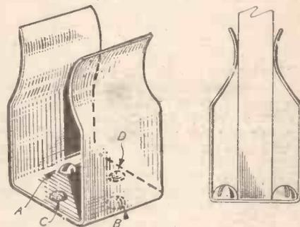
Fig. 5.—How to make the glass clip for Fig. 4. C and D are soldered ends of the contacting wires.
