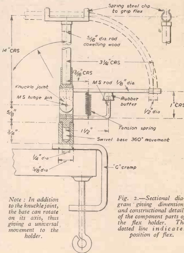
Note: In addition to the knuckle joint, the base can rotate on its axis, thus giving a universal movement to the holder.
