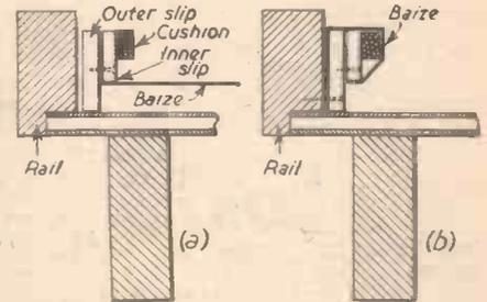
Fig. 7.—Sections of slips and cushions.
