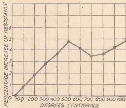
Fig. 3.—Curve relating temperature to percentage increase of resistance for 80/20 per cent. nickel-chrome alloy.
