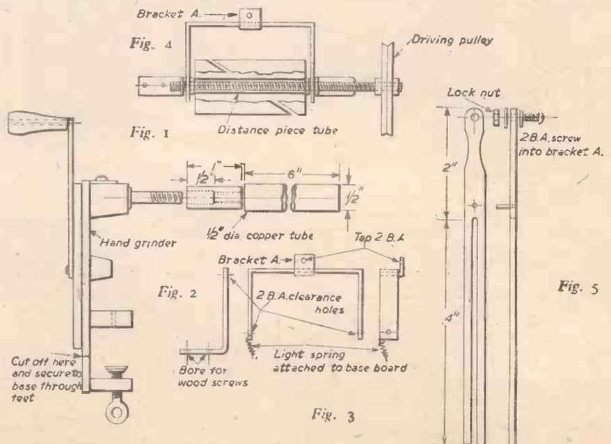
Details of the operating handle, traverser and brackets.
