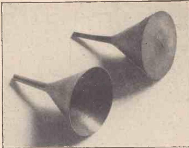
Fig. 5.—Copper funnel electroformed on plastic master shown above.
