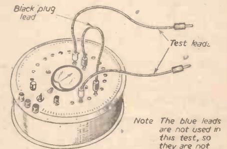
Fig. 11.—Using the instrument as a D.C. voltmeter.
