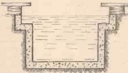
Fig. 5.—Method of arranging dwarf walls surmounted by projecting coping slabs.
