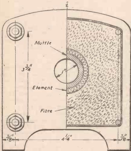
Fig. 1.—An end elevation in part section of a 200-watt electric furnace.
