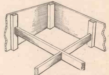
Fig. 3.—Alternative method of fixing the cross struts.
