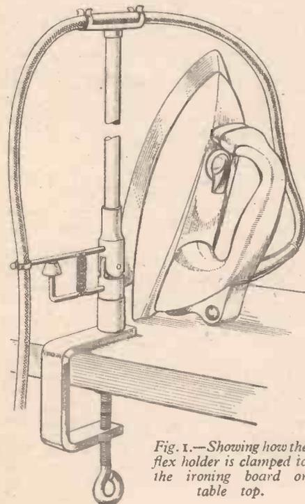
Fig. 1.—Showing how the flex holder is clamped to the ironing board or table top.
