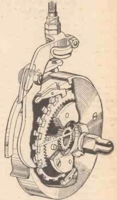
The Novo-Vaxel hub type two-speed gear.
