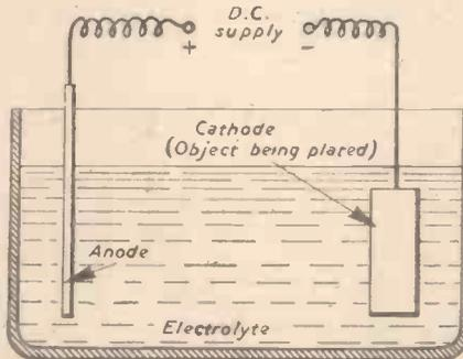
Fig. 3.—Diagram of connections to plating bath.
