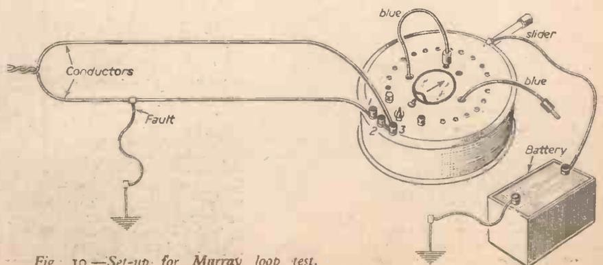
Fig. 10.—Set-up for Murray loop test.
