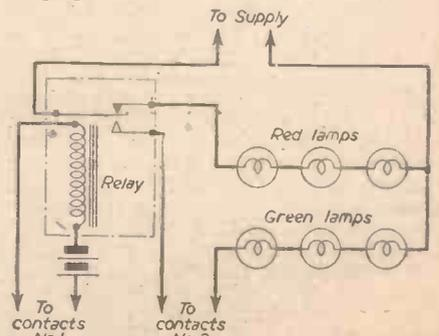
Fig. 4.—Change-over and flashing circuit.
