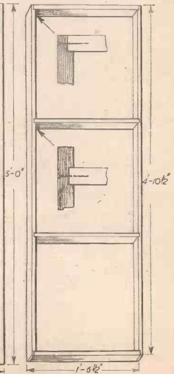
Fig. 3.—The frame to which the plywood top is attached.
