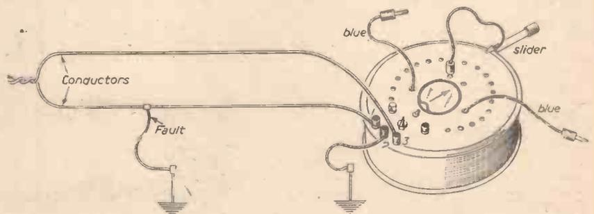
Fig. 9.—Set-up for loop test experiment.
