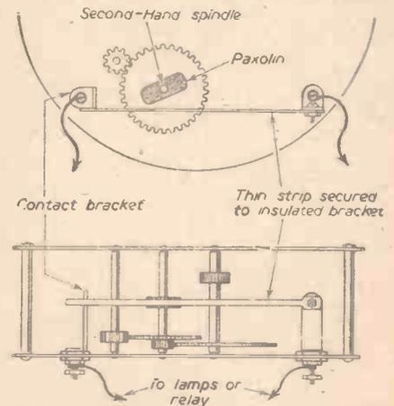
Fig. 3.—How the contacts are actuated.
