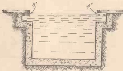
Fig. 4.—Using concrete slabs to cover the edges of the pool walls.
