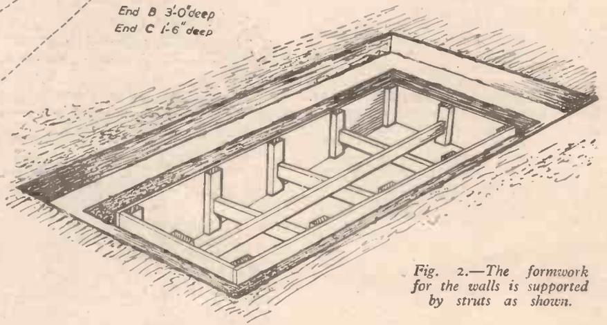
Fig. 2.—The formwork for the walls is supported by struts as shown.
