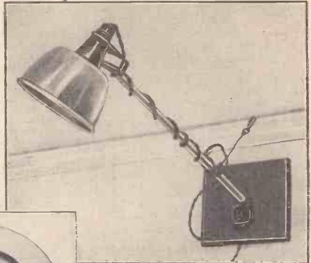
intensity, 2ft. from a 100-watt bulb, is 22ft. candles without the reflector and approximately 51ft. candles with it. This is an increase of 130 per cent., which enables lamps of lower wattage to be used and is therefore economical.
