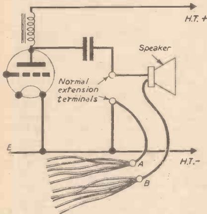
Fig. 1.—How to arrange the output circuit for radio games.
