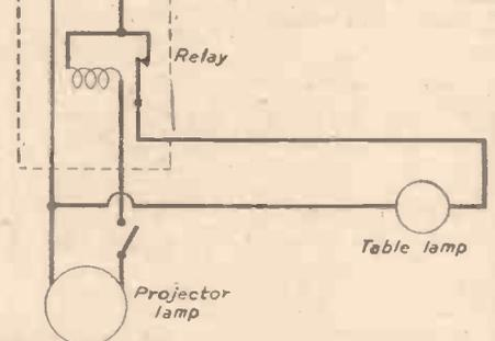
plugs into a wall switch plug, rather as a two-way adaptor does. It has two two-pin sockets—one for the projector and one for a table lamp. The current is switched on, lighting the table lamp, and when the projector is switched on (it has its own switch built in) then the table lamp goes out; when the projector is switched off, on comes the table lamp.
