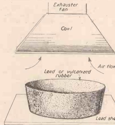
Fig. 2.—Simple equipment for etching. The fan can be replaced with a chimney stove pipe if the up-draught is sufficiently strong.
