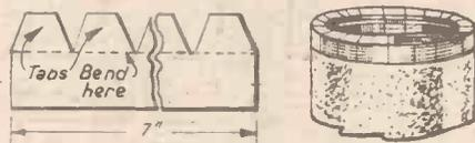
Fig. 3.—How the paper is cut to hold the disc in position. Fig. 4.—The flat ring of card placed on one end of the cylinder.
