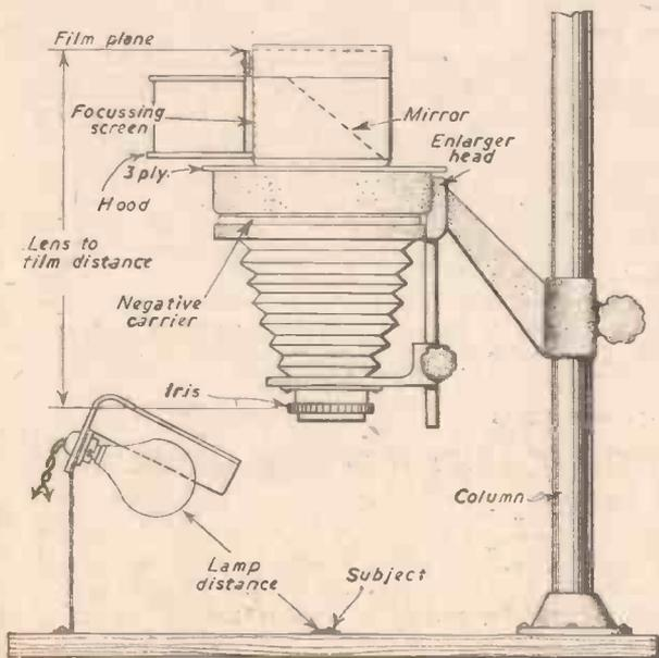
Fig. 1.—Set-up with reflex camera.
