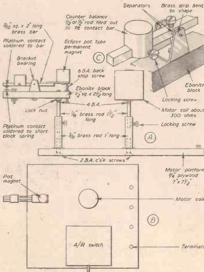
Fig. 5.—Motor platform, motor coil and magnetic switch.
