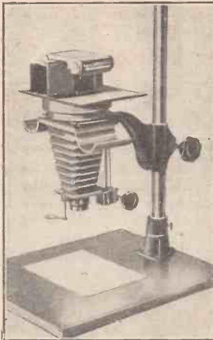
Fig. 3.—Enlarger with camera in place of lamp house.
