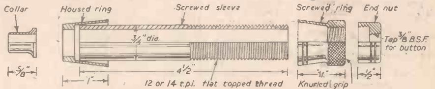
Fig. 2.—Handle and reel fittings (half full size). The material used is duralumin.
