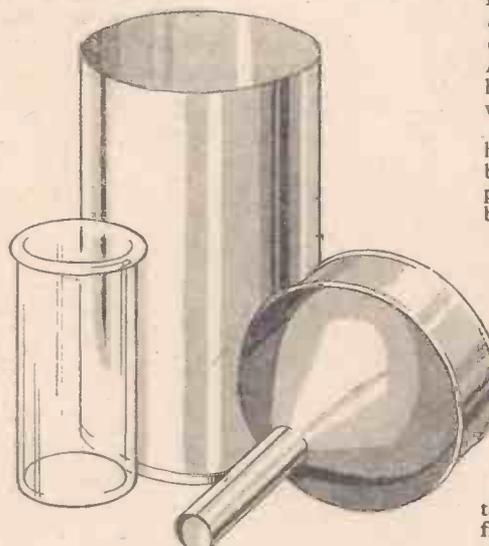
A perspective view of the rain-gauge components
