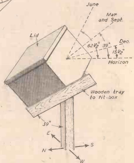
Fig. 4.—Mounting the recorder in a tray on a post, set at an angle of 39 deg. to the horizontal, and with the four corners approximately facing the compass points.
