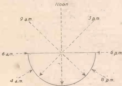
Fig. 1.—Showing the basic principle of the sunshine recorder—a half cylindrical pinhole camera. Note that a single cylinder will record somewhat less than 12 hours sunshine only.
