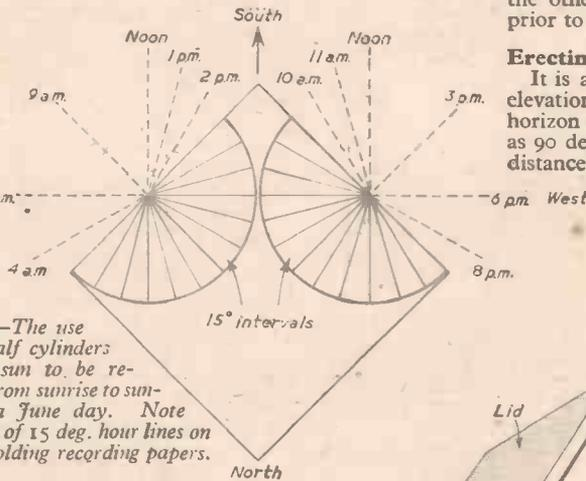
Fig. 2.—The use of two half cylinders enables sun to be recorded from sunrise to sunset on a June day. Note marking of 15 deg. hour lines on blocks holding recording papers.
