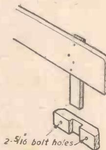
Fig. 3 (Above).—The back board and the method of fixing.
