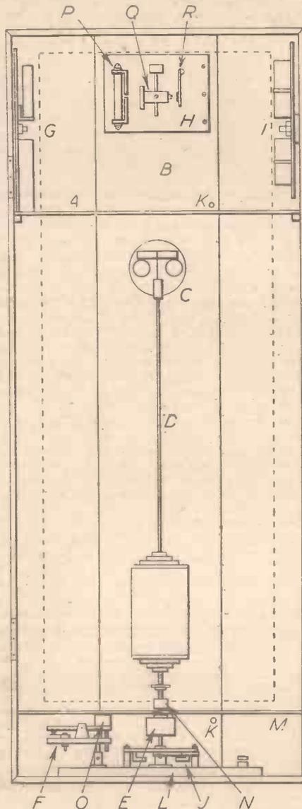
Fig. 1.—Lay-out and general principle. Key : A—Movement shelf; B—Backboard; C—Suspension; D—Pendulum; E—Motor Coil; F—Magnetic switch; G—Power unit; H—Escapement; I—Reserve batteries; J—Advance and retard switch arm in normal position; K—Hole in backboard through which 4 leads pass; L—Motor platform; M—Motor cover; N—Armature; O—Permanent magnet; P—Escapement coil; Q—Escapement armature; R—Escapement contact.
