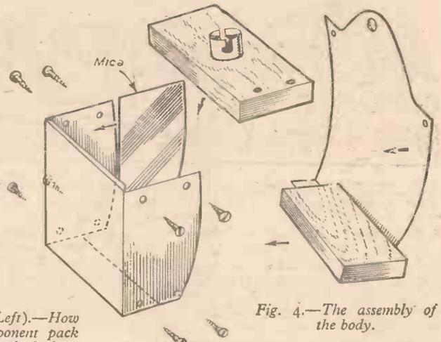
Fig. 4.—The assembly of the body.
