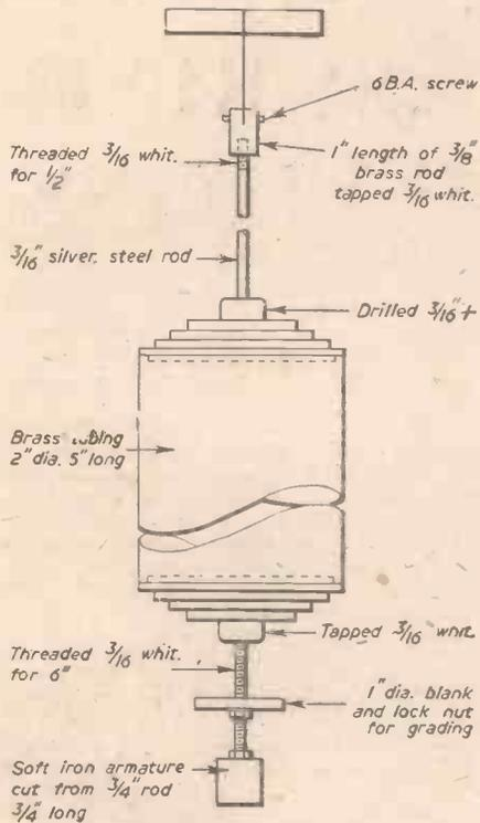
Fig. 4.—Pendulum details.
