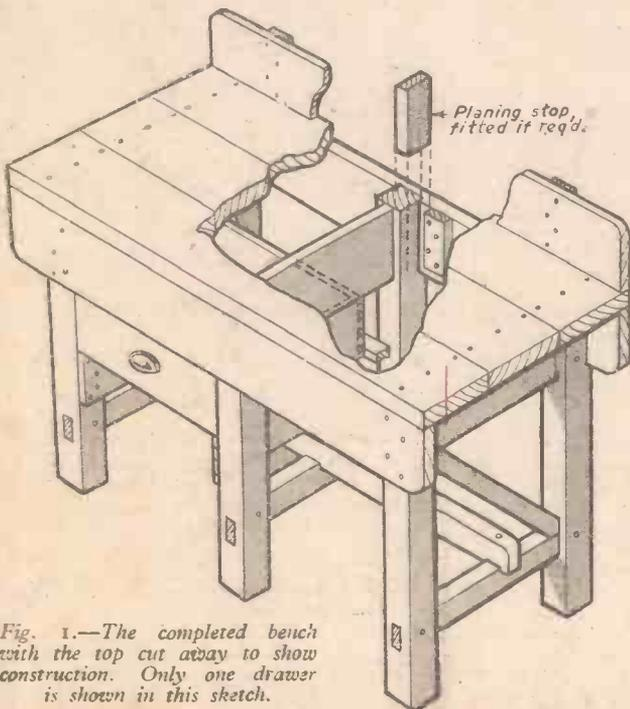
Fig. 1.—The completed bench with the top cut away to show construction. Only one drawer is shown in this sketch.
