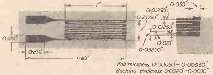
Fig. 3.—Foil strain gauge, the pattern of which is produced on a backing of Araldelyde lacquer.
