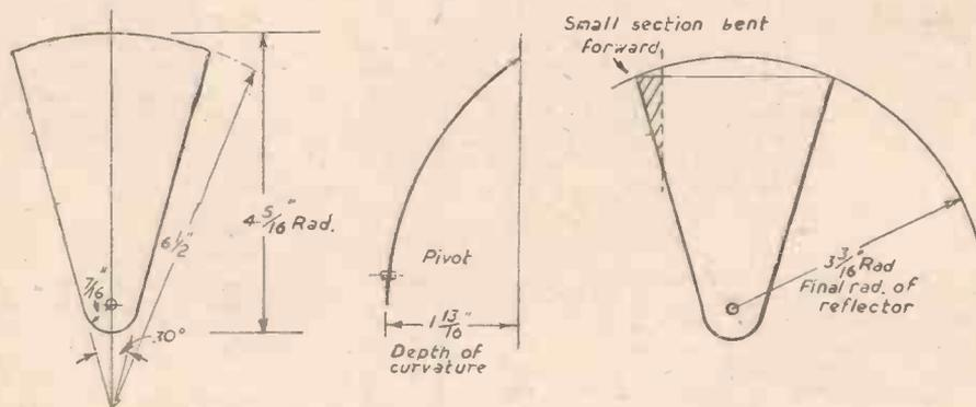
Fig. 2.—The development of the reflector segments.
