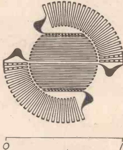
Fig. 4.—Four-gauge diaphragm developed in conjunction with the Admiralty Research Laboratory.
