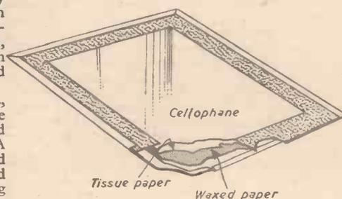
Fig. 3.—Assembling the writing tablet.
