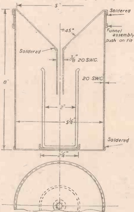
Constructional details of a rain-gauge.
