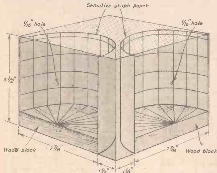
Fig. 3—Diagram showing the essential dimensions of the completed recorder. The 1/16in. hole may be replaced by a ½in. slot and either should be countersunk on each side.
