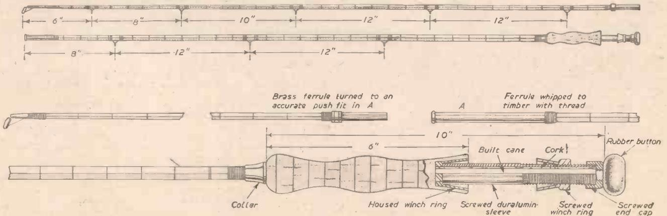
Fig. 1.—The completed rod, showing spacing of the rings, the joint ferrules and the handle construction.
