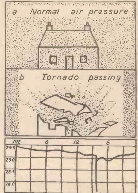
Fig. 11 (top).—The explosive effects. (Bottom) Typical barogram of a tornado.
