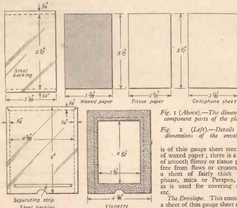
Fig. 1 (Above).—The dimensioned component parts of the platen.
