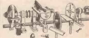
The most versatile tool ever offered to the public. Wood-turning lathe, rise and fall and fully tilting circular saw, hooded grindstone with drill sharpening attachment, sanding and drilling attachments, all accessories as illustrated. Complete £6.15.0 S.A.E. FOR LEAFLET
