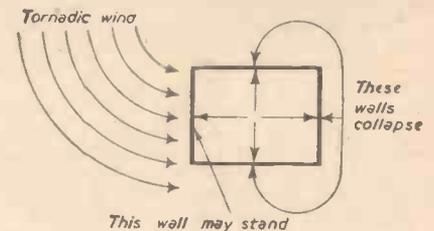
Fig. 12.—Outward collapse of walls.
