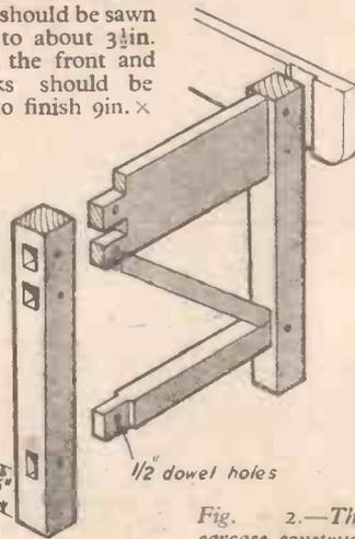
Fig. 2.—The carcass construction.
