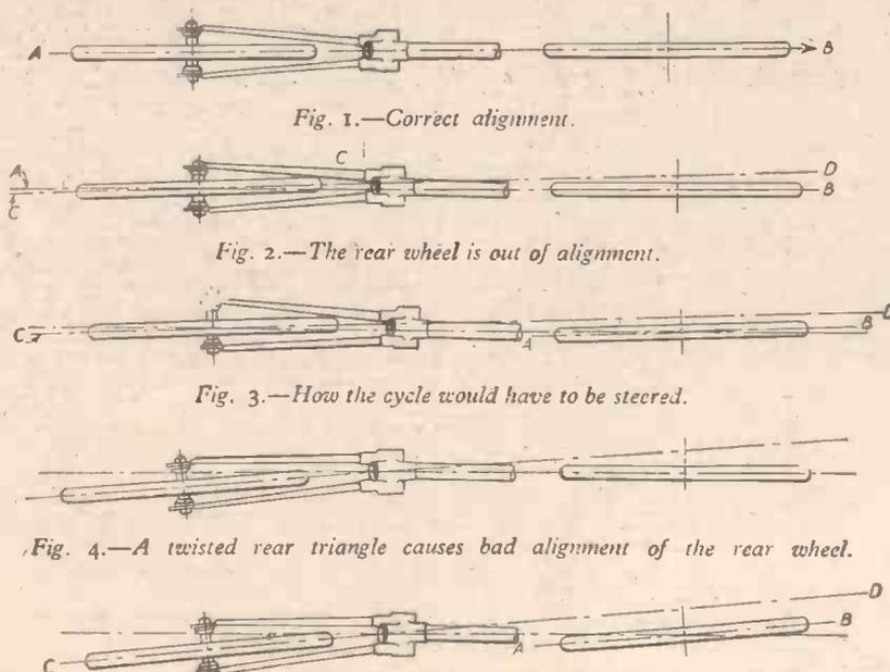
Fig. 1.—Correct alignment.
