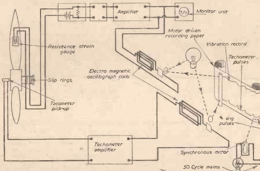
Fig. 1.—Layout of apparatus for recording alternating stresses from propeller blades.
