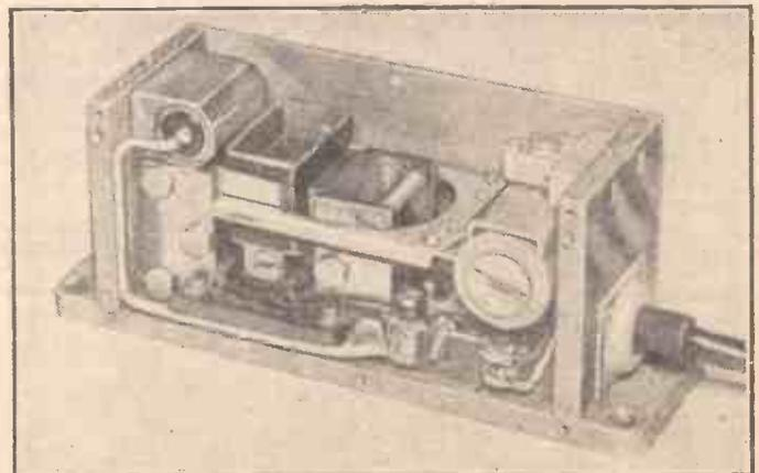
Fig. 2.—View of the de Havilland moving coil pick-up with cover removed. Note the compactness of this instrument.
