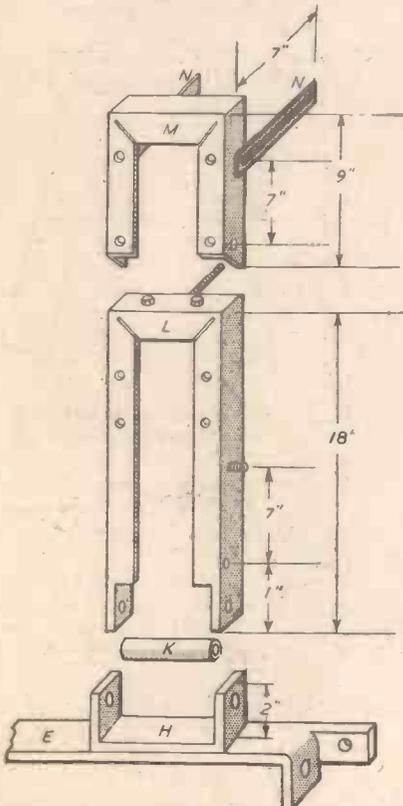
Fig. 5.—General assembly of motor and countershaft frames.
