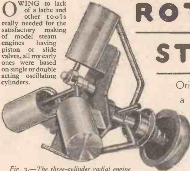
Fig. 3.—The three-cylinder radial engine.
