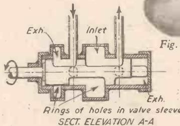
Rings of holes in valve sleeve
