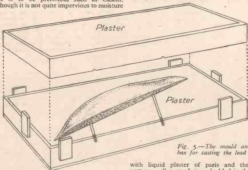
Fig. 5.—The mould and its box for casting the lead keel.
