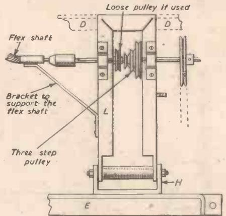
Fig. 9 (above).—The countershaft line-up
