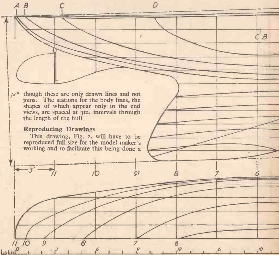
1/2" though these are only drawn lines and not joints. The stations for the body lines, the shapes of which appear only in the end views, are spaced at 3in. intervals through the length of the hull.
