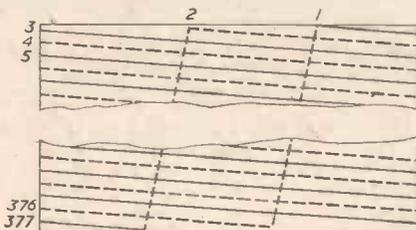
Fig. 2.—Method of interlacing; showing path of flying spot. Line fly-back lines are not shown.
