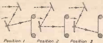
Fig. 5.—The mode of tilt to offset downward movement of film.
