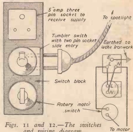
Figs. 11 and 12.—The switches and wiring diagram.
