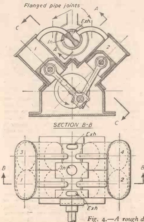
Fig. 4.—A rough design for a four-cylinder V engine.
