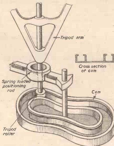
Fig. 7a.—The tripod roller in the kidney-shaped cam. The spring loading enables the centre pole of tripod to float around the hole in the main casting—its position being decided by the position of the roller in the cam.
