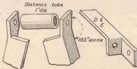
Fig. 2 (left).—Tops of legs and spacer.
