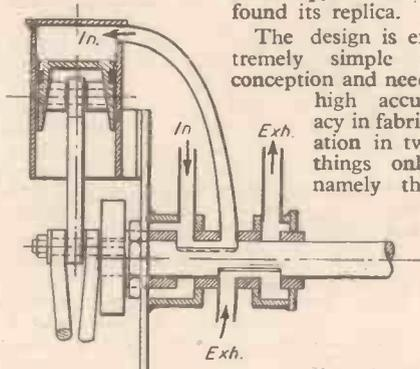
Fig. 1.—One cylinder of the three-cylinder radial engine.
