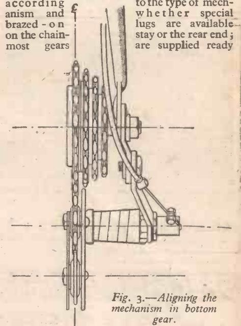
Fig. 3.—Aligning the mechanism in bottom gear.
