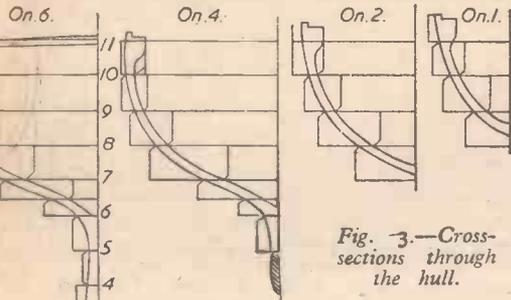
Fig. 3.—Cross-sections through the hull.
