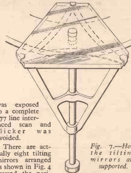
Fig. 7.—How the tilting mirrors are supported.
