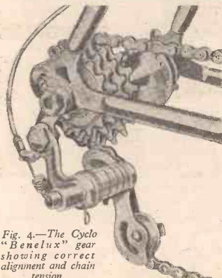
Fig. 4.—The Cyclo "Benelux" gear showing correct alignment and chain tension.
