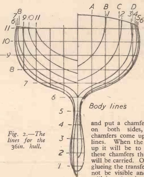
Fig. 2.—The lines for the 36 in. hull.
