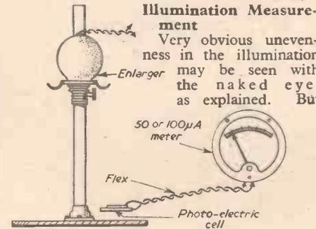
Fig. 5.—Measuring strength and evenness of illumination.
