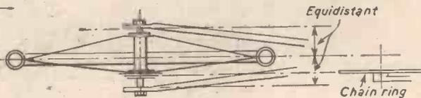
Fig. 2.—Correct chain alignment and the properly dished wheel.
