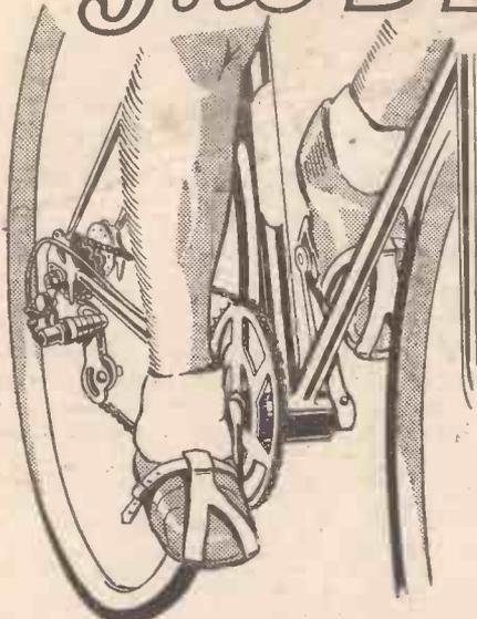
**D**UE to the infinite variety of ratios obtainable the derailleur gear is used almost universally by the cycling enthusiast, both in the fields of touring and racing; indeed, for the mass start rider it is an indispensable accessory.
