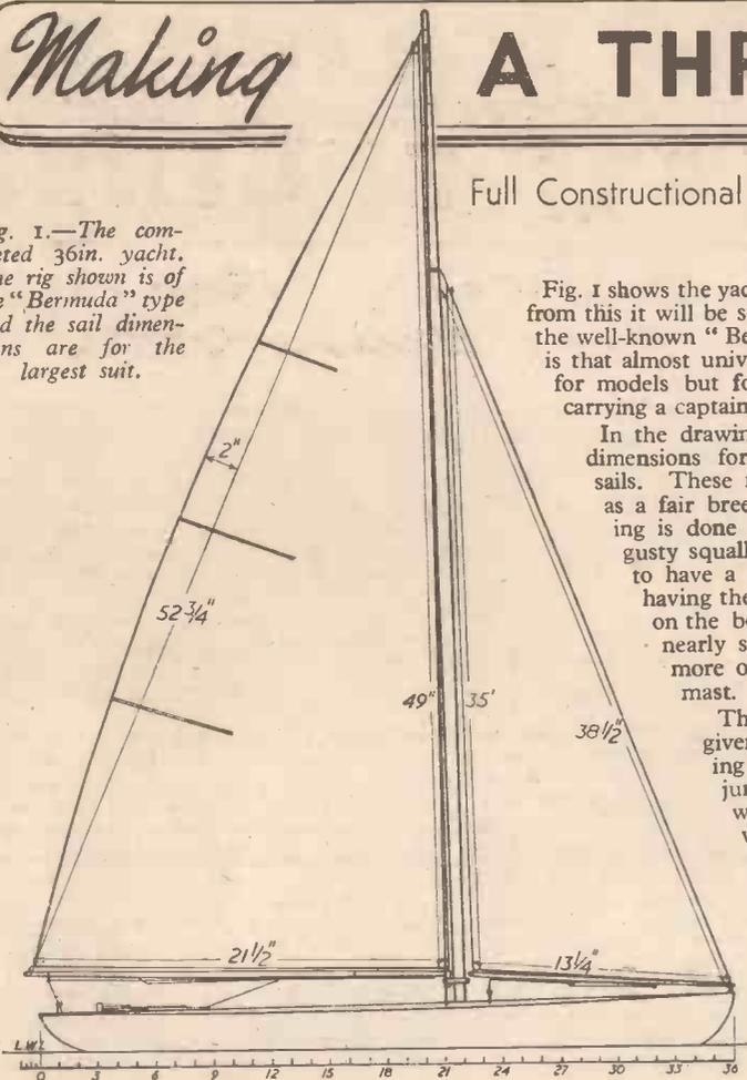
Fig. 1 shows the yacht in sheer elevation; from this it will be seen that the rig is of the well-known "Bermuda" type, which is that almost universally used not only for models but for quite large yachts carrying a captain and crew.
