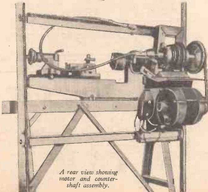
A rear view showing motor and countershaft assembly.
