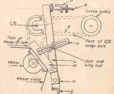
Fig. 6. — The motor and countershaft assembly.
