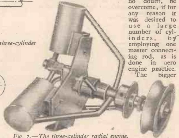
Fig. 2.—The three-cylinder radial engine.
