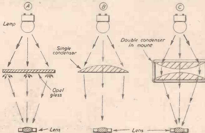
Fig. 2.—Diffused and condenser lighting.
