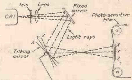
Fig. 3.—A simplified picture showing the arrangement of fixed and tilting mirrors in the Mechau camera.
