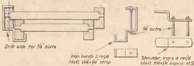
Fig. 6.—Details of the various irons required.
