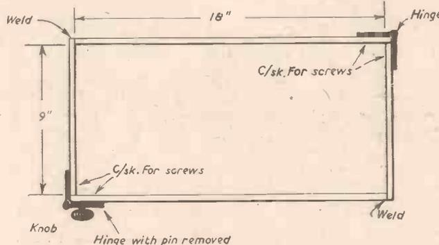
Fig. 1.—Constructional details of the casting frame.
