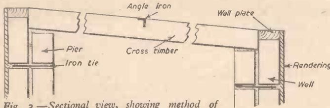
Fig. 3.—Sectional view, showing method of tying piers, and roof construction.
