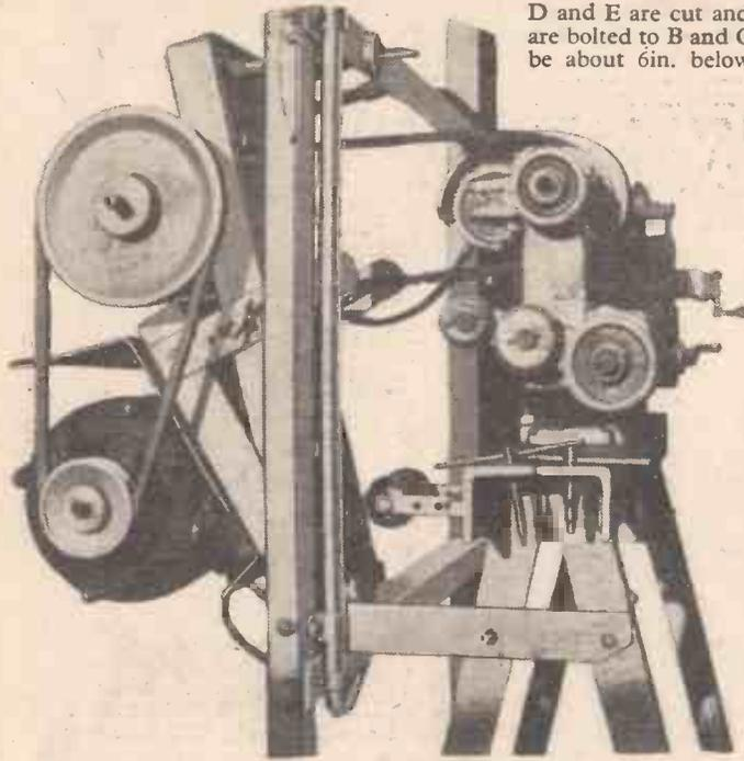
A view from the left of the lathe stand. Note shield round motor.
