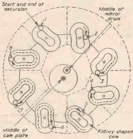
Fig. 8.—The position of the tripod roller at successive instants.
