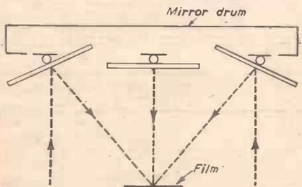
Fig. 6.—The mode of tilt to offset rotational movement of mirror drum.
