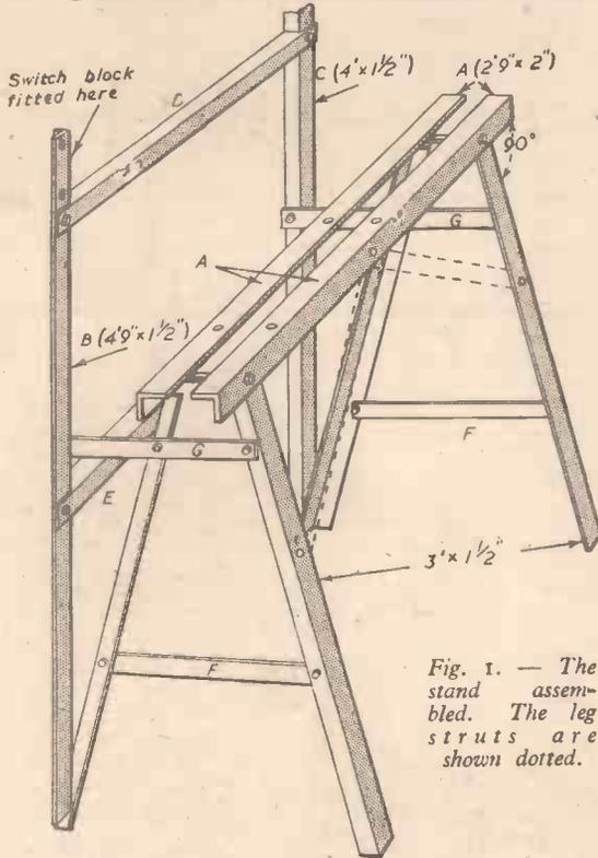
Fig. 1. — The stand assembled. The leg struts are shown dotted.
