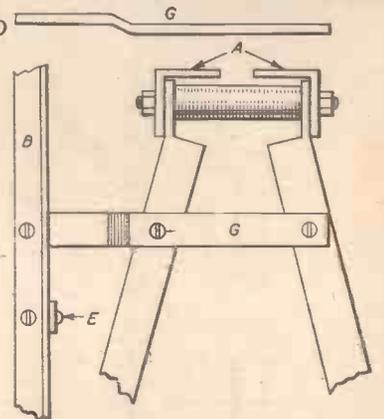
Fig. 3. — An end view of the lathe bed (A) and the supports (G).
