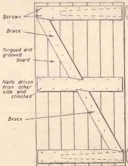
Fig. 4.—Constructional details of the doors.
