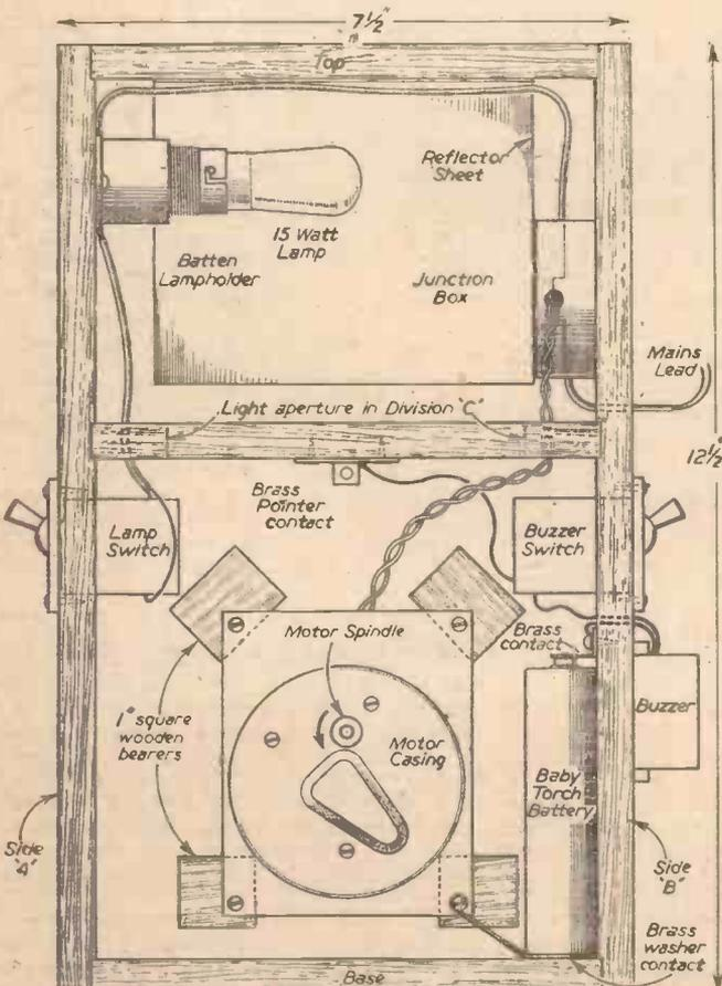
Fig. 1.—General arrangement of Safelight and Timer.
