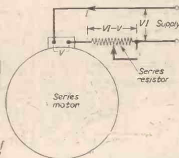
Fig. 6.—Use of a series resistor with a series motor.
