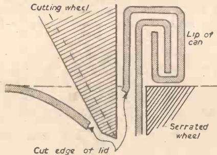
Fig. 6.—Enlarged detail from Fig. 5, showing how cut edge of lid is flattened against side of can.
