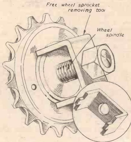
Fig. 1.—Freewheel removal tool (inset) and how it is used.
