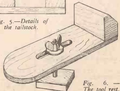
Fig. 6.—The tool rest.
