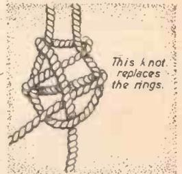
Fig. 7.—Double sheet bend.
