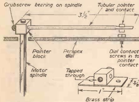
Fig. 6.—The pointer and pointer contacts.
