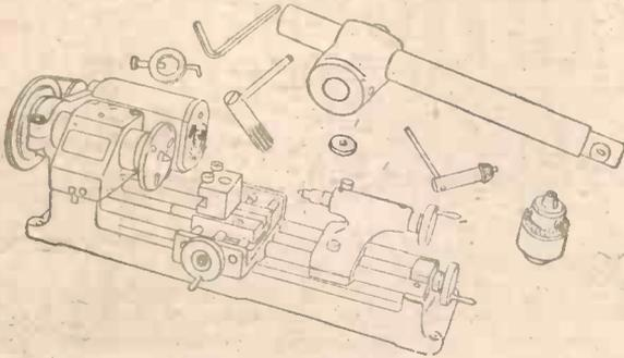
Only 16in. long, the Emco-Unimat is capable of several standard workshop practices to highly critical limits. The basic tool will buff, turn, polish, drill, grind and mill, and a full range of extra equipment vastly increases the scope of the tool.
