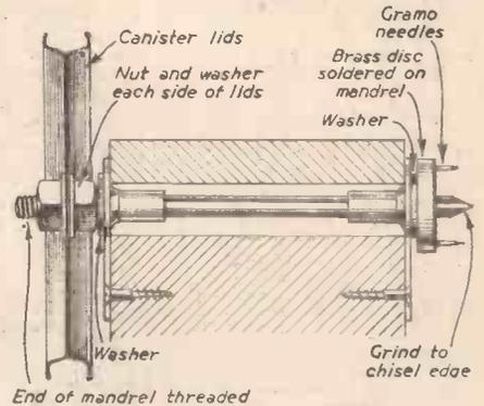
Fig. 4.—A sectional view of the headstock showing mandrel and chuck details.
