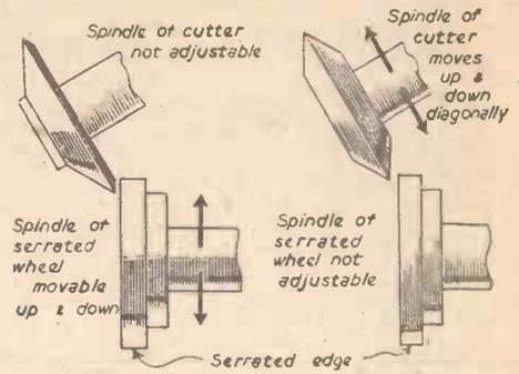
Fig. 7.—This arrangement probably gives a slight undercutting effect to neaten the cut edge of the lid.
