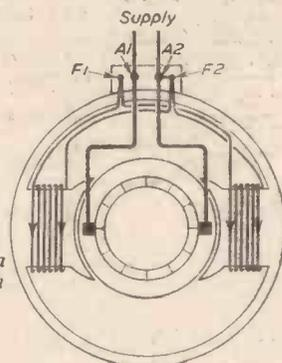
Fig. 7 (Above).—One method of using a shunt motor on half voltage or less.
