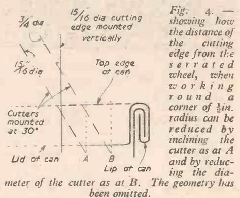
opener E (Fig. 1). A lever rotates the bush, through which the spindle of the serrated wheel passes eccentrically, and this lowers the serrated wheel, so that the lip of the tin can be put between the two wheels. Returning the lever raises the can into the cutting position, as seen in Fig. 6, forcing the cutting wheel through the lid of the
