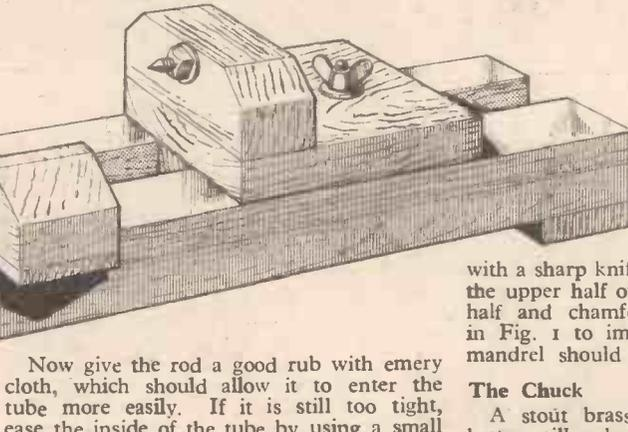
Fig. 3.—Upper half of headstock slotted.
