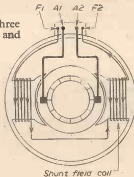
Fig. 2 (Left).—Connections of a shunt motor.
