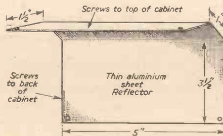
Fig. 8.—The aluminium reflector.
