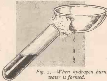
Fig. 2.—When hydrogen burns water is formed.
