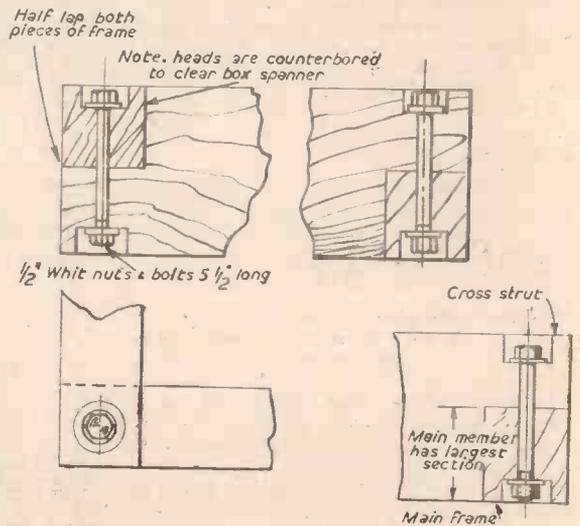
Fig. 2.—Method of jointing and bolting the frame.
