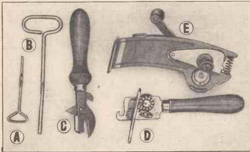
Fig. 1.—A selection of can openers. A—a sardine tin key. B—A larger and improved version. C—The traditional can opener. D—Serrated wheel type. E—An improved design.
