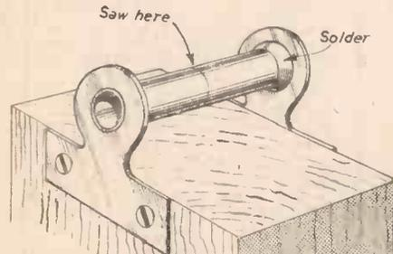
Fig. 2.—A perspective view of the headstock assembly clamped to a piece of wood.
