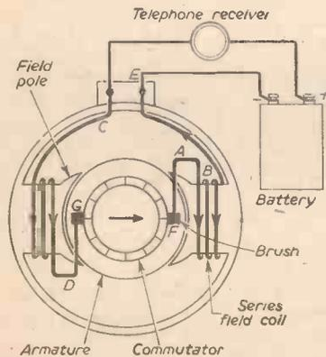
Fig. 1.—Connections of a series motor and method of test.
