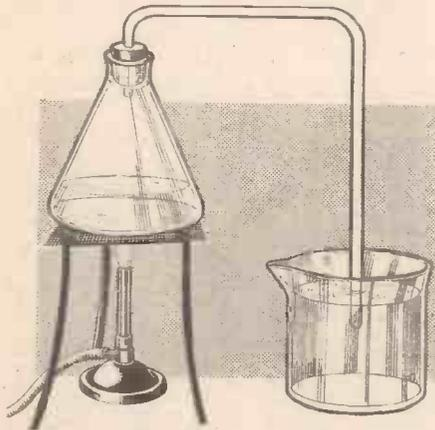
Fig. 1.—Apparatus for making hydrochloric acid.
