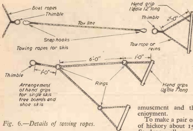
Fig. 6.—Details of towing ropes.
