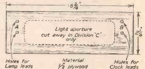
Fig. 4.—Shape and dimensions of top, bottom and division "C."
