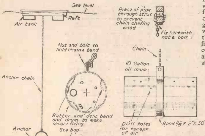
Fig. 3.—Details of the anchor.
