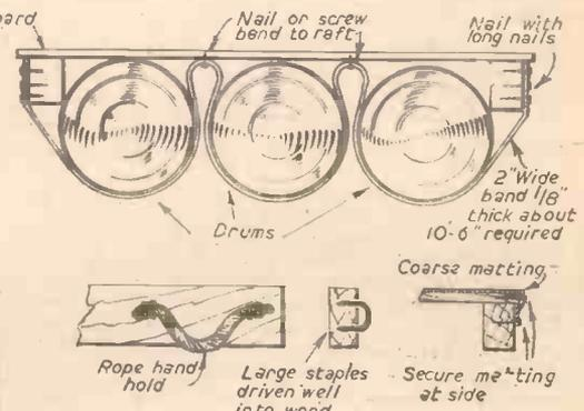
Fig. 5.—Fitting the drums, the rope handholds and the matting.
