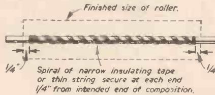
Fig. 2.—Preparing the metal core.
