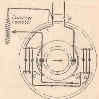
Fig. 3 (Left).—Connections of a compound motor.
