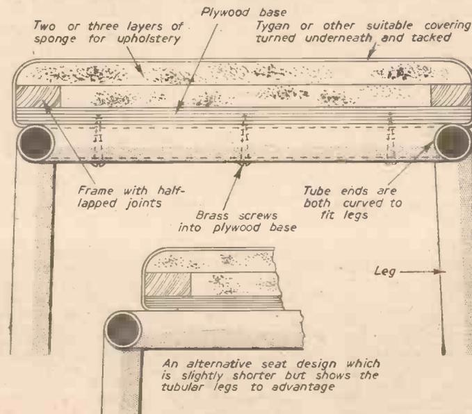
Fig. 5.—A cross-section through the seat illustrating the method used for attaching it to the frame.
