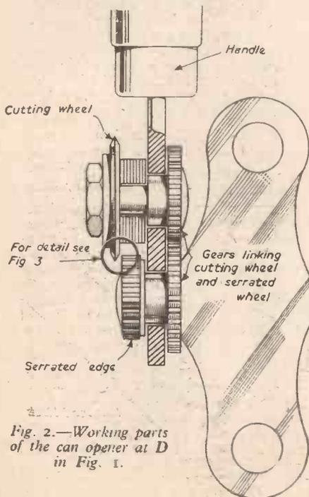
Fig. 2.—Working parts of the can opener at D in Fig. 1.
