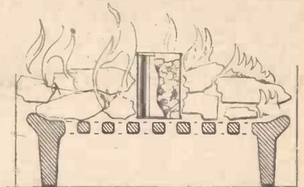
Fig. 9.—Tin of slack coal placed in fire to be coked and burnt.
