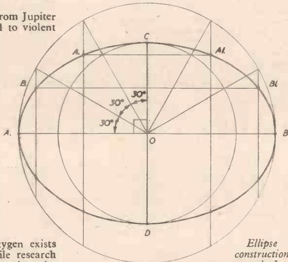
then, where parallels A-A<sub>1</sub>, B-B<sub>1</sub>, intersect perpendiculars, mark points.
