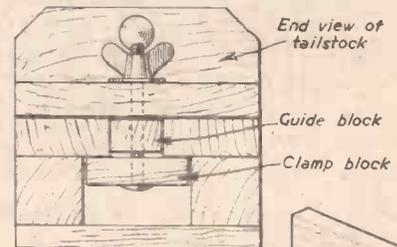
Fig. 5.—Details of the tailstock.
