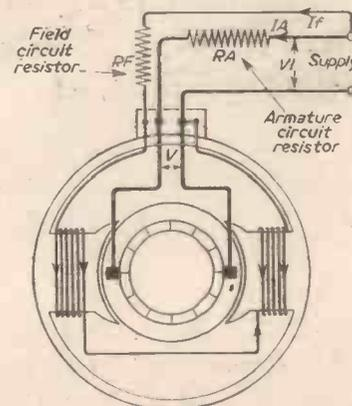
Fig. 8 (Right).—Method of using a shunt motor on increased voltage.
