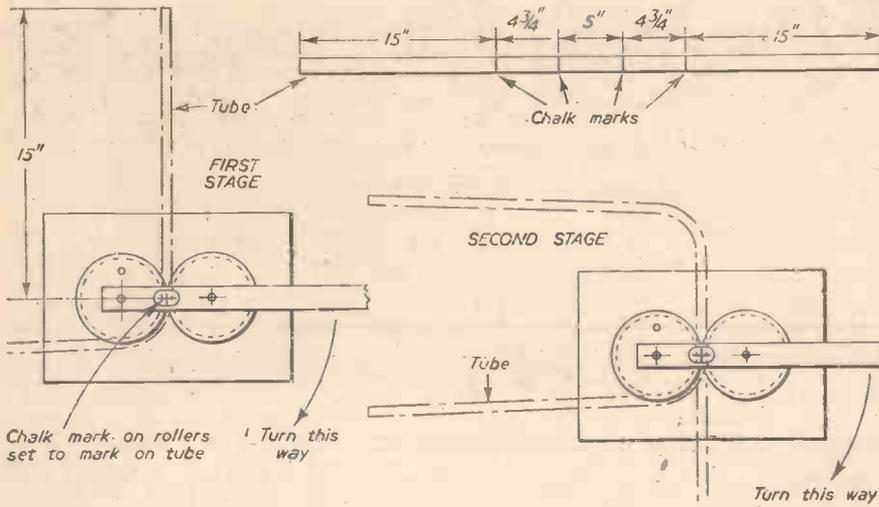
Fig. 4.—Brief sketches showing the tube in position ready for bending.
