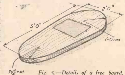
Fig. 5.—Details of a free board.
