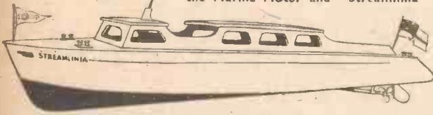
The "Streamlinia" Motor Boat Hull is carved from seasoned timber and finished painted ready for final finishing coat. It will carry plant up to 61 lbs., is designed for speed and is suitable for steam, electric or i.c. drive. Excellent for radio control. Length 3ft. 3in., beam 8in., price £9.14.0.
