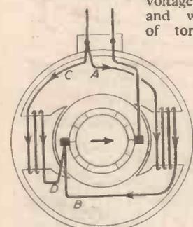
Fig. 5.—Reconnection of series field coils in parallel.
