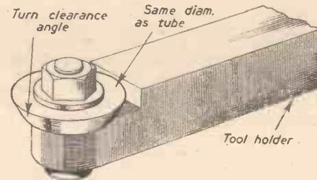
Fig. 3.—A tool holder which a lathe user can make for turning profiles similar to that needed for the machining of these grooves in the rolls.
