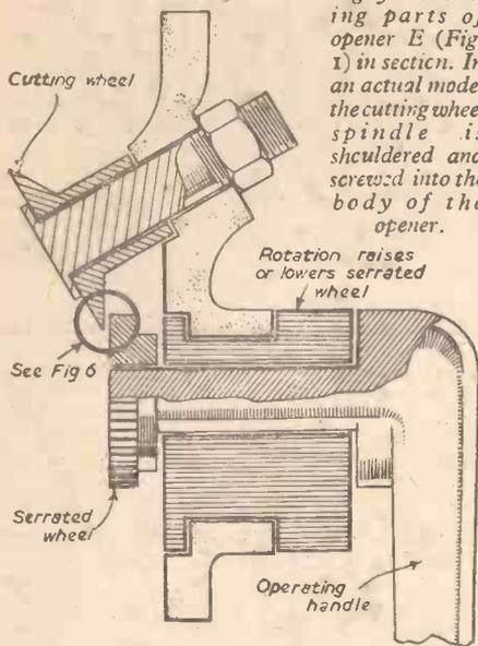
Fig. 5.—Working parts of opener E (Fig. 1) in section. In an actual model the cutting wheel spindle is shouldered and screwed into the body of the opener.
