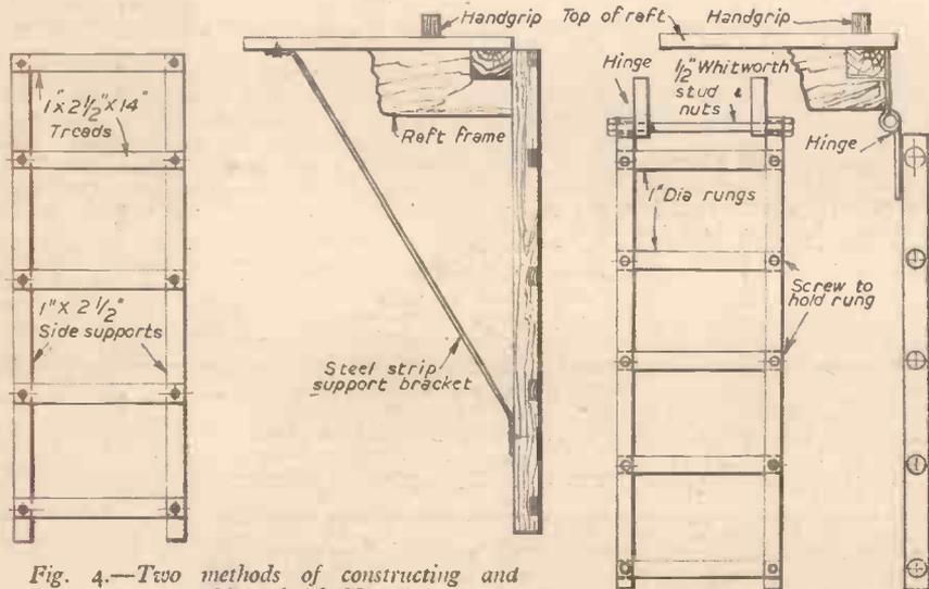
Fig. 4.—Two methods of constructing and attaching the ladder.
