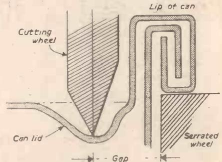
Fig. 3.—Enlargement of detail inside circle in Fig. 2. The gap between cutting wheel and serrated wheel is so wide that the can lid bends instead of shearing.
