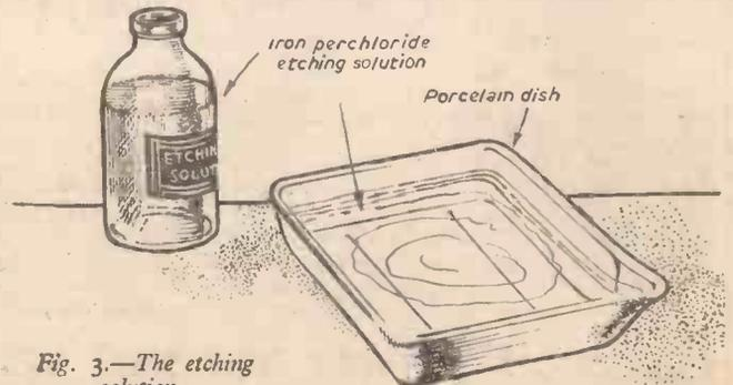
Fig. 3.—The etching solution.
