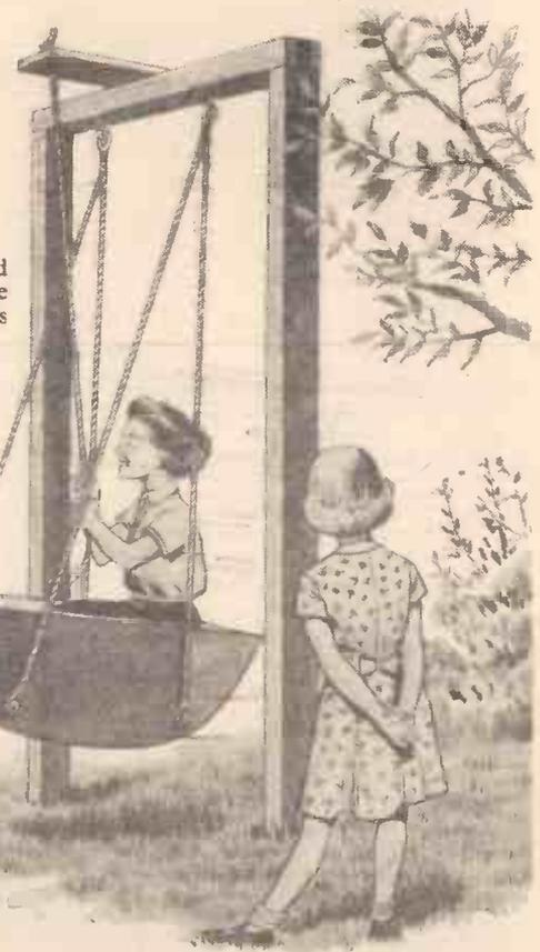
through a hole in the crossbar, and secured tightly with a washer and nut so that the rope could not jump off, as shown in Fig. 4.
