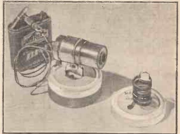
Fig. 30.—Heat ray detector complete (less screen).
