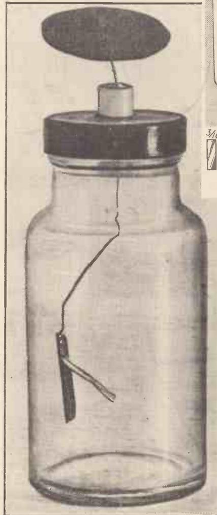
Fig. 3.—A type "A" electroscope
