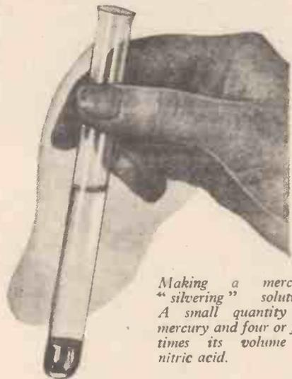
Making a mercury "silvering" solution. A small quantity of mercury and four or five times its volume of nitric acid.
