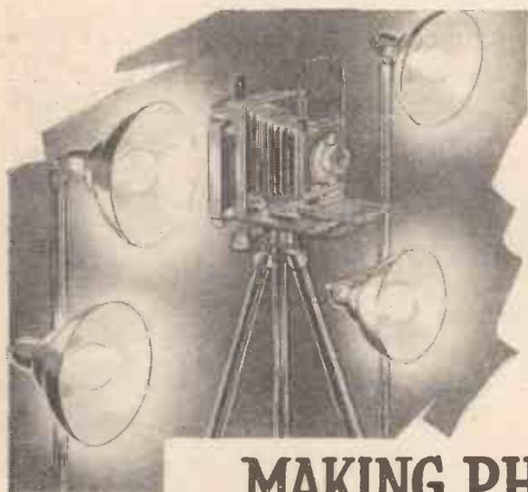
run the bulbs at a greatly reduced consumption (and intensity) till the last moment before pressing the trigger, when they are taken up to full consumption and intensity.
