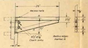
Fig. 3.—Details of the arm-piece.
