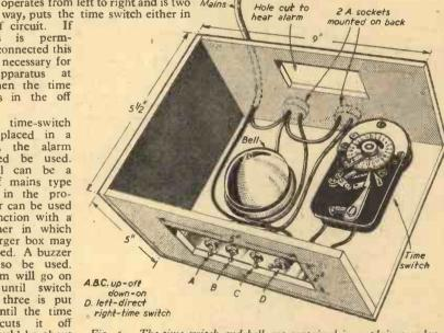
Fig. 1 .- The time switch and bell are contained in a plain wooden box with a lid (not shown).
