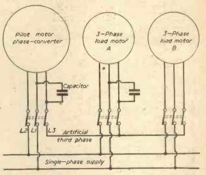
Fig. 4.—Use of phase-converter for feeding three-phase motors from single-phase mains.
