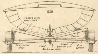
Fig. 10.—The loaded traiter.
