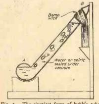
Fig. 1 .- The simplest form of bubble tube.
