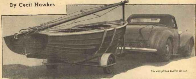
HIS boat trailer was designed specifi-THIS boat trailer was designed specifically to transport a National 12ft. sailing dinghy, but with suitable modifications to the hull supports it would be capable of carrying light craft up to 14ft. over-all length. In practice the trailer has proved to have very good road holding qualities and the boat rides quite steadily behind the towing vehicle. behind the towing vehicle.
