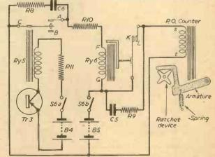
Fig. 37.—Circuit of the electronic transistor counter.
