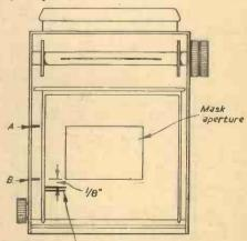
Position of mark on backing paper Fig. 3.—Back of camera.
