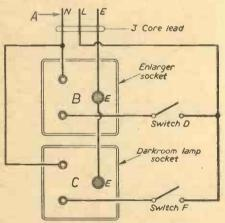
Fig. 2.—Distribution panel wiring.
