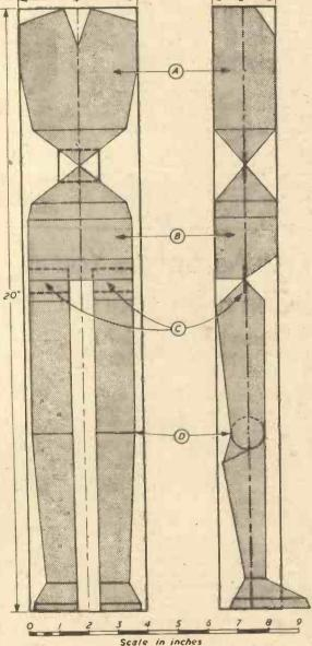
Fig. 2.—Details of the body and legs.
