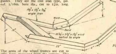
Fig. 6.—Angle iron to the above dimensions is employed to make the swinging arm frames. pivoted wheel carriers and the cradle which
