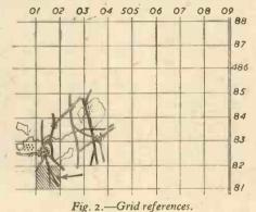
each direction) and another figure added to each part of the reference for the larger square. The point indicated would therefore be 019815. Finally, the 100 kilometre square of which the I kilometre squares are part must be indicated by its letter reference and the full map reference would be TA019815.
