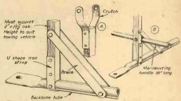
Fig. 13.—Details of the mast support, crutch and manœuvring handle.
