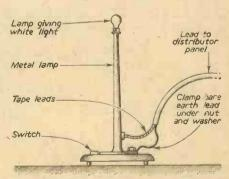
Fig. 5.—Electrical precautions in the improvised darkroom.
