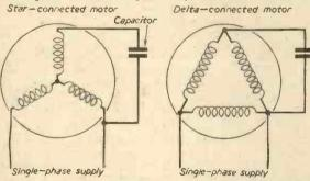
Fig. 3.—Capacitor methods of starting three-phase motors on a single-phase supply.
