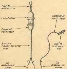
Fig. 3.—Connecting the distribution panel in the bathroom.
