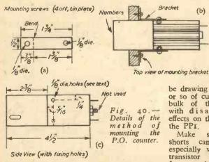
The tin-plate must not be wide enough to short on to the terminals.
