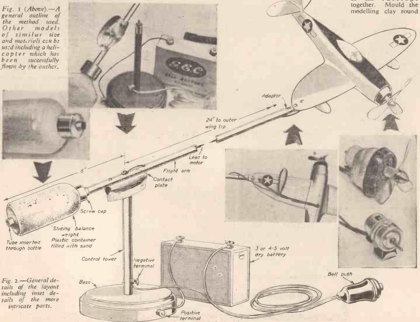
Fig. 2.—General details of the layout including inset details of the more intricate parts.
