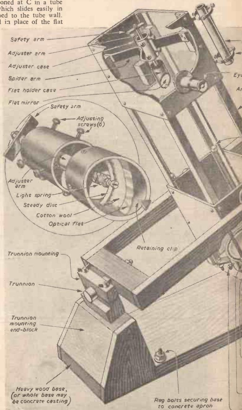
Fig. 3.—Layout of one construction for the telescope in a cradle mounting. Readers as the angle between cradle and base must
