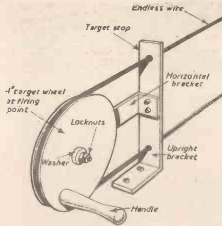
Fig. 10.—The target mechanism at firing point.
