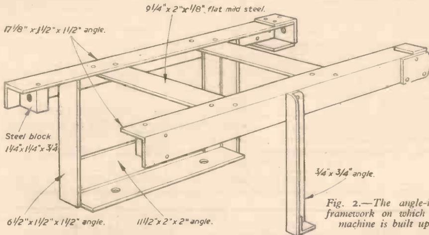
Fig. 2.—The angle-iron framework on which the machine is built up.
