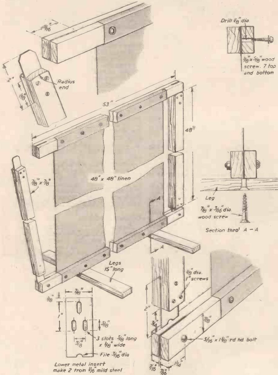
Fig. 1.—Full details and dimensions for construction.
