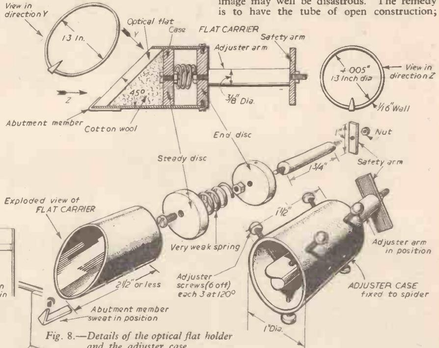
Fig. 8.—Details of the optical flat holder and the adjuster case.
