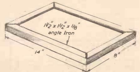
Fig. 3.—1 1/2 in. x 1 1/2 in. x 1/8 in. angle iron frame.
