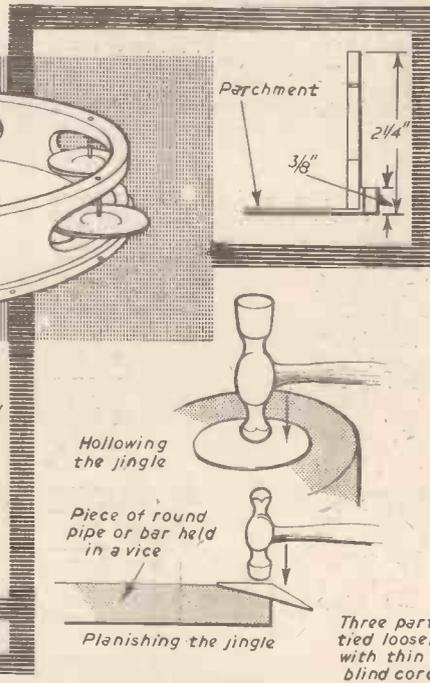
for each instrument, are hollowed out from some thin brass sheet of about 20 gauge thickness. If required, these may be made of thin tin plate sheet instead.
