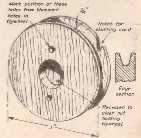
Fig. 5.—Details of the starting pulley.
