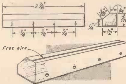
Fig. 5.—Details of the bridge.
