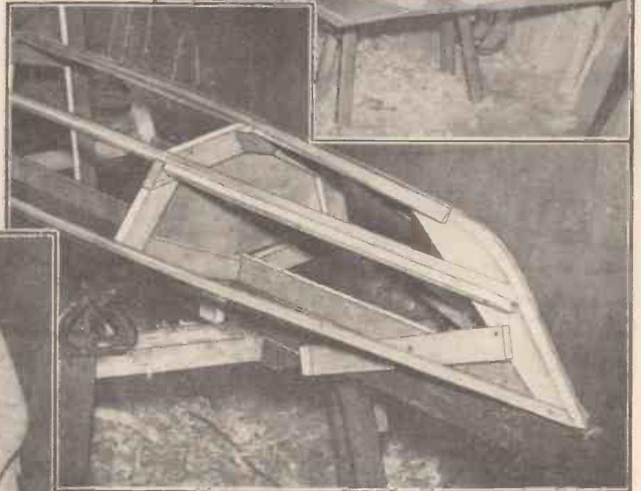
Before fixing the three remaining panels it is as well to fair off the edge of this first panel at the chine stringer so that the builder is better prepared for the task on the other three. From Fig. 20, it will be observed that the plywood has to be filed away to a very oblique angle towards the bow. Many of the nails will be found to be in the way. They must be punched down because they would catch in the teeth of the file and be dragged sideways in the plywood. When doing this
