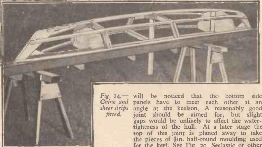
Fig. 14.—Chine and sheer strips fitted.
