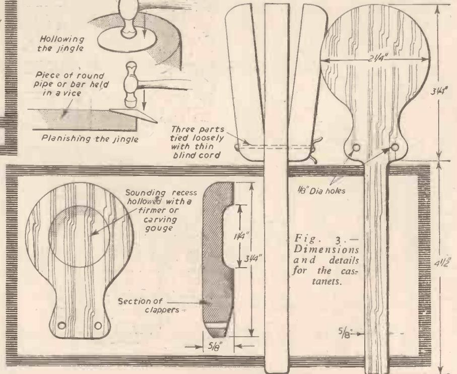
Fig. 3.—Dimensions and details for the castanets.
