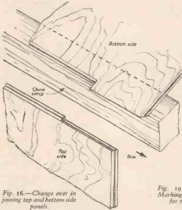
Fig. 16.—Change over in joining top and bottom side panels.
