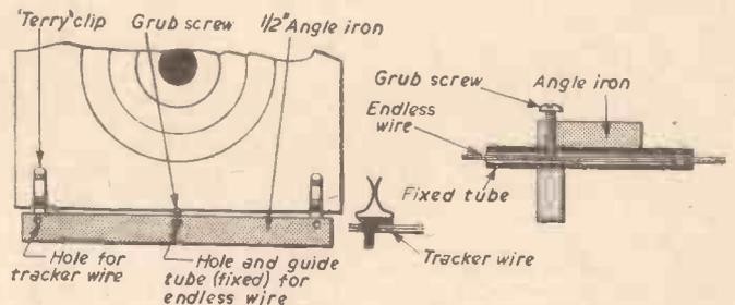
Fig. 8.—Front and side views of the target holder.
