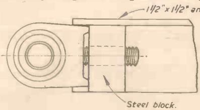
Fig. 3.—Fitting of plummer blocks at fixed (pulley) end.
