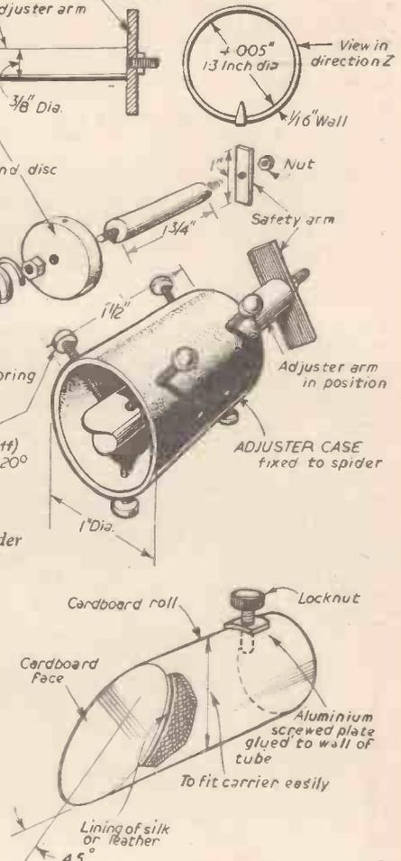
Fig. 9.—Details of cap for optical flat.
