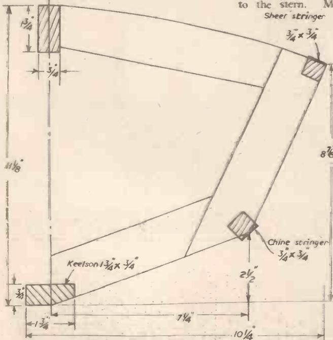
Fig. 8.—Half plan of fore and aft frames.
