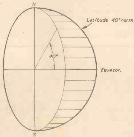
Fig. 2.—The lines of latitude are named after the angle they make at the centre of the earth.
