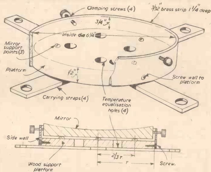
Fig. 5.—Perspective view of mirror cell and sectional view with mirror in position.
