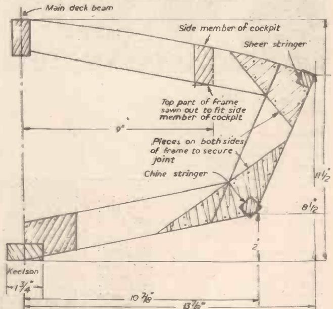
Fig. 9.—Dimensions of the centre frame.
