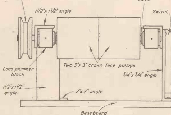
Fig. 5.—Pulley-end view of machine without table top.
