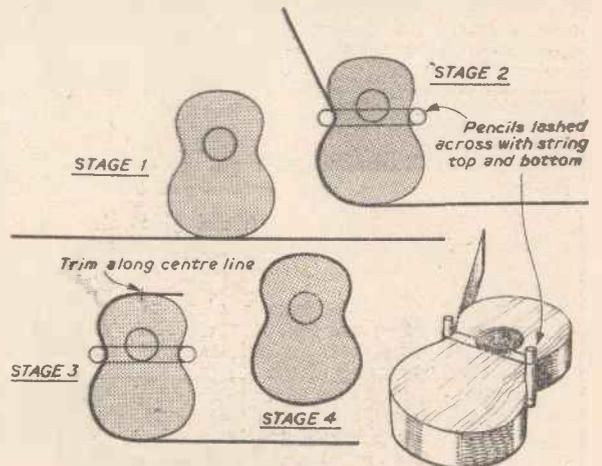
Fig. 2.—Four stages in fitting the sides.
