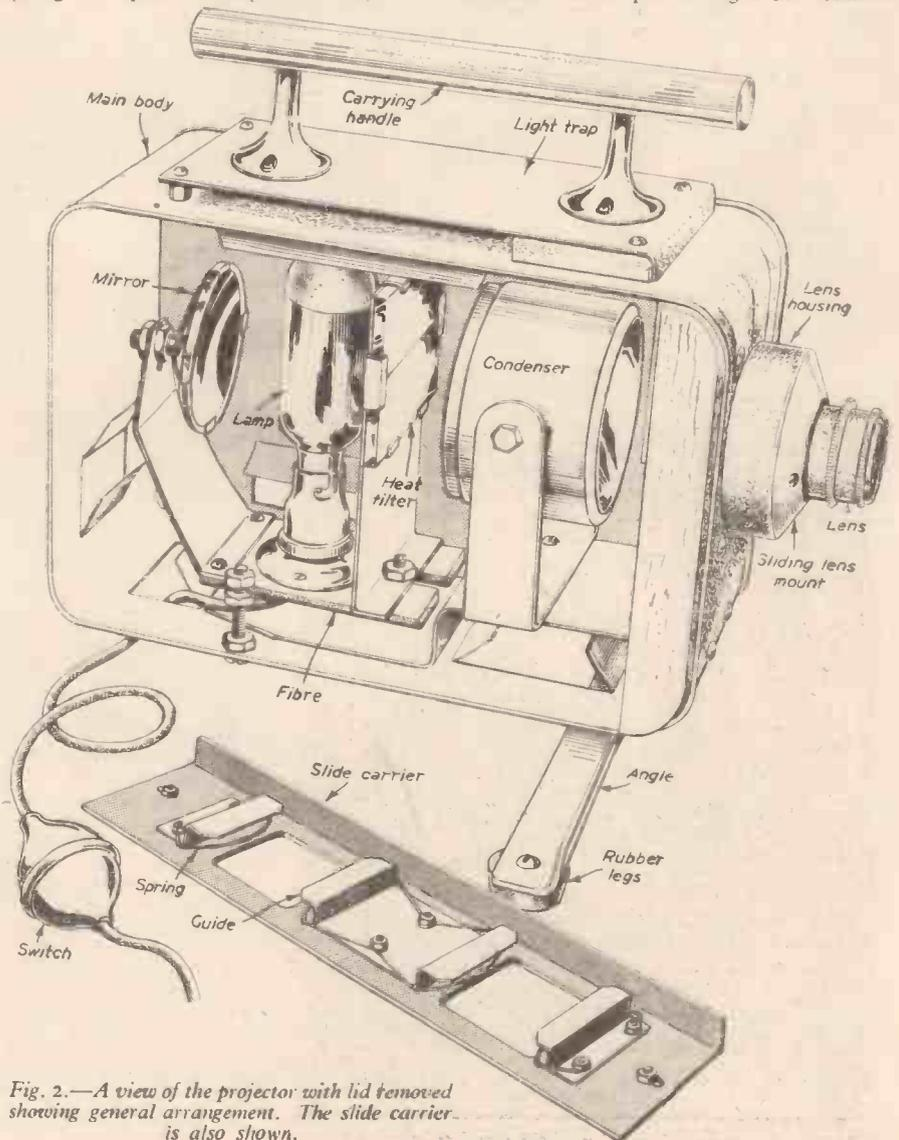
Fig. 2.—A view of the projector with lid removed showing general arrangement. The slide carrier is also shown.
