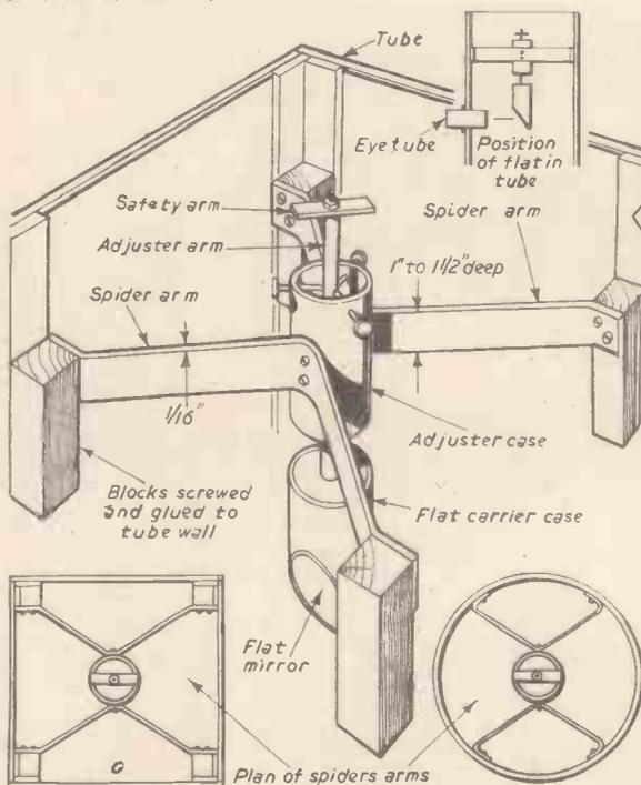
Fig. 7.—Holding and adjusting the optical flat holder.
