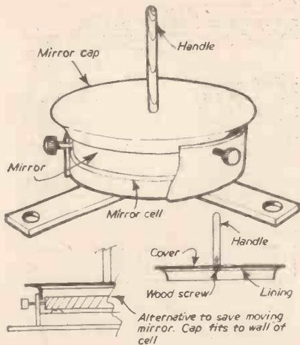
Fig. 6.—Details of the mirror cap.
