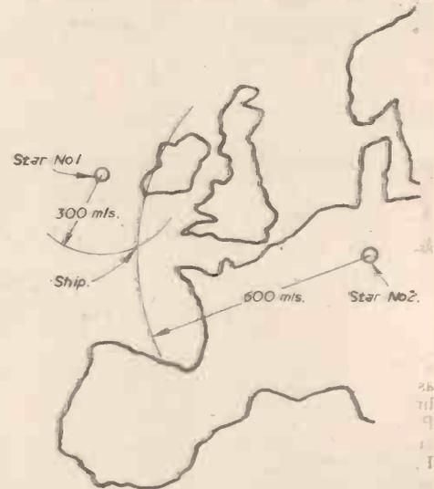
Fig. 7.—When taking his position from two stars, the navigator's position is where the circles cut.
