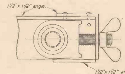
Fig. 4.—Fitting plummer blocks at adjustable end.
