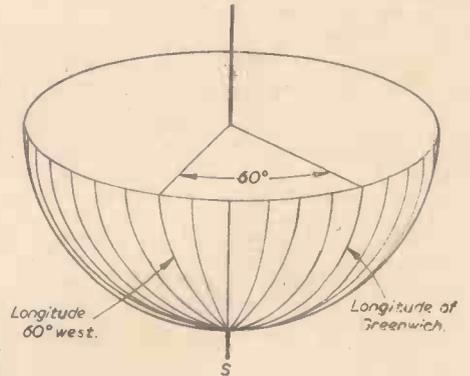
Fig. 3.—The lines of longitude are divided into degrees, the line that runs through Greenwich is taken as longitude 0.
