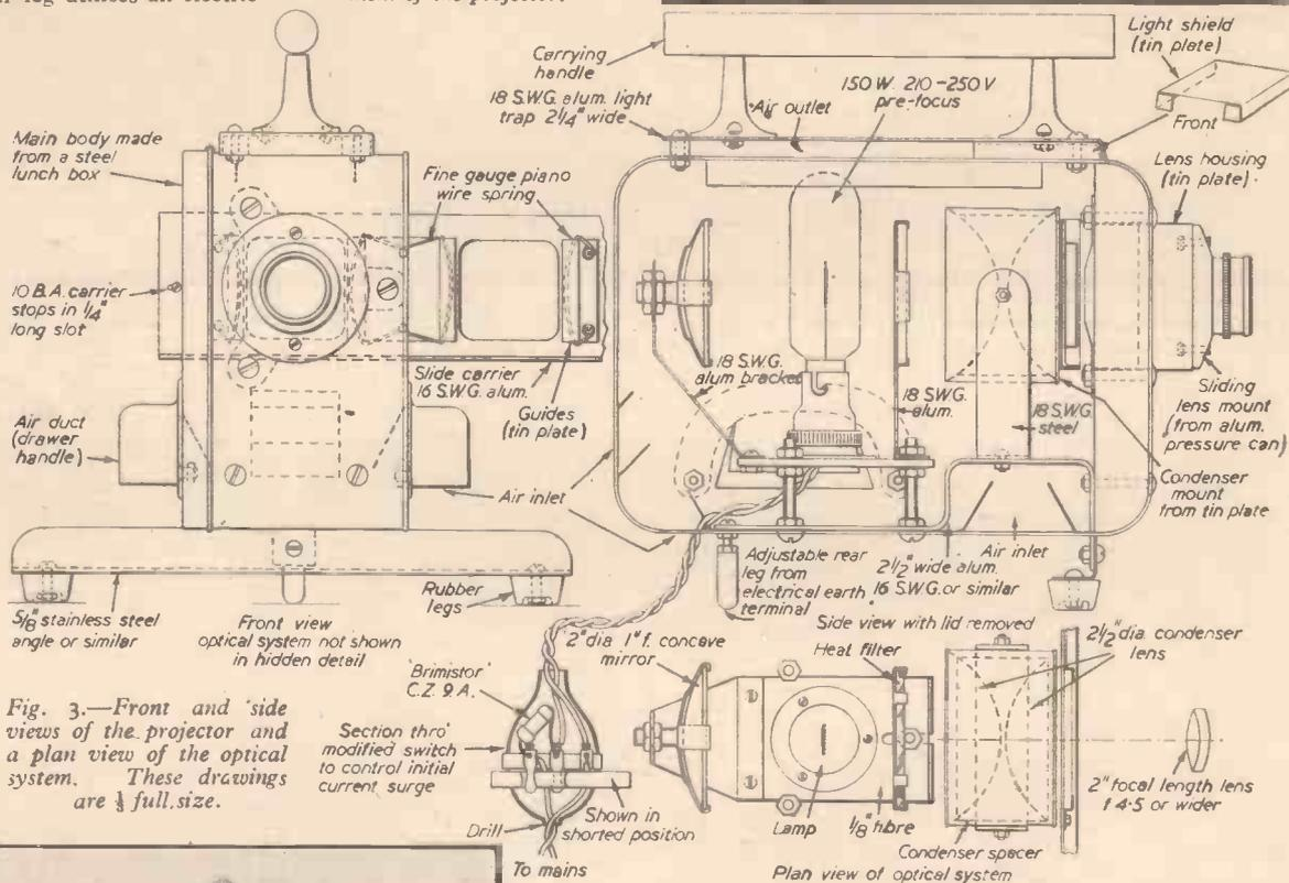
Fig. 3.—Front and side views of the projector and a plan view of the optical system. These drawings are ½ full size.
