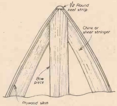
Fig. 15.—Showing how the chine and sheer strips meet the chamfer on the bow piece.
