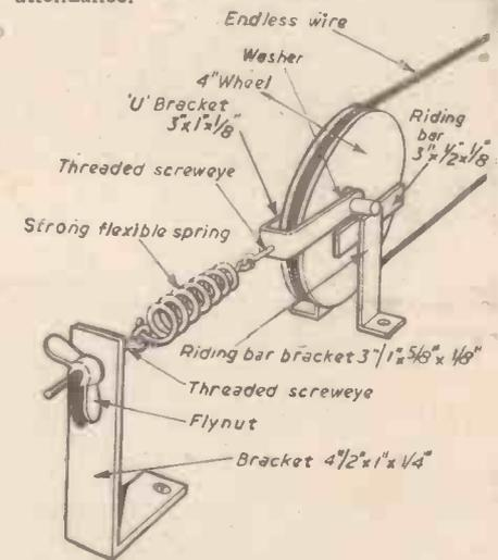
Fig. 11.—Details of target mechanism at far end of the range.
