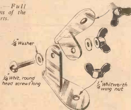
Fig. 3.—General arrangement details.
