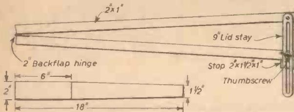
Fig. 1.—Taper jig details.
