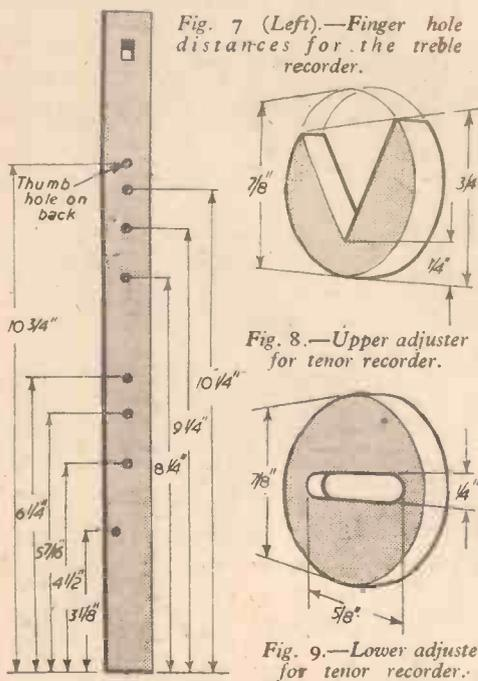
Fig. 7 (Left).—Finger hole distances for the treble recorder.
