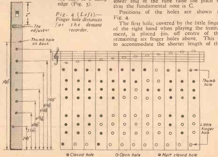
Fig. 4 (Left).—Finger hole distances for the descant recorder.
