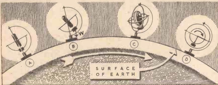
Fig. 6.—The gyroscope is made north seeking.
