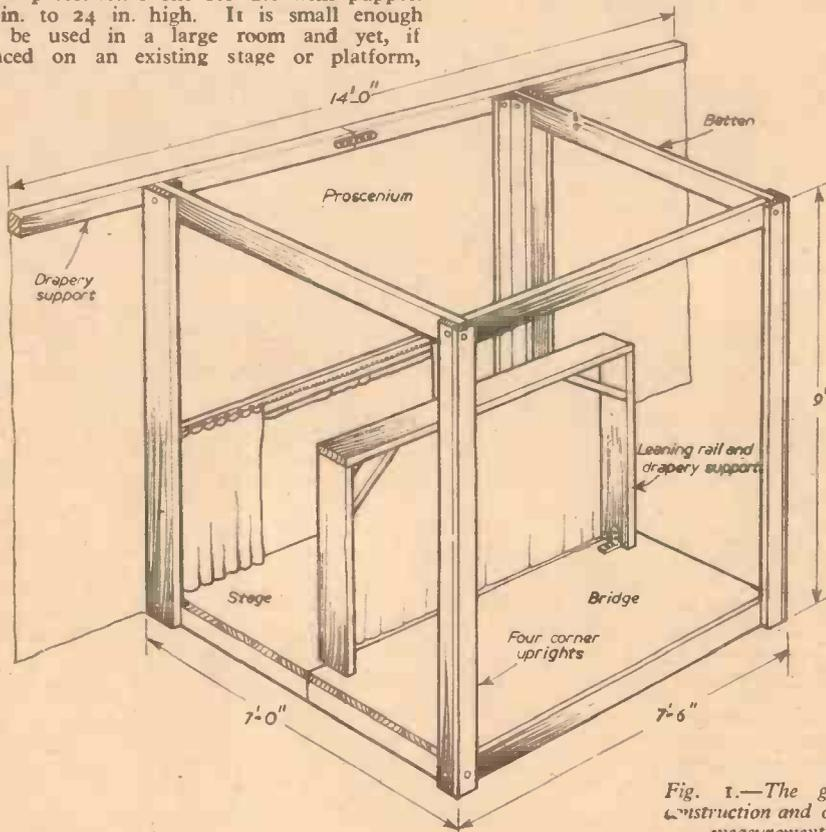
Fig. 1.—The general construction and overall measurements.
