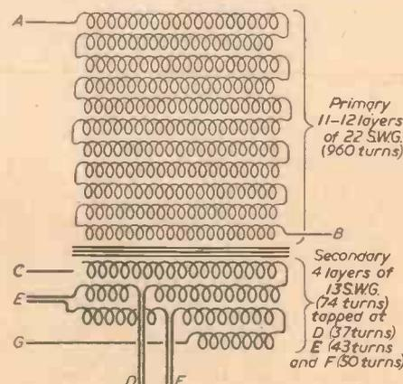
Fig. 4.—Details of transformer winding.
