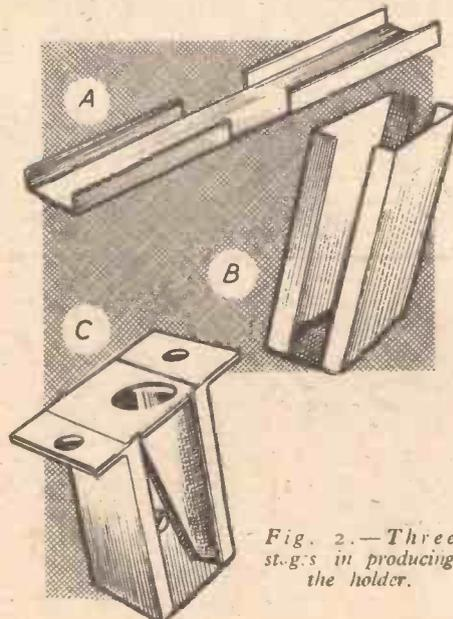
Fig. 2.—Three stages in producing the holder.
