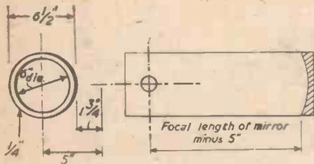
Fig. 15.—Position of eye tube for round tube.
