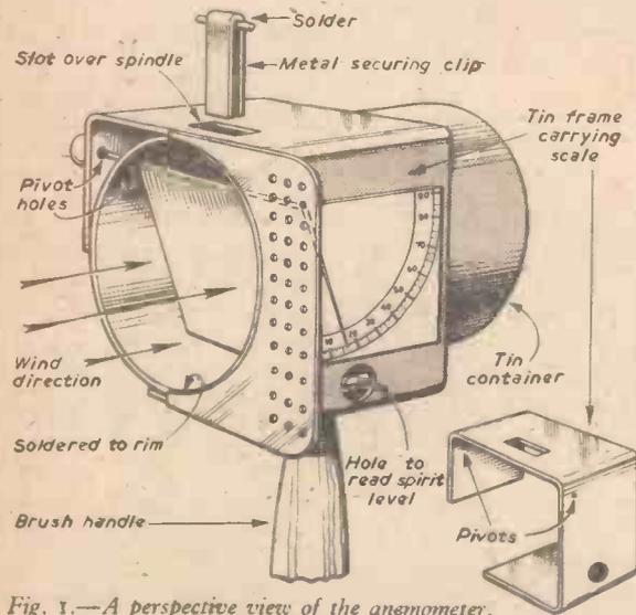
Fig. 1.—A perspective view of the anemometer.
