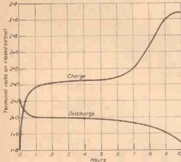
Fig. 1.—Variation of terminal voltage of a lead-acid accumulator cell on charge and discharge.
