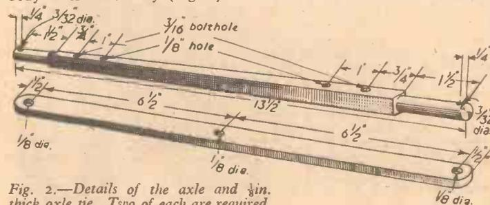
Fig. 2.—Details of the axle and  $\frac{1}{2}$  in. thick axle tie. Two of each are required.
