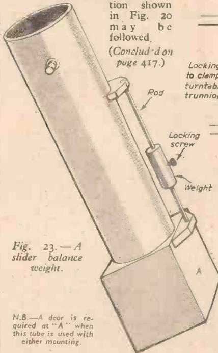
Fig. 23.—A slider balance weight.
