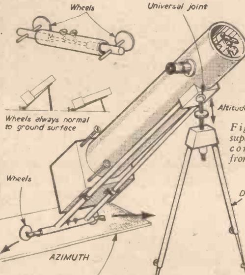
Fig. 18 (Above)—A perspective view of the Sellers dipod mounting.
