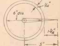
To contain the rays from a point minor axis of flat mirror must be diameter of main mirror divided by 9.6
