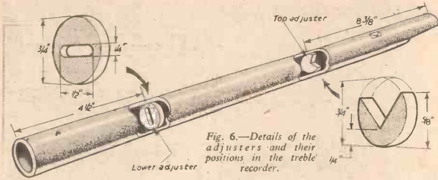
Fig. 6.—Details of the adjusters and their positions in the treble recorder.
