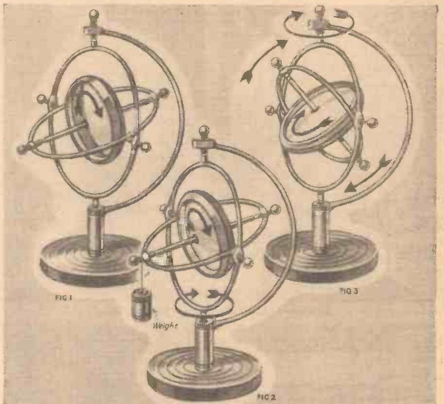
Fig. 1.—The gyroscope. Fig. 2.—A weight attached. Fig. 3.—The gyroscope turning bodily in a vertical plane.
