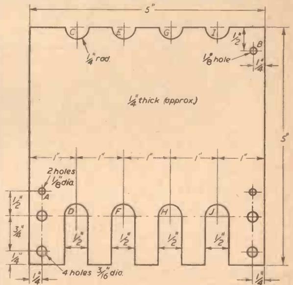
Fig. 5.—Dimensions of asbestos board resistor support.
