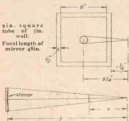
The proportion which y bears to x gives the proportion of the diameter of the mirror which the minor axis of the flat mirror must be in order to contain the rays from a point. But for anything wider than this one has in effect to deal with two cones more or less divergent. It is the outside of these cones which must be included in the minor axis
