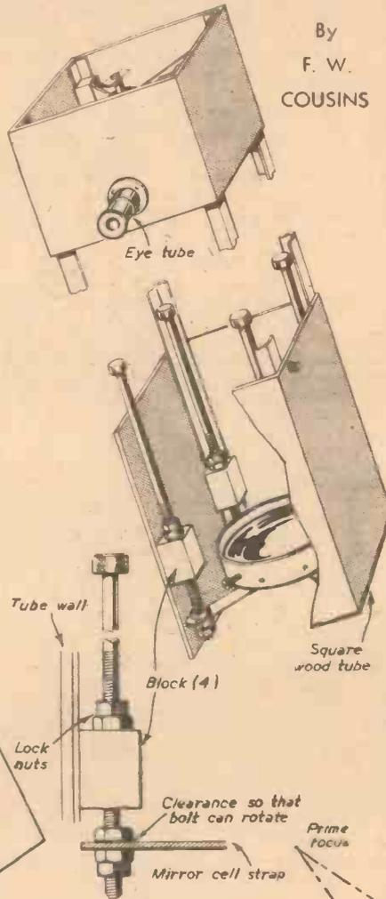
Fig. 11 (Above).—A refined mirror adjustment system.
