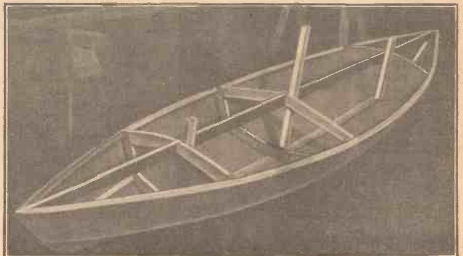
Fig. 21.—The kayak removed from the building form.
