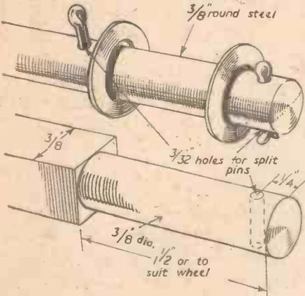
Fig. 4.—Two methods of fixing the wheels.
