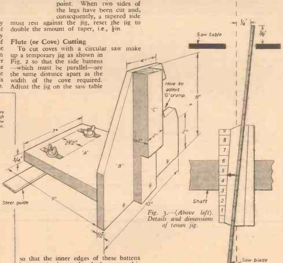
Fig. 3.—(Above left). Details and dimensions of tenon jig.
