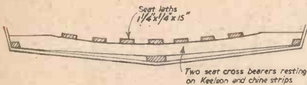
Fig. 24.—Dimensions of the seat.
