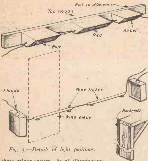
Fig. 3.—Details of light positions.
