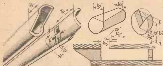
Fig. 2.—Making the recorder mouthpiece. Fig. 3.—Details and fitting of the mouth-piece plug and adjuster.
