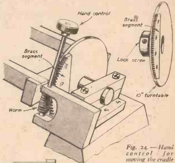
Fig. 24.—Hand control for moving the cradle in a direction counter to the earth's rotation.
