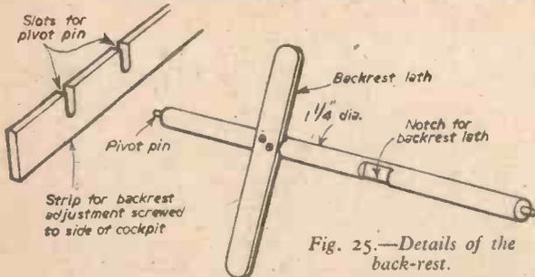
Fig. 25.—Details of the back-rest.
