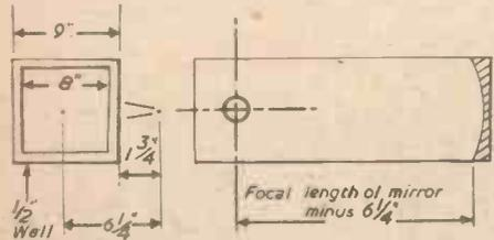
Fig. 16.—Position of eye tube for square tube.
