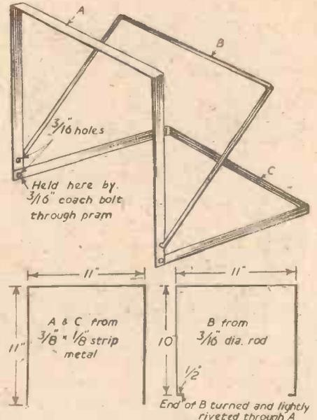
Fig. 8.—Constructing the hood frames.
