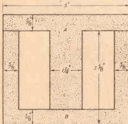
Fig. 2.—Dimensions of transformer core stampings.
