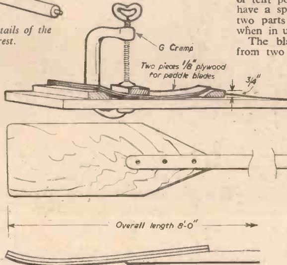
Fig. 26.—Building up the paddles and attaching the handle and drip ring.
