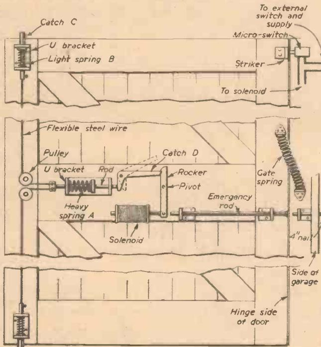
The garage door system shown diagrammatically.
