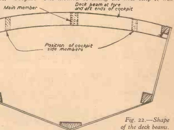
Fig. 22.—Shape of the deck beams.
