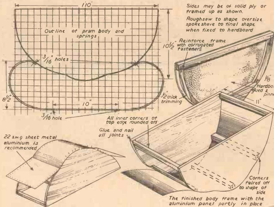
are 18 s.w.g. panel pins, and should be inserted at about 2 in. intervals starting at the middle and working the metal into the curves a little at a time. All nails and pins should be punched below the surface of hardboard or plywood, and flush with the metal surface.
