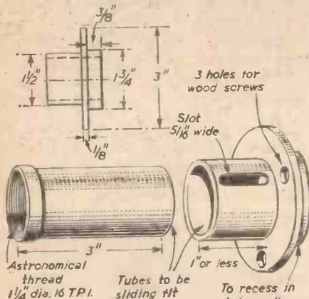
Fig. 17.—Eyepiece draw tube assembly.
