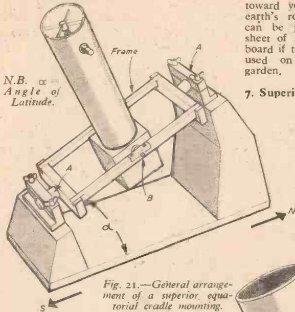
Fig. 21.—General arrangement of a superior, equatorial cradle mounting.
