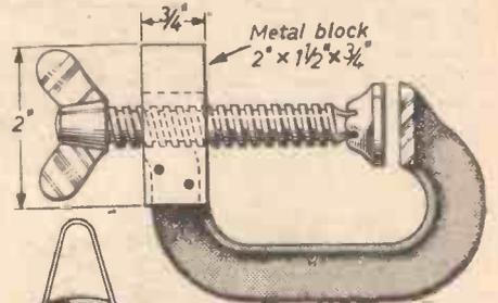
Fig. 7.—How a G-cramp is used to make the movable vice. The shaded portion is cut away.
