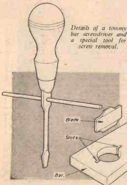
Details of a tommy bar screwdriver and a special tool for screw removal.
