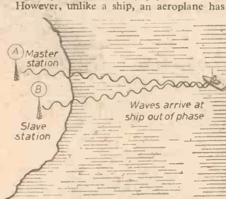
Fig. 8.—Waves from station B arrive sooner than from station A, as B is nearer. This means that the waves are out of phase.
