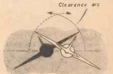
Fig. 4.—The port wing must roll through a large angle to avoid wing scything.
