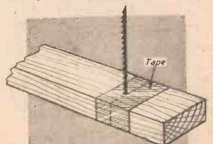
TO prevent splitting when sawing through small strips of wood on the fret-machine, simply wrap a piece of transparent adhesive tape round the strip at the point of the cut.
