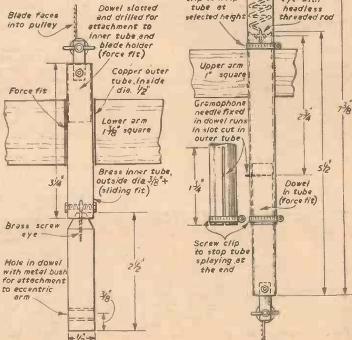
Fig. 3.—Full details of the head and toe of the jig-saw.
