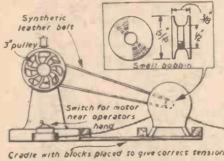
Fig. 5.—Details of the sewing machine electrification.
