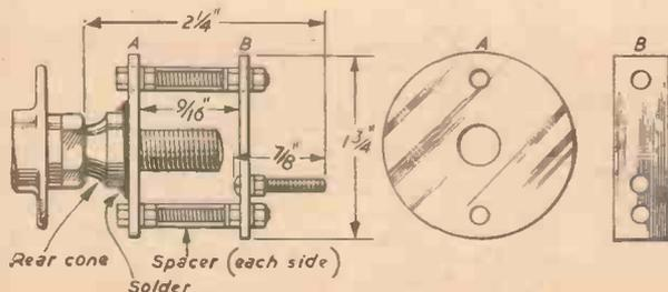
Fig. 2.—Details of the eccentric device.
