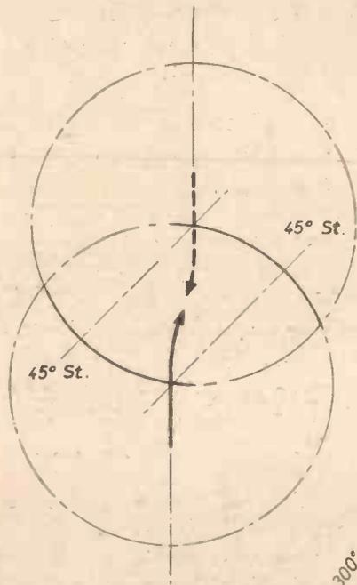
Fig. 7.—The dangerous sector—both aircraft swing to starboard.
