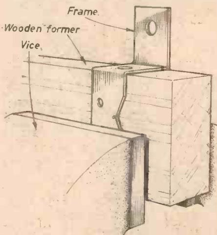
Fig. 3.—Bending the frames using a wooden former and vice.
