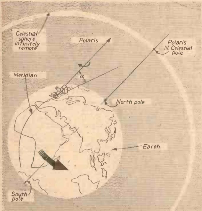
Fig. 2.—How the telescope is placed on the meridian.
