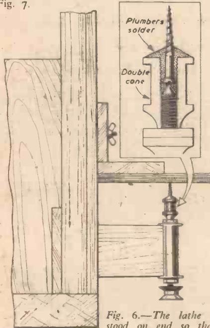
Fig. 6.—The lathe is stood on end so that the screw centre is vertical.
