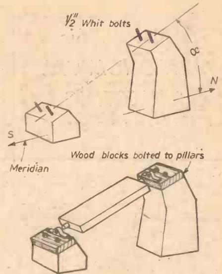
Fig. 4.—Suggested design for a rigid concrete mounting for the cradle.
