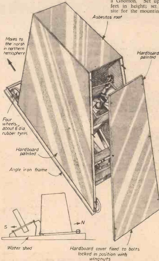
Fig. 1.—A simple run-off shed to protect the cradle-mounted telescope, for photography and
