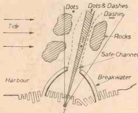
Fig. 5.—Entering a dangerous harbour by following the narrow path where both dots and dashes are audible.
