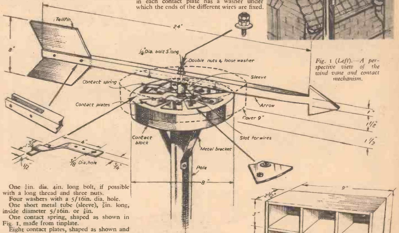
One 1/2in. dia. 4in. long bolt, if possible with a long thread and three nuts.
