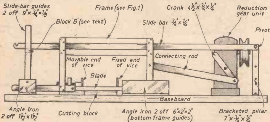
Fig. 4.—A front view of the completed machine.
