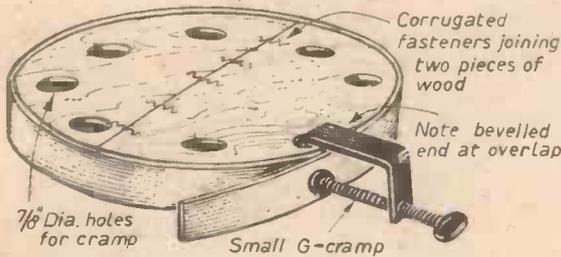
Fig. 4.—Cramping the hoop strip around the former.
