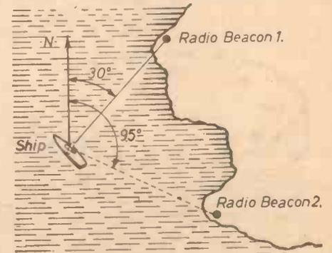
Fig. 3.—How a "fix" can be obtained from two shore-based radio beacons.
