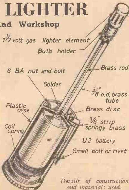
Details of construction and material used.
