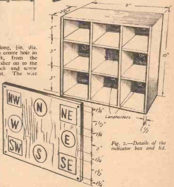
Fig. 2.—Details of the indicator box and lid.
