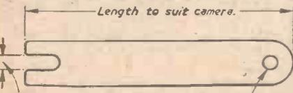
To fit under tripod bush screw. 2 B.A. clearance.
