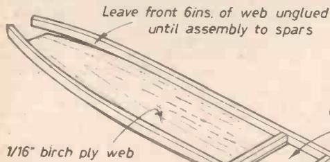
Fig. 7.—Perspective view of a tailplane rib.
