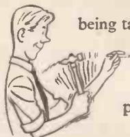
A. Keep turning the tool as it is being tapped with a light hammer. This prevents the tool jamming in the hole. A succession of light rapid blows will more quickly penetrate the masonry than heavy blows with a large hammer.
