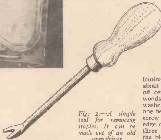
Fig. 2.—A simple tool for removing staples. It can be made out of an old screwdriver.
