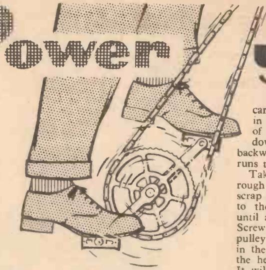
ance to the pedals when the device is screwed to the floor. One inch from the bottom of the "feet" make a small hacksaw cut and hammer in the upper side of the frame tube, making a hole for the fastening screw (Fig. 1). Screw the pedalling frame to the floor beneath the bench at a point directly beneath where the lathe headstock will be.
