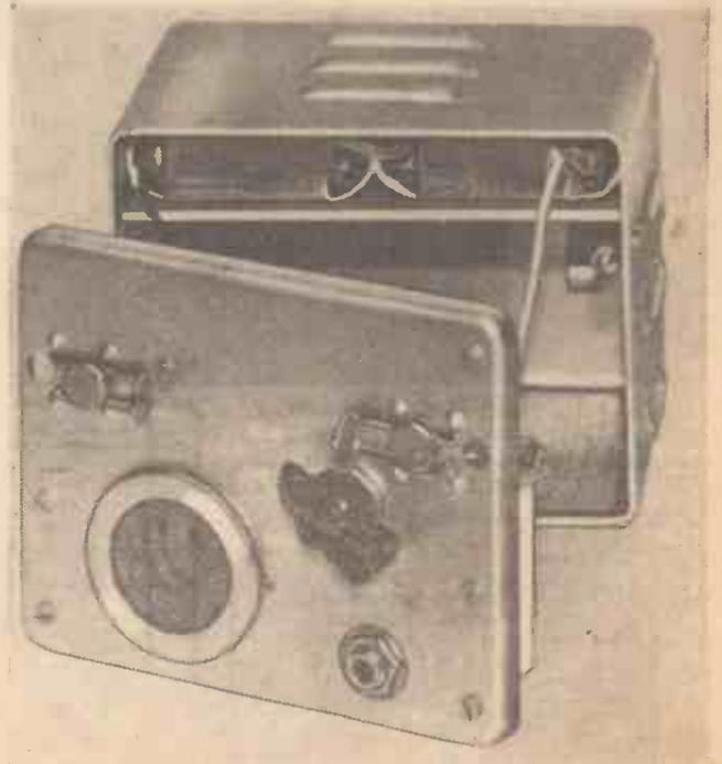
Fig. 5.—Front view showing battery shelf.
