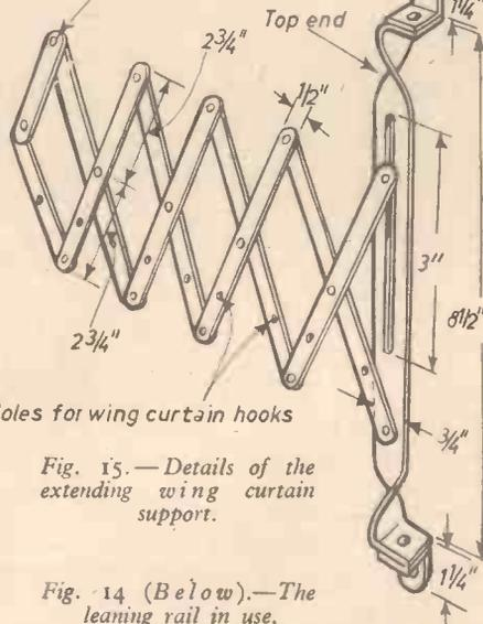
Fig. 15.—Details of the expanding wing curtain support.
