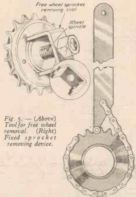
Fig. 5.—(Above) Tool for free wheel removal. (Right) Fixed sprocket removing device.
