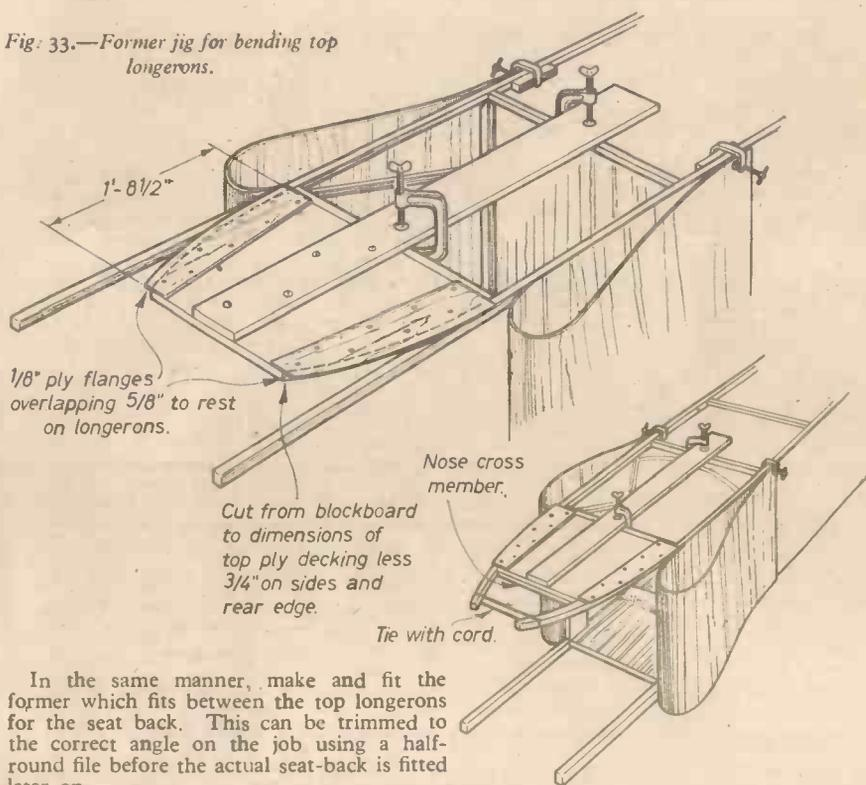
In the same manner, make and fit the former which fits between the top longerons for the seat back. This can be trimmed to the correct angle on the job using a half-round file before the actual seat-back is fitted later on.
