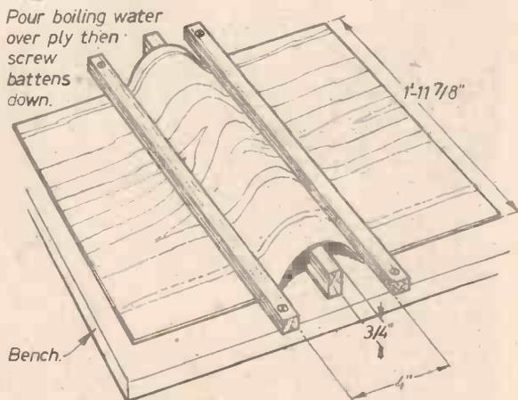
Fig. 32.—Pre-forming floor ply for seat cross supports.
