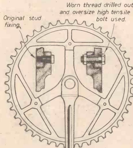
Fig. 1.—The three-pin chainwheel and method of dealing with worn threads.
