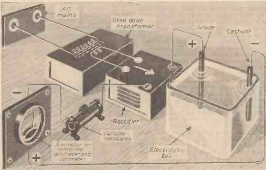
Fig. 1.—The electroplating circuit shown pictorially.
