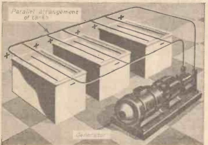
Fig. 2.—Parallel arrangement of tanks.
