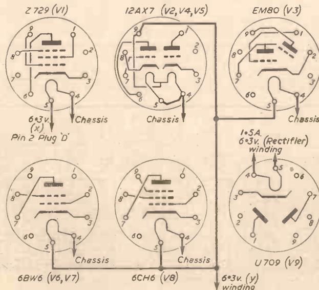
Fig. 20.—Valve base details showing heater wiring.
