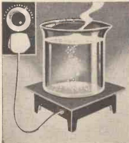
Fig. 4.—Apparatus for raising the temper of plating solutions.
