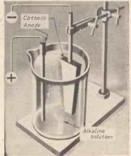
Fig. 6.—Apparatus for electrolytic cleaning.
