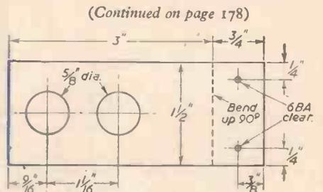
Fig. 7.—Sub-chassis detail.
