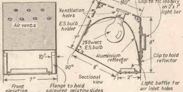
Fig. 21.—Details and dimensions of the lighting boxes.
