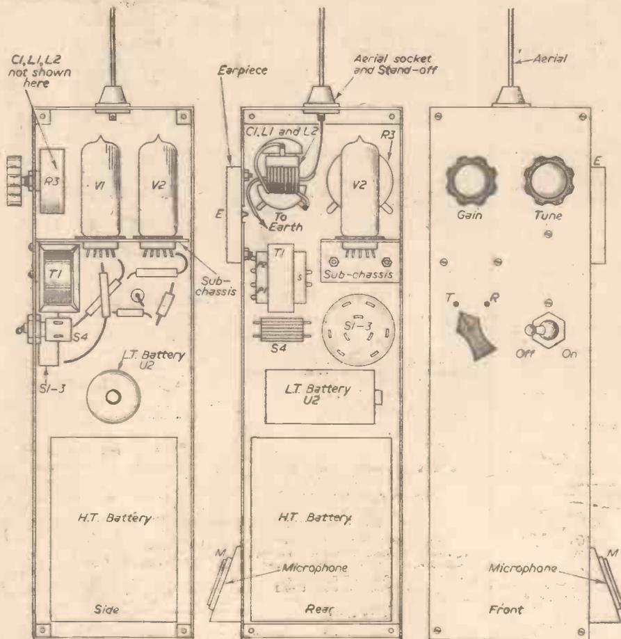
Fig. 8.—Internal and front panel layout.
