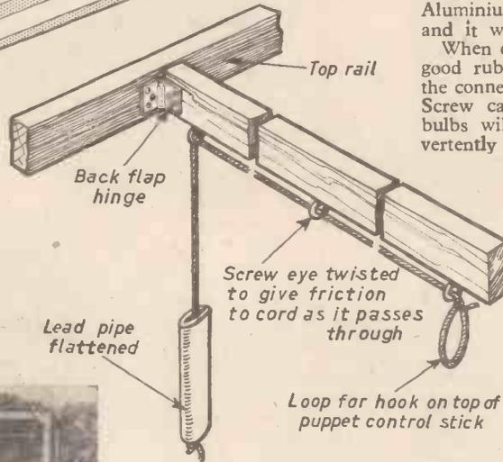
Fig. 19.—Details of the gallows for supporting the puppets when not in use.
