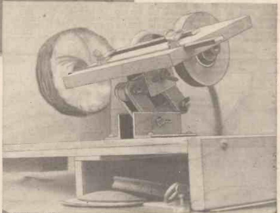
are provided with a central ¼in. hole in the uprights. The upper pair, screwed to the underside of the table, have a ¼in. slot about 1½in. long cut in the upright flanges. Quarter-inch bolts pass through these holes and slots and thus permit the lattice assembly to swing in the lower pair of brackets and both swing and travel along the upper pair. Fig. 5 furnishes a perspective view of this mechanism.
