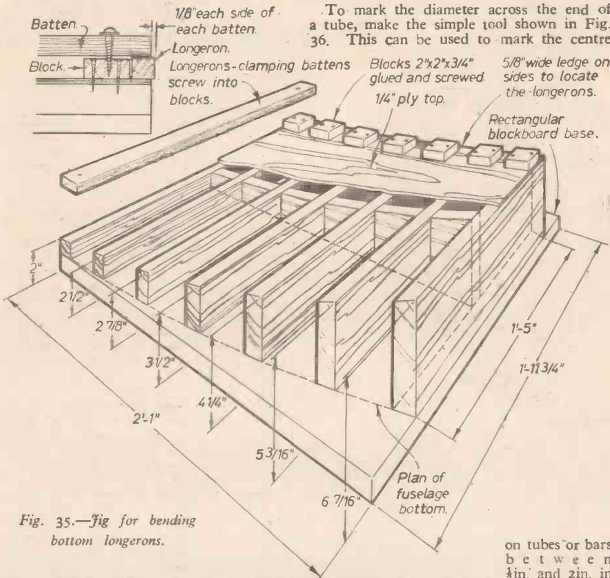
Fig. 35.—Jig for bending bottom longerons.
