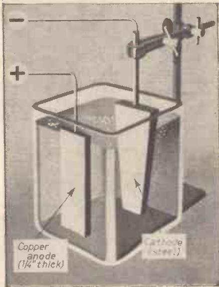
Fig. 3.—A plating tank suitable for the amateur.
