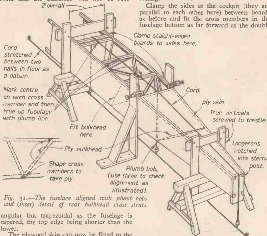
Fig. 31.—The fuselage aligned with plumb bobs and (inset) detail of rear bulkhead cross struts.
