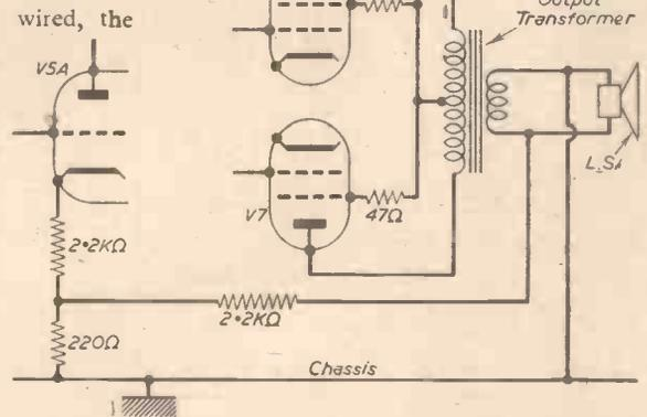
Fig. 21.—Modification to obtain 7 watts output.
