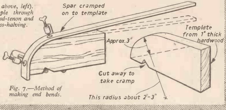
Fig. 7.—Method of making end bends.
