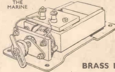
The Marine motor is a powerful permanent magnet unit suitable for model boats up to 39 ins. long and will give many years' service. It will operate from two 3-cell dry batteries coupled in series or from a 6-volt accumulator. Length 3 $\frac{1}{2}$  ins. Width 2 ins. Height 1 $\frac{1}{2}$  ins. Weight 11 $\frac{1}{2}$  ozs. Price 63/3
