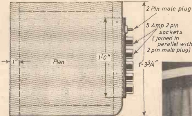
Fig. 23.—Dimensions of the record player table and electric supply board.
