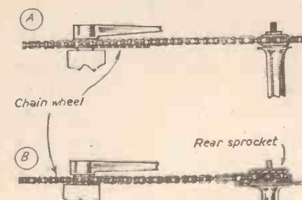
Fig. 4.—(A) Chain out of line. (B) Chain correctly lined up on centre sprocket.
