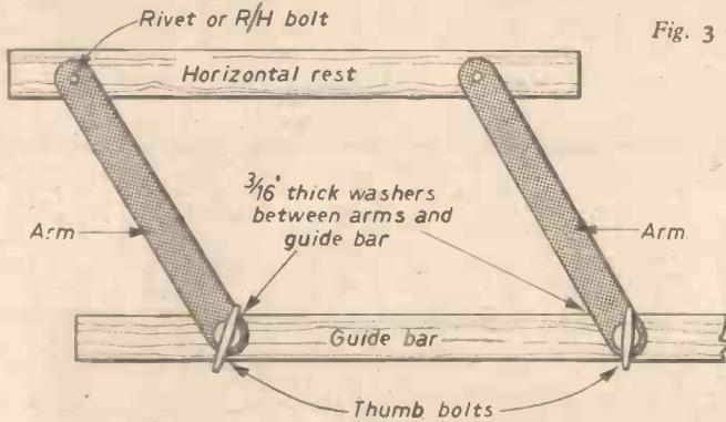
Fig. 3 (Left).—The horizontal or parallel rule rest. Fig. 4 (Below).—Sliding angle gauge and oak table.
