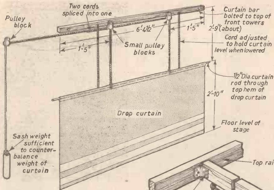
Fig. 17.—Details of the curtain raising and lowering mechanism.
