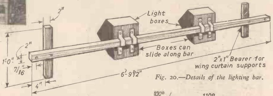
Fig. 20.—Details of the lighting bar.
