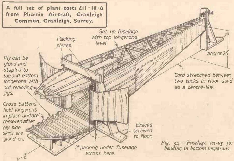
Fig. 34.—Fuselage set-up for bending in bottom longerons.
