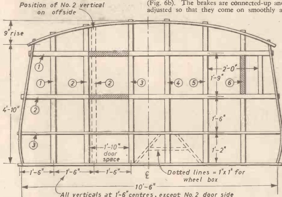
Fig. 9a.—Details of the side framing.
