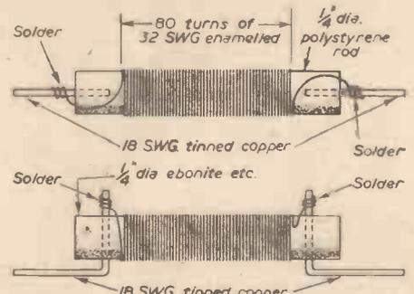
Fig. 3.—R.F. choke construction.
