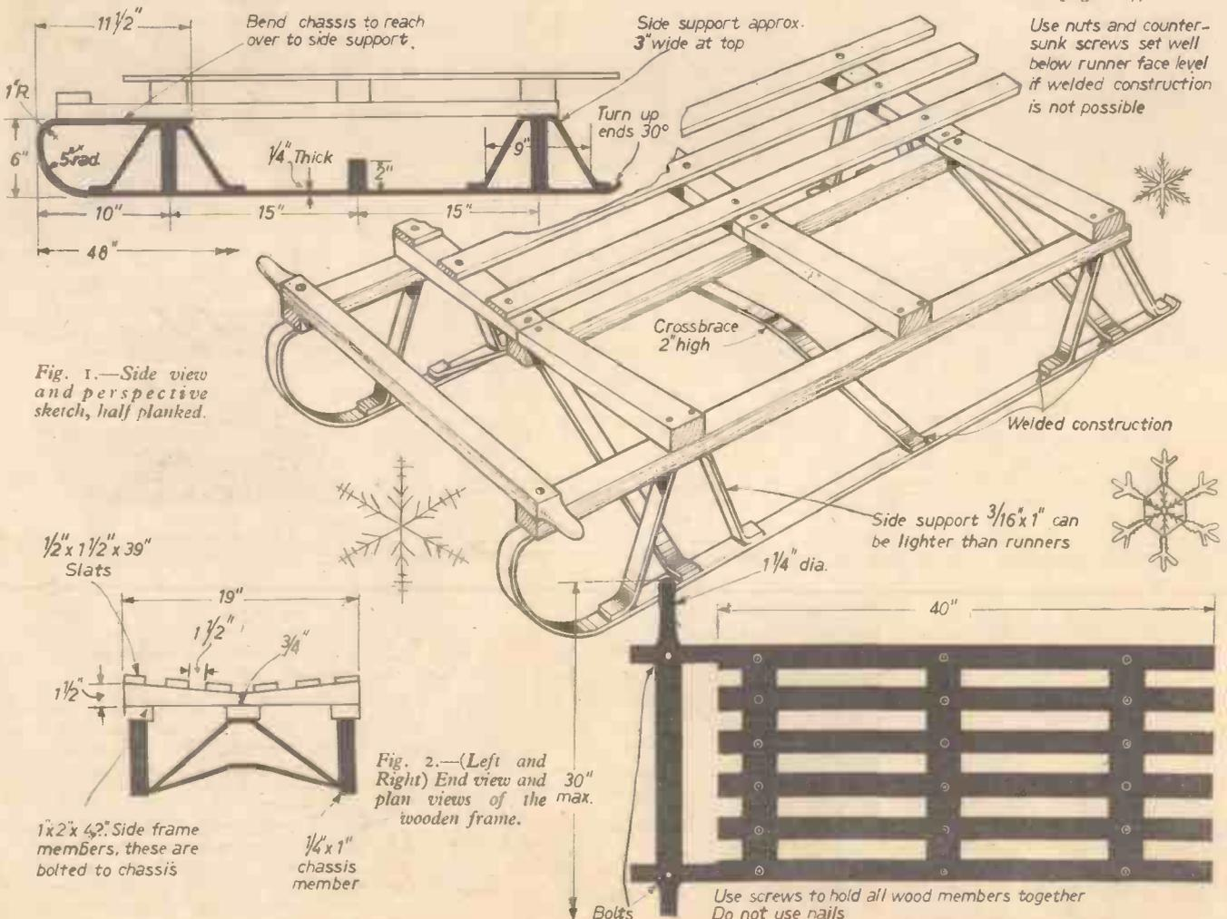
Fig. 1.—Side view and perspective sketch, half planked.
