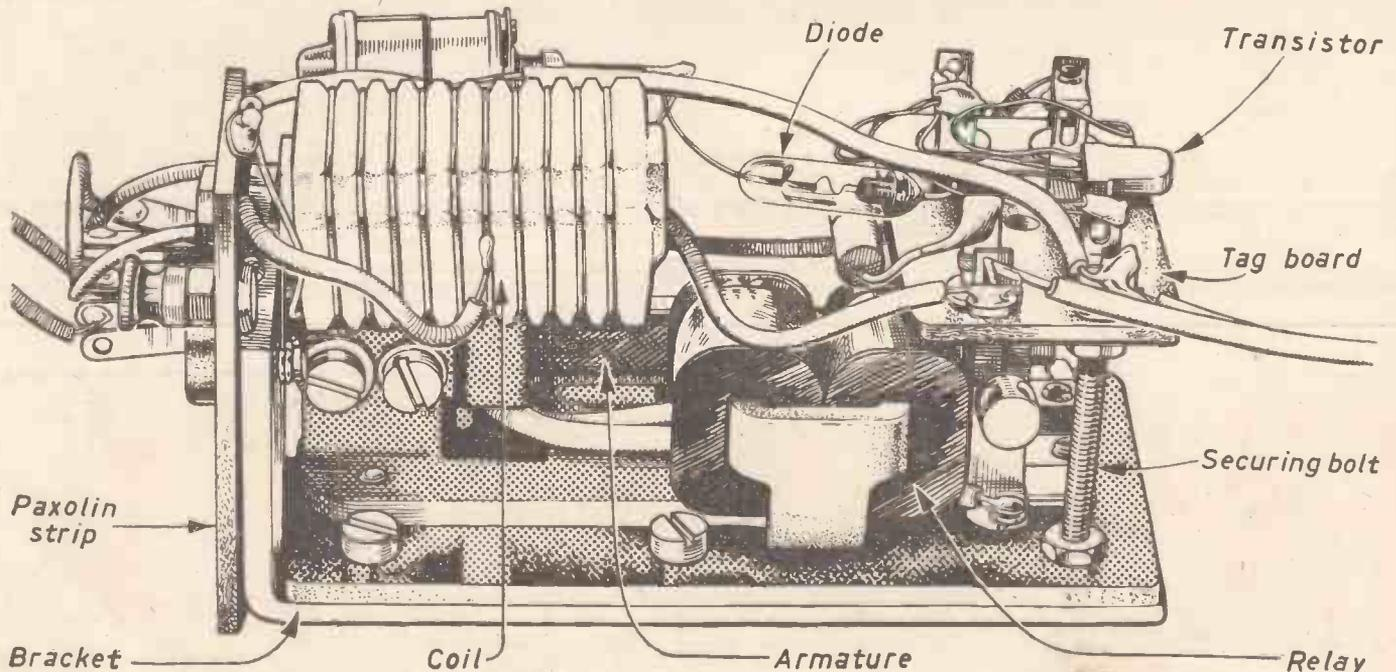
Fig. 1.—An enlarged perspective view of the completed receiver showing some of the principal wiring.
