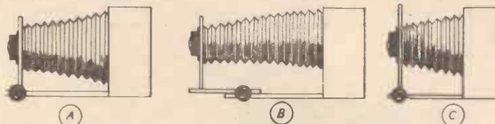
Fig. 1 (A).—The lens at normal closest focus—about 3ft. ; (B) using double extension, lens distant twice its focal length from negative, giving life-size image ; (C) distant view—lens closer to negative than at (A).
