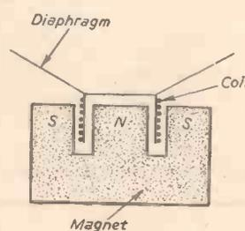
Fig. 6.—Moving coil microphone.
