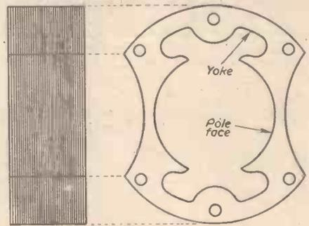
Fig. 4.—A laminated stator field system.
