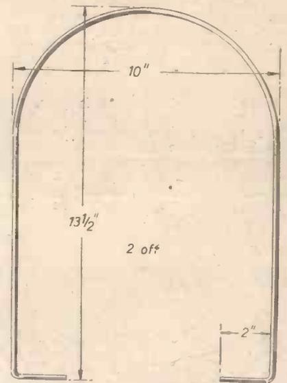
Fig. 5.—Wire ribs to support leather covering.
