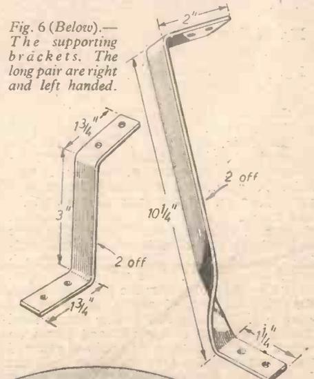
Fig. 6 (Below).—The supporting brackets. The long pair are right and left handed.
