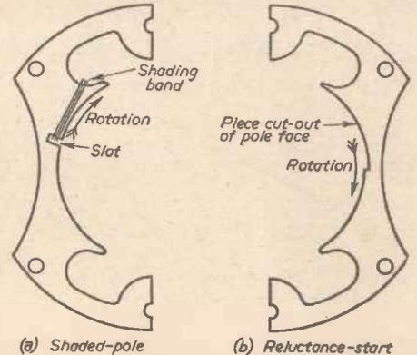
Fig. 10.—Modification of laminated field systems for operation on A.C.
