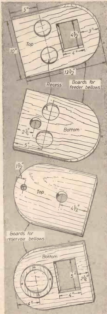
Figs. 1 and 2.—Details of the top and bottom of the feeder bellows and reservoir bellows respectively.
