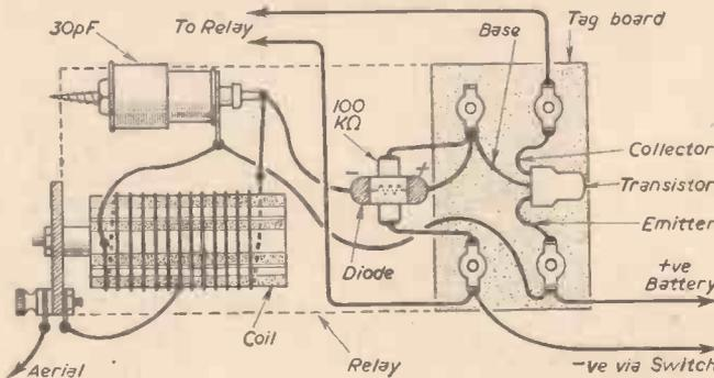
Fig. 5 (Below).—A view showing coil and tagboard mounting.
