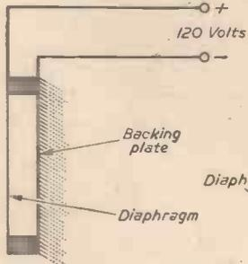
Fig. 2.—Condenser microphone.
