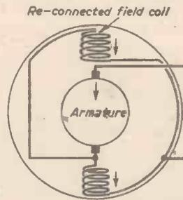
Fig. 7.—Reconnection of series field coils in parallel with each other.
