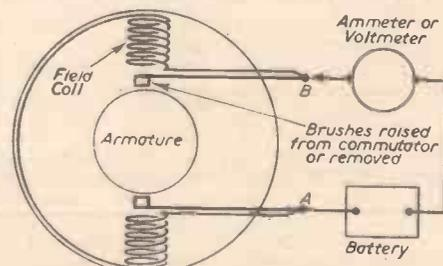
Fig. 3.—Method of testing connections of field windings.
