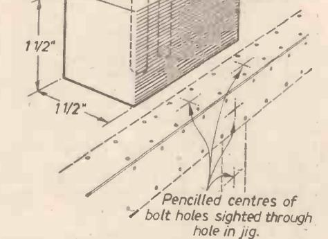
Fig. 40.—Jig for aligning drill when boring holes.
