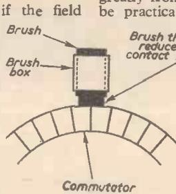
Fig. 8.—Method of reducing brush thickness.
