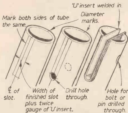
Fig. 37.—The three stages in marking out, cutting and finishing a tube fork-end.
