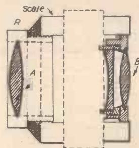
Fig. 2.—Rotation of the inner screws, by focus ring R, varies the position of front cell A in relation to fixed back cell B.
