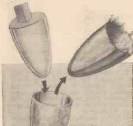
Fig. 3.—The sequence of using a male mould, then using the resulting female laminate as a mould to form the final laminates.
