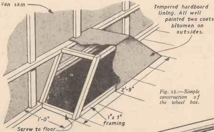
Fig. 12.—Simple construction of the wheel box.
