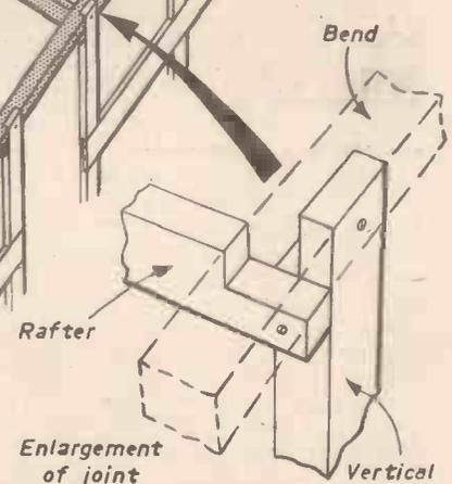
made, by wetting them and bracing them over a pile of bricks. It is not essential to do this as the roof curve is quite a small one, but it does help to reduce the tension.
