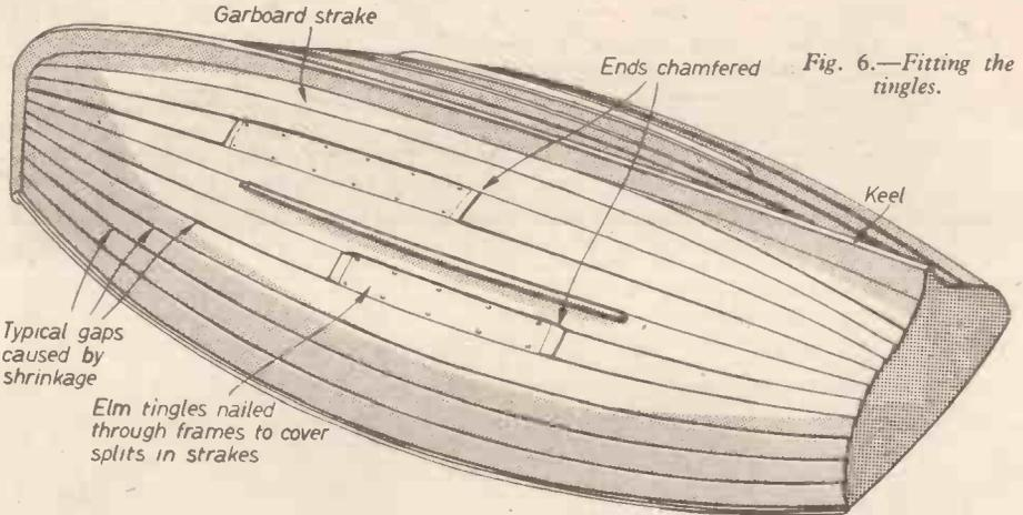
Fig. 6.—Fitting the tingles.
