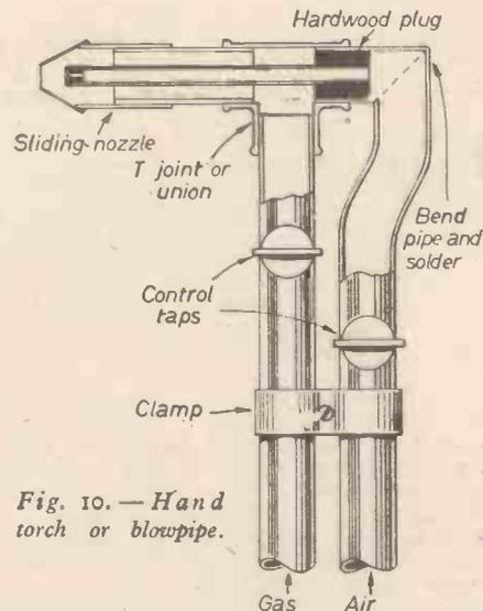
Fig. 10.—Hand torch or blowpipe.
