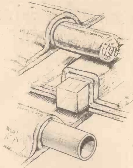
Fig. 5.—Three examples of bonded ribs for reinforcement.
