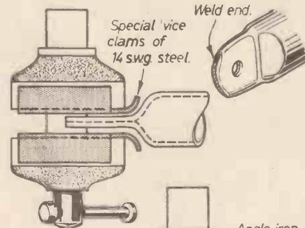
Fig. 38.—How to flatten a tube end in a vice. Heat tube cherry-red before and after forming.
