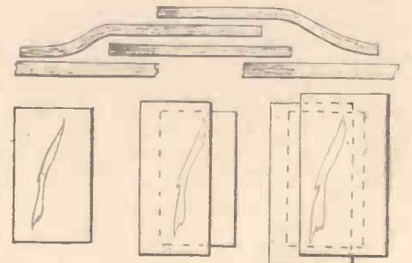
Fig. 8 (Right).—The procedure for repairing tears and splits.
