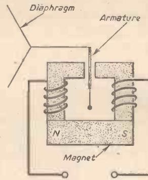
Fig. 5.—Balanced armature microphone.
