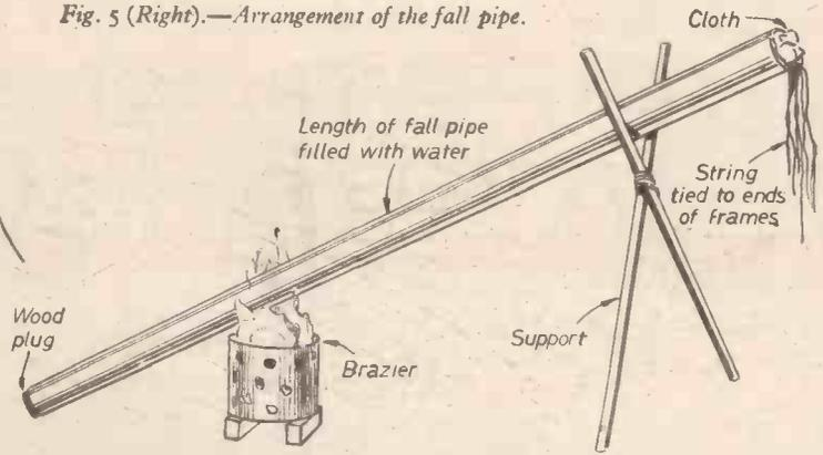
Fig. 5 (Right).—Arrangement of the fall pipe.
