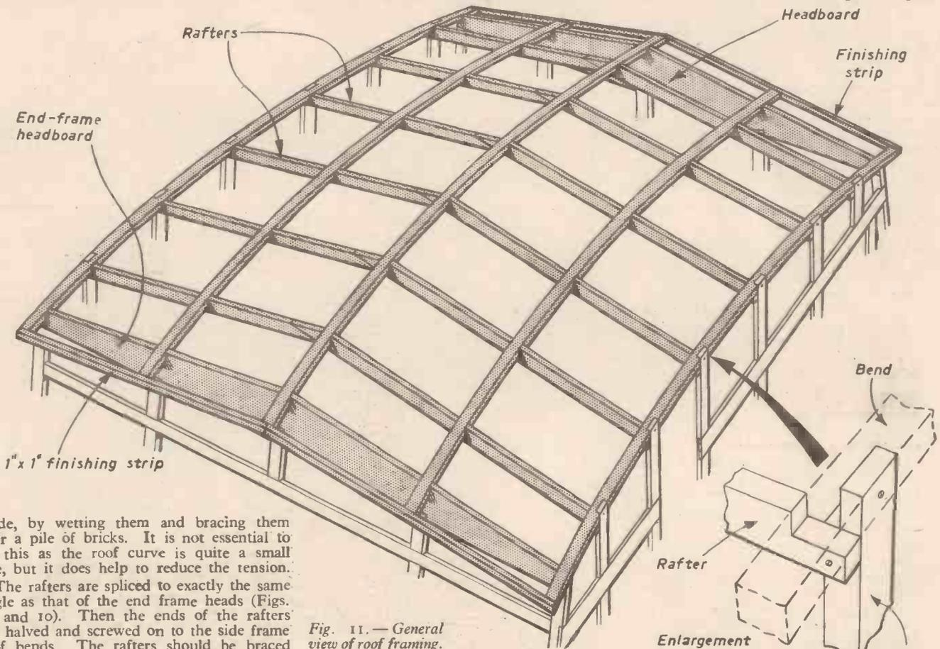
Fig. 11.— General view of roof framing.
