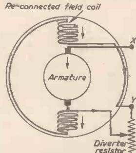
Fig. 6.—Use of a diverter resistor with a series motor.
