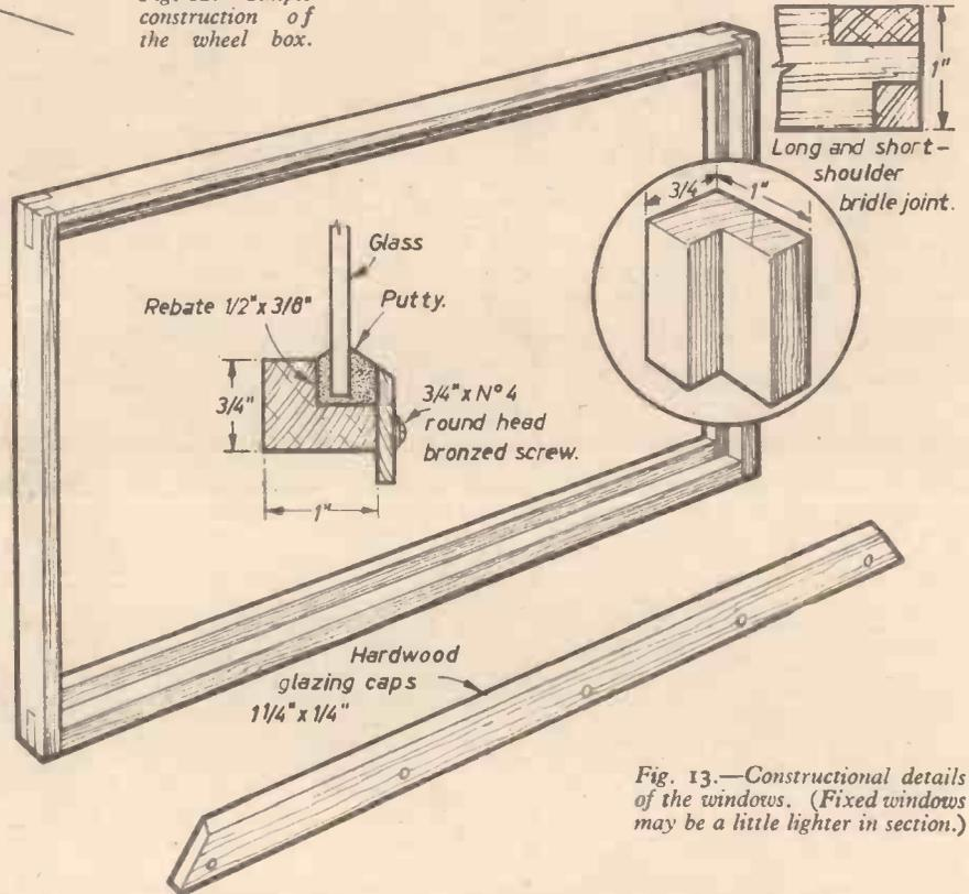
Fig. 13.—Constructional details of the windows. (Fixed windows may be a little lighter in section.)
