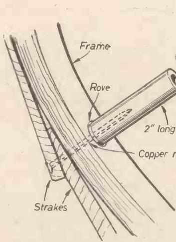
Fig. 4.—The tool used for fixing the rove.
