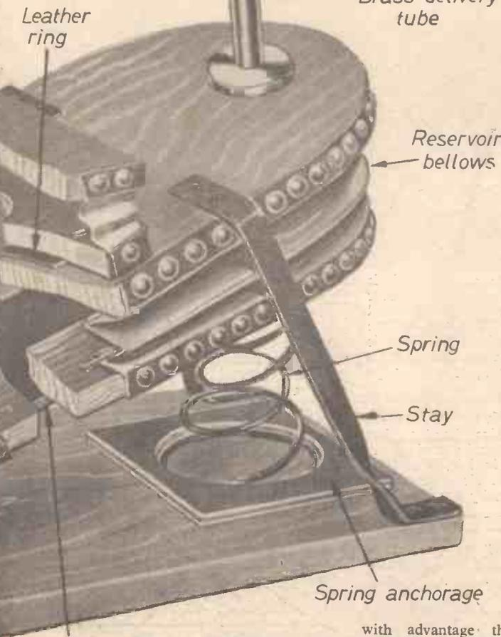
Fig. 4.—A perspective view of the bellows cut away to show the valves and springs.
