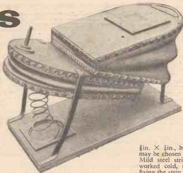
shown in Fig. 3. These blanks when filed up and flat should be drilled, countersunk, and each pair bent to shape on a temporary pin of 8 s.w.g. rod or wire. The trouble entailed in making the hinge system can be minimised by purchasing steel or brass flap hinges, withdrawing the pins, and drilling out, if the hole or barrel is too small to take 8 s.w.g. rod. Two ribs of 8 s.w.g. galvanised iron wire are now made, one for each bellows, to support the leather cover, and are shaped
