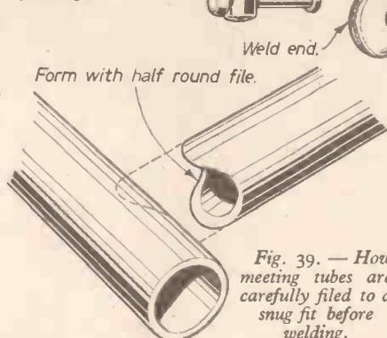
Fig. 39.—How meeting tubes are carefully filed to a snug fit before welding.
