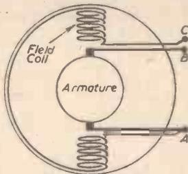
Fig. 2.—Connections of a two-pole shunt motor.
