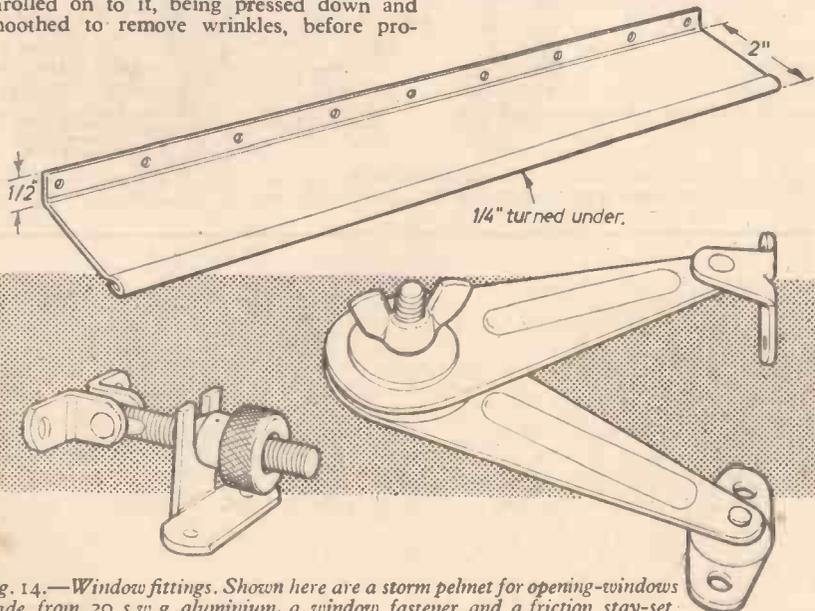
Fig. 14.—Window fittings. Shown here are a storm pelmet for opening-windows made from 20 s.w.g. aluminium, a window fastener and a friction stay-set.
