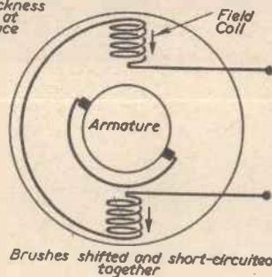
Fig. 9.—Arrangement of a repulsion motor.
