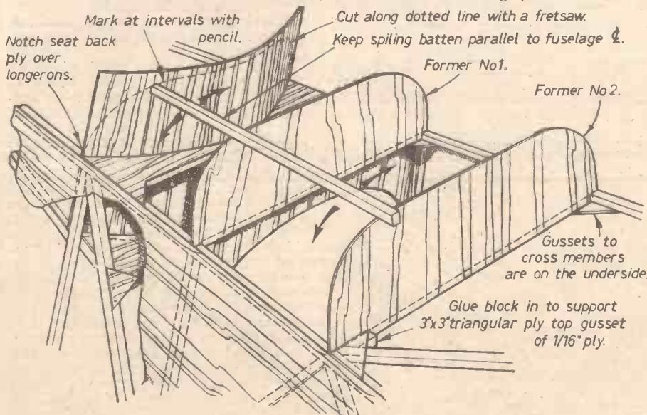
Fig. 42.—How to mark out the curve of the seat back former.
