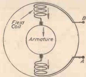
Fig. 1.—Connections of a two-pole series motor.
