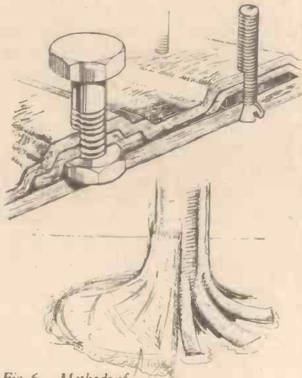
Fig. 6.—Methods of including nuts, bolts and brackets in a laminate.
