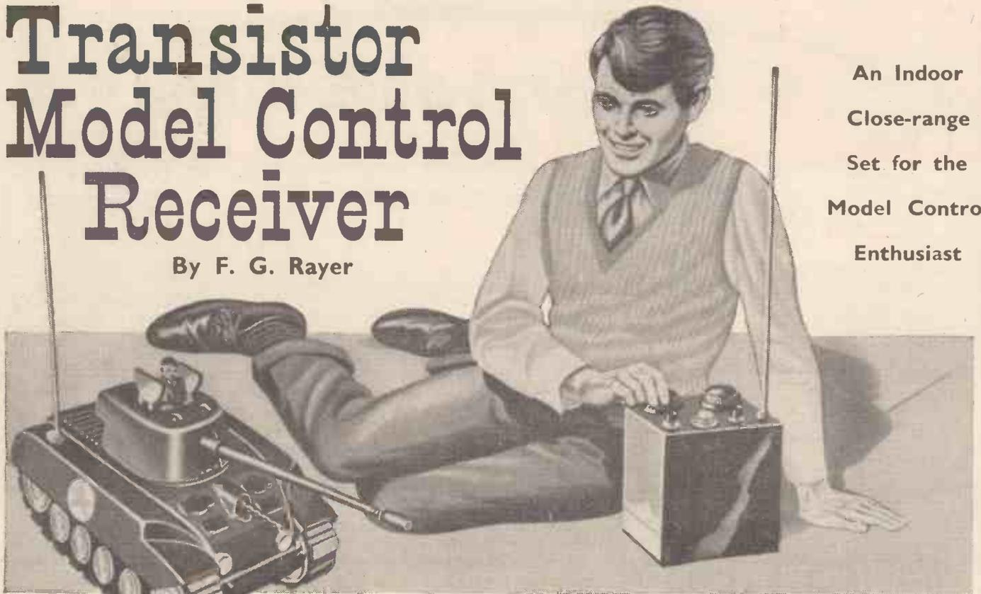
Only One Transistor is Used and Power is Obtained from 4½V. Dry Batteries
