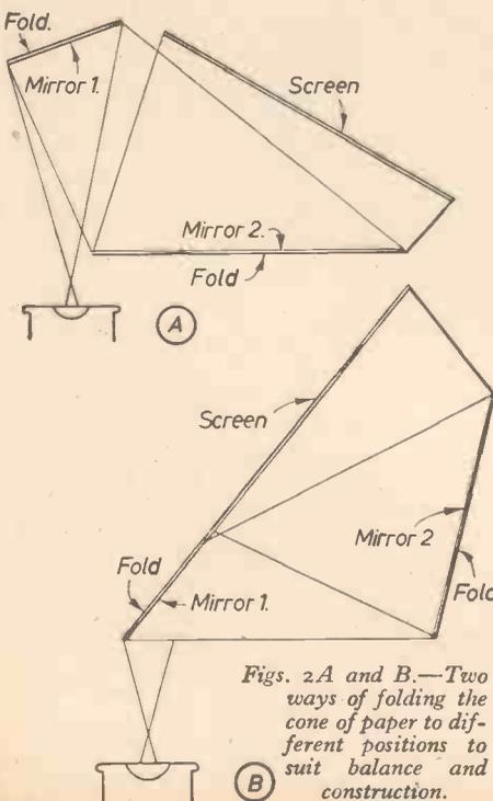
Figs. 2A and B.—Two ways of folding the cone of paper to different positions to suit balance and construction.
