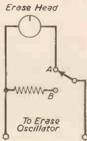
Fig. 3.—Circuit for making erase head inoperative during superimposition.
