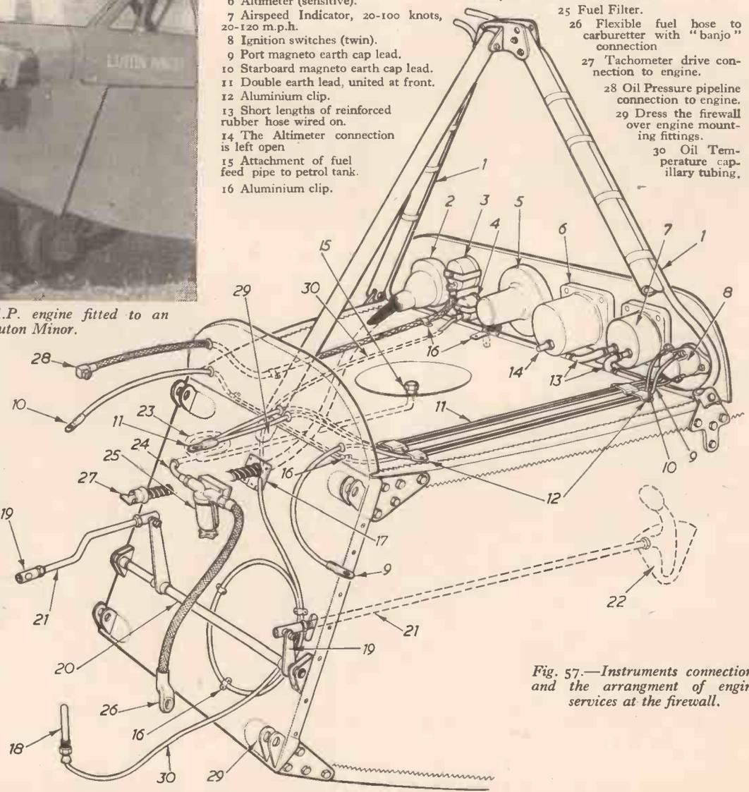
Fig. 57.—Instruments connections and the arrangement of engine services at the firewall.
