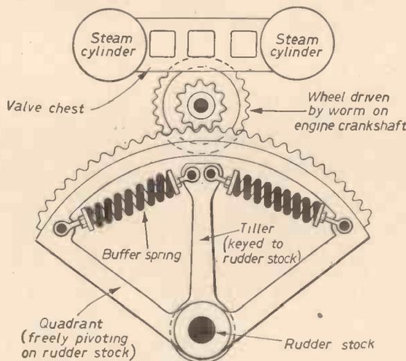
Fig. 2.—Steam steering gear.
