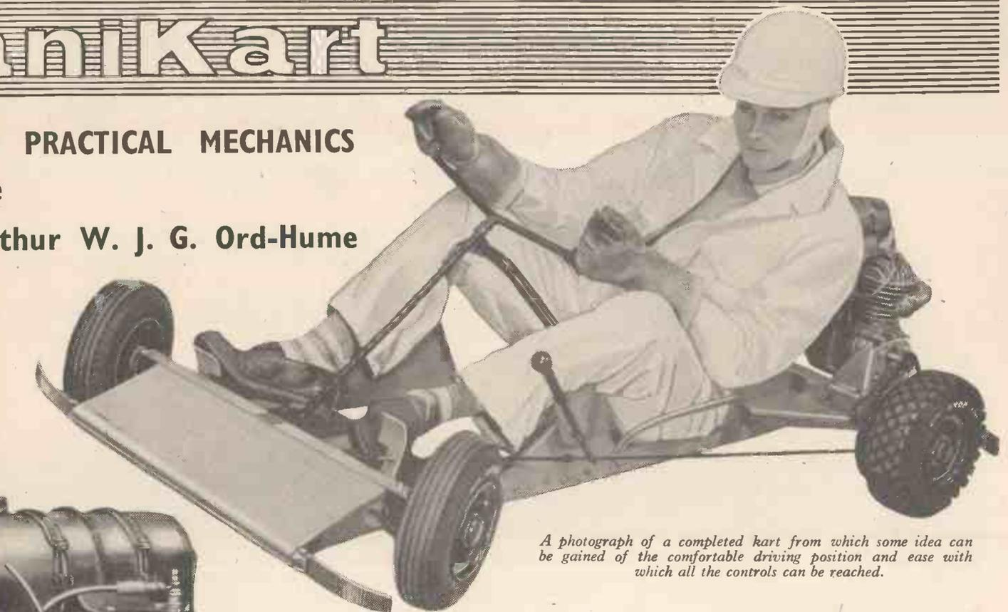
*A photograph of a completed kart from which some idea can be gained of the comfortable driving position and ease with which all the controls can be reached.*
