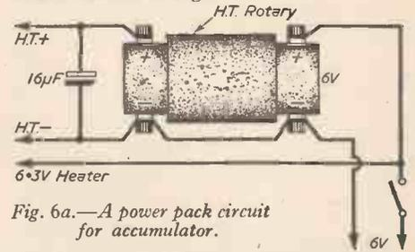
Fig. 6a.—A power pack circuit for accumulator.
