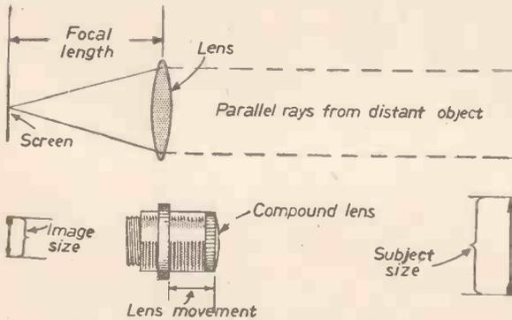
Fig. 1.—Finding the focal length of a lens.
