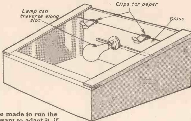
THIS can be in the form of a light box, which can be simply made of wood, as shown above. The glass top is open along the back so that clips can be used for holding the original and tracing paper. The lamp is on a bracket which may be traversed from side to side. With the light shining through, tracing graphs or other originals becomes a simple matter. The sketch above shows construction.
