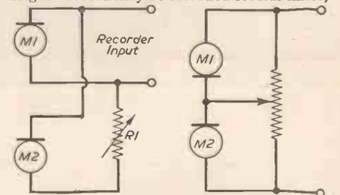
Figs. 4. and 5.—Two mixing Circuits.
