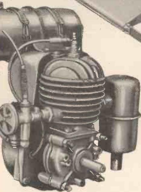
*A view of the J.A.P. model JS8 two-stroke engine. Details of this engine are obtainable from the Villiers Engineering Co., Ltd., Marston Road, Wolverhampton. The silencer is discarded and an elbow exhaust pipe fitted.*
