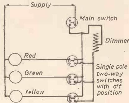
conjunction with a separate switch for each colour of lamp. If you require to be able to switch each lamp instantly from the dimmer to full strength, each outlet circuit could be controlled by means of a single-pole two-way switch as indicated above, each having an "off" position.
