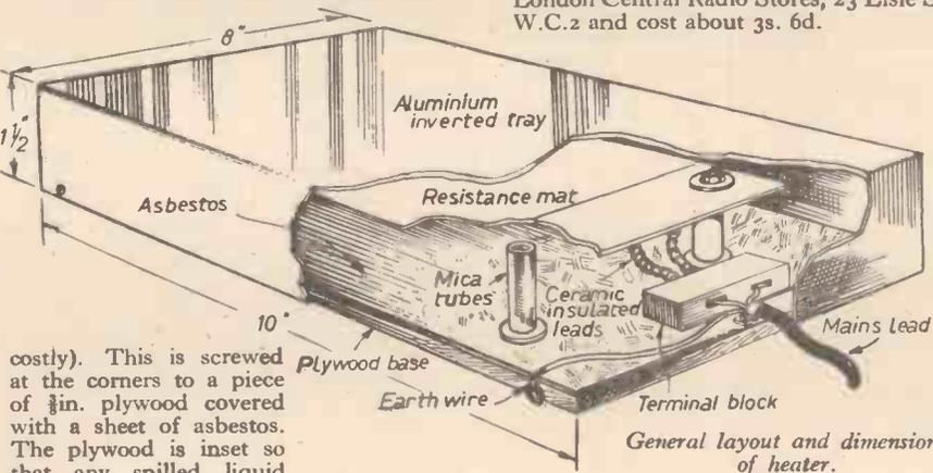
costly). This is screwed at the corners to a piece of  $\frac{1}{2}$  in. plywood covered with a sheet of asbestos. The plywood is inset so that any spilled liquid
