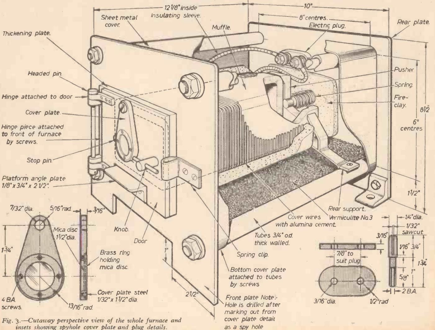
Fig. 3.—Cutaway perspective view of the whole furnace and insets showing spyhole cover plate and plug details.
