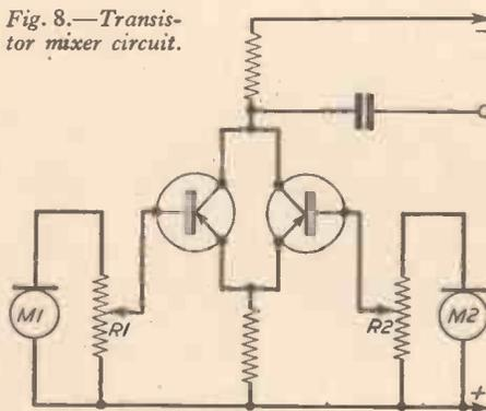
the variable resistance  $R_1$ , which can control only one of the signals. In practice, the recorder input would be adjusted to receive the signal from  $M_1$ , and then  $R$ , would be adjusted until  $M_2$  was balanced with  $M_1$ . The value of  $R_1$  depends, of course, on the impedances of the inputs.
