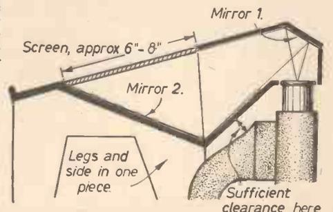
Fig. 5.—Side view of large projection unit for use with a strong light.
