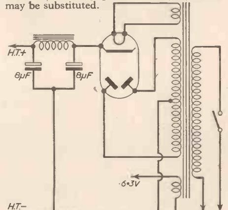
Fig. 6b.—Power pack circuit for A.C. mains.
