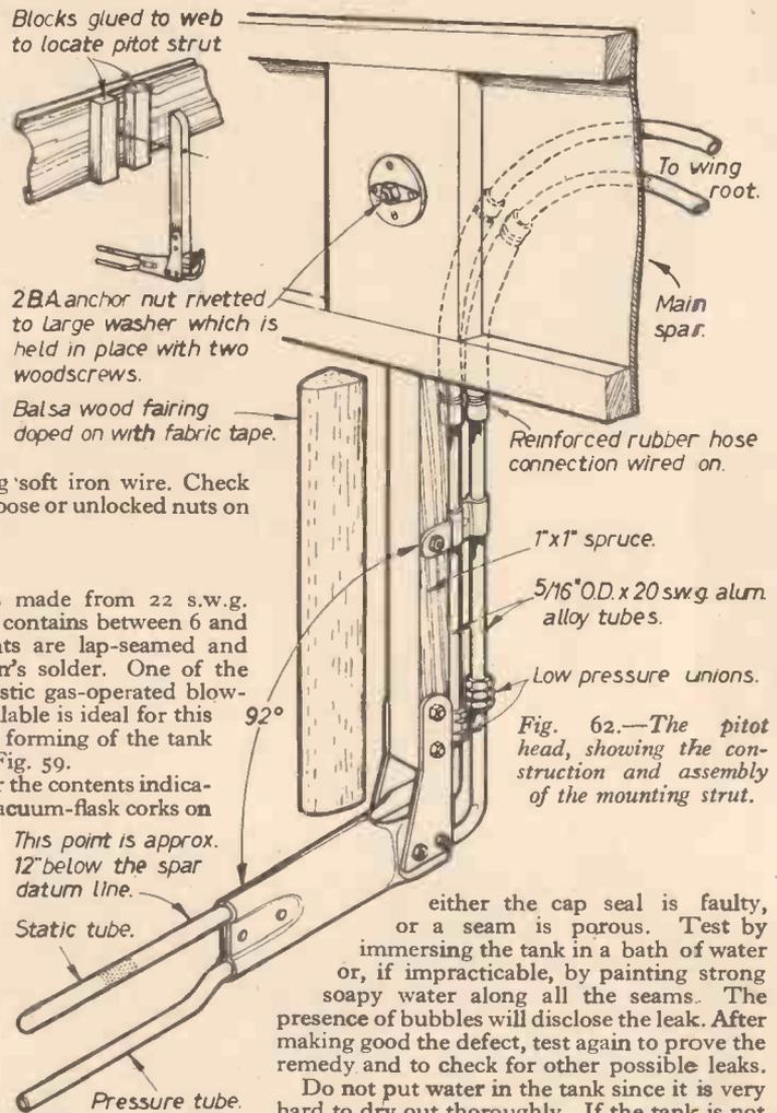
Fig. 62.—The pitot head, showing the construction and assembly of the mounting strut.
