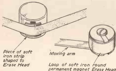
Fig. 2.—Two further methods of cutting out the erase head.
