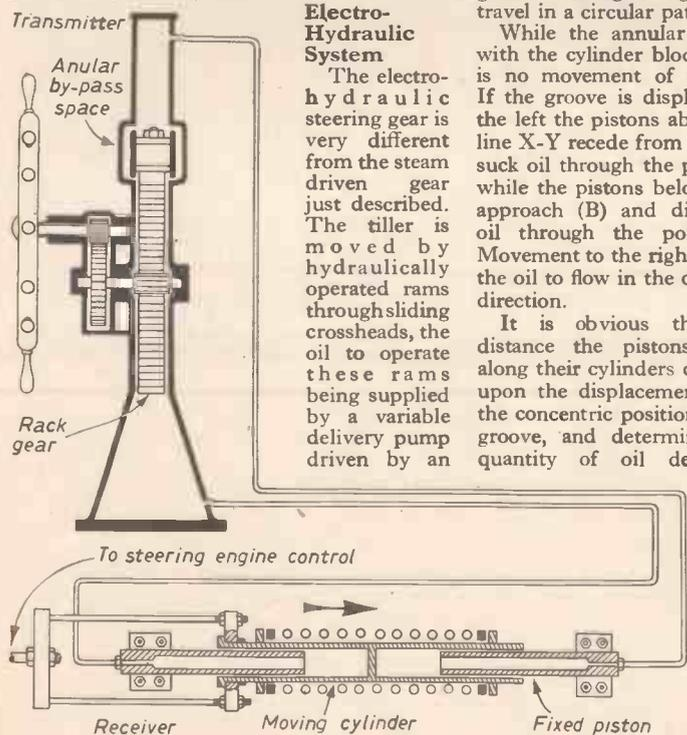
Fig. 6.—Telemotor control system.
