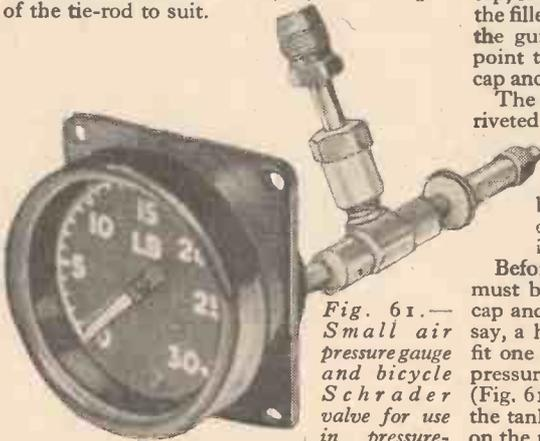
Fig. 61.—Small air pressure gauge and bicycle Schrader valve for use in pressure-testing the tank for leaks.
