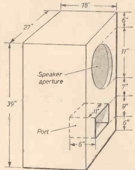
Fig. 3.—Inside dimensions of a cabinet with a ducted port.
