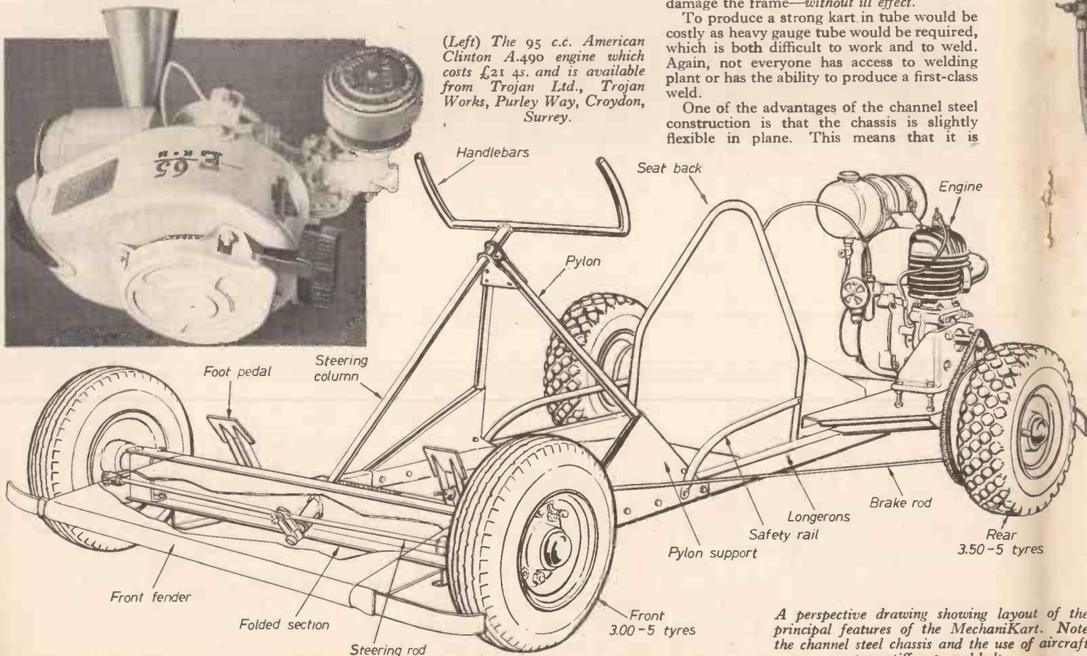
A perspective drawing showing layout of the principal features of the MechaKart. Note the channel steel chassis and the use of aircraft type stiff-nuts and bolts.
