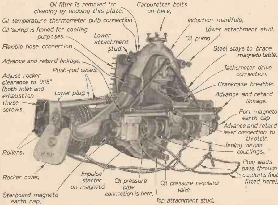
Fig. 58.—Some of the engine details shown to facilitate installation; the engine is upside down and viewed from the rear.
