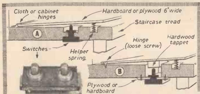
Fig. 1.—The pressure pad and two methods of switch mounting.
