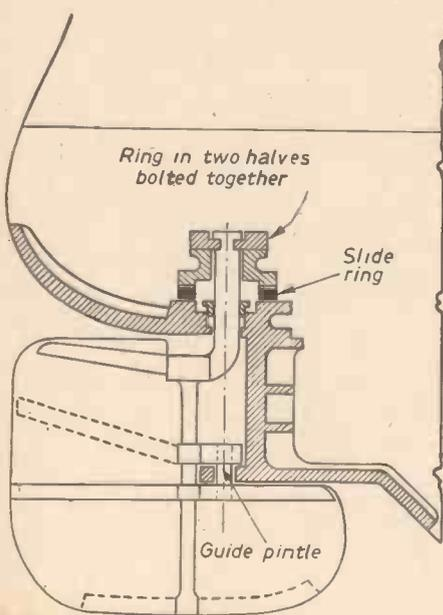
Fig. 1.—A balanced rudder.
