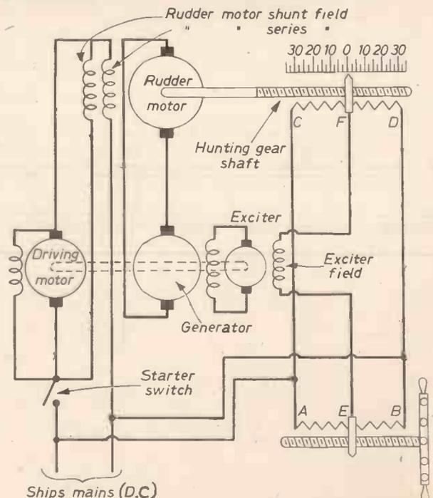
Fig. 7.—Electric steering gear.
