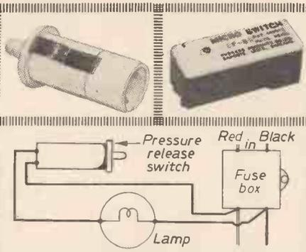
Fig. 4 (Left).—Cupboard switching; (A) using A55; (B) using micro switch. Fig. 5 (Top right).—A55 and micro switch. Fig. 6 (Bottom right).—Cupboard switch circuit wiring.
