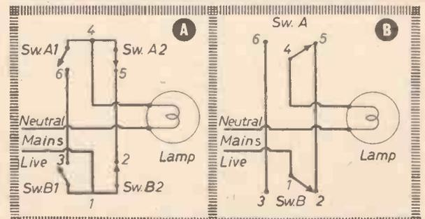
Fig. 3.—(A) Wiring of button switches for staircase lighting and (B) conventional two-way switching.
