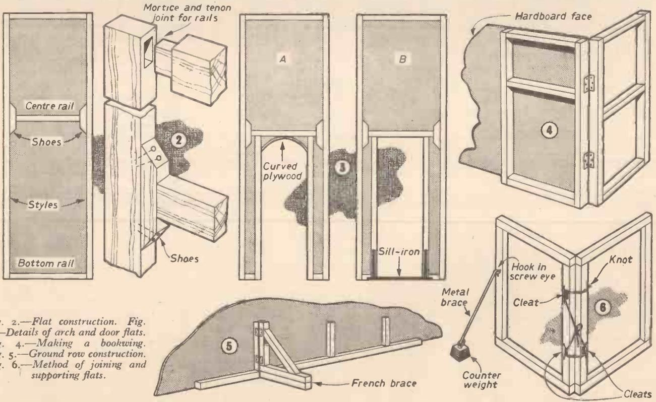
Fig. 2.—Flat construction. Fig. 3.—Details of arch and door flats. Fig. 4.—Making a bookwing. Fig. 5.—Ground row construction. Fig. 6.—Method of joining and supporting flats.
