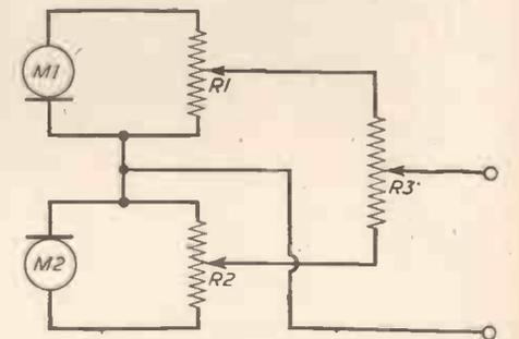
Fig. 6.—A more elaborate mixing circuit.
