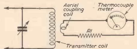
Fig. 3.—Measuring radio frequency power developed.
