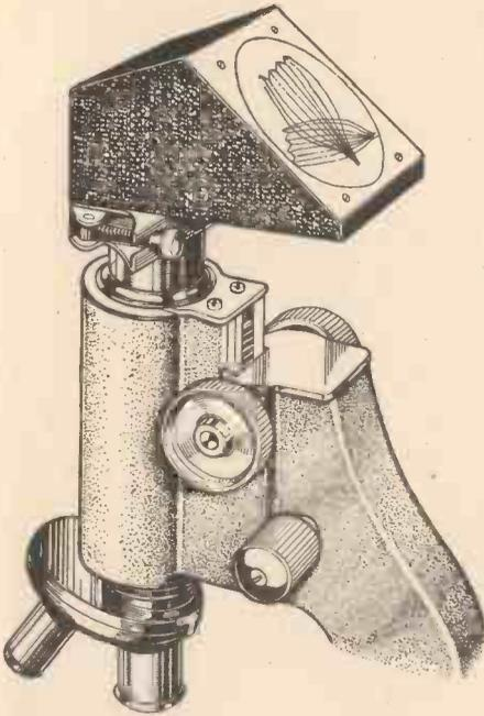
Fig. 1.—A projection head on a microscope.
