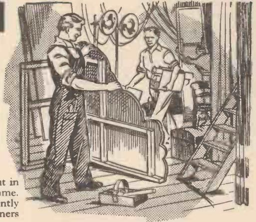
THE two main requirements of good scenery are that it should be light in weight and strong. It should also, where possible, stack compactly when in storage. The scenic flat made of a canvas-covered timber frame has come to be the accepted basic scenic unit. It is both strong and light and can be repainted over and over again. The scene visualised in Fig. 1 is made up of scenery described in this article.
