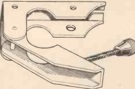
Fig. 3.—The type of clip most suitable for attachment to the draw tube.
