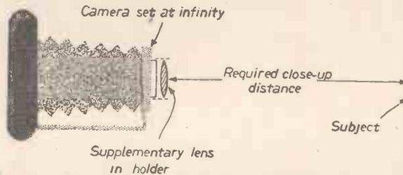
Fig. 2.—Focal length of a supplementary.
