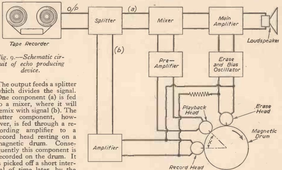
Fig. 9.—Schematic circuit of echo producing device.
