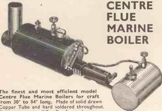
The finest and most efficient model Centre Flue Marine Boilers for craft from 30" to 84" long. Made of solid drawn Copper Tube and hard soldered throughout. Fittings comprise "Pop" safety valve, screw-down fine-adjustment regulator, Pressure gauge and syphon, Water gauge and check valve for feed pump.
