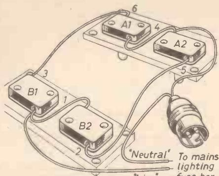
Fig. 2.—Wiring of button switches.
