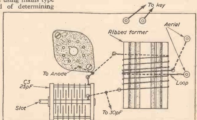
Fig. 4.—Mains transmitter layout.
