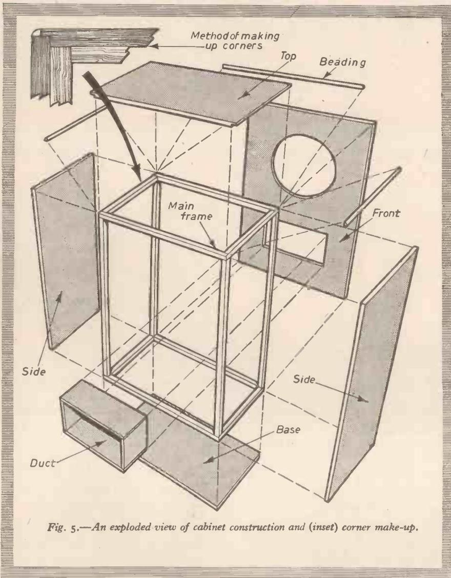
Fig. 5.—An exploded view of cabinet construction and (inset) corner make-up.
