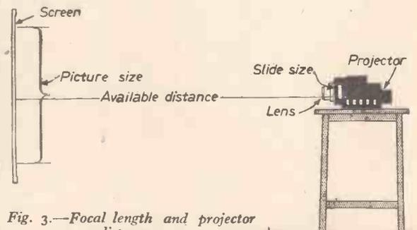
Fig. 3.—Focal length and projector distance.
