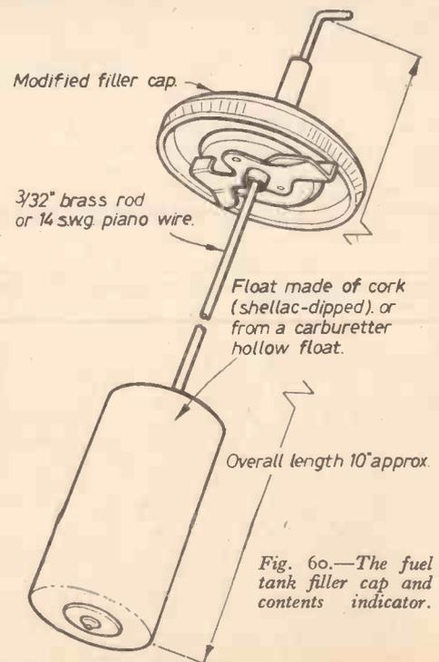
Fig. 60.—The fuel tank filler cap and contents indicator.
