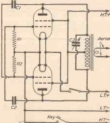
Fig. 1.—Two-valve battery operated transmitter.
