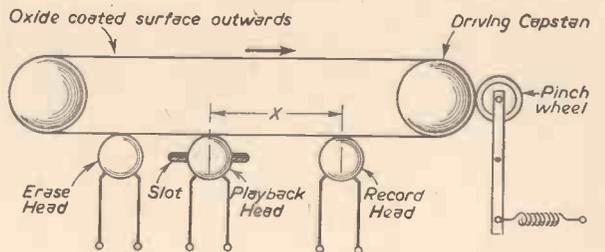
Fig. 10.—Magnetic drum replaced by endless loop of tape.
