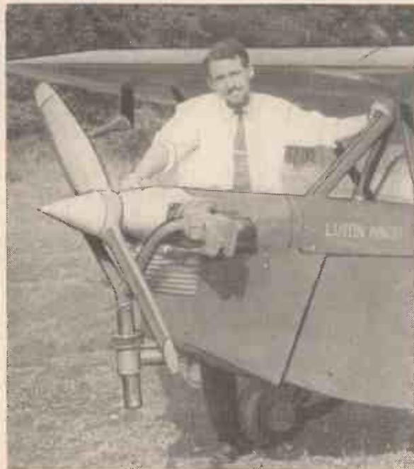
Fig. 56.—The Aeronca J.A.P. engine fitted to an amateur-built Luton Minor.
