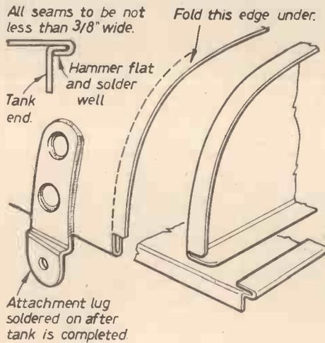
Fig. 59.—Details of the petrol tank construction.
