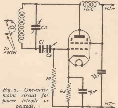
Fig. 2.—One-valve mains circuit for power tetrode or pentode.
