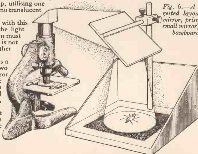
Fig. 6.—A suggested layout of mirror, prism (or small mirror) and baseboard.
