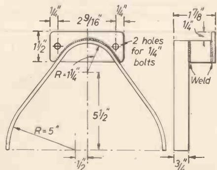
Fig. 28.—Chain guard detail for Clinton engine. Make from 1/8 in. thick or 10 gauge M/S plate. The chain guard for the J.A.P. engine is similar.
