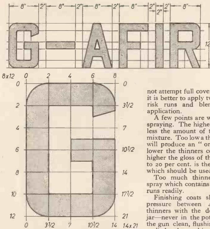
Fig. 79.—The thickness of the strokes in the letters is equal to the width of the spaces between the letters. The dash is made the full width of one letter as shown.
