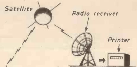
Fig. 2.—How an "orbital post office" would work.
