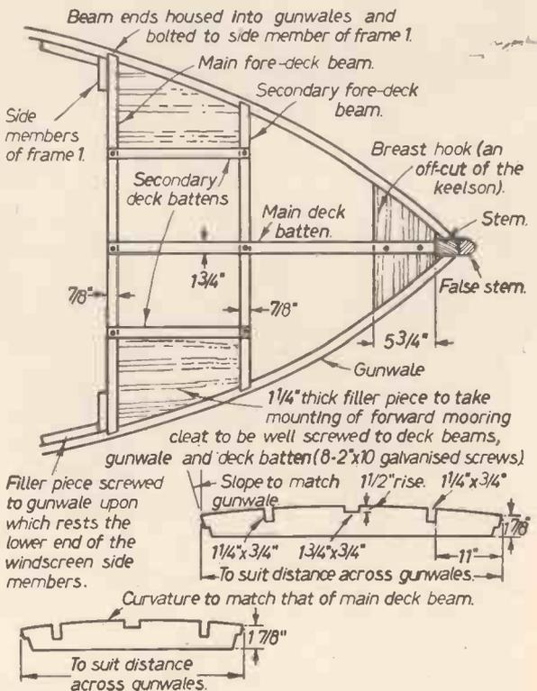
Fig. 22 (Right).—Details of the fore deck.
