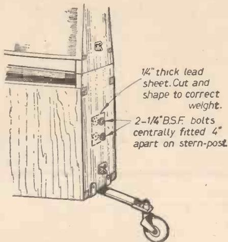
Fig. 84.—Fixing the lead ballast.
