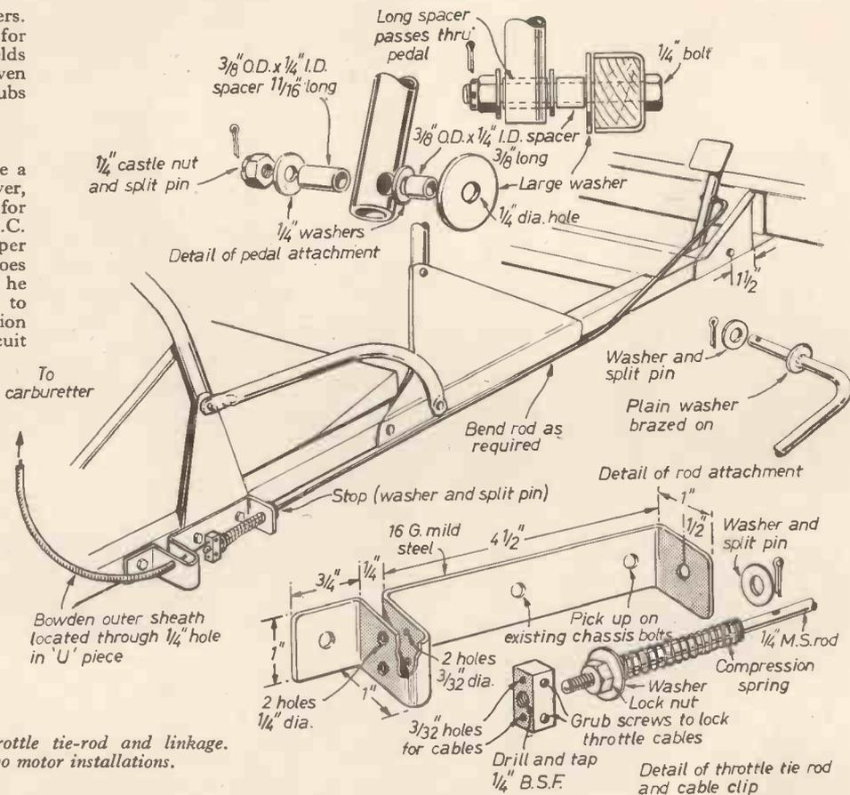
Fig. 29.—The assembly of the throttle tie-rod and linkage. This may be used for one or two motor installations.
