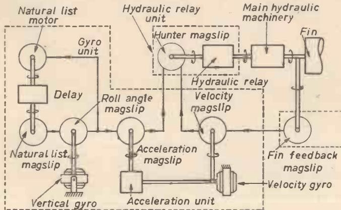
Fig. 8.—Schematic diagram of the control and hydraulic system.
