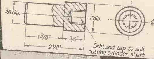
Fig. 7.—Cutting cylinder drive assembly.
