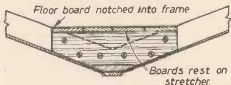
Fig. 19 (Left).—Section of the cabin floor.
