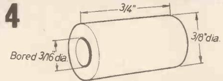
Fig. 4.—Engine support packers (Bt. M.S.)
