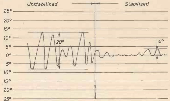
Fig. 10.—Reduction in rolling when using stabilisers.
