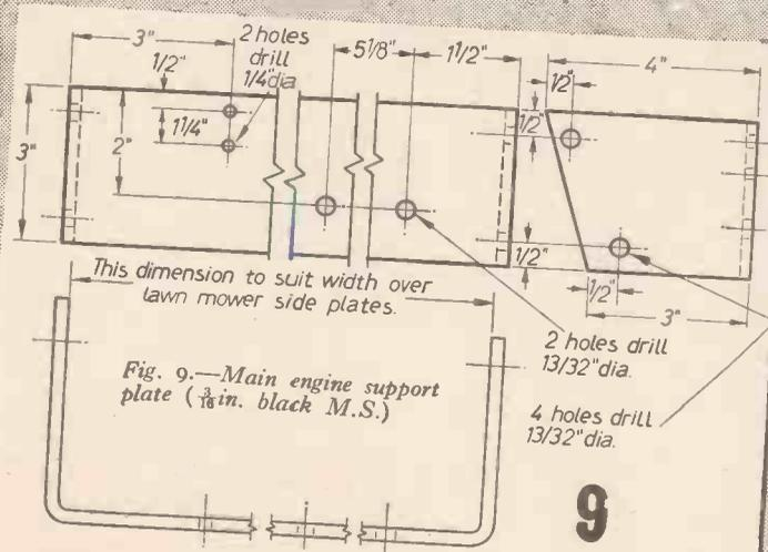
Fig. 9.—Main engine support plate (1/8 in. black M.S.)
