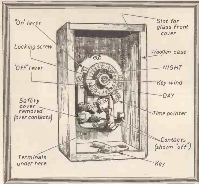
Fig. 40.—A useful reconditioned time switch.
