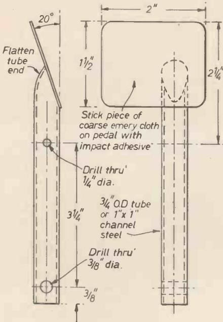
Fig. 25.—Detail of the foot pedals. Two are required, handed.
