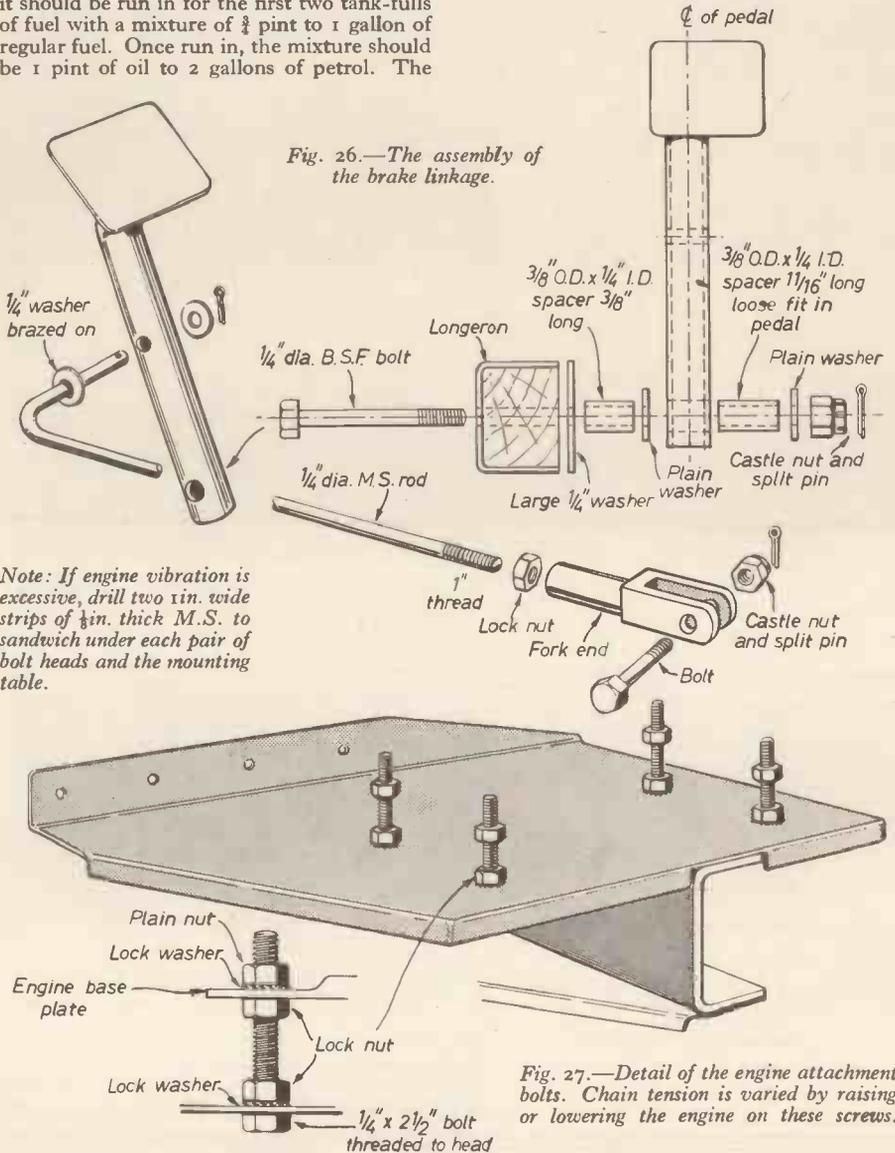
Note: If engine vibration is excessive, drill two tin. wide strips of 1/8 in. thick M.S. to sandwich under each pair of bolt heads and the mounting table.
