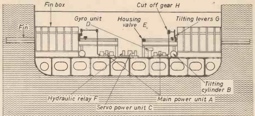
Fig. 7.—How the stabilisers are located in the ship.
