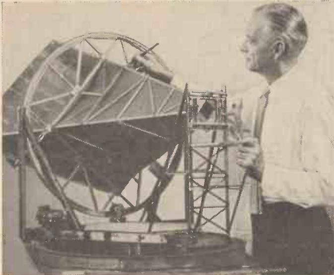
Fig. 1.—A model of a large horn antenna, to be soft in length and the aperture 20ft. × 20ft.
