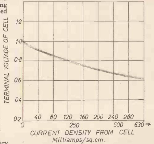
Fig. 5.—The characteristics of a single fuel cell.
