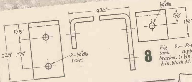
Fig. 8.—Petrol tank support bracket. (1 1/4 in. x 1/8 in. black M.S.)
