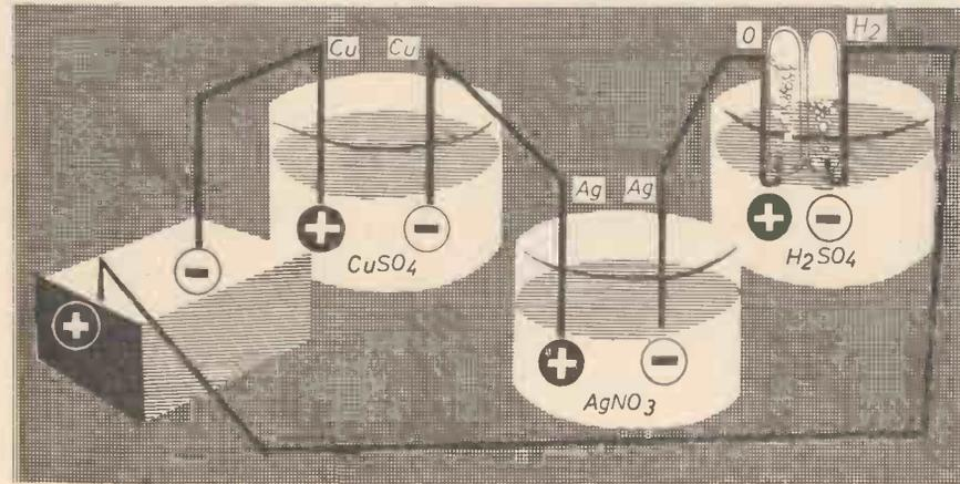
Fig. 1.—The basic principles of electrolysis.
