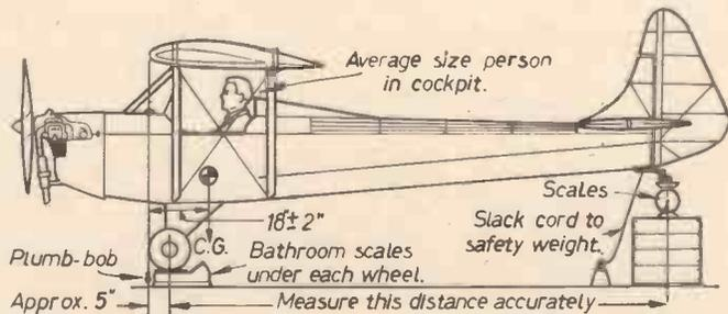
Fig. 82.—Completed aircraft set up in the rigging position on scales showing the position of the centre of gravity.
