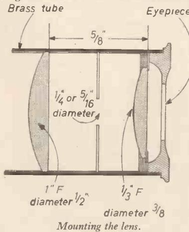
brass tube and held in place by rings of Bristol board. Midway between the lenses a stop must be placed, the hole through which can be about  $\frac{1}{8}$ in. or  $\frac{1}{16}$ in. dia. The two lenses are both plano-convex and these are mounted with the domed side towards the O.G., flat sides towards the observer's eye. They can be obtained from Broadhurst Clarkson and Co. Ltd., of 63 Farringdon Road, London, E.C.1.
