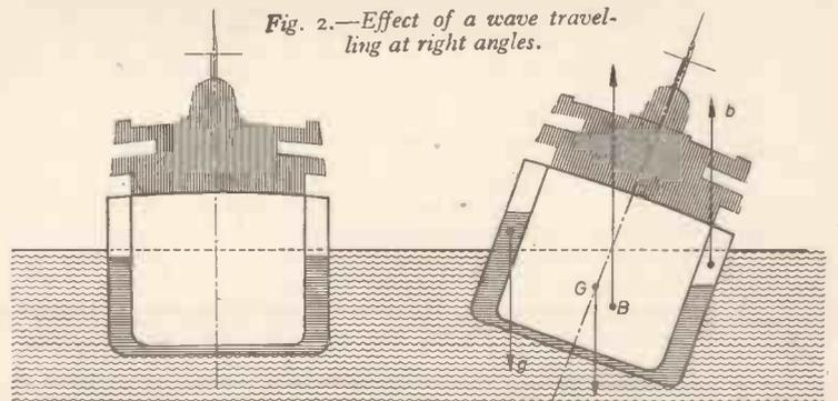
Fig. 3.—Water tank anti-rolling device.
