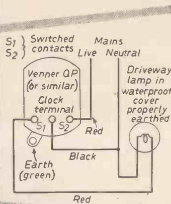
Fig. 39.—Wiring for a drive-way light.
