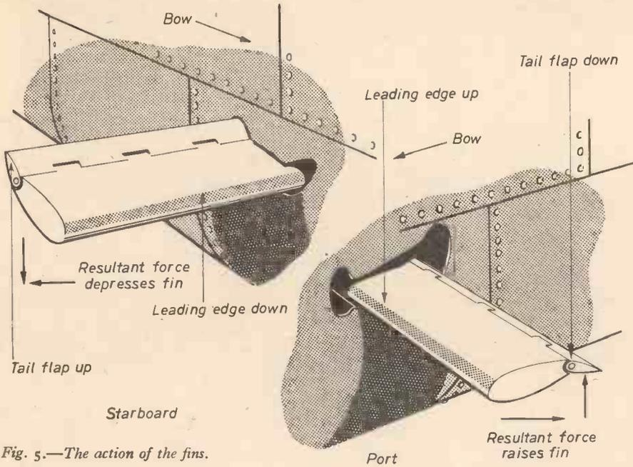
Fig. 5.—The action of the fins.
