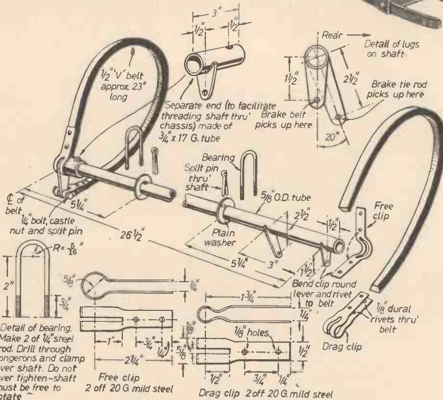
Fig. 24.—Brake torque shaft detail. Note that the shaft is inserted through the chassis holes from the left-hand side. On the right is shown the assembly of the brake pulley to the 72-tooth drive sprocket; concave side of pulley facing in towards chassis centre-line.
