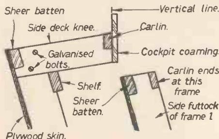
Fig. 20 (Left).—Longitudinal members attached to side deck knees, and Fig. 21.—Carlin ends at frame 1.
