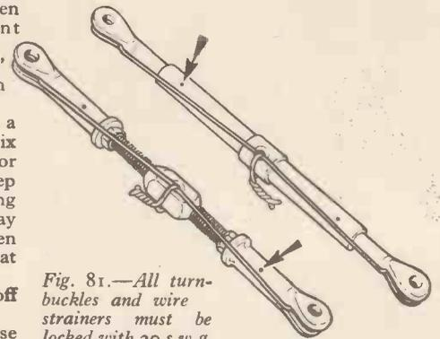
Fig. 81.—All turnbuckles and wire strainers must be locked with 20 s.w.g. soft iron wire as shown. The arrows indicate the "safety" holes. It must not be possible to insert a pin through these, otherwise insufficient length of thread is being subjected to the tension load.
