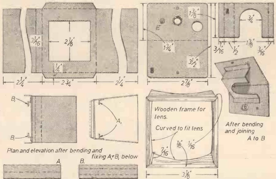
Fig. 5.—Slide and diffuser holder, lampholder and switch plate and lens securing frame.
