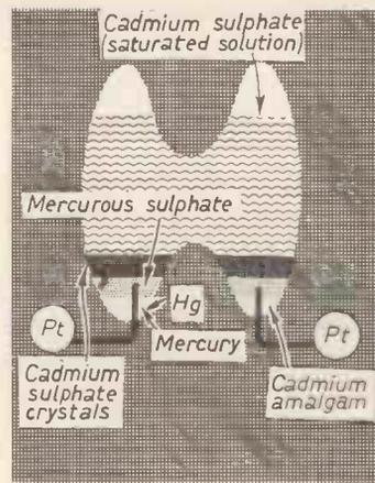
Fig. 3.—The cadmium cell.
