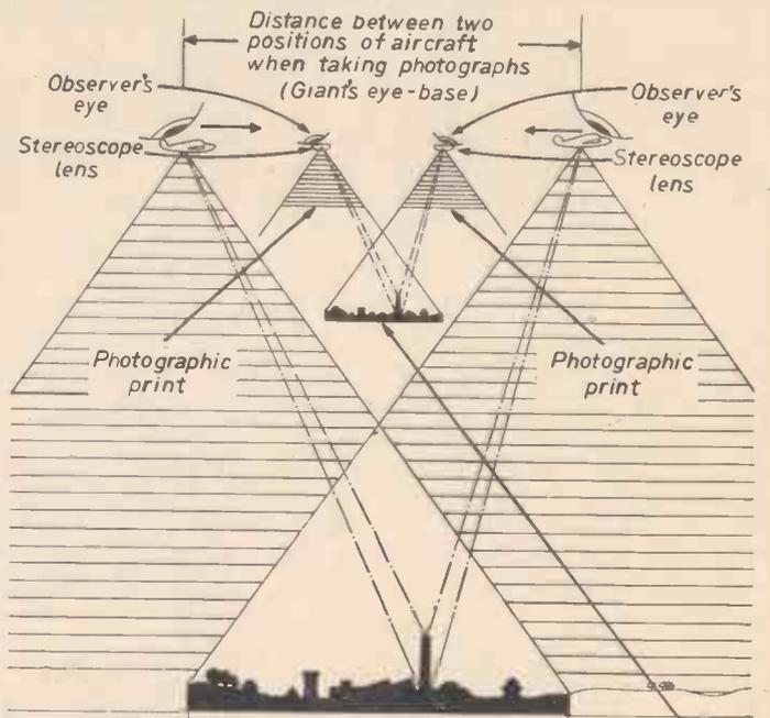
Fig. 4.—Diagram illustrating the three-dimensional model produced by examination of a pair of air photographs with a stereoscope. Area common to both photographs as it would appear in nature to a giant with eyes as far apart as the distance between two successive positions of the aircraft (air base). Space model in mind of observer
