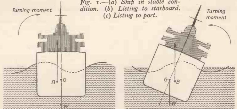
Fig. 2.—Effect of a wave travelling at right angles.
