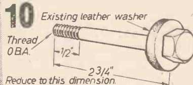
Fig. 11.—Method of securing silencer to lawn mower frame.
