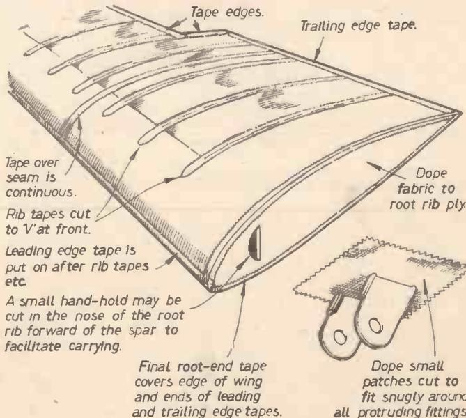
Fig. 78.—Taping operations.
