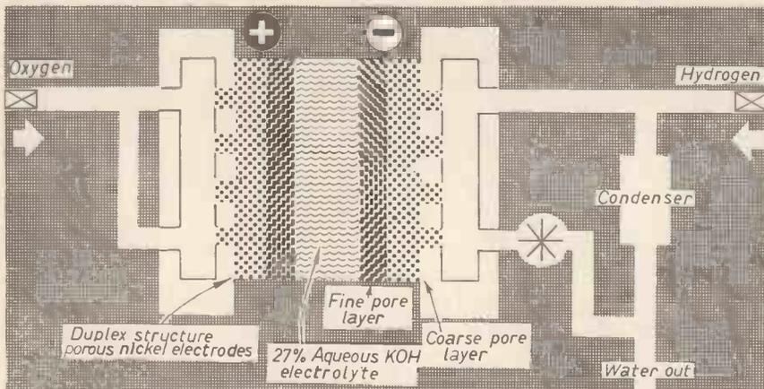
Fig. 6.—Cross section of a single cell.
