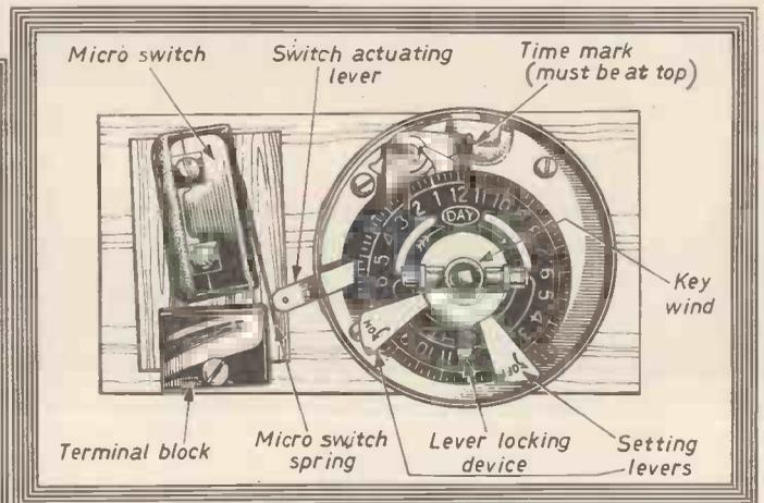
Fig. 41.—Another reconditioned timeswitch suitable for use in the home.
