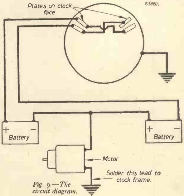
Fig. 9.—The circuit diagram.
