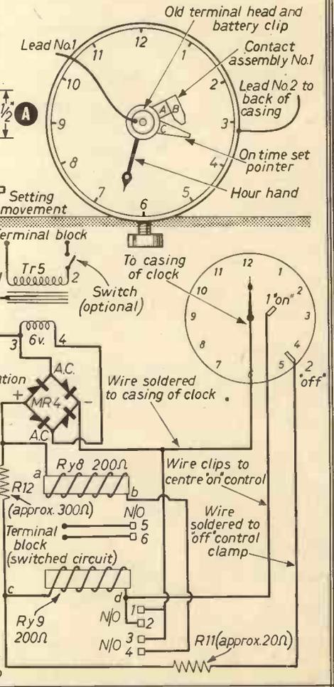
Fig. 53.—On/off time switch circuit.
