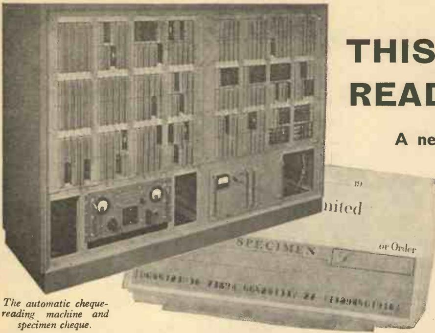
The automatic cheque-reading machine and specimen cheque.
