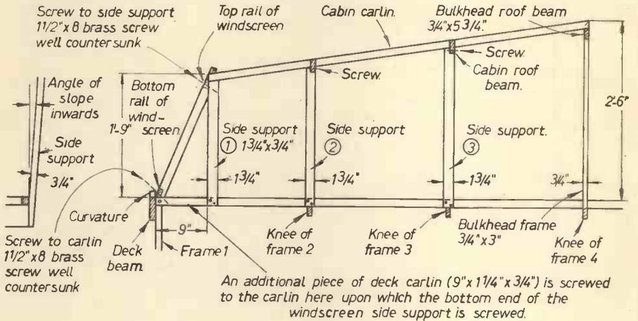
Fig. 29.—Details of cabin side structures.
