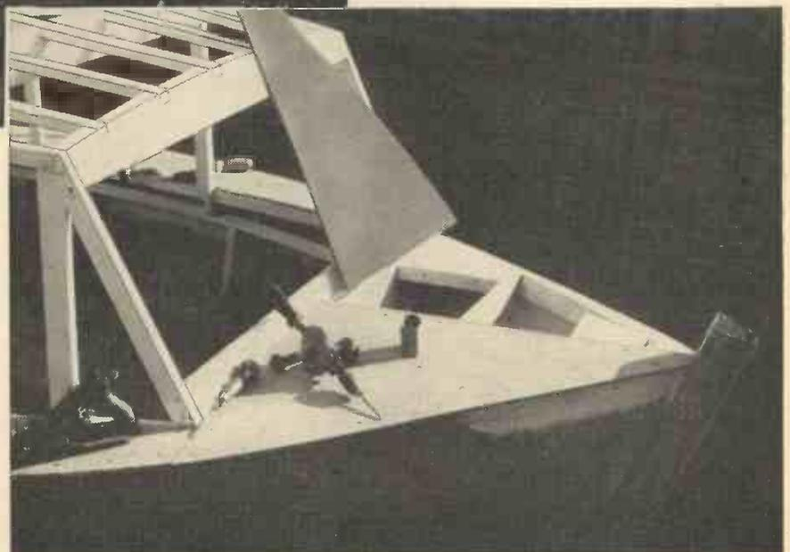
Fig. 31.—Fitting the fore-deck.
