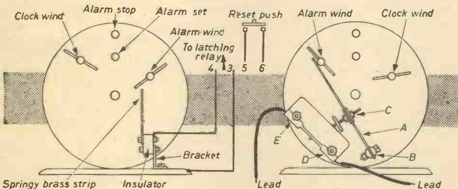
Fig. 43.—Simple alarm clock time switch.
