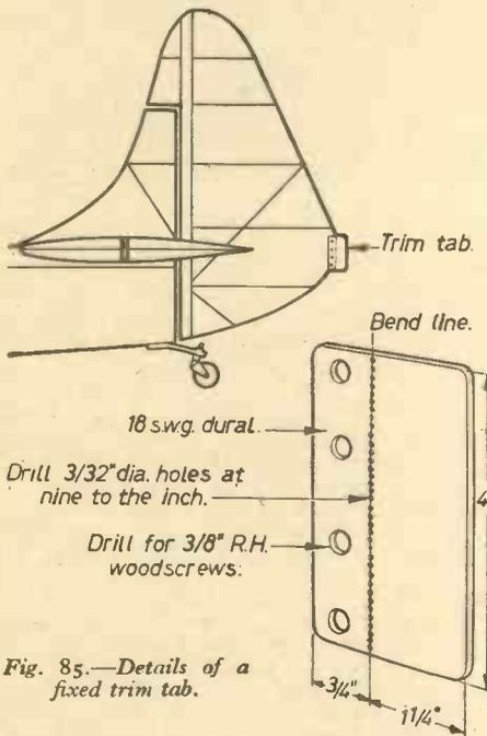
Fig. 85.—Details of a fixed trim tab.
