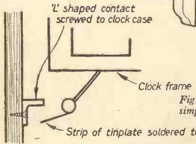
Fig. 8 (Left)—The simple trigger switch.
