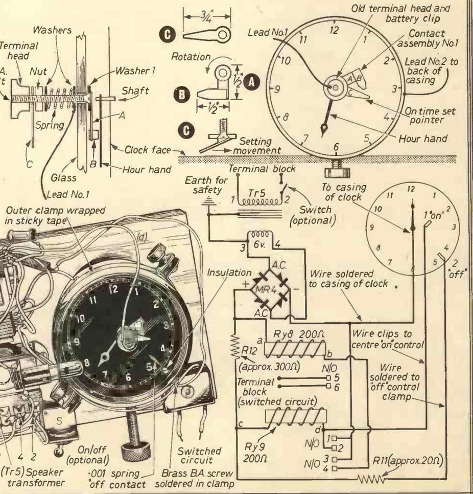
Fig. 52.—Complete layout and wiring of the on/off time switch using 14-day movement.
