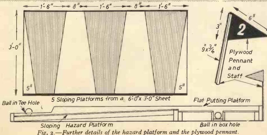
Fig. 2.—Further details of the hazard platform and the plywood pennant.
