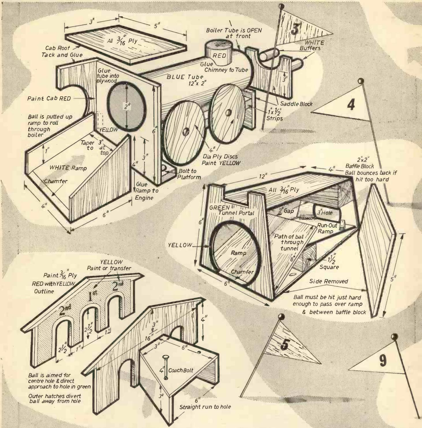
Fig. 3.—The engine hazard.
