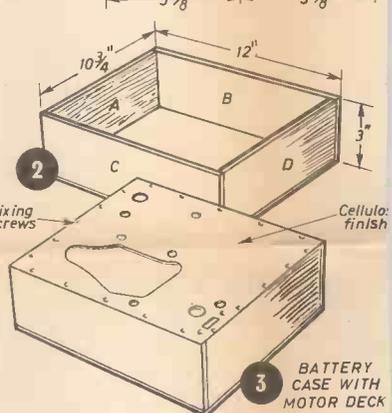
3 BATTERY CASE WITH MOTOR DECK
