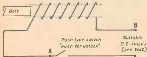
Fig. 67.—Circuit for single coil automatic door bolt.
