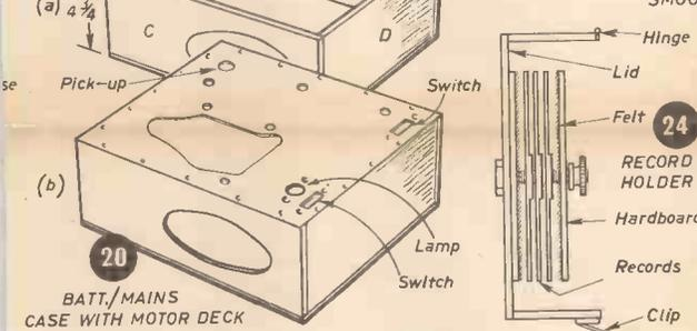
20 BATT./MAINS CASE WITH MOTOR DECK
