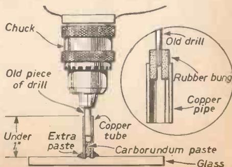
the cut. Drilling is shown in progress in Fig. 13.
