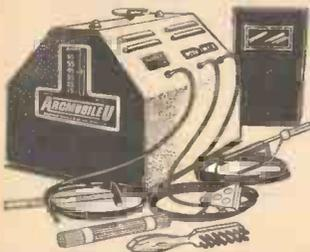
£17.10.0 (inc. delivery). Cash with order. A complete self-contained Arc Welder using standard flux-coated electrodes of 14g. and 16g. 210/250 V. A.C. Mains consumption 13 Amps. Welds sheet metal down to 22g. and steel and iron section up to 3/16in. thick in a single run. Heavier sections can be welded by multiple runs (building up). Infinitely variable welding current by hand-wheel. Maximum welding current 65 Amps. Minimum 15 Amps. Weight 85 lbs. Dimensions: 11in. high, 12in. wide, 13in. long.
