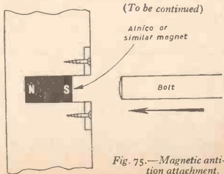
Fig. 75.—Magnetic anti-vibration attachment.
