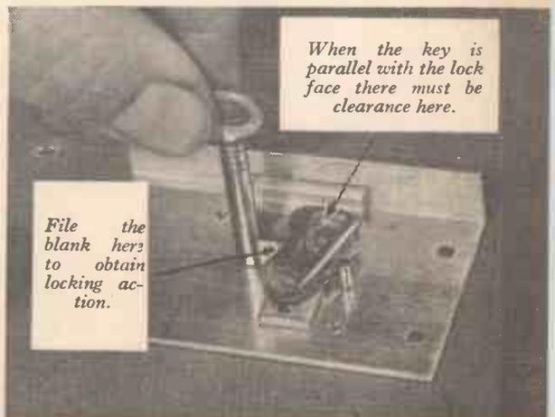
When the key is parallel with the lock face there must be clearance here.
