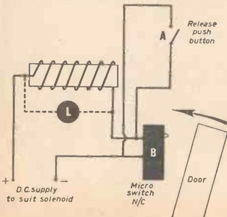
Fig. 73.—(Left) Circuit for automatic locking as door is closed (single solenoid systems).
