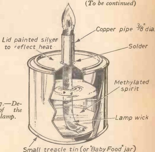
Fig. 17.—Details of the spirit lamp.
