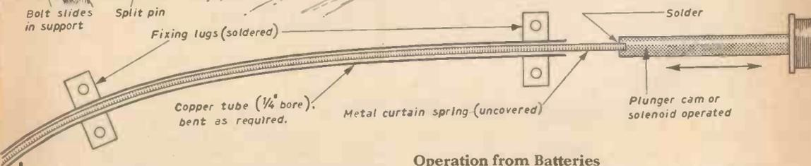
Fig. 70.—(Below) Remotely situated bolt.
