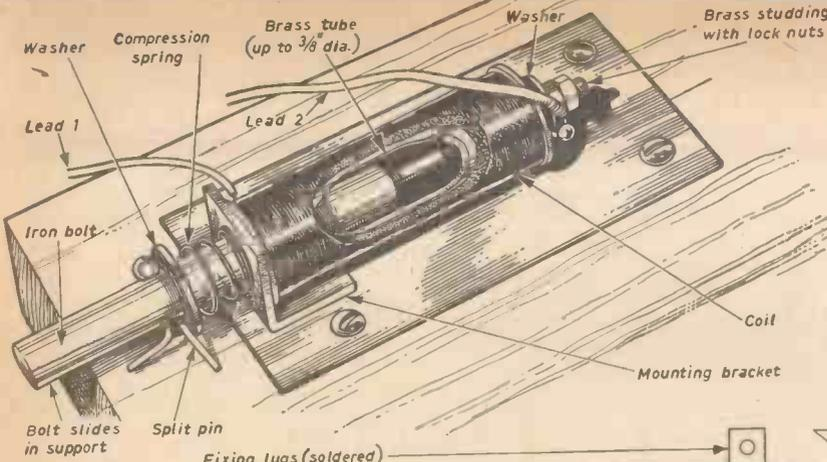
Fig. 69.—(Left) Auto-door bolt using direction indicator coil.
