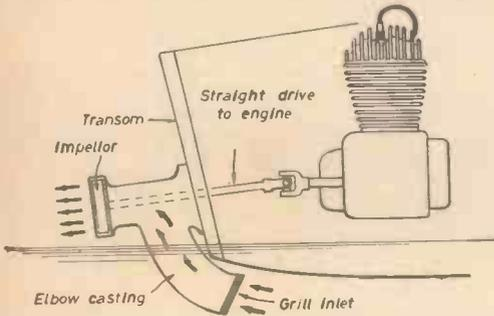
principle illustrated above. Water is drawn from beneath the engine and thrust out at an angle of 90 deg. I have a proprietary engine working on this principle. A similar type is available using a horizontal impeller and a vertical drive shaft, so that using this type the engine could be mounted immediately above as shown in your sketch in the June issue.—Sgt. CRIMMINS (Famagusta).
