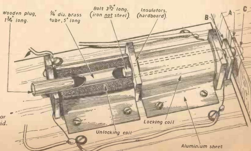
Fig. 71.—Electromagnetic door bolt, using double wound solenoid.
