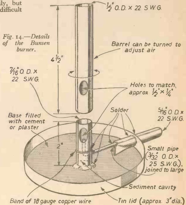
Fig. 14.—Details of the Bunsen burner.
