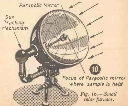
Fig. 10.—Small solar furnace.
