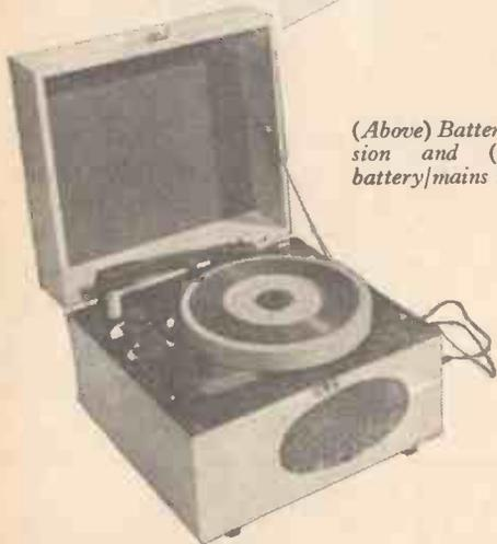
**T**WO prototypes were constructed, one to work off a 12V. car battery or, after modification, 6V., and another to work off a car battery or the mains. There is no conventional chassis, and the motor deck is the output transistor heat sink, so amplifier and motor box are made up first and fitted with the correctly drilled motor deck, followed by
