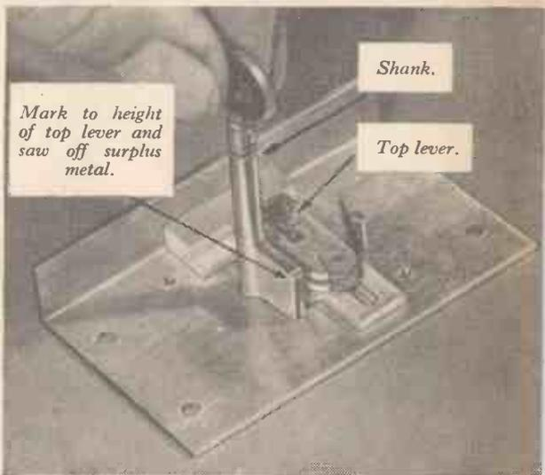
Mark to height of top lever and saw off surplus metal.
