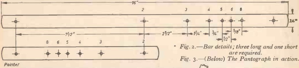
• Fig. 2.—Bar details; three long and one short are required.
