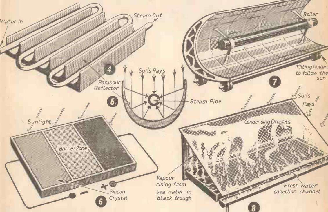
Fig. 4.—Solar collector for steam generation. Fig. 5.—Details of operation of reflectors. Fig. 6.—A solar battery. Fig. 7.—Giant solar powered steam generator. Fig. 8.—Solar still to make fresh water from salt water.
