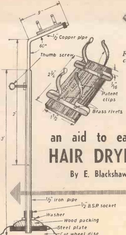
Fig. 1.—Details of the base and main upright member.
