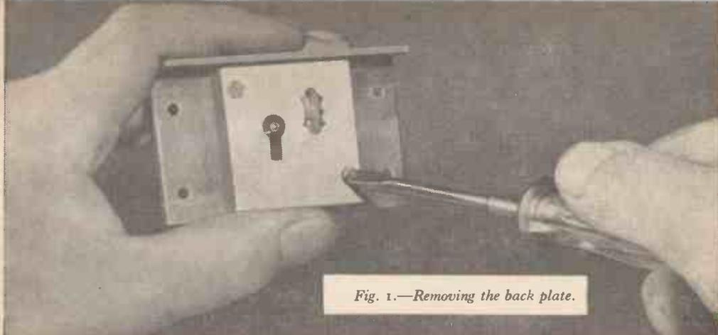
Fig. 1.—Removing the back plate.
