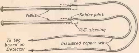
Fig. 8.—Details of the test prods.
