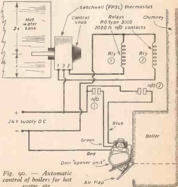
Fig. 90. — Automatic control of boilers for hot water, etc.
