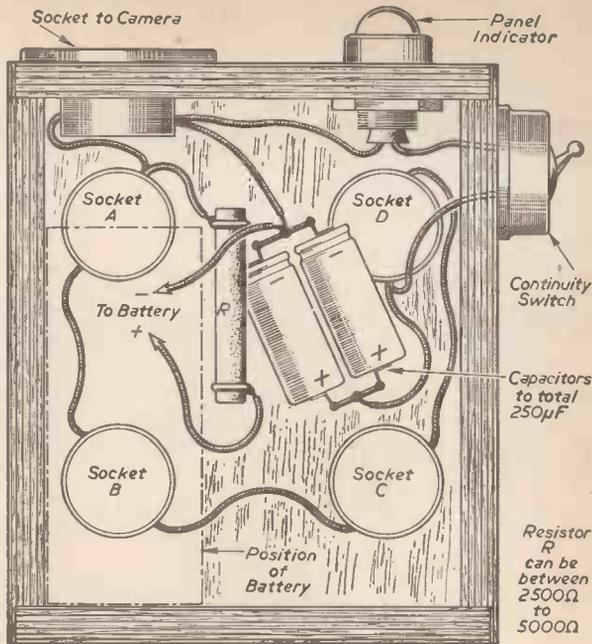
Fig. 3.—Point to point wiring diagram.
