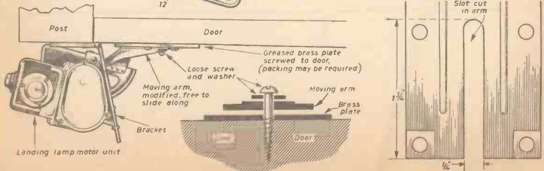
Fig. 83.—(Below) Top view as mounted on door post and details of modification to moving arm.
