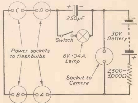
Fig. 2.—The theoretical circuit.
