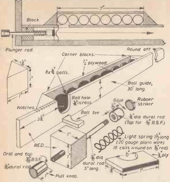
Fig. 2.—The striker mechanism and ball magazine.
