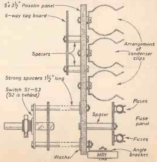
Fig. 5. (Right)—End view of paxolin panel showing method of mounting components.
