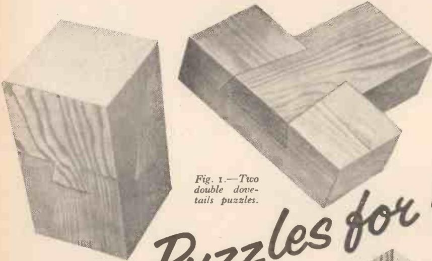
Fig. 1.—Two double dovetail puzzles.
