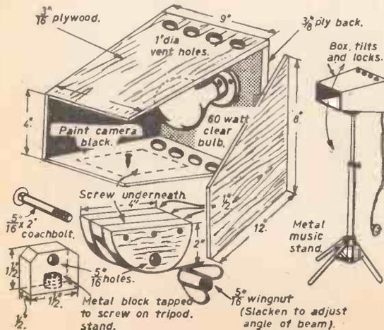
Fig. 2. (Left)—Dimensions of lamp housing of the beam projector.
