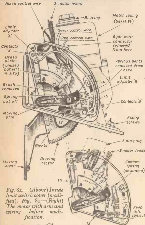
Fig. 82.—(Above) Inside limit switch cover (modified). Fig. 81—(Right) The motor with arm and wiring before modification.
