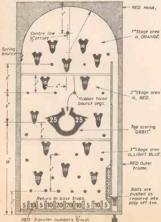
trap at the bottom end of the table. The trap is made entirely of  $\frac{1}{4}$  in. ply with a back measuring 1 in.  $\times$  16  $\frac{3}{4}$  in. and the legs from pieces 1 in.  $\times$  2 in. End divisions are spaced at 1  $\frac{1}{8}$  in. but those between are all at 1  $\frac{1}{8}$  in. centres. Paint the trap yellow (Fig. 7).
