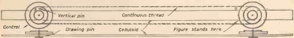
Fig. 5.—Control for three dimensional figures.
