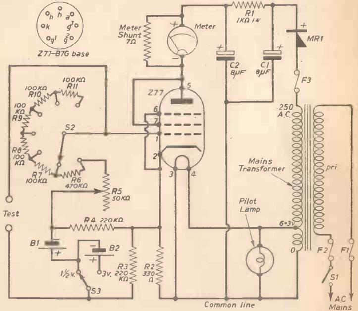
Fig. 1.—Theoretical circuit and valve base details.
