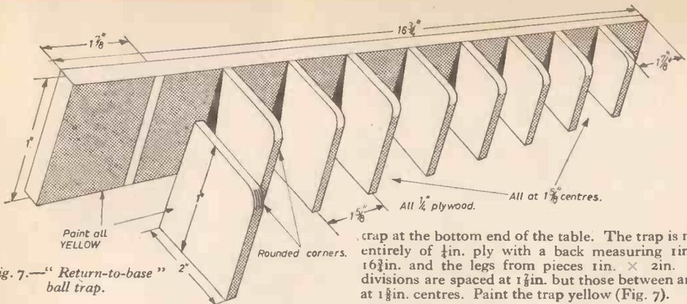
Fig. 7.—"Return-to-base" ball trap.
