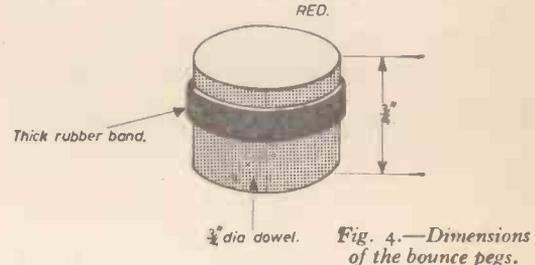
Fig. 4.—Dimensions of the bounce pegs.
