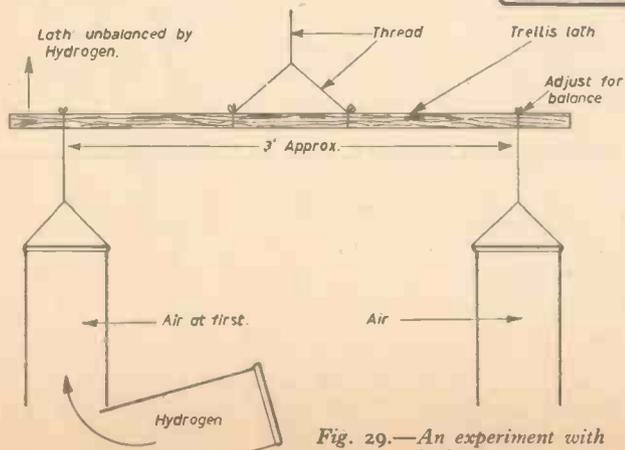
Fig. 29.—An experiment with hydrogen.
