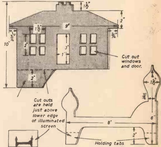
Fig. 8.—Dimensions for the house in the wood.
