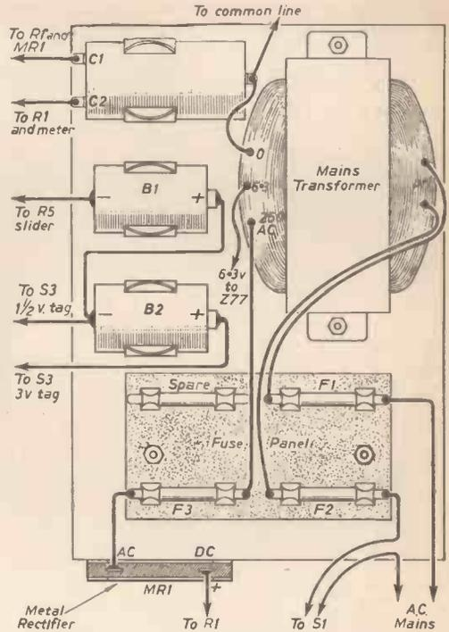
Fig. 4. (Above right)—Point to point wiring of the power pack.
