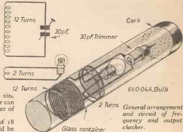
To put another transmitter on frequency, hold the tube near the transmitter coil, and tune the transmitter until the bulb lights, the tube always being kept as far from the transmitter coil as possible.
