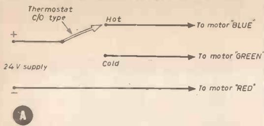
Fig. 89.—(Left) Greenhouse automatic ventilation. (A) Circuit where thermostat will take 2A. D.C. (B) Circuit where thermostat will not pass 2A. D.C. (C) Circuit using two adjustable thermostats.
