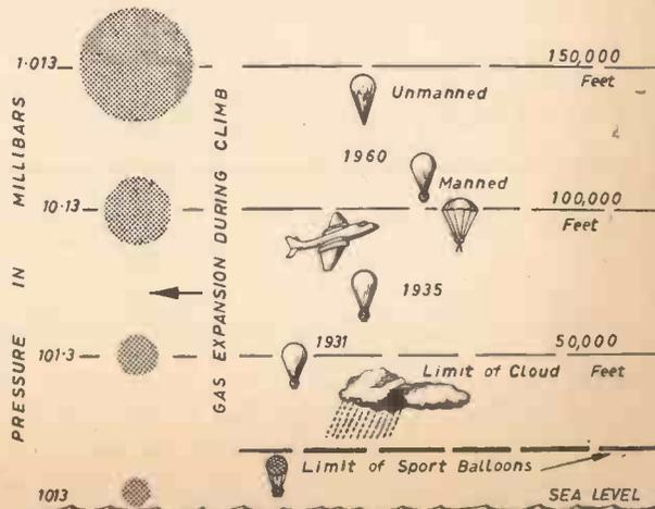
Fig. 2.—Demonstrating the decrease in atmospheric pressure with heights.
