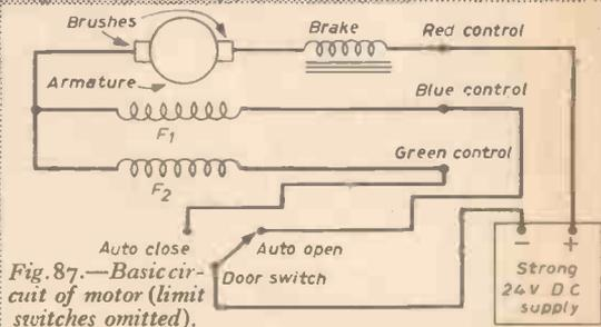
Fig. 87.—Basic circuit of motor (limit switches omitted).
