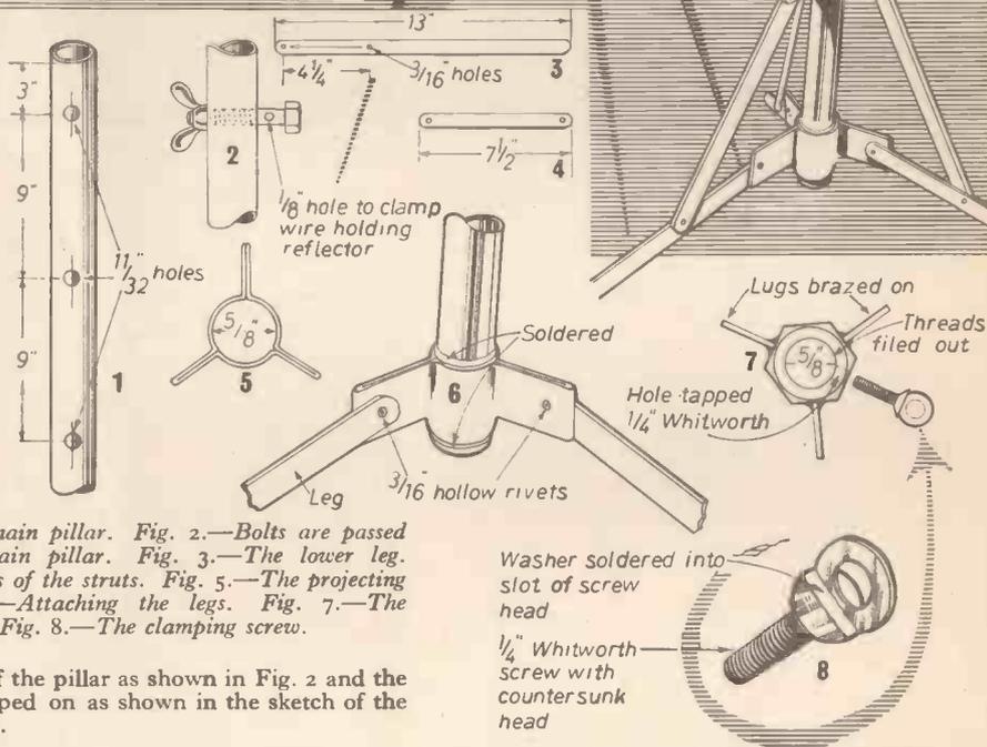
Fig. 1.—The main pillar. Fig. 2.—Bolts are passed through the main pillar. Fig. 3.—The lower leg. Fig. 4.—Details of the struts. Fig. 5.—The projecting lugs. Fig. 6.—Attaching the legs. Fig. 7.—The clamping ring. Fig. 8.—The clamping screw.
