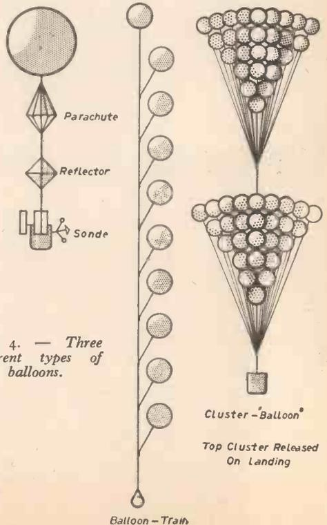
Fig. 4. — Three different types of balloons.
