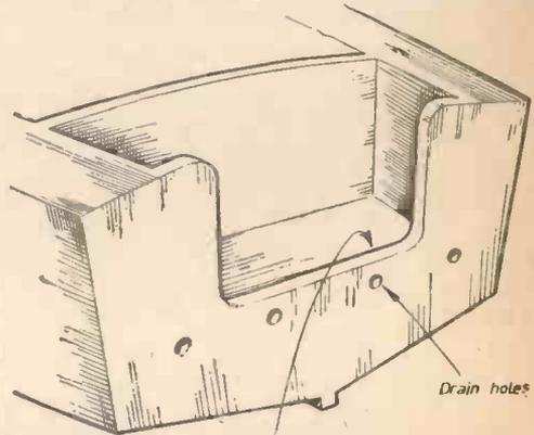
Floor of well low enough to provide enough space for clamps of engine on transom.
