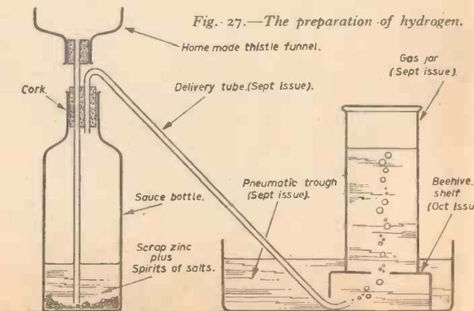
Fig. 27.—The preparation of hydrogen.
