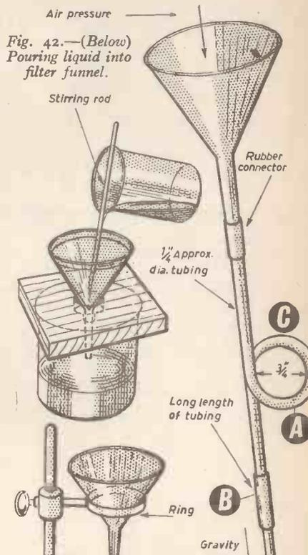
Fig. 42.—(Below) Pouring liquid into filter funnel.
