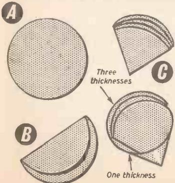
Fig. 41.—Basic filtering apparatus. A, B and C show how to fold a filter paper.
