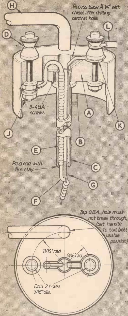
Fig. 1.—Pyrometer assembly. A—base; B—cover; C—tube; D—terminal; E—insulating beads; F—24G Nichrome wire; G—copper strip; H—handle; J—clamping nut.
