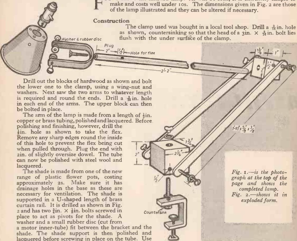
Drill out the blocks of hardwood as shown and bolt the lower one to the clamp, using a wing-nut and washers. Next saw the two arms to whatever length is required and round the ends. Drill a  $\frac{3}{8}$  in. hole in each end of the arms. The upper block can then be bolted in place.
