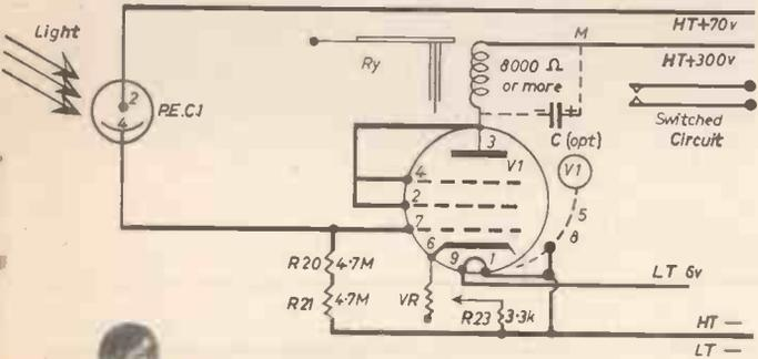
Fig. 116 (Left)—Theoretical circuit of photo electric switch unit No. 1.
