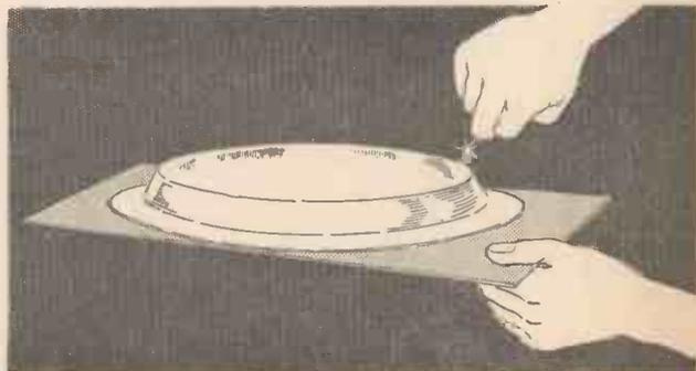
Having now described the generation and testing of a static charge, we can also proceed to experiment. Assuming you have "excited" the sheet and placed the baking tin in position, put a little pile of puffed rice or oats, or chips of elder pith on the top of the tin. On lifting the sheet the pile will disintegrate and the puffed oats will fly up into the air. I once tried a pile of dry flour and this flowed into the air in a steady stream like a snowstorm.
