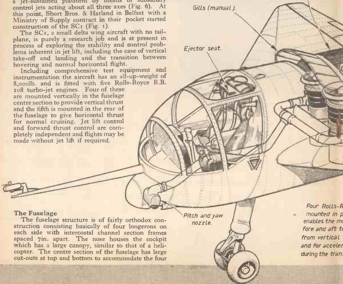
Four Rolls-Royce R.B. 108 turbo-jet engines are mounted in the fuselage centre section to provide vertical thrust and the fifth is mounted in the rear of the fuselage to give horizontal thrust for normal cruising. Jet lift control and forward thrust control are completely independent and flights may be made without jet lift if required.
