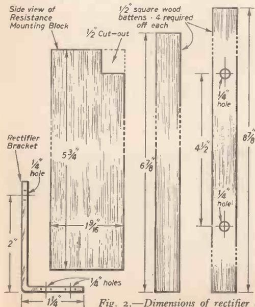
Fig. 2.—Dimensions of rectifier bracket, resistance supporting block and side woods.
