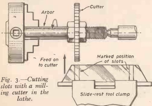
Fig. 3.—Cutting slots with a milling cutter in the lathe.
