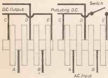
Rectifier wiring and fitting the switches.
