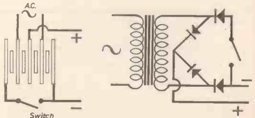
An alternative is to put a vibrator on the output of the transformer/rectifier, followed by a transformer and another rectifier wired as above. I suggest Mr. Lingwood puts a switch in the unit.—J. N. Arundale (Scarborough).
