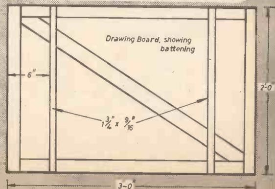
Fig. 4.—Drawing board details.
