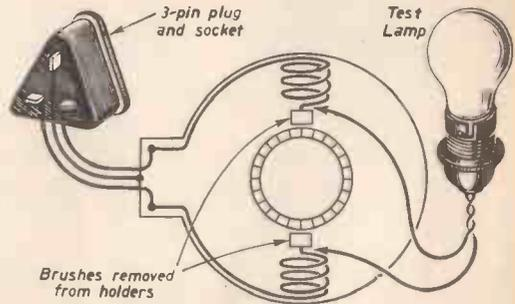
Fig. 6.—Testing a series model for short circuited armature.
