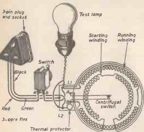
Fig. 1.—Supply testing a 1-phase induction motor.
