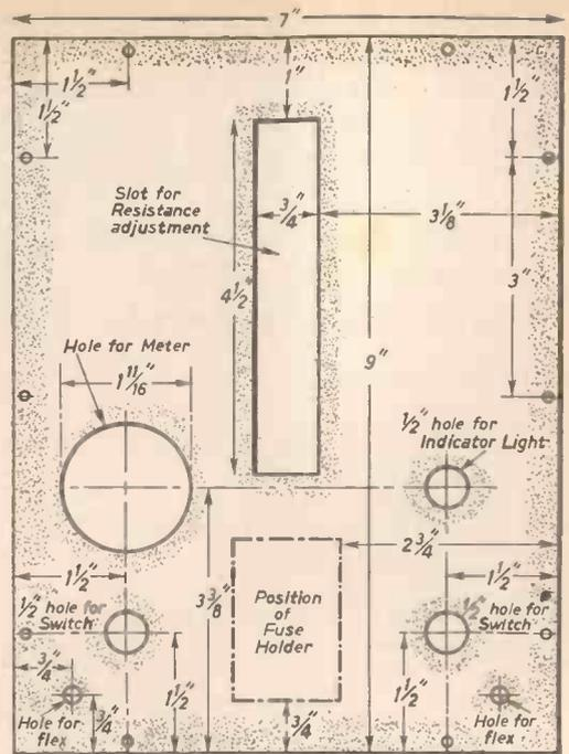
Fig. 6.—Dimensions for the paxolin panel.
