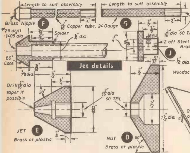
Fig. 3.—Details for making the jet.
