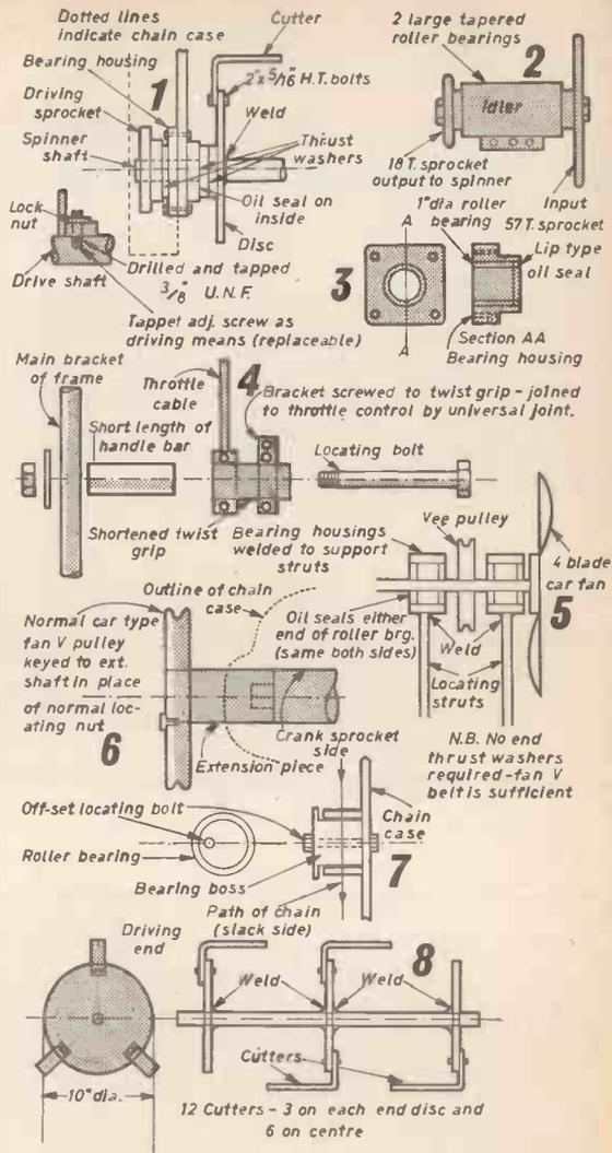
Fig. 1.—Spinner end thrust and driving device. Fig. 2.—The idler. Fig. 3.—Spinner end bearings. Fig. 4.—Throttle twist grip installation. Fig. 5.—The fan drive. Fig. 6.—Fan drive pulley from crank shaft. Fig. 7.—Spinner drive chain adjustment. Fig. 8.—Spinner discs and cutters.
