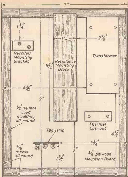
Fig. 3.—Rear mounting board showing positions of various components.
