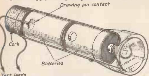
Fig. 2.—Section of a torch modified for testing.
