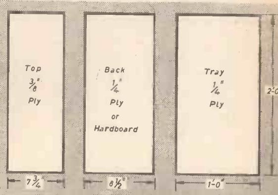
Fig. 3.—The three panels and alternative board bearer.
