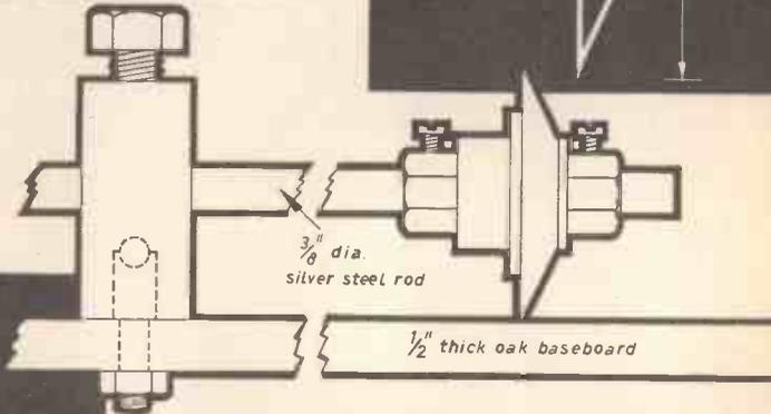
Fig. 3.—Side view of the cutter set up ready for use.
