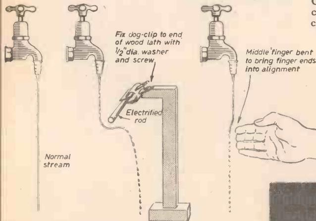
Fig. 1.—Adjusting the faucet and deflecting water.
