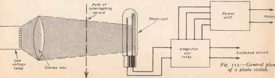
Fig. 112.—General plan of a photo switch.
