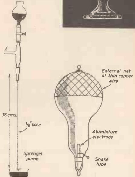
Fig. 4.—Sprengel pump and snake tube.
