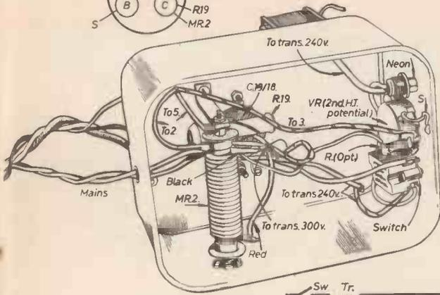
Fig. 113.—General arrangement and layout of power pack.
