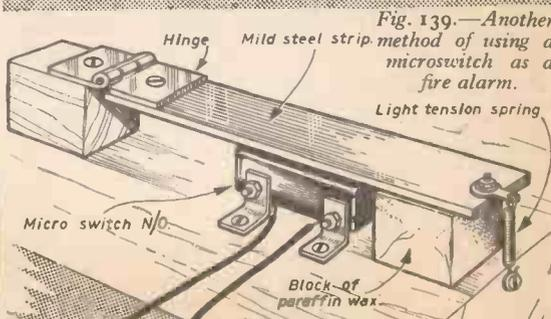
Fig. 139.—Another method of using a microswitch as a fire alarm.
