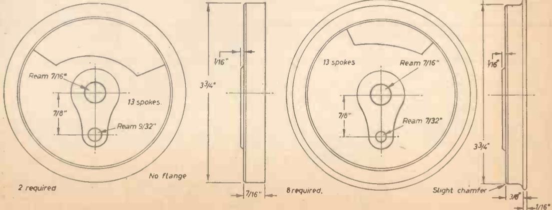
central. Clamp the jig to the wheel boss, and drill the boss  $\frac{1}{8}$  in. using the hole in the jig to guide the drill. After drilling all ten, put a  $\frac{1}{2}$  in. parallel reamer through all the holes in the flanged wheels. Those in the driving wheels (flat treads) are opened out with a  $\frac{1}{4}$  in. drill and reamed  $\frac{3}{8}$  in. Bigger crankpins are needed to take the driving stresses.
