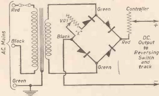
Fig. 2.—Substituting a variable resistor.
