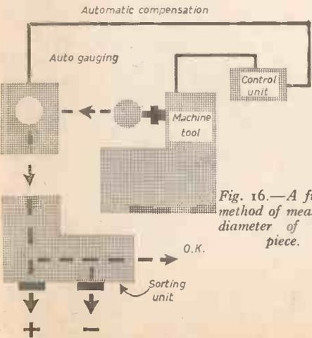
Fig. 16.—A further method of measuring diameter of work-piece.
