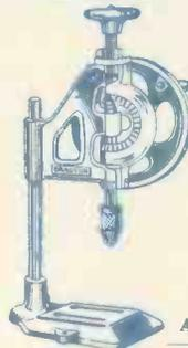
A new model, really well designed and of sturdy construction. This machine is made of cast iron—NOT light alloy. Automatic feed and in. self-centring Drill Chuck. Vertical feed 2in. Weight approximately 28lb.
