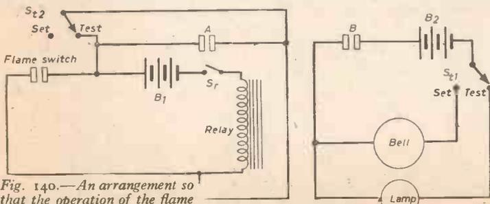
Fig. 140.—An arrangement so that the operation of the flame switch may be tested periodically to make sure all is well.
