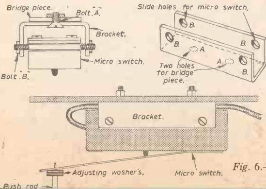
Fig. 6.—Method of mounting and operating the microswitch.
