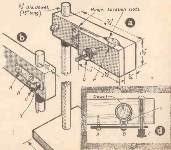
Fig. 55.—Constructional details of a burette stand
