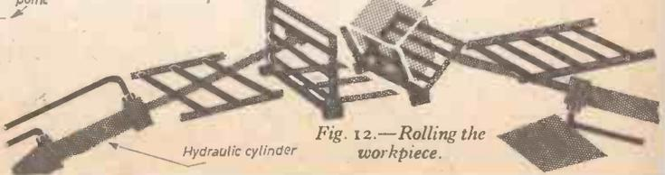
Fig. 12.—Rolling the workpiece.
