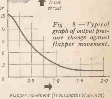
Fig. 8.—Typical graph of output pressure change against flapper movement.
