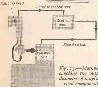
Fig. 15.—Method of checking the outside diameter of a cylindrical component.
