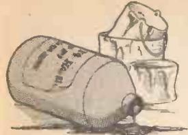
**T**HE forge described uses for its air supply a domestic vacuum cleaner and will be found very useful for those who wish to make their own small castings of brass, aluminium, etc. It can also be used for the forging of lathe tools.
