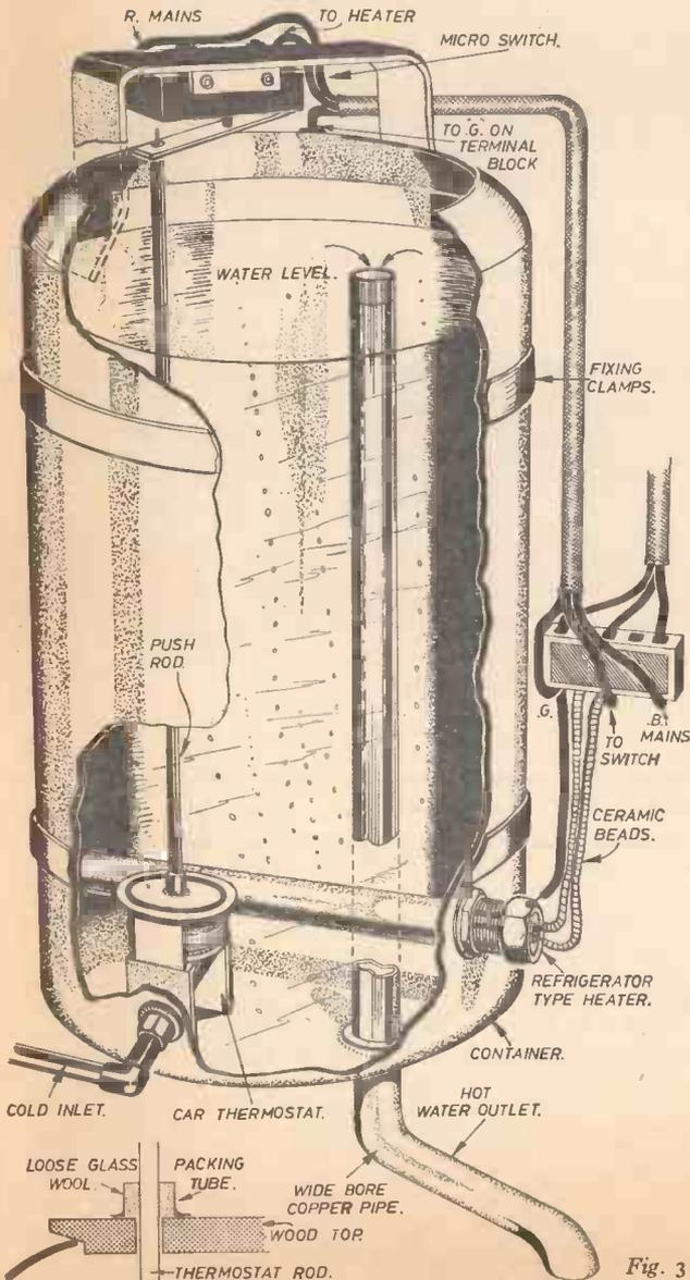
Fig. 3 (left)—Perspective view of the completed heater.
