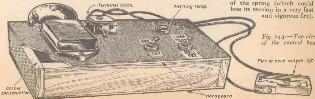
Fig. 143.—Top view of the control box.
