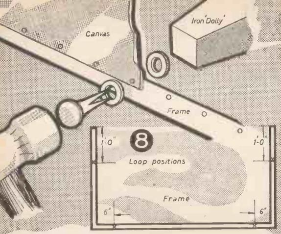
the rivet, the prongs are flattened back with a light hammer, a "dolly" at the rivet head taking the force of the blows. This operation is repeated all the way round the frame (Fig. 8).
