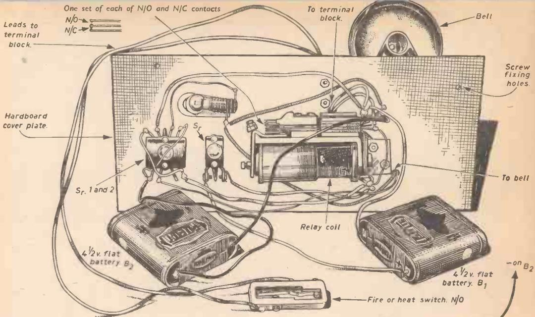
Fig. 142.—The underside of the control panel of the fire alarm showing box construction and wiring.
