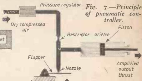
Fig. 7.—Principle of pneumatic controller.
