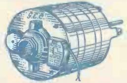
Made by the world-famous General Electric Company—a guarantee of quality. BRAND NEW. Continuous rated. For 230/250 Volts, 1440 r.p.m. A.C. Split Phase start induction Type. 2" x 1/4" Dia. Spindle. Can be operated in vertical position too. Dia. 6".
