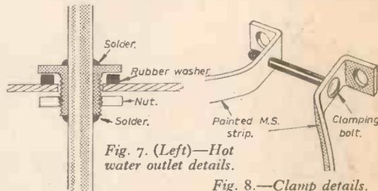
Fig. 7. (Left)—Hot water outlet details.
