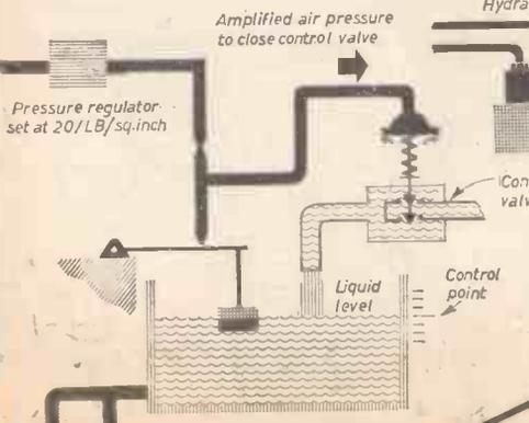
Fig. 9.—Diagrammatic arrangement of liquid level controller.
