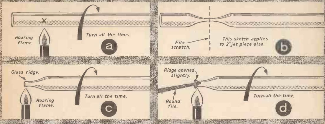
Fig. 53.—Stages in forming the lower end of a burette.
