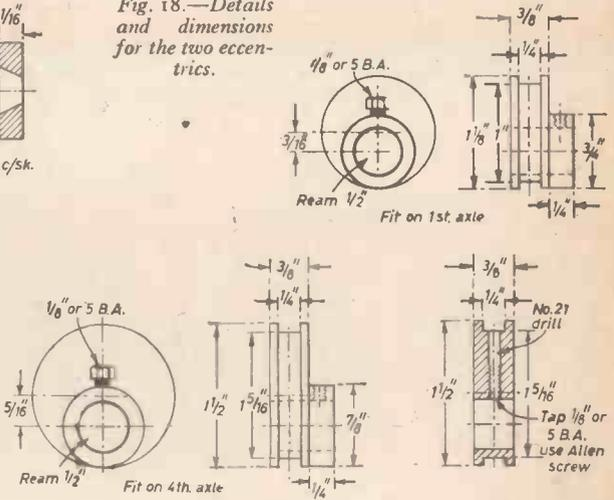
for the lubricator drive is turned in exactly the same way, but from  $1\frac{1}{2}$  in. round steel, to the dimensions given in Fig. 18 (top).
