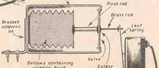
Fig. 138.—How a discarded, but working, automobile thermostat may be used as a fire alarm when coupled to a microswitch.
