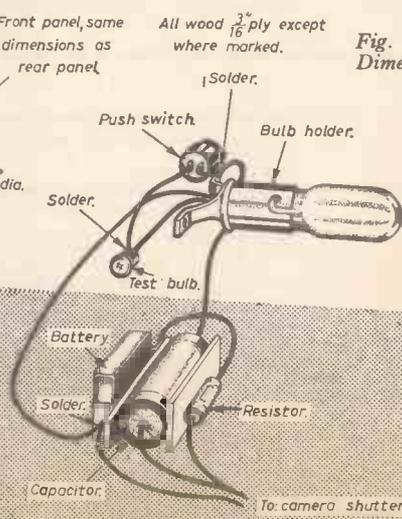
Fig. 3.—How the components are wired.
