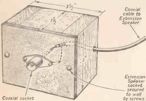
Fig. 155.—A very simple form of extension speaker socket fitted in a box for screwing to the wall.
