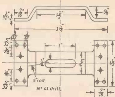
side. To cut the slot, first drill a few 3/32 in. holes along the centre-line, run them into a slot with a round file, and finish to size with a half-round file. A piece of 1/4 in. round steel should slide easily from one end to the other.
