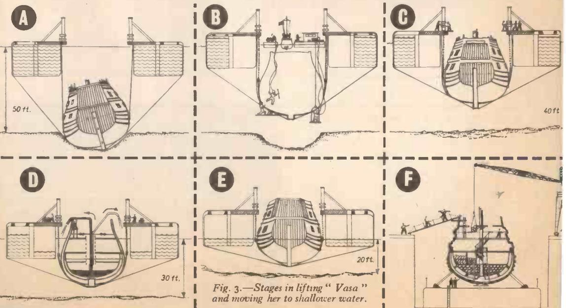
Fig. 3.—Stages in lifting "*Vasa*" and moving her to shallower water.
