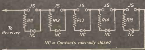
Fig. 162.—An improved series system, which requires some knowledge of radio as another transformer is required in the receiver for perfect operation.
