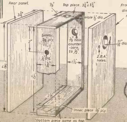
Fig. 2.—(Extreme left) Dimensions for the casing.
