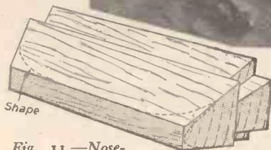
Fig. 11.—Nose-block details.
