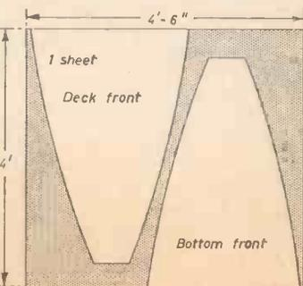
Fig. 6 (Left).—Cutting diagram for the three main sheets of 3/8 in. marine plywood.
