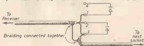
Fig. 161.—A special form of wiring for a series extension system as in Fig. 160.
