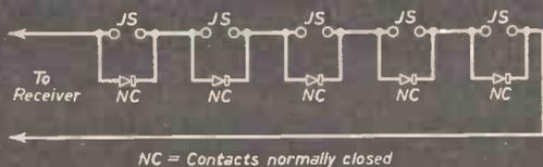
Fig. 160.—A simple series speaker system using normally closed jack sockets.
