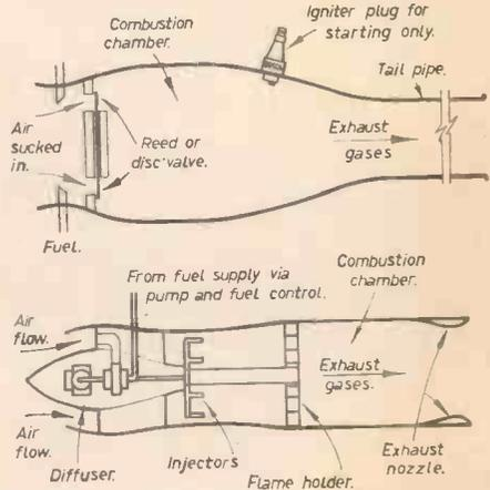
(Top) The pulse-jet. (Below) Details of the ram-jet.
