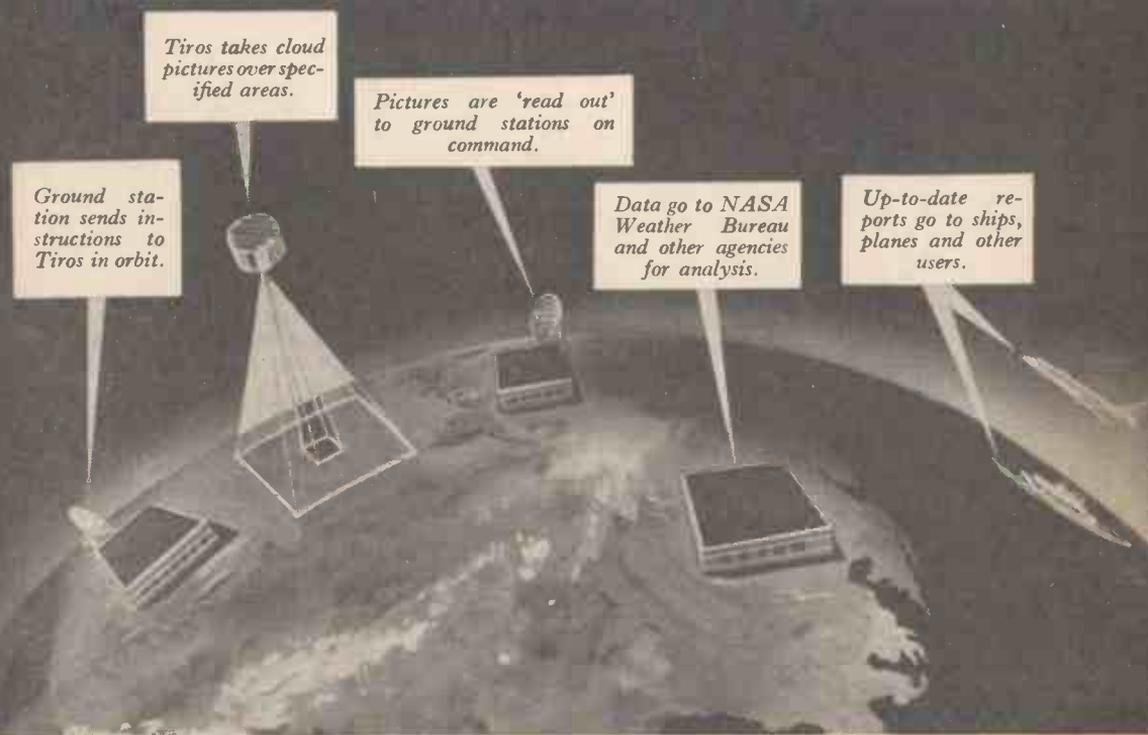
*The major orbital and ground elements of the Tiros II television-infrared weather observation system.*
