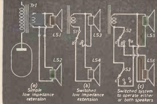
Fig. 157.—Various extension speaker systems.  $Tr_1$  is the transformer or valve output transformer. Loudspeakers 1, 3 and 5 are the original ones, 2, 4 and 6 are extensions.  $S_2$  and  $S_3$  are ganged.
