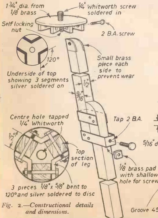
Fig. 2.—Constructional details and dimensions.
