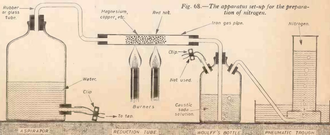
Fig. 68.—The apparatus set-up for the preparation of nitrogen.
