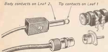
Fig. 154.—The special type of Post Office jack plug and socket used in many of the systems to be described. Also a co-axial plug and socket which is an alternative.
