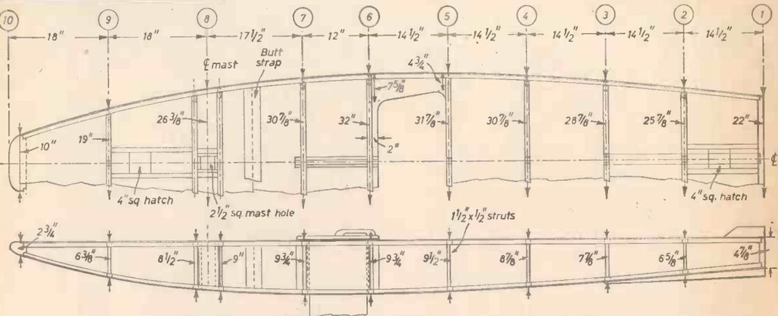
Fig. 5.—Plan and side elevation showing all framing, centre-board box and mast box.
