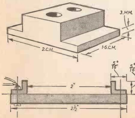
Fig. 5.—Battery panel with clips fitted.
