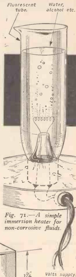
Fig. 71.—A simple immersion heater for non-corrosive fluids.
