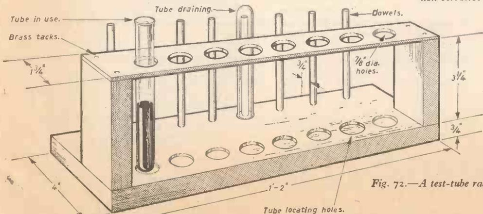
Fig. 72.—A test-tube rack.
