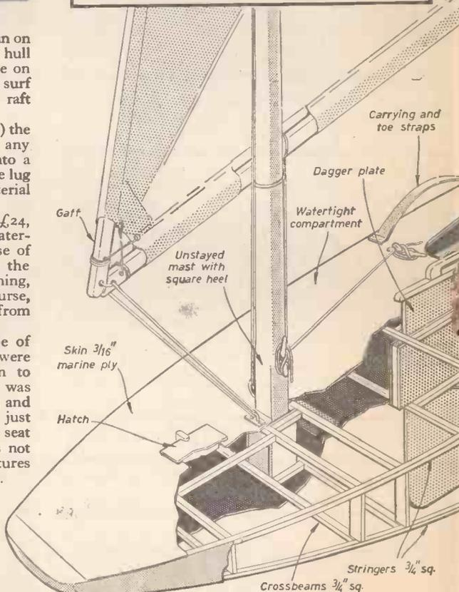
Fig. 1.—Cutaway perspective view showing general construction and rigging details.
