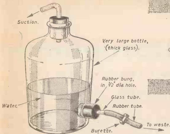
Fig. 69.—Details of the aspirator.
