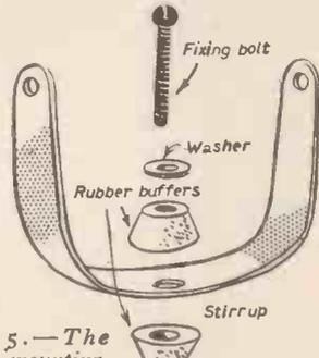
Fig. 5.—The stirrup mounting.
