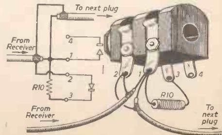
Inserting jack plug closes contacts 1 and 4, and opens 2 & 3
