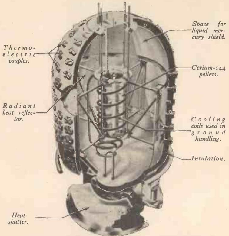
*A cutaway drawing of the SNAP 1-A atomic generator shows the outer thermocouple studded metal container and the device's inner construction. During the ground-handling prior to launching, the hollow interior of SNAP 1-A can be filled with liquid mercury, which acts as a radiation shield. The mercury would be drained out moments before lift-off to reduce weight.*
