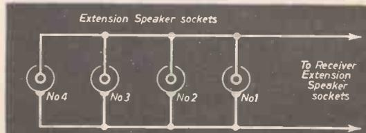
Fig. 158.—Four sockets wired in parallel for a simple system. Some precautions are necessary.
