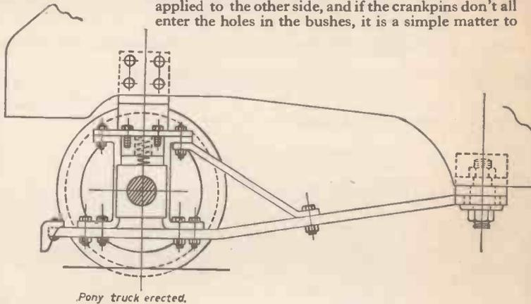
Fig. 25.—Side, plan and front views of the assembled pony truck.
