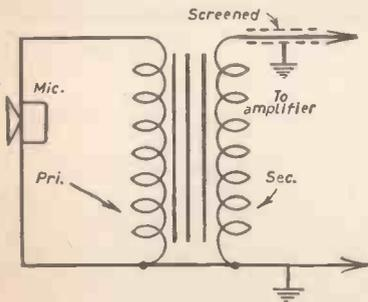
Fig. 4.—The transformer connections.
