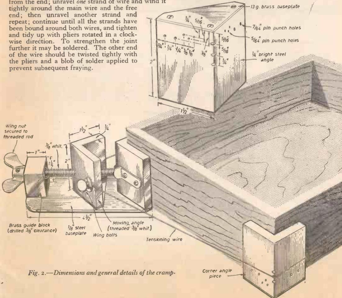
Fig. 2.—Dimensions and general details of the cramp.
