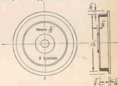
Fig. 30.—Wheel and axle.
