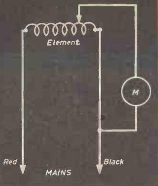
Fig. 7.—Circuit for low-voltage motor.
