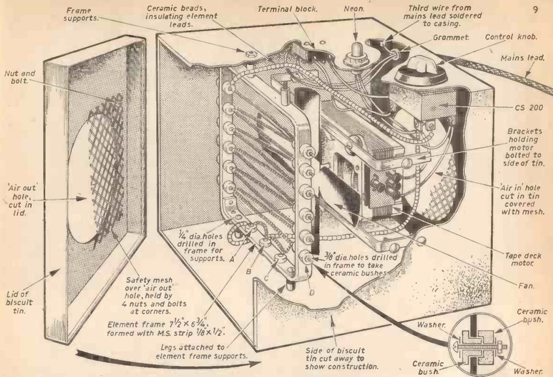
Fig. 4.—Cutaway perspective view of the complete heater.
