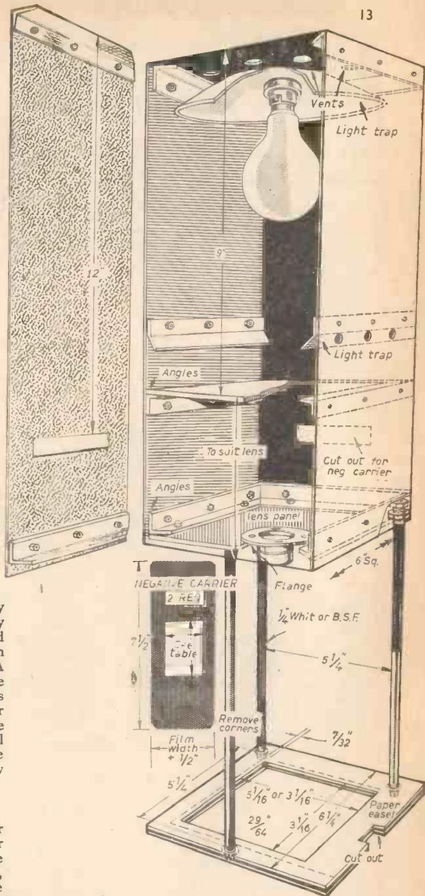
Fig. 2.—General arrangement and details of the enprinter together with dimensions.
