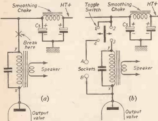
Fig. 2.—(a) Typical output circuit. (b) Modified output circuit.
