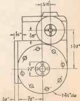
Fig. 47.—How to set up covers for finishing.
