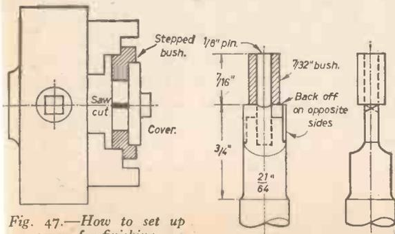
Fig. 48. (Left)—Special pin drill for piston lands.
