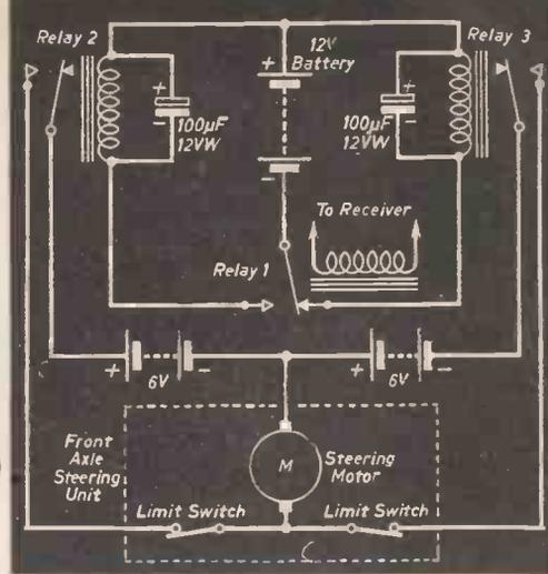
Fig. 11.—Steering motor circuit.
