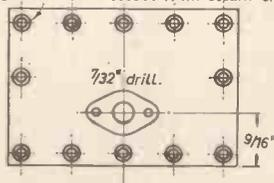
be set out as shown in Fig. 46, centrepopped, and drilled No. 34. Smooth off any burring by rubbing on a piece of emerycloth as mentioned for truing up the port face.
