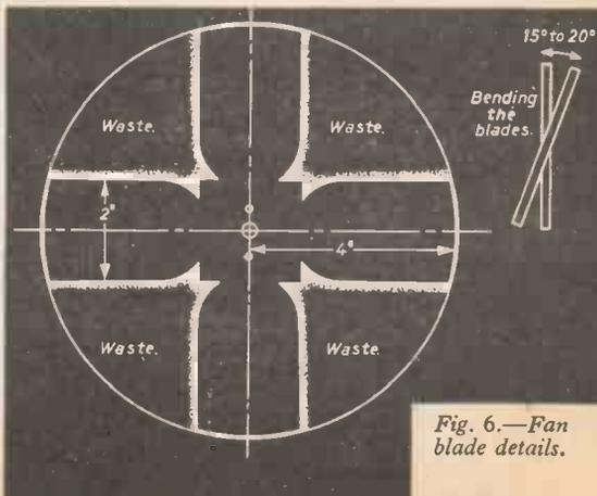
Fig. 6.—Fan blade details.
