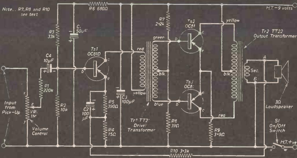
Fig. 5.—Amplifier circuit diagram. Experienced readers may prefer to use this instead of the wiring diagram.
