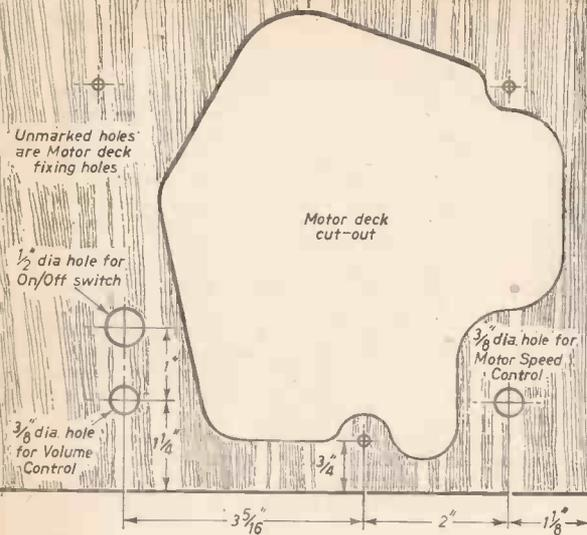
Fig. 3.—The cutaway portion and drilling positions of the motor board.
