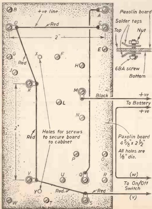
Fig. 6 (Left).—Underside wiring of the amplifier.
