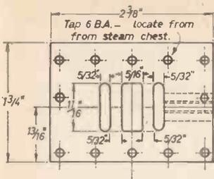
Fig. 44.—Cylinder port face.
