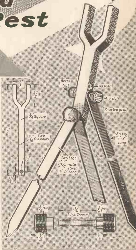
Measurements and constructional details of the rest.
