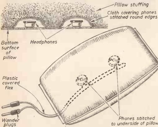
Fig. 1.—Installing the earphones.
