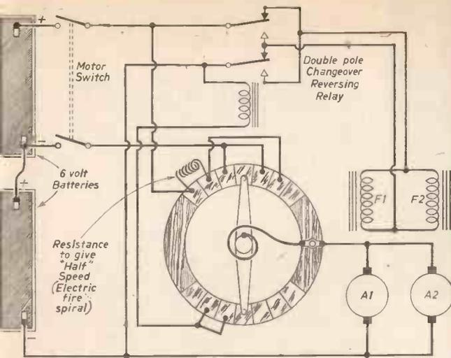
Fig. 9.—Connecting the speed control unit to batteries and motors. F = field and A = armatures.
