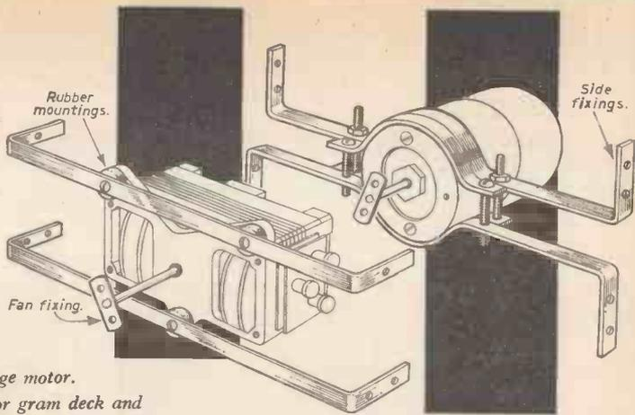
Fig. 8. (Right).—Mounting clamps for gram deck and round motors.
