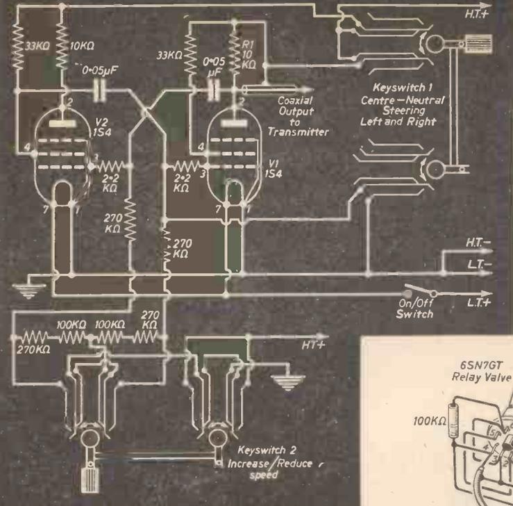
Fig. 15.—The multivibrator control box.
