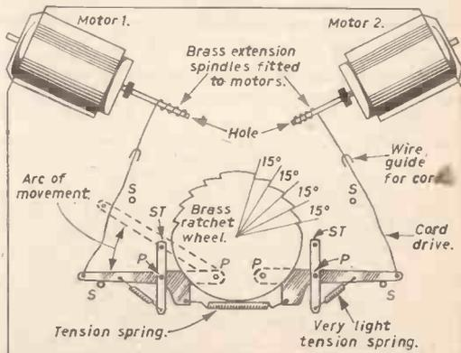
Fig. 7.—Engine speed control contact side. A = full speed ahead. B = half speed ahead. C = slow speed ahead. D = Stop. E = slow reverse. F = half reverse speed. G. = not used. Fig. 8.—(Right) Engine speed control drive side.
