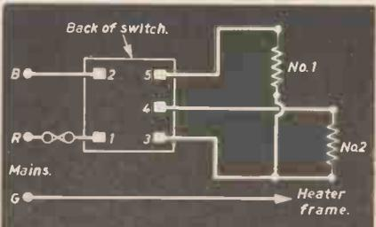
WIRING FOR 3 HEAT WITH 2 ELEMENTS.
