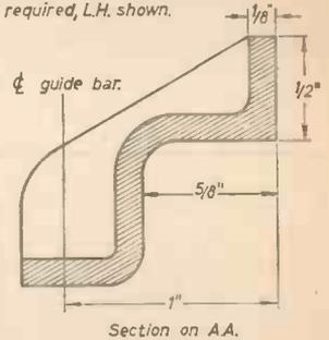
Fig. 62.—Three drawings giving details of the guide bar brackets.
