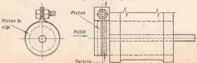
Fig. 60.—The packing pusher.
