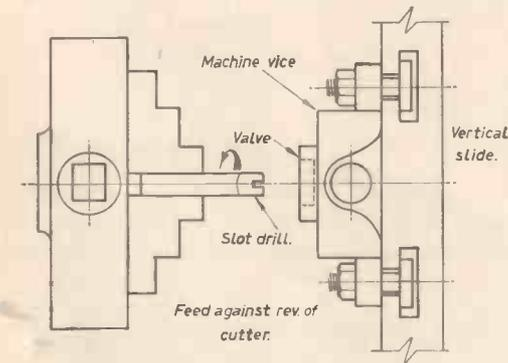
Fig. 58.—(Left) Slide-valve set up for cutting exhaust cavity.
