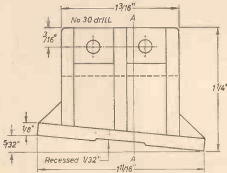
Fig. 61.—Guide bar details and measurements.
