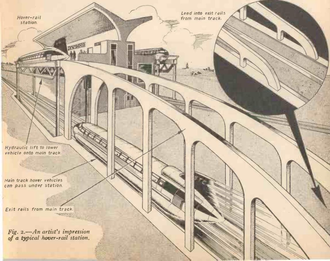
Fig. 2.—An artist's impression of a typical hover-rail station.
