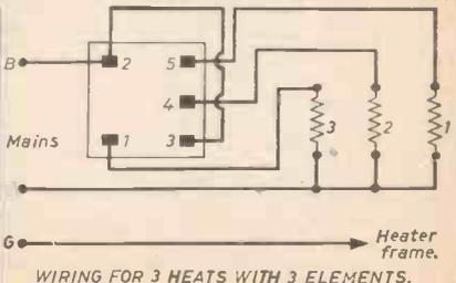
WIRING FOR 3 HEATS WITH 3 ELEMENTS.
