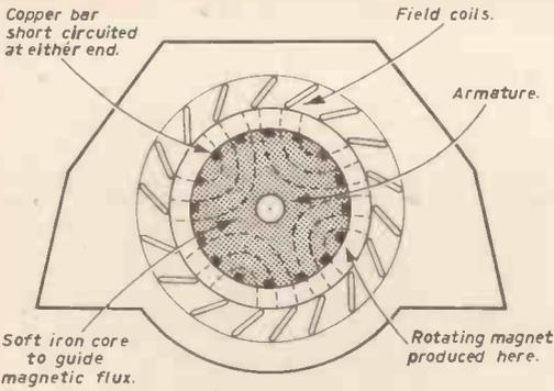
Fig. 3.—Conventional Induction motor showing armature, field coils, and method of rotation.
