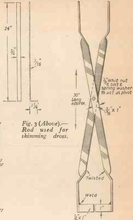
Fig. 3 (Above).—Rod used for skimming dross.
