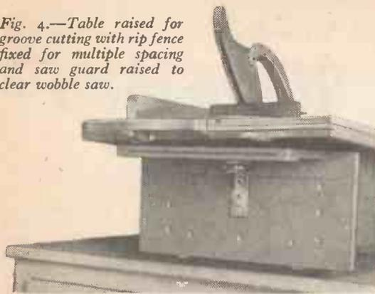
within reason, but it must be remembered that the position of the two  $\frac{3}{16}$  in. clearance holes in the brackets must allow the back of the wheel to clear the face of the rear bracket. Fig. 4 shows the mechanism in use, the saw blade projecting only  $\frac{1}{16}$  in., and Fig. 2 shows it completely unthreaded in order to "get at the works" for changing saws and clearing sawdust.
