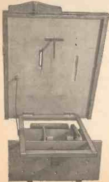
Fig. 2.—Table completely raised for saw changing. Note enlarged hole for wobble saw and indent for belt clearance.
