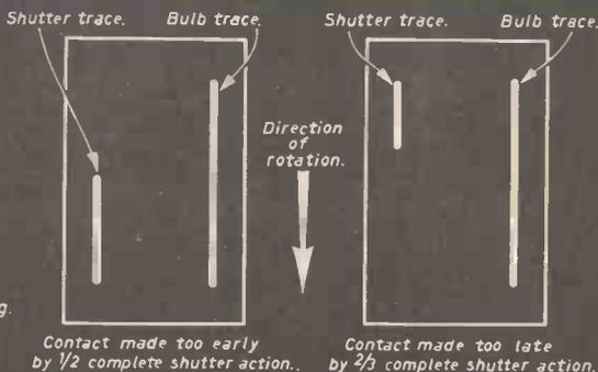
FIG. 3. LINES PRODUCED BY EARLY AND LATE FIRING
