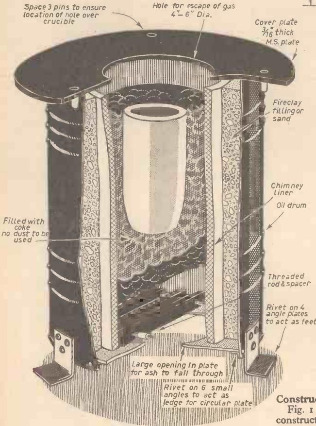
Fig. 1.—This cross section view shows how a lining is made and the method adopted for holding the lower fire bar plate.
