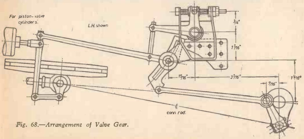
Fig. 68.—Arrangement of Valve Gear.
