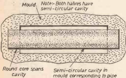
Fig. 6.—Plan of the mould for the pipe shown in Fig. 5.
