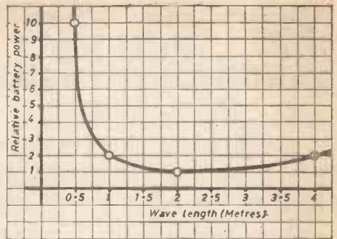
Fig. 5.—Chart showing battery power required in the satellite for various wavelengths.
