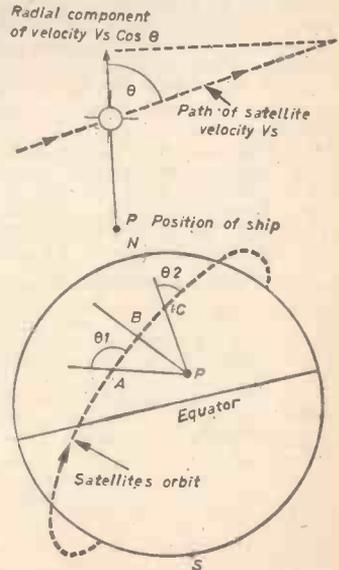
Fig. 3. (Right) — Determination of ship's position.
