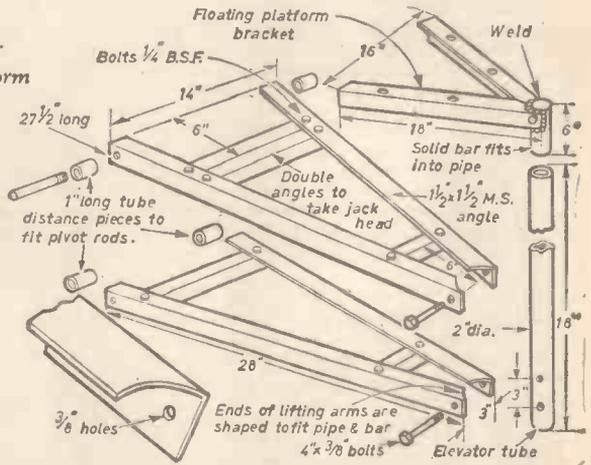
The elevator tube is an 18 in. length of 2 in. dia. pipe drilled with ¼ in. holes at 3 in. centres to accommodate the cross bolts of the lifting arms. With the jack in position, the tube should rise and fall vertically from floor level to maximum height. Adjust the screw neck of the jack piston to give contact with the angles of the upper arm when the piston is at lowest stroke.
