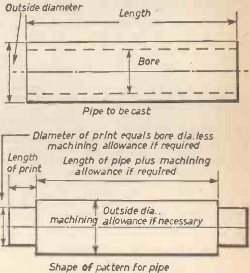
Fig. 5.—Details of casting hollow articles.
