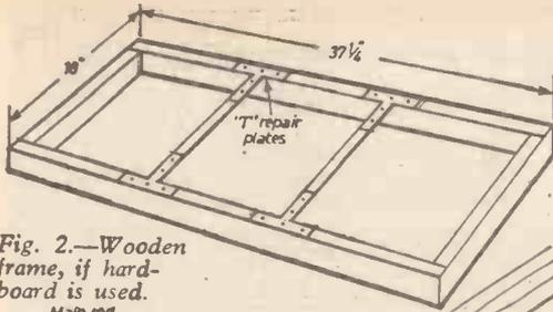
Fig. 2.—Wooden frame, if hard-board is used.
