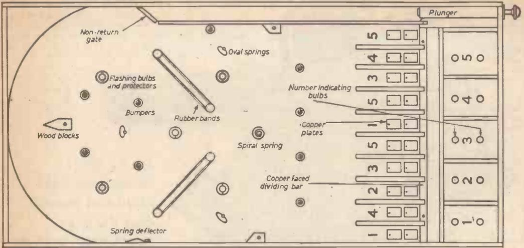
Fig. 7.—Plan of the lay-out of hazards, etc.
