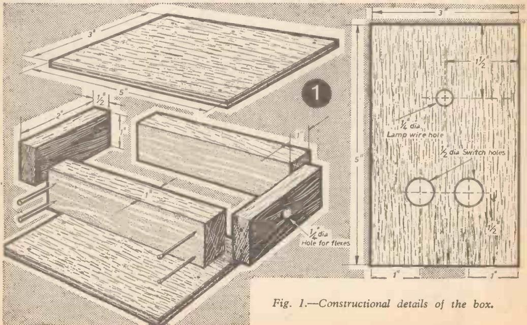
Fig. 1.—Constructional details of the box.
