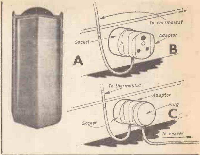
Fig. 5. (Above) —(a) the adaptastat; (b) first plugging operation; (c) second plugging operation.
