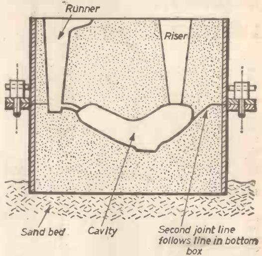
Fig. 7.—Moulding irregular shaped articles.
