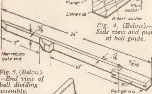
Fig. 4. (Below).—Side view and plan of ball guide.
