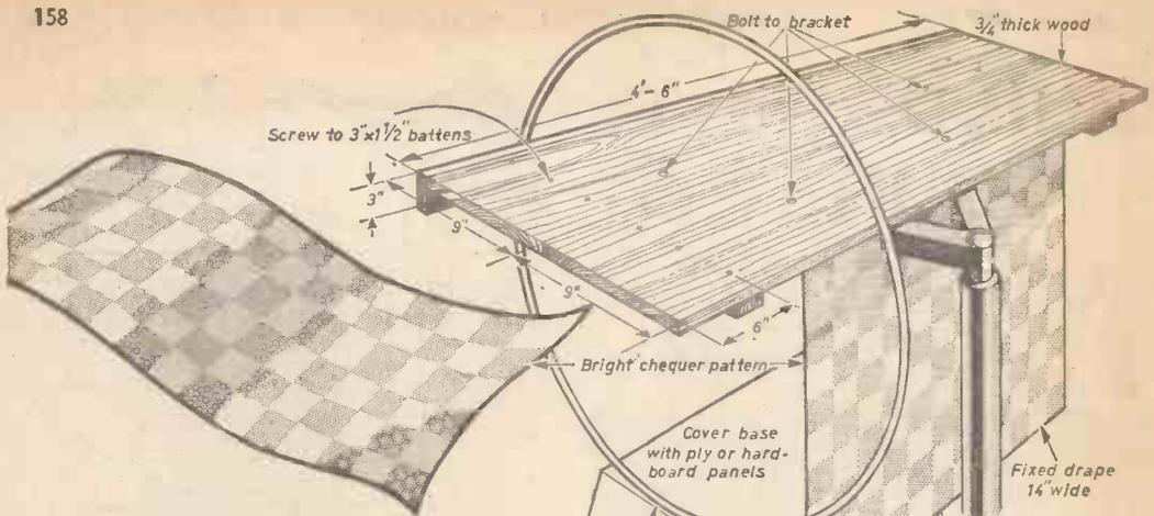
Fig. 7.—Making the platform and drapes and passing hoop over girl.
