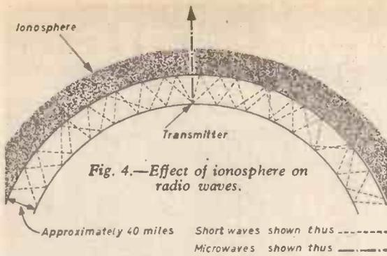
Fig. 4.—Effect of ionosphere on radio waves.
