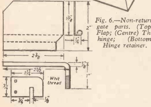
Fig. 6.—Non-return gate parts. (Top) Flap; (Centre) The hinge; (Bottom) Hinge retainer.
