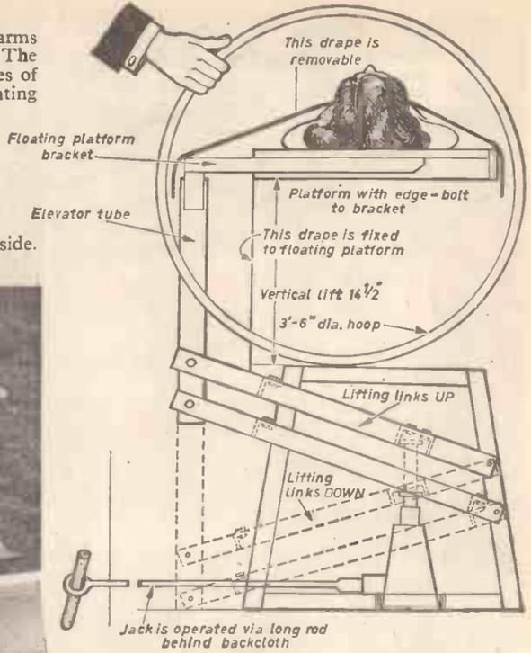
Fig. 5.—(Above) End view of assembled illusion.
