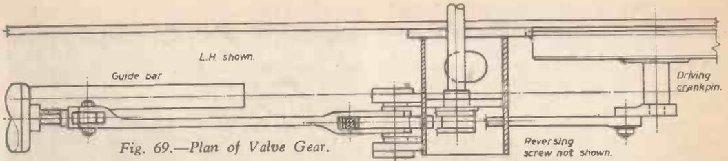
Fig. 69.—Plan of Valve Gear.
