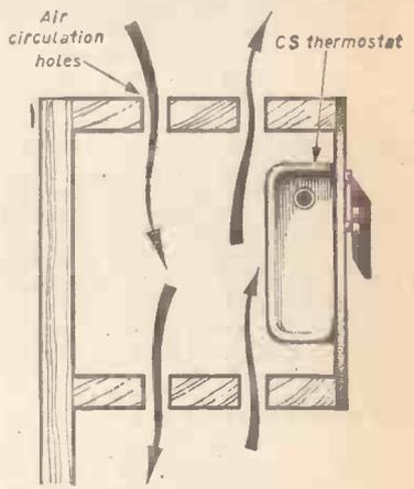
Fig. 4. (Right)—Shelf mounting the CS thermostat.
