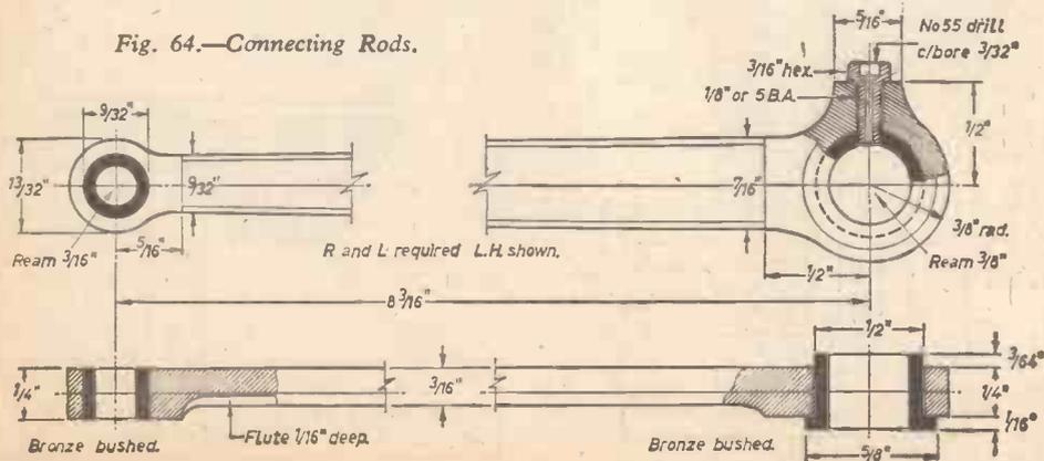
in Fig. 64. Note that it projects through  $\frac{3}{4}$  in. and forms a distance-piece between the coupling-rod boss and the big-end. The projection which represents the full-size oil box is drilled No. 40, tapped  $\frac{1}{4}$  in. or 5B.A. and furnished with a hexagon-headed brass screw, drilled through No. 55, the head being counterbored  $\frac{3}{8}$  in. This screw runs right into the big-end bush as shown in Fig. 64.
