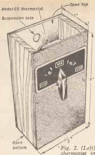
Fig. 2. (Left)—CS thermostat in box mounting.
