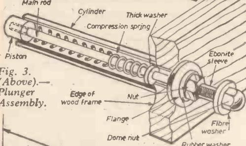
Fig. 3. (Above).—Plunger Assembly.
