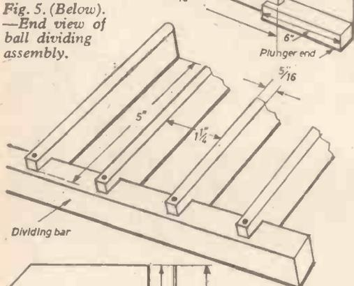
Fig. 5. (Below).—End view of ball dividing assembly.
