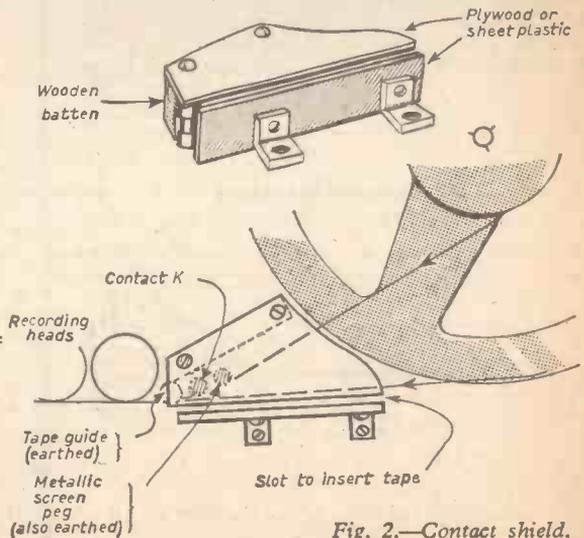
Fig. 2.—Contact shield.
