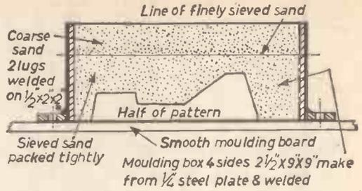
Fig. 1.—First stage in the preparation of a mould.
