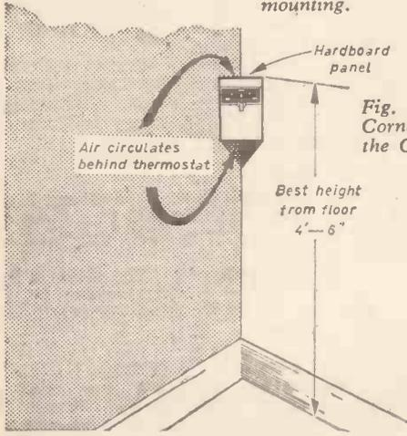
Fig. 3. (Left)—Corner mounting the CS thermostat.
