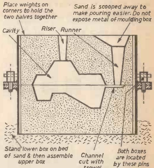
Fig. 4.—The mould finally assembled ready for pouring.
