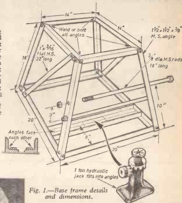
Fig. 1.—Base frame details and dimensions.
