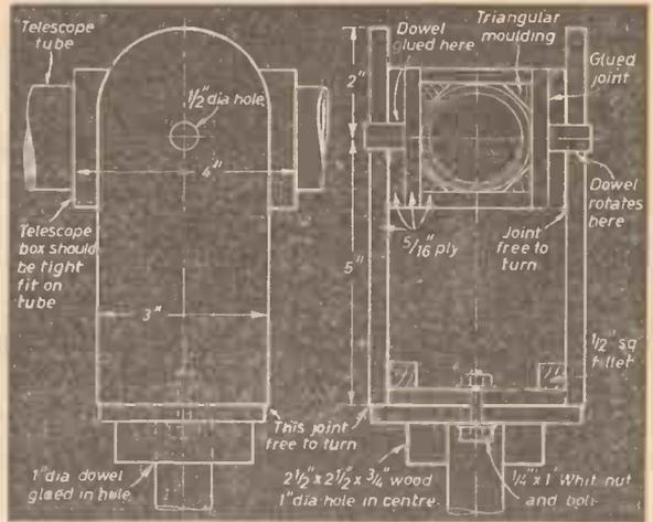
Fig. 3.—Side and plan view of the Stand.
