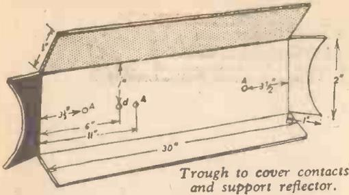
Trough to cover contacts and support reflector.
