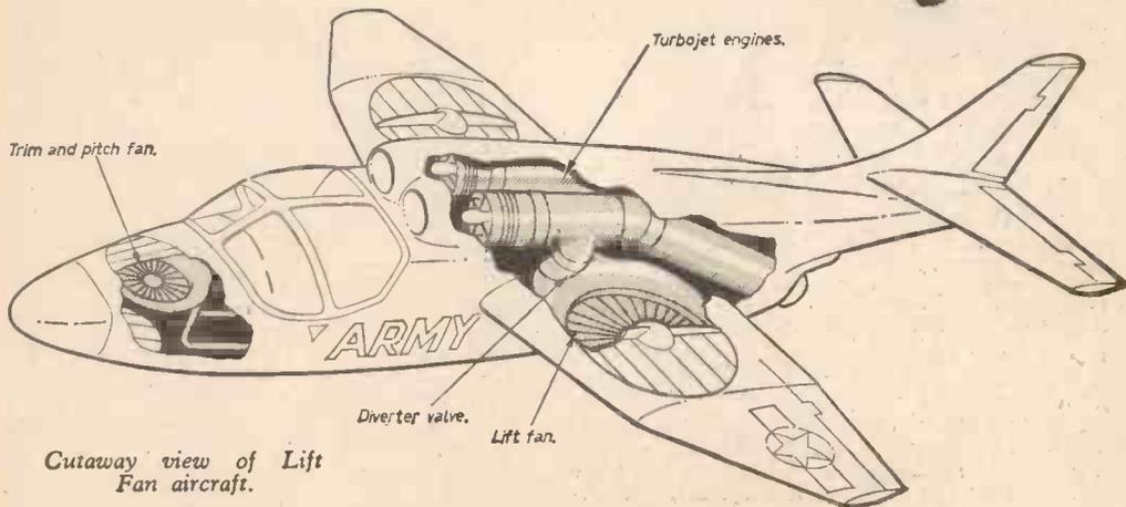
Cutaway view of Lift Fan aircraft.
