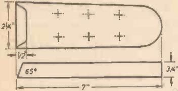
Fig. 4.—Details of the head.
