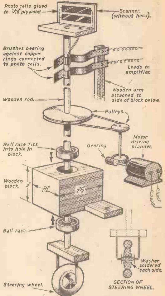
Fig. 2.—Front block details.
