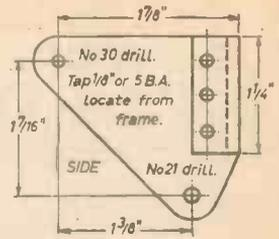
back end of the bracket after bending, so that both sides line up. Attach the completed bracket to the stay by six  $\frac{1}{8}$  in. iron rivets, as shown in the two arrangement drawings, Fig. 117.
