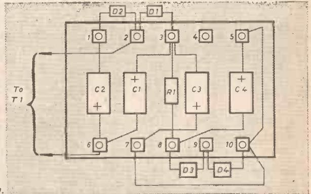
Fig. 1.—Circuit diagram of Power Supply.
