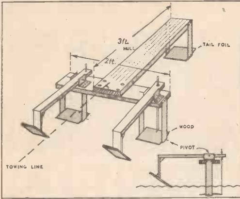
This highly simplified model can be built in a few hours and when towed at some 8-10 m.p.h. will demonstrate the remarkable stability and seaworthiness of an incidence control system. It will negotiate waves of 5ft high with ease.
