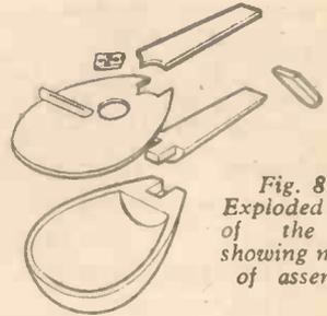
Fig. 8.—Exploded view of the lute showing method of assembly.
