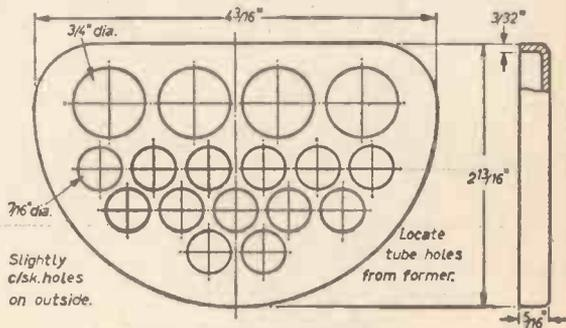
COMBUSTION CHAMBER TUBEPLATE.
