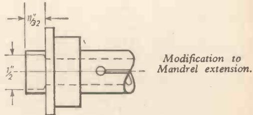
Open out 3/8" bore at wheel end to 1/2" dia. x 11/32" or 3/8" deep to take washer
