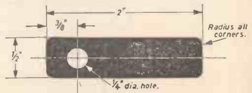
Fig. 2.—The connecting plate.
