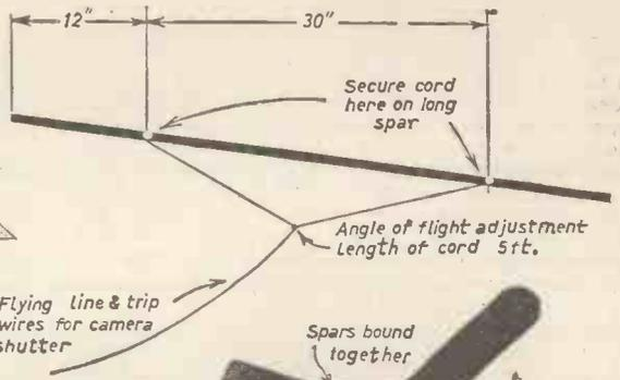
Flying line & trip wires for camera shutter
