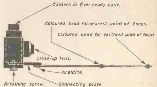
Fig. 1.—The device attached to the camera.
