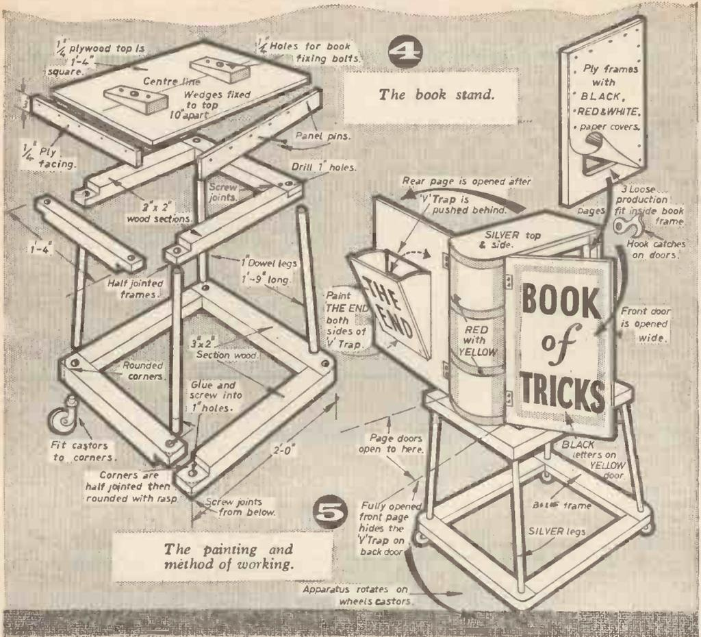
Drill the bolt holes through the ply platform then temporarily support the book in place and mark and drill the holes for the fixing bolts in the frame. After drilling, the book is mounted with two 3in. long coachbolts with the wingnuts underneath. Tack decorative ply facings round the platform edge.
