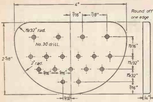
FORMER AND TUBE-DRILLING JIG FOR COMBUSTION CHAMBER TUBEPLATE.
