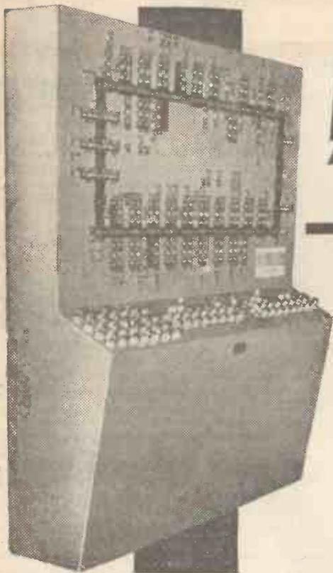
*Control console of the 76-station transfer machine described in the article.*
