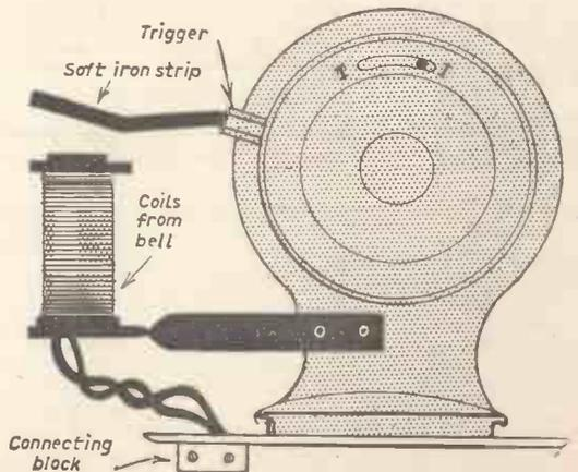
the small piece of metal that holds them together on the metal frame, and the armature. The camera to be used for the aerial photograph governs the position in which the tripping unit should be mounted. In the writer's prototype, the camera used was an old "Coronet" that had seen many good sights at ground level, and was considered by modern standards as being "out of date".
