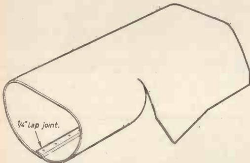
FIREBOX AND COMBUSTION CHAMBER AFTER BENDING.
