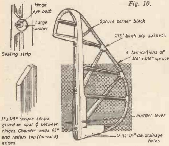
Fig. 10.—General arrangement of the rudder.
