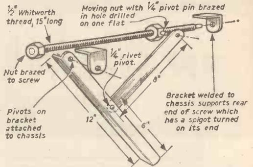
To operate the trailer leg mechanism the screw is turned with a wheel brace. The moving nut thus travels along the screw and the leg is raised or lowered. With such a leg at each corner it is possible to support the trailer firmly in a level position on any uneven ground.
