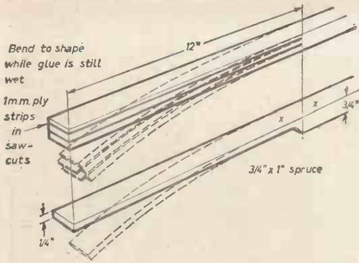
Fig. 6.—Two methods of shaping the tailplane rear spar boom ends.
