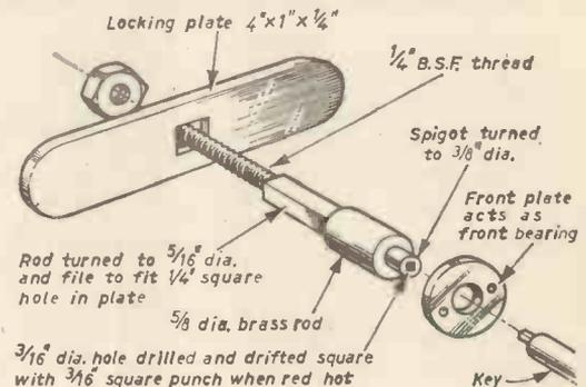
Exploded view of door lock mechanism, to be set in rail dividing the two doors. The plate fits into a recess in each door when turned by a square key. The smaller the square key hole, the more difficult is the lock to pick.
