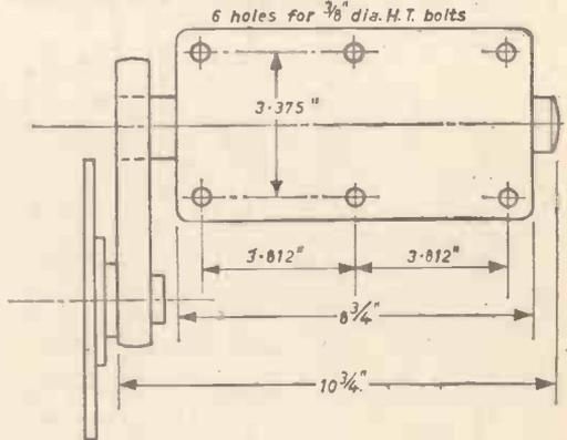
Plan view of a Flexitor unit without wheel. Attach to cross members with G-cramps so that the wheel "toes in" correctly then drill fixing holes to suit. Toe in from wheel rim to trailer centre line should be 1/8in. for 8-10in. wheels, 3/16in. for 12-13in. wheels and 1/4in. for 16in. wheels.
