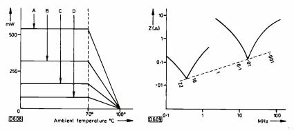
Fig. 2 (left): Maximum permissible power dissipation for various capacitor body sizes. A 15-5mm thick, 27-5mm pitch; B 11mm thick, 22-5mm pitch; C 8-5mm thick, 15mm pitch; D 4-5mm thick, 10mm pitch.
