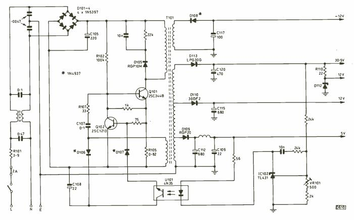
Fig. 1: The power supply circuit used in the Wyse WY120 terminal unit.
