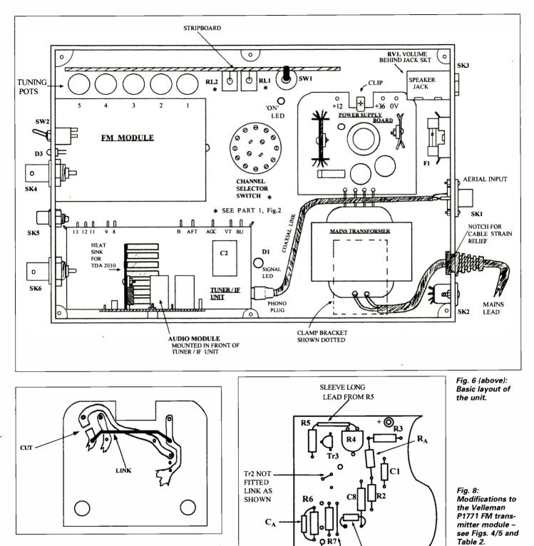
Fig. 7: The cut-and-link modification on the print side of the power supply PCB.
