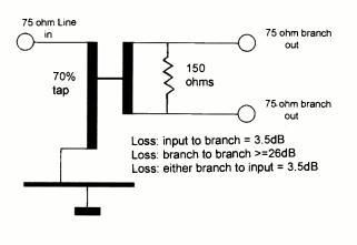
Fig. 3: A two-way equal splitter circuit.
