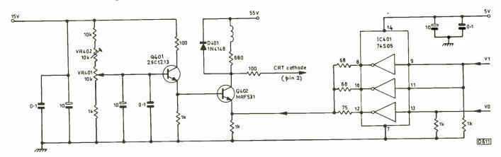
Fig. 2: The video drive circuit. The 55V supply for Q402 is obtained from D205 (RGP5100) and C217 (10µF) in the line output stage.
