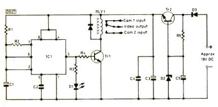
Fig. 1: Circuit diagram of the scart switcher unit. The video inputs and the output (flying lead) are all connected to pin 20 of the relevant scart connector.
