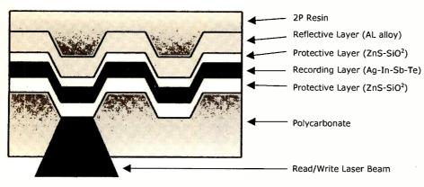
Fig. 1: Structure of a DVD-RW disc.
