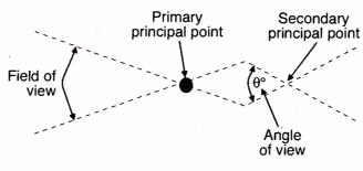
Fig. 3. Relationship between the angle view and the field of view.
