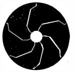
Fig. 4. Sliding plates perform the function of a mechanical iris.
