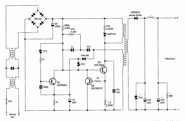
Fig. 1: Circuit diagram of the Olivetti LT7-700005-06 AC adaptor. This type of circuit is widely used in small PCs and AC adaptors.
