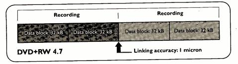
Fig. 6: Lossy and lossless linking.
