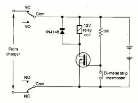
Fig. 4: Relay circuit to switch off the charger.
