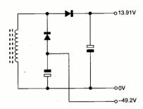
Fig. 2: Negative rectifier circuit added temporarily to measure the peak flyback voltage.
