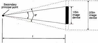
Fig. 2. Angle of view (q) changes for different format size lens/image device.
