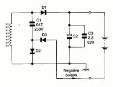
Fig. 3: Modifications to the secondary side of the switch-mode power supply to provide pulse charging.
