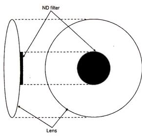
Fig. 12. Principle of the neutraldensity spot filter.
