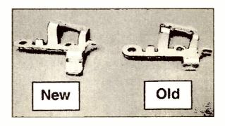
Fig. 3: The new and old cylinder mounting plates used in VCR Models V229B, V429B, V709B and V729B.
