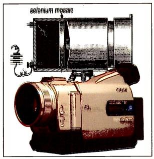
Fig. 3. Ayrton & Perry in the UK and Carey in the USA proposed imaging systems using arrays of selenium photocells. Although 120 years of technological development separate today's digital camcorder from Carey's 1880 scheme, they both employ the same principle of using imaging arrays for the camera.
