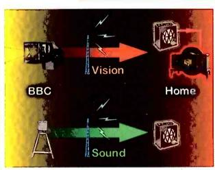
Fig. 6. The BBC's first Television Service opened in 1932 with Baird's 30-line system, which was by then mature. With the vision signal so low in bandwidth that it could be treated like audio, the BBC Television Service only needed a camera in the studio, a spare medium-wave transmitter, an extra radio set in the home and a display adaptor – the Baird Televisor. The 30-line system's major benefit was that no new equipment or technology had to be developed.
