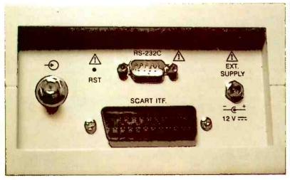
Photo 1: The connectors at the side of the meter.
