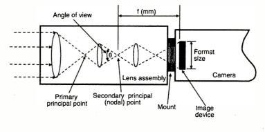
Fig. 1. Shows a simple fixed lens illustrating the main features of CCTV lens systems.
