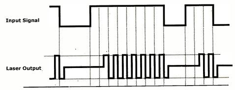
Fig. 3: Comparison between the input data signal and laser output for recording.
