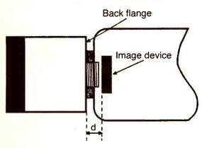
Fig. 7. For a C mount, d is 17.5mm while for a CS mount, d is 12.5mm.
