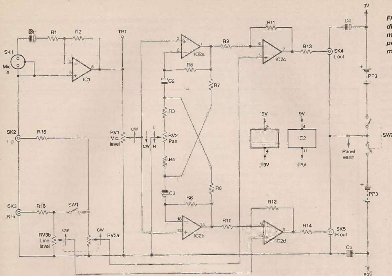
Fig. 1: Circuit diagram of the microphone preamplifier/mixer unit.
