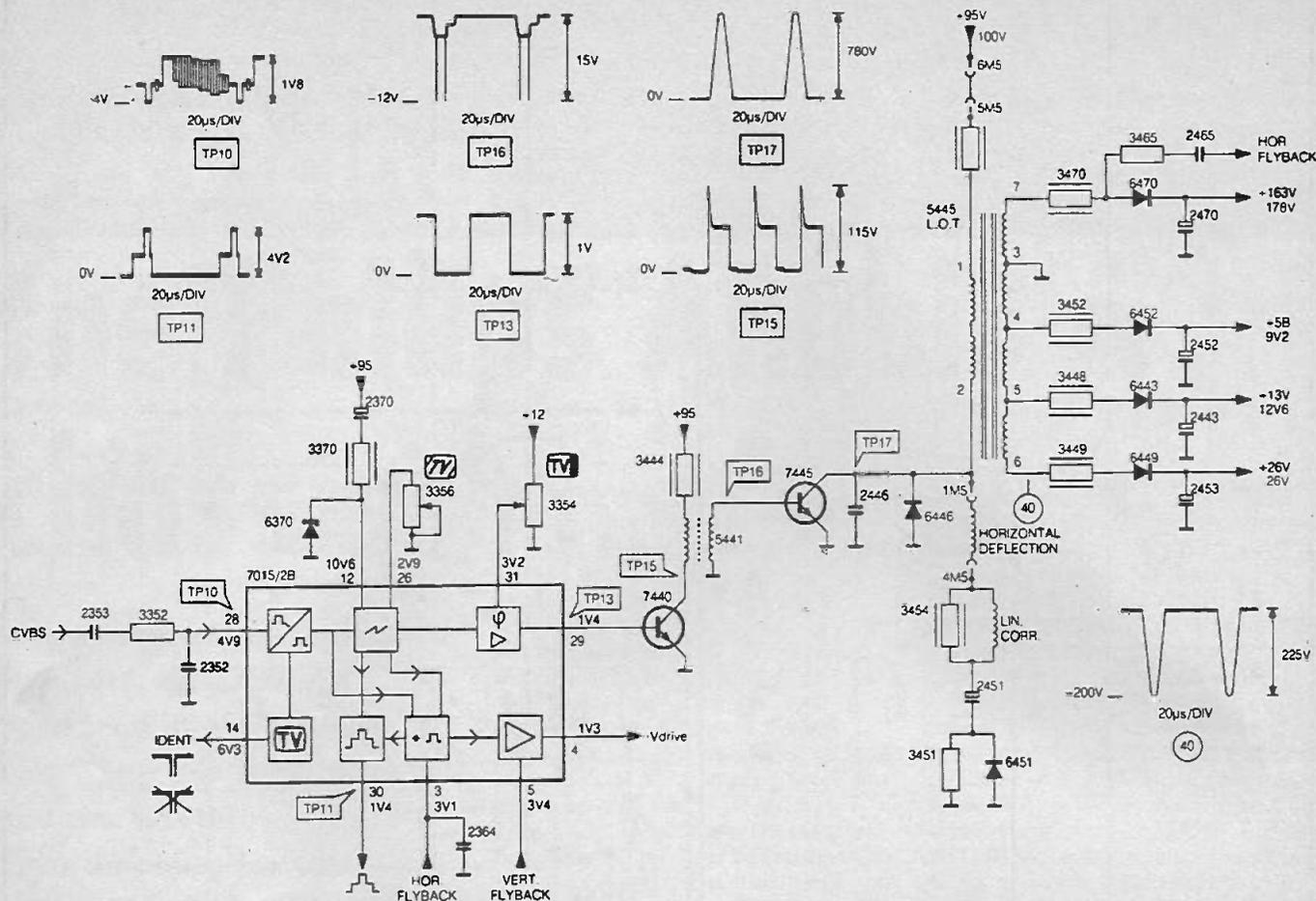
Fig. 2: Basic circuit, much simplified, of the line timebase. IC7015 contains both the line and field generators, with line drive output at pin 29 and field drive output at pin 4. It also contains the IF strip. Illustration courtesy of Philips Service.
