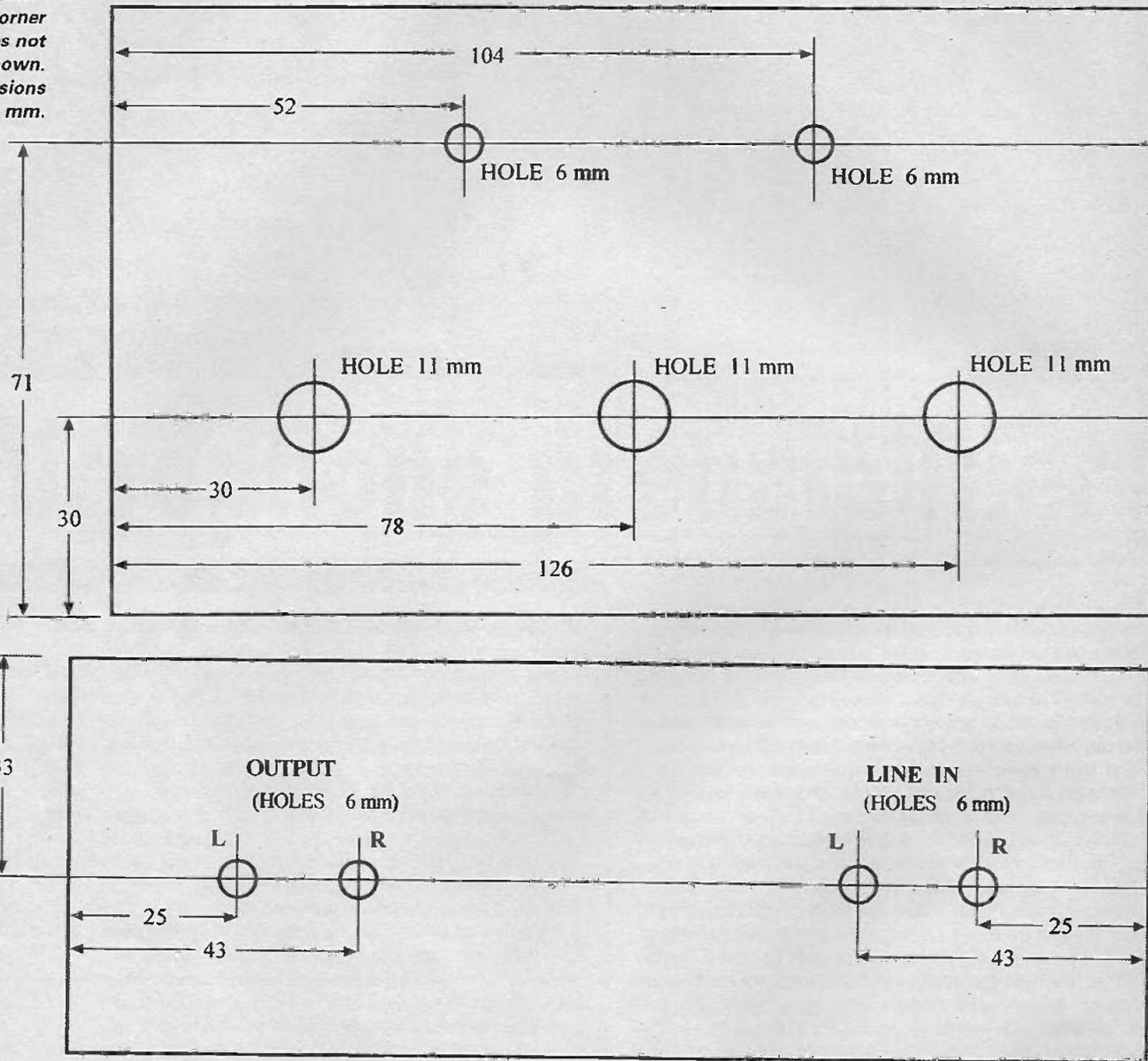
Fig. 3: Case drilling details, (a) rear sockets, (b) mic. input socket at the right-hand side. Dimensions in mm.
