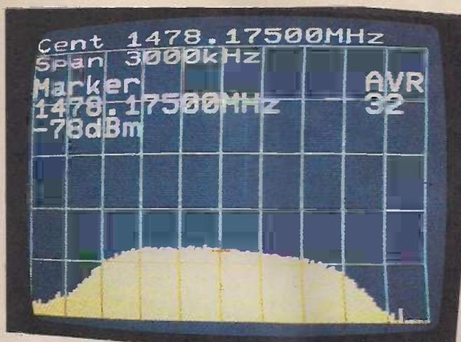
**Photo 1:** Afristar beam 1 spectrum for right-hand polarised signals. To take this photograph the signals from the aerial were split between the receiver and a signal analyser. Photo taken in Portugal.
