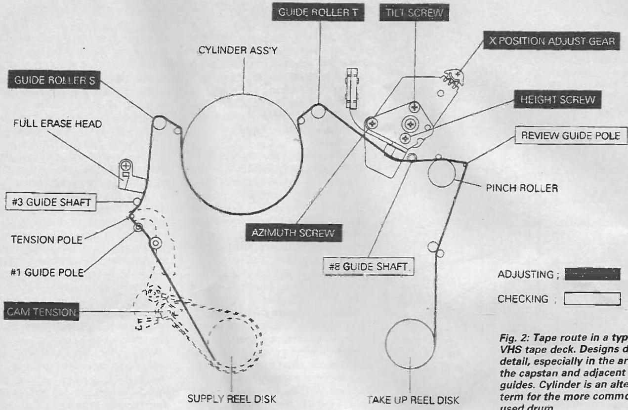
**Fig. 2: Tape route in a typical VHS tape deck. Designs differ in detail, especially in the area of the capstan and adjacent tape guides. Cylinder is an alternative term for the more commonly-used drum.**
