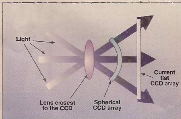
A spherical CCD photosensor enables the lens system to be greatly simplified.
