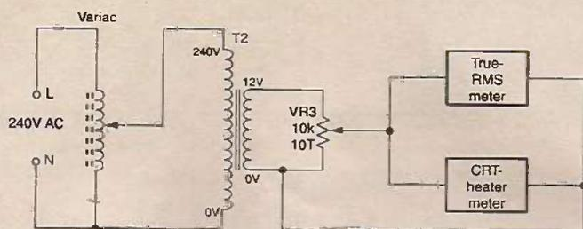
Fig. 2: Calibration set-up.
