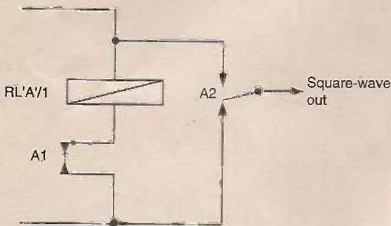
**Fig. 5. Not far removed from the simple buzzer circuit,** this one produces a square wave whose amplitude is equal to the supply voltage.
