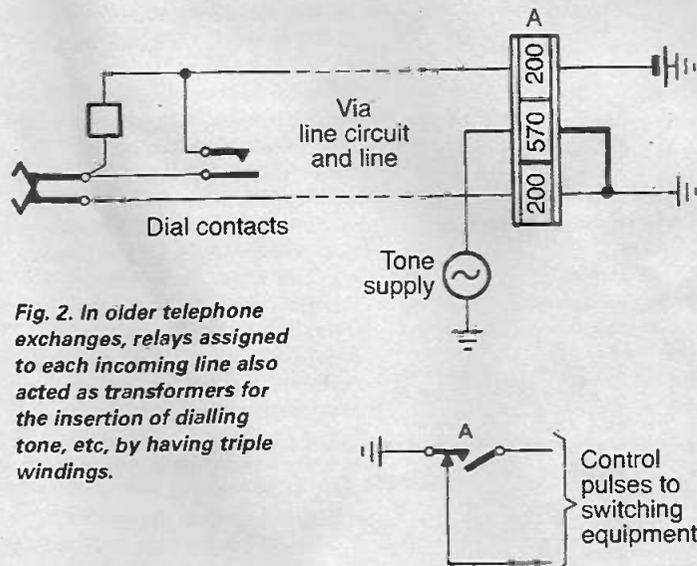
Fig. 2. In older telephone exchanges, relays assigned to each incoming line also acted as transformers for the insertion of dialling tone, etc, by having triple windings.
