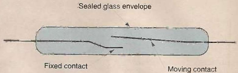
**Fig. 7. Not strictly a relay, the hermetically sealed reed switch is suitable for low power applications.** It can be activated by a magnet or by a coil – in which case it becomes a relay.
