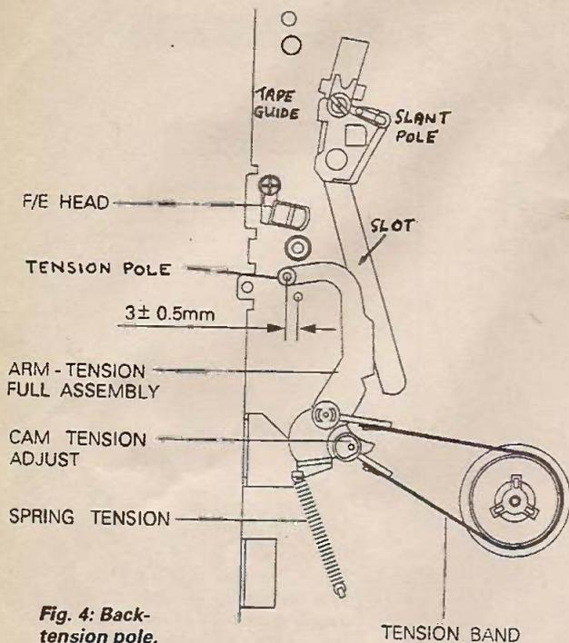
**Fig. 4: Back-tension pole, band and setting arrangement (cam tension adjust). Note the setting indication by the pole.**
