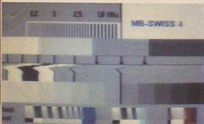
has insufficient torque to overcome the tape friction around the drum wrap while the capstan continues to feed tape to the 'sticky' drum. In such a case cleaning and polishing the lower drum can be tried, but probably won't help. The cure, a new lower drum assembly, is expensive.
