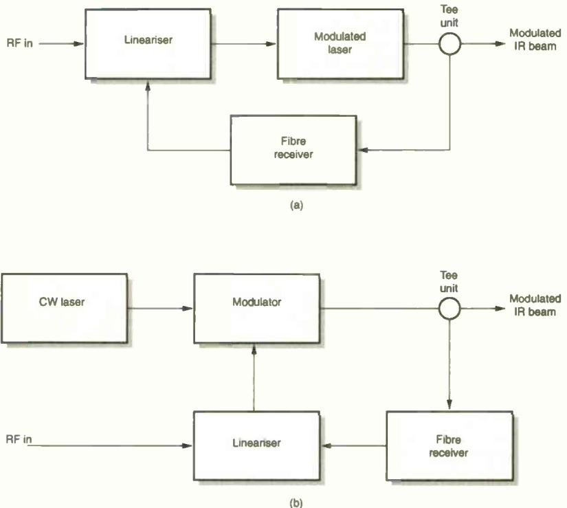
Fig. 2: Block diagrams of the two main types of laser transmitter, (a) DFB laser and (b) YAG laser.
