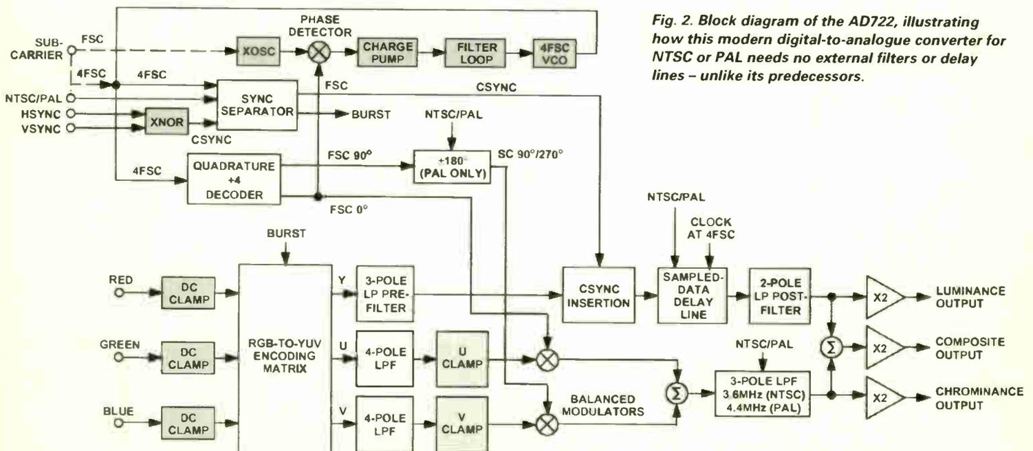
Fig. 2. Block diagram of the AD722, illustrating how this modern digital-to-analogue converter for NTSC or PAL needs no external filters or delay lines – unlike its predecessors.
