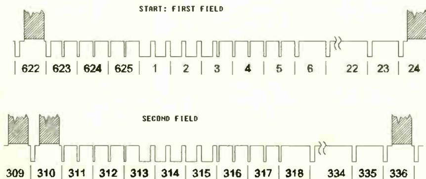
Fig. 1. PAL interlaced waveforms for each field.
