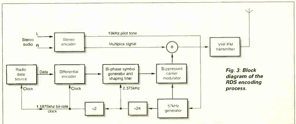
Fig. 3: Block diagram of the RDS encoding process.
