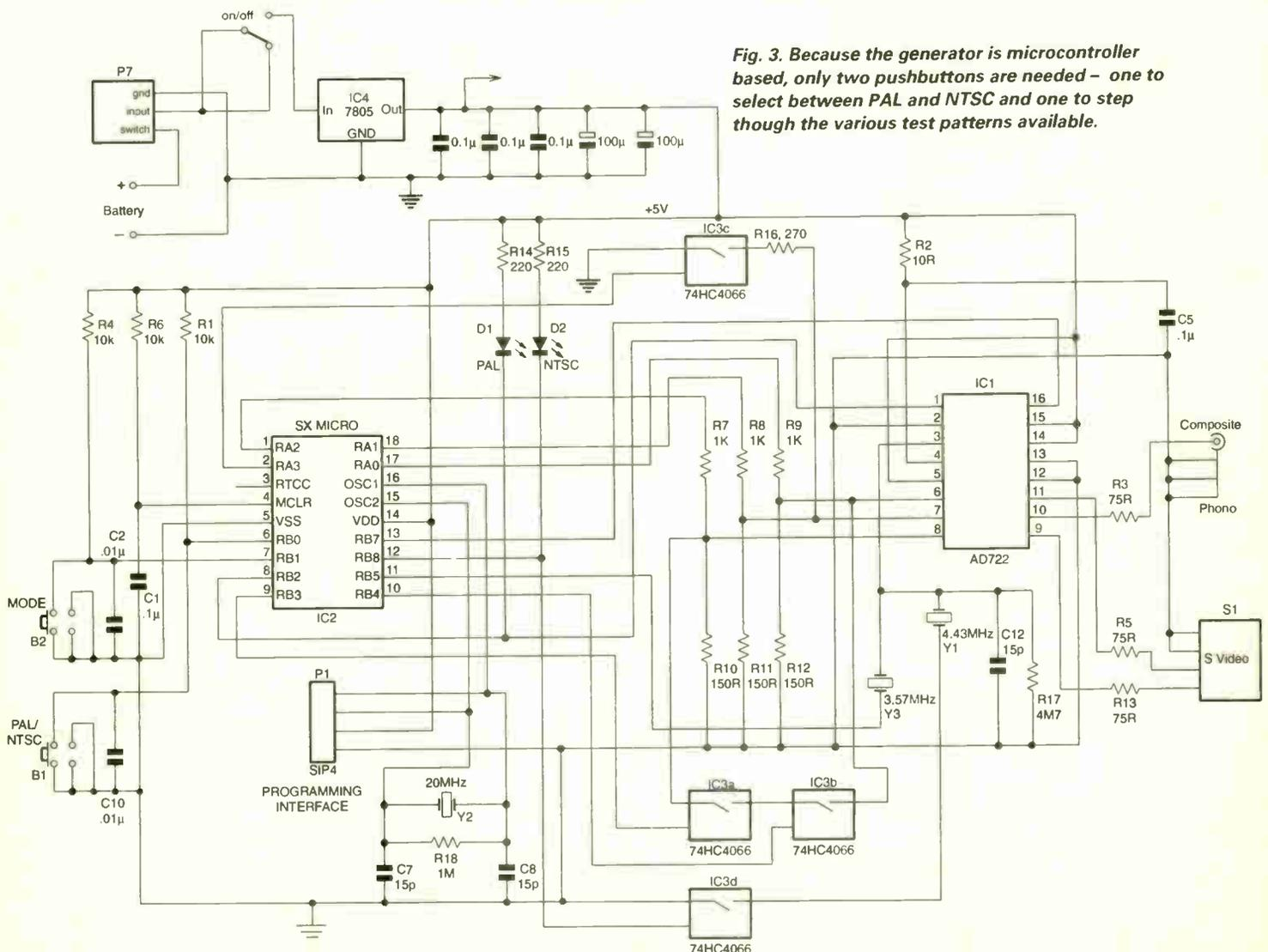
Fig. 3. Because the generator is microcontroller based, only two pushbuttons are needed – one to select between PAL and NTSC and one to step through the various test patterns available.
