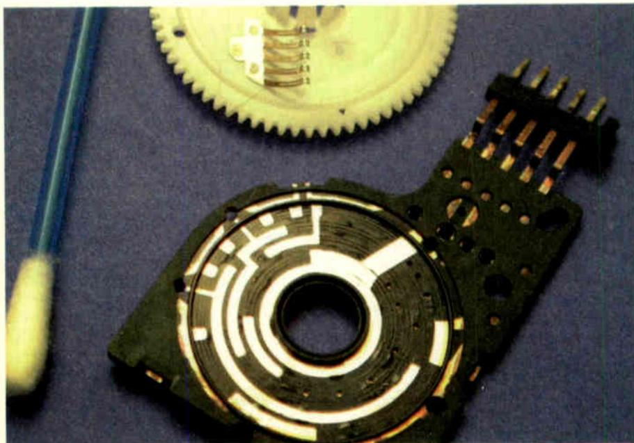
Fig. 1: Inside a typical rotary mode switch.
