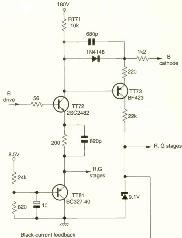
Fig. 8: RGB output stage circuitry, seven-transistor version.
