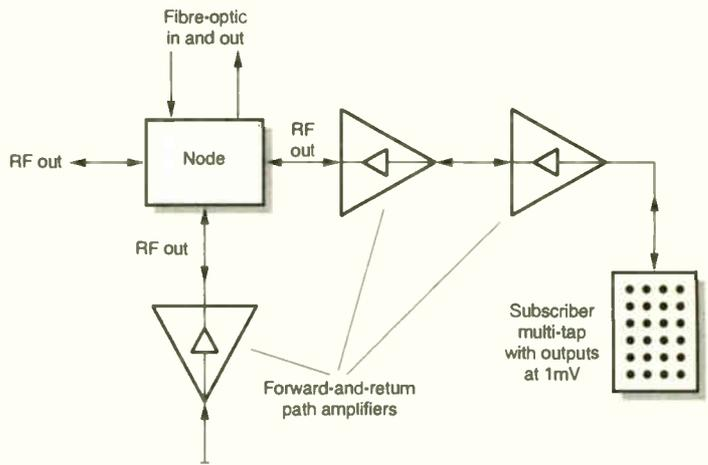
**Fig. 5: Typical HFC network.**
